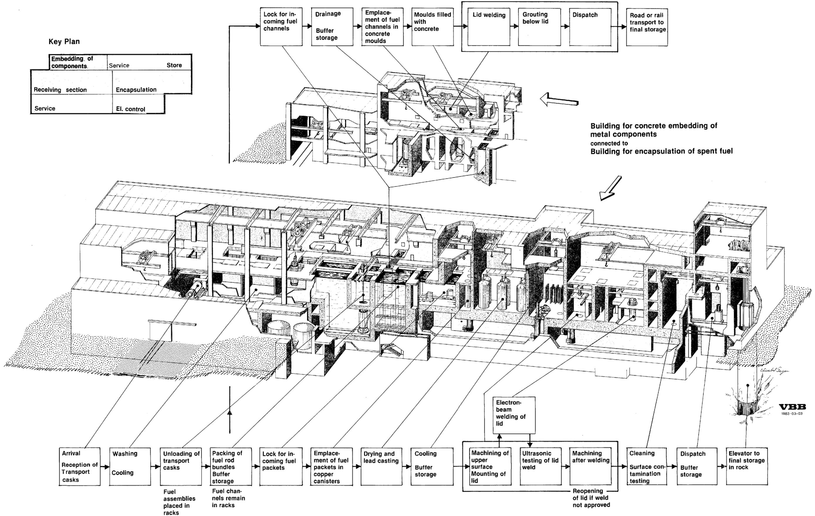
Fig 2. Encapsulation station with process scheme.
