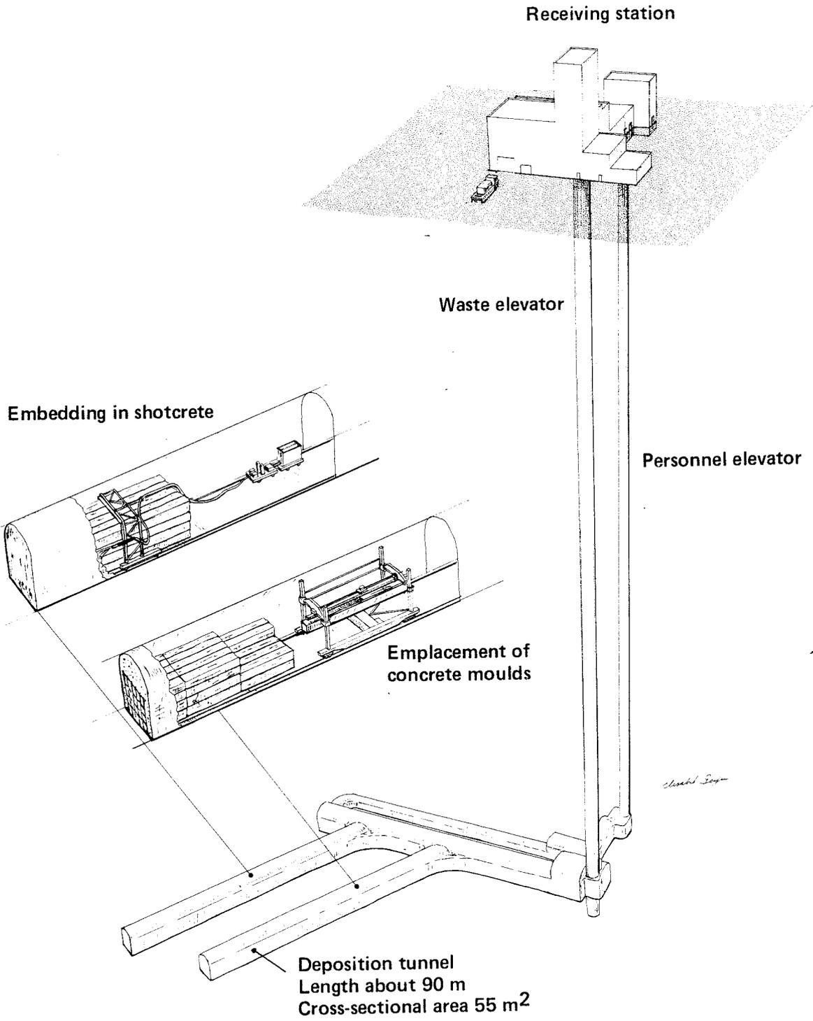
Fig 6. Final repository of fuel box containers
