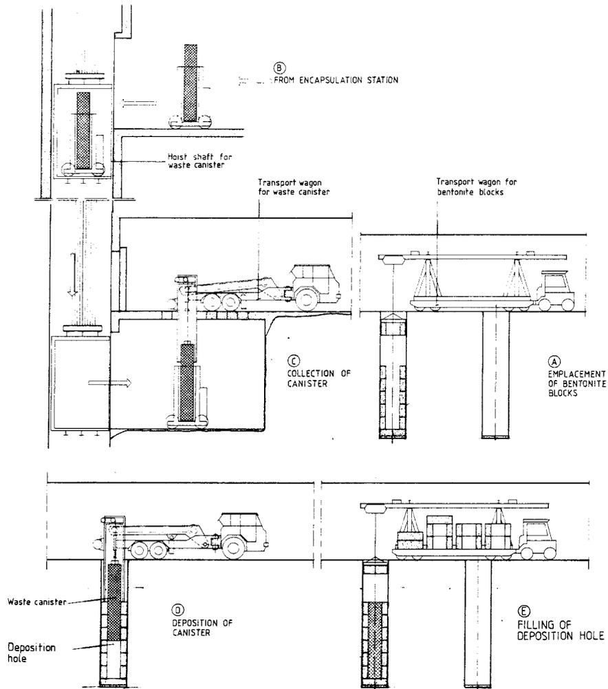
Fig 5. Transport of canisters to final repository
