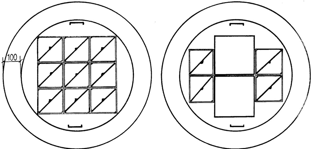
Fig 3. Canister with 9 BWR- or 2 PWR- and 4 BWR-elements
