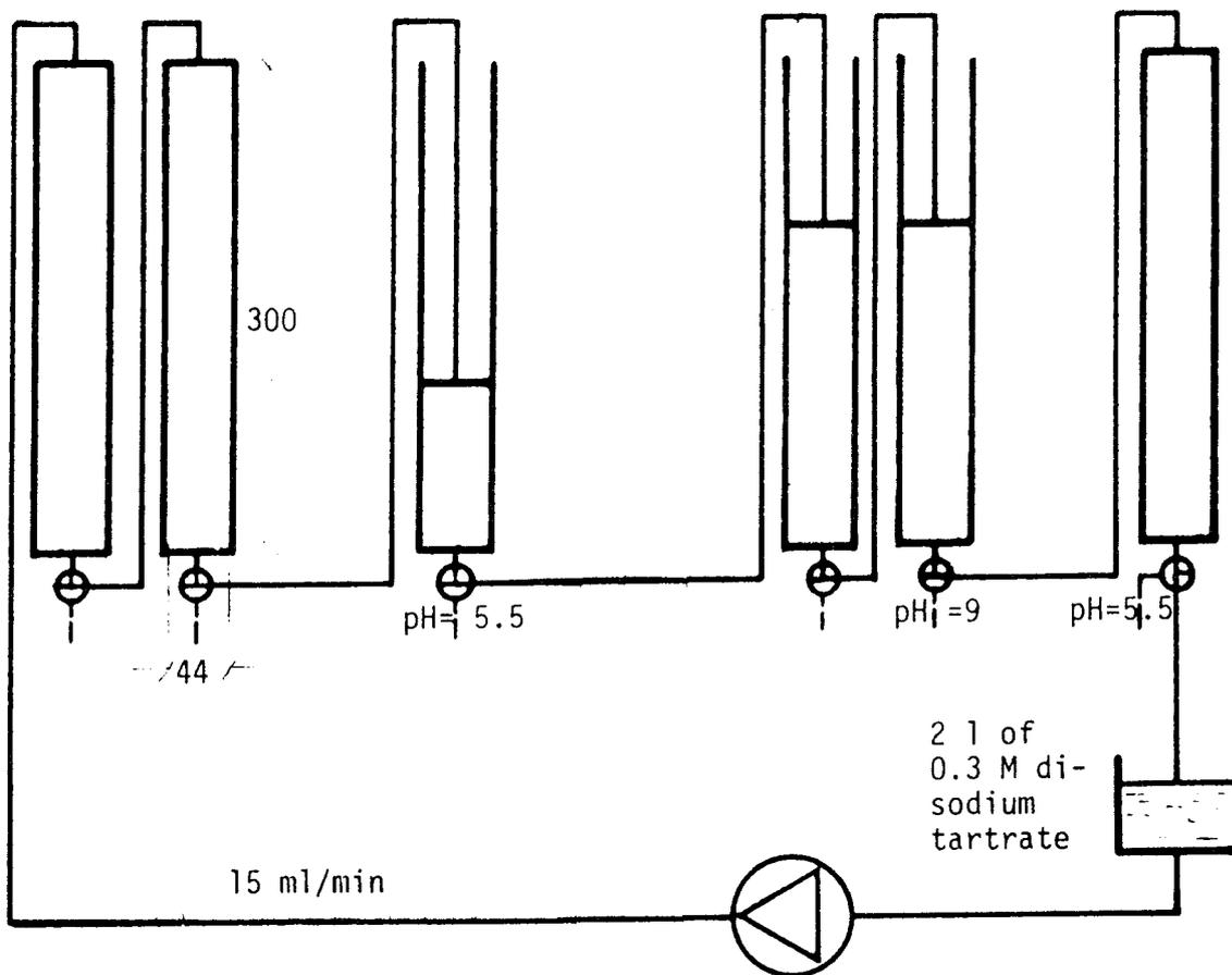
The columns and beds are drawn to scale, with connections and circulating system. The flow rate in the beds is  $\sim 1 \text{ ml/cm}^2 \cdot \text{min}$ . Dimensions are in mm.
