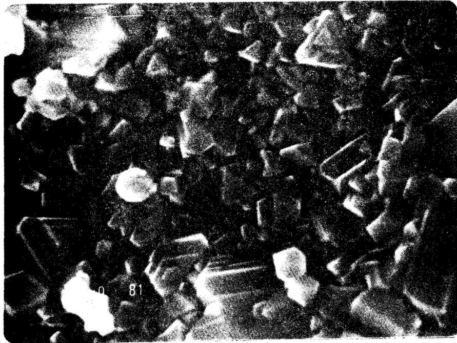
Figure 17 Ammonium titanate heat treated at  $900^{\circ}\text{C}$ . 3 500X
