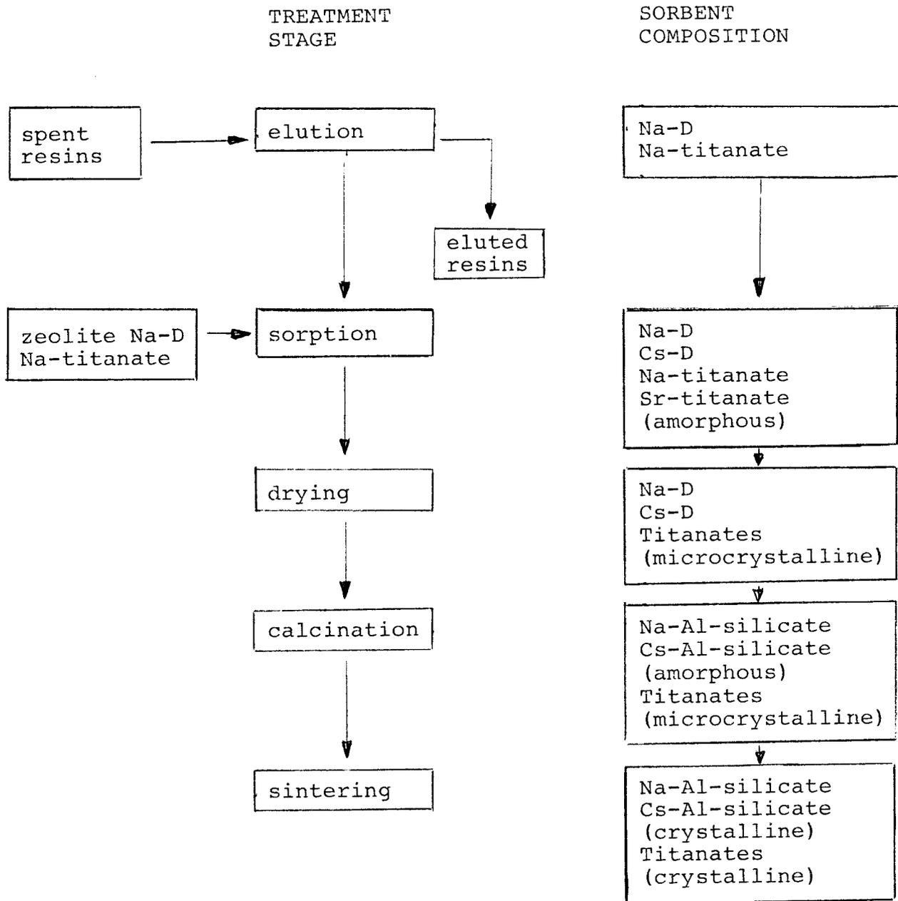
Figure 12 Principal scheme illustrating sorption of Cs and Sr on zeolite Na-D and Na-titanate after their elution from spent resins, and appearing phases in the following heat treatment stages.
