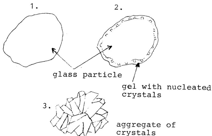
Figure 7 Illustration of zeolite crystallization from glass under hydrothermal conditions.
