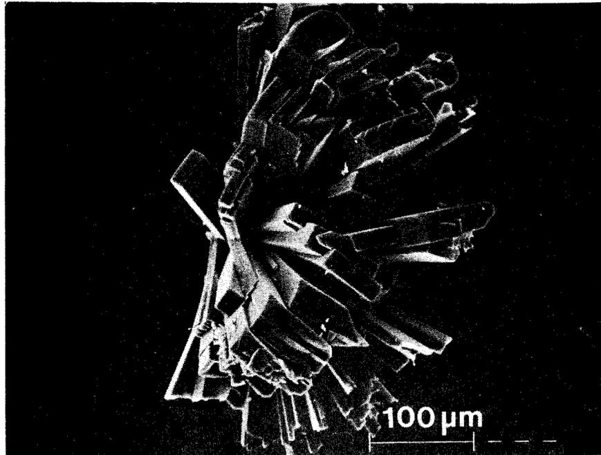
Figure 11 Synthetic mordenite grown from a glass with an Si to Al ratio of 6:1 in 0.1 M NaOH-solution for 20 hours at 300°C.
