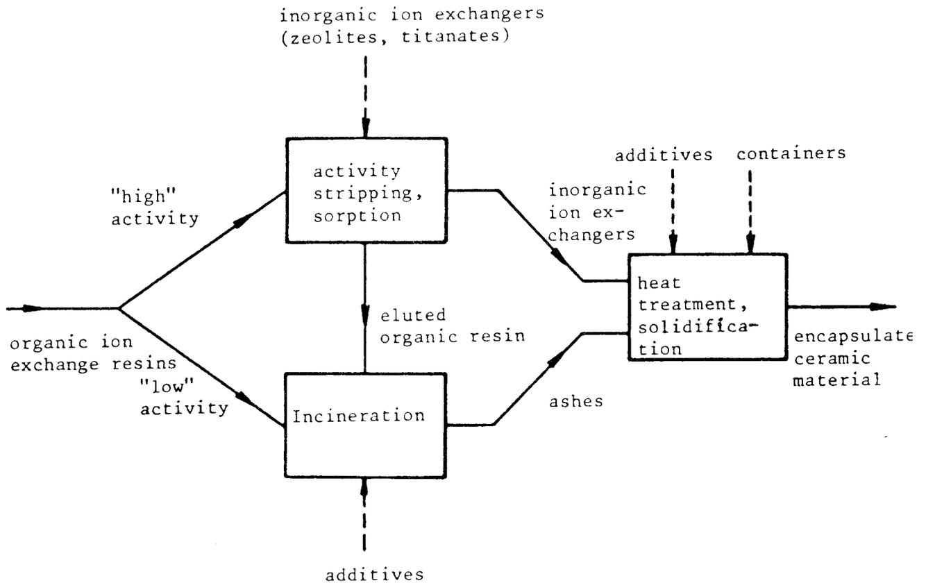
Figure 1 Block diagram of a new system for the treatment of spent organic ion exchange resins.
