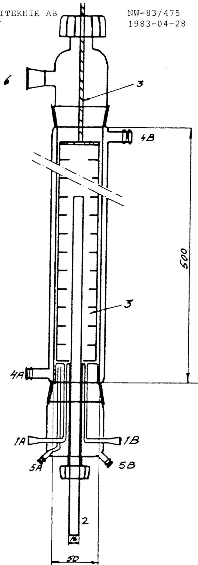
Figure 3 Glass apparatus used for the preparation of titanates from  $\text{TiCl}_4$ . 1A and 1B are inlets for  $\text{TiCl}_4$  and base solutions, 2 is outlet for the slurried product, 3 is a steel stirrer with shaft, 4-5 are ports for cooling water, 6 is a vent.
