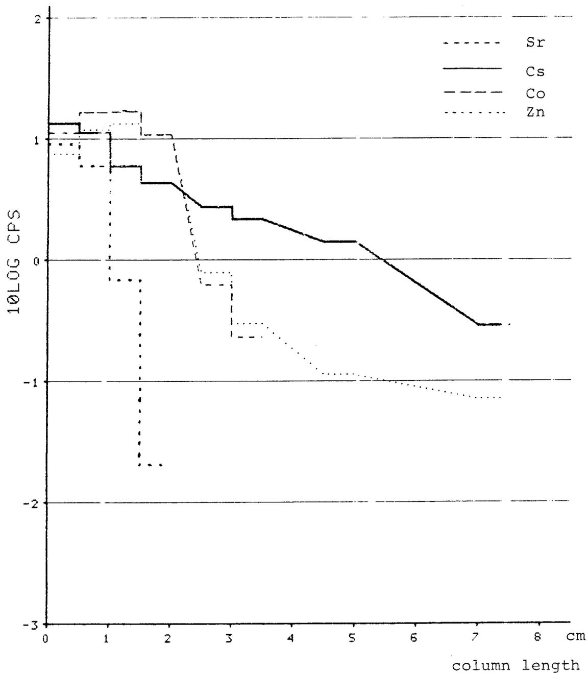
Figure 15 Sorption of Sr, Cs, Co and Zn from 0.3 M sodium tartrate solutions on a small scale sodium titanate column.
