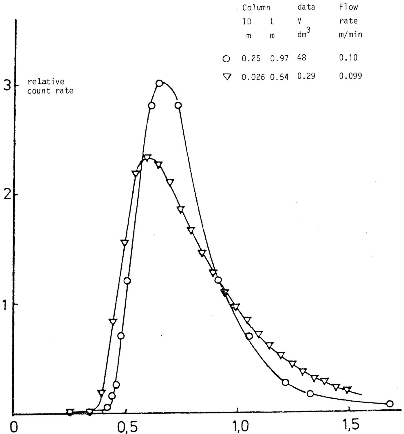
Figure 16 Distribution of Tc-99m in the effluent from sodium titanate columns, grain size 1 mm long, 1 mm diameter. The activity is given as the relative count rate versus bed volumes of effluent after the injection of  $\text{TcO}_4^-$  to the influent, 0.3 M sodium tartrate solution.
