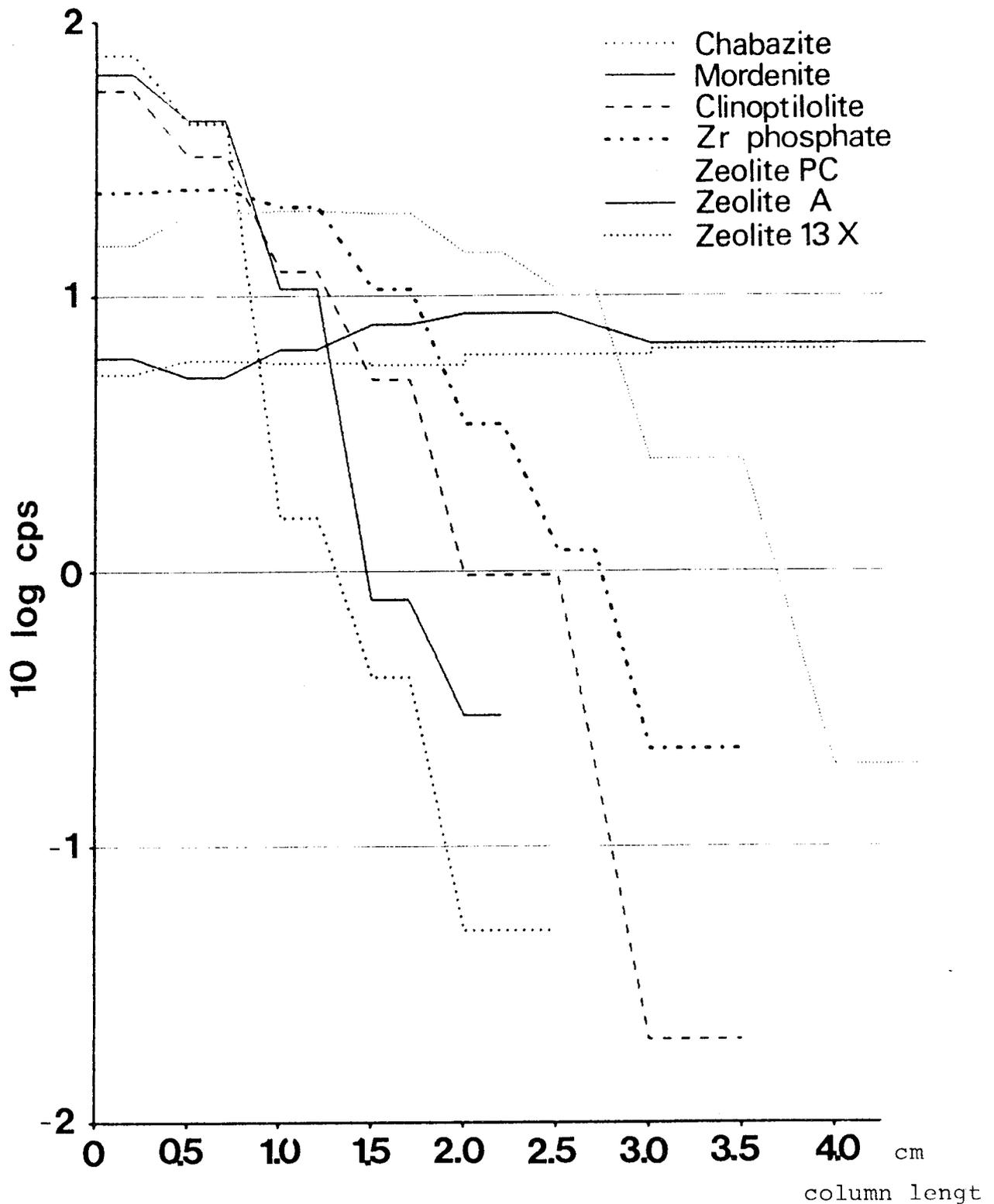
Figure 14 Sorption of Cs from 0.3 M sodium tartrate solution on different zeolites in small scale columns.
