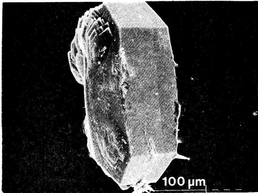
Figure 10 Synthetic mordenite grown from a glass with an Si to Al ratio of 11:1 in 0.25 M NaOH-solution for 48 hours at 200°C.
