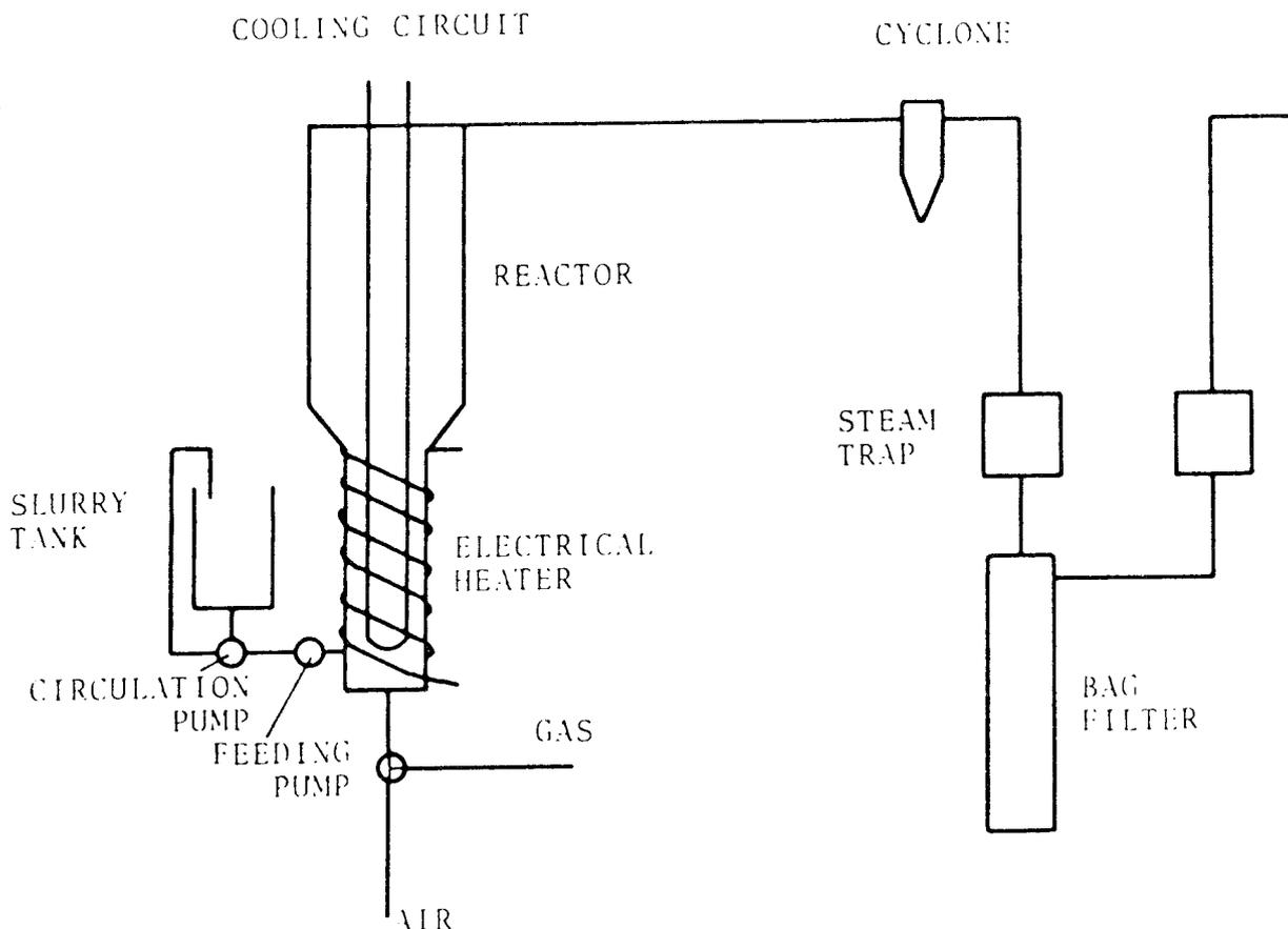
Figure 19 Experimental arrangement for studies of fluidized bed incineration of spent resins.
