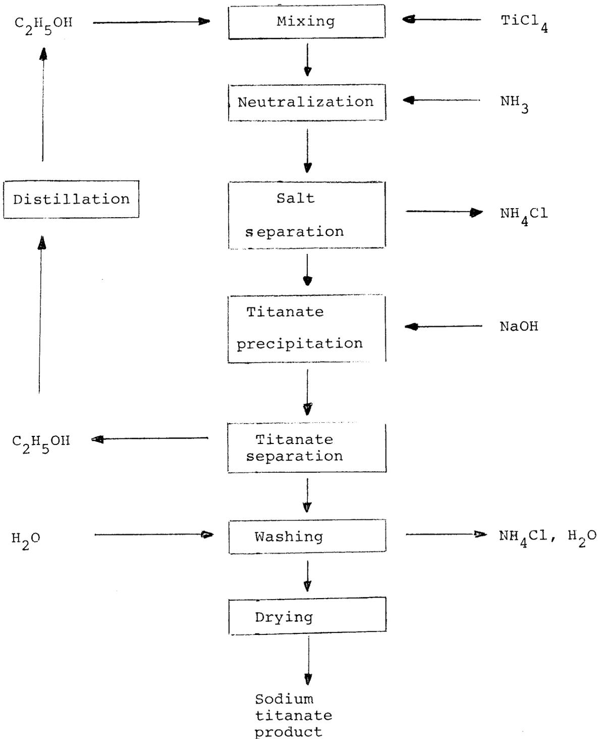
Figure 4 Flow sheet for the preparation of sodium titanate from  $\text{TiCl}_4$  with a preneutralization step.
