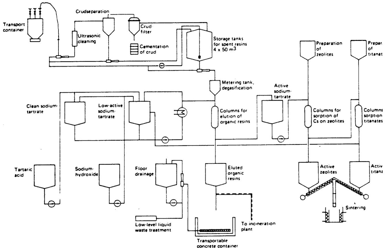
Figure 21 PILO flowsheet designed as a basis for a preliminary engineering study.
