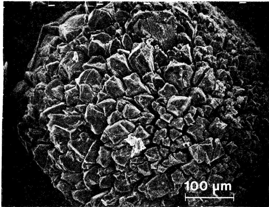
Figure 9 A variety of zeolite P grown from a glass with an Si to Al ratio of 3:1 in 1M NaOH-solution for 48 hours at 150°C. The cracks are caused by water loss of the zeolite in the evacuated microscope.
