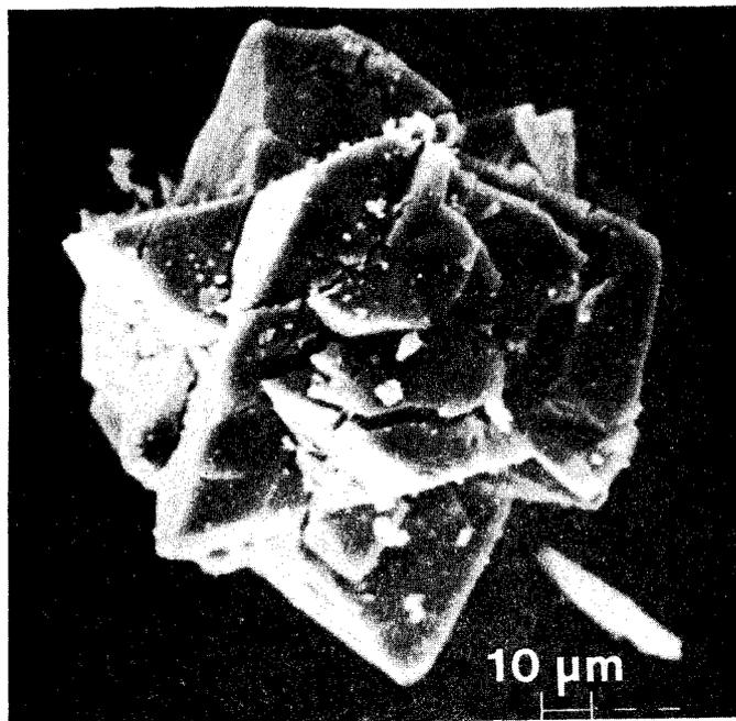
Figure 8 A low silica variety of zeolite P, grown from a glass with an Si to Al ratio of 1:1 in 0.25 M NaOH-solution for 2 weeks at 150°C. The cracks are caused by water loss of the zeolite in the evacuated microscope.
