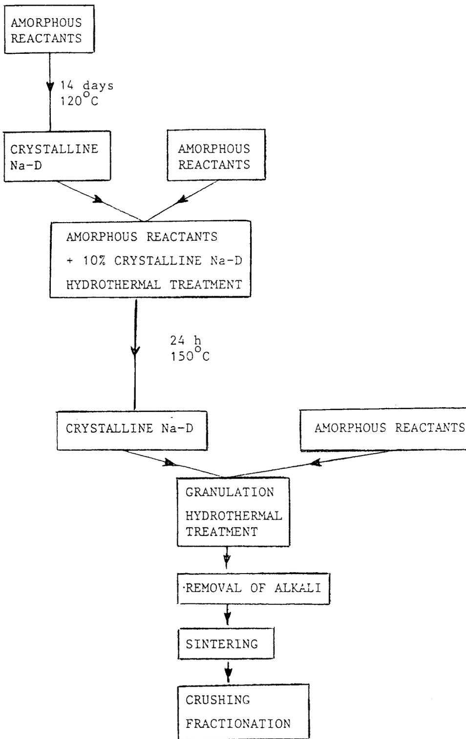
Figure 6 Scheme for the preparation of granular zeolite Na-D without binder.
