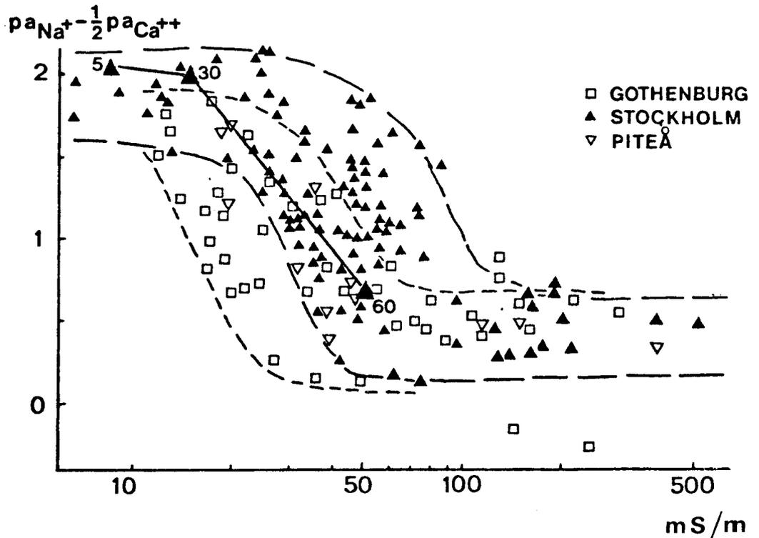
Fig. 3. Ion exchange on clays illustrated by the expression  $pa_{\text{Na}^+} - 0,5pa_{\text{Ca}^{++}}$  plotted against electric conductivity. Interconnected triangles with figures 5-30-60 means water sampled in one well at 5, 30 and 60 m depths.
