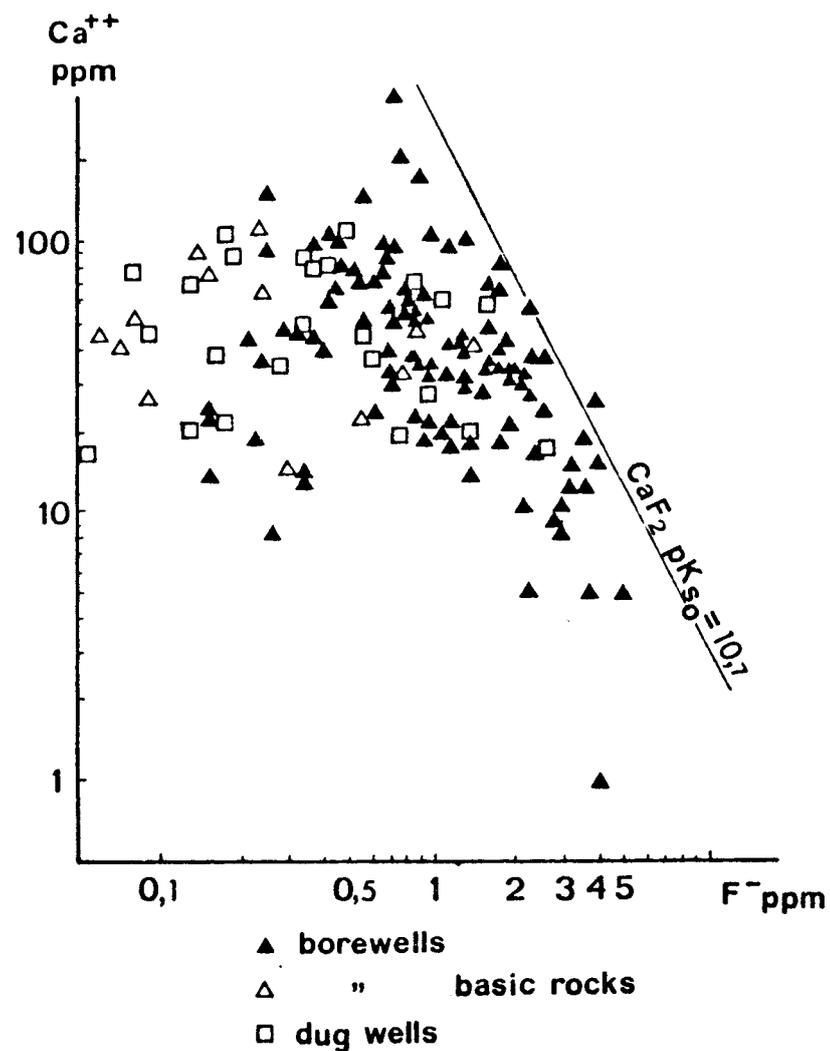
Fig. 8. Relation between  $\text{Ca}^{++}$  and  $\text{F}^-$  in ground waters.
