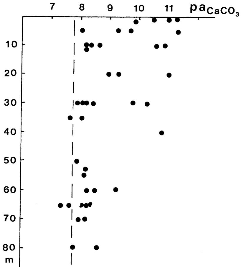
Fig. 4. Activity product for  $\text{CaCO}_3$  in ground waters plotted against depth of sampling. Broken line indicates saturation with respect to calcite.
