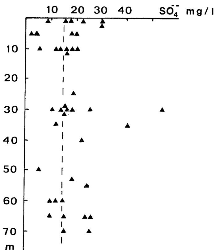
Fig. 7.  $\text{SO}_4^{--}$  in ground water as a function of sampling depth. Hatched line = atmospheric contribution.
