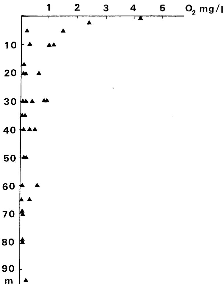
Fig. 9. Content of  $O_2$  as a function of sampling depth for wells at Gnesta and Skokloster.
