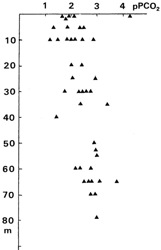
Fig. 2. Negative logarithm of partial pressure of carbon dioxide in ground water as a function of the sampling depth. Same wells as in fig. 1.
