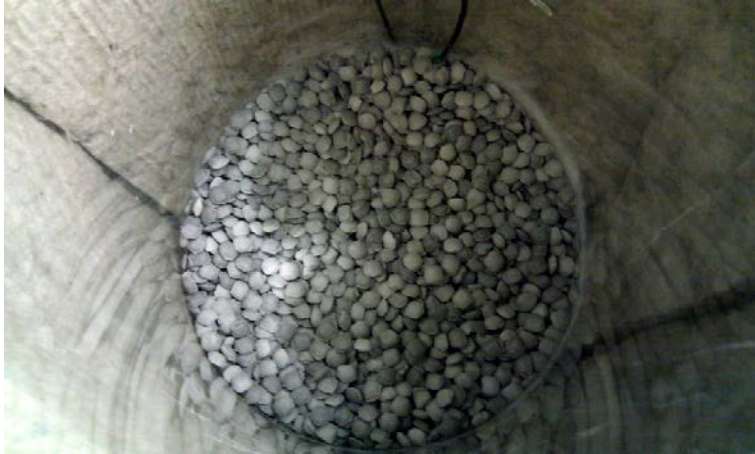
Figure 2-12. The pellets before test start, as seen from the top of the set-up. The cables to the two RH/T-sensors in the filling is seen at the top of the picture.
