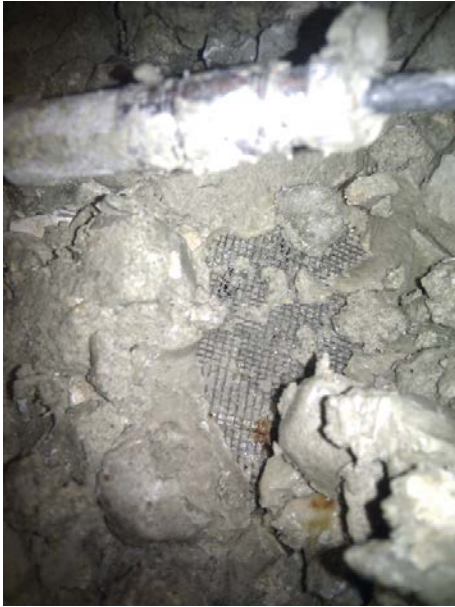
Figure 2-19. At the bottom net a more homogeneous wetted zone had formed in the room2 test.
