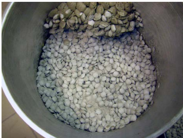
Figure 2-5. Termination of Oven1 test. Most of the pellets are excavated. Note that the pellets adjacent to the net is dry as compared to the "condensation nucleus".
