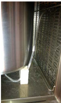
Figure 2-2. Detail of the “pot” in the oven. The tubing connected to the inlet at the bottom is visible.
