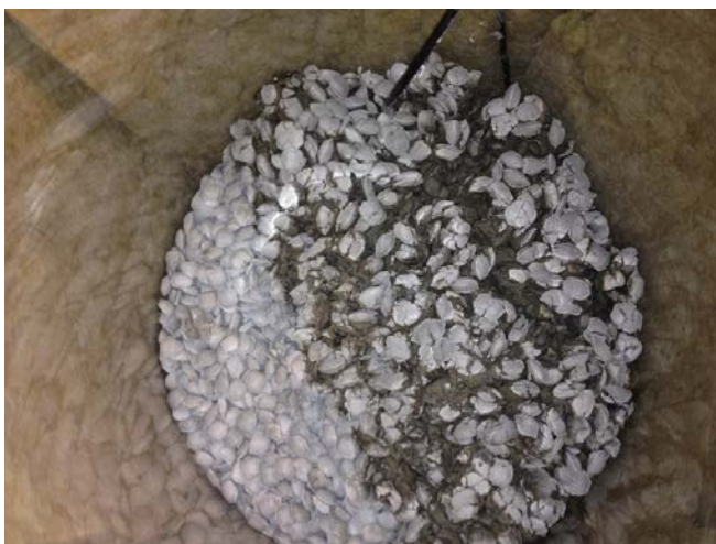
Figure 2-22. A straight front of condensation propagated across the pellets during the course of the Room3 test. Picture taken after approximately 7 days of testing. Note the similarity with Figure 2-14.
