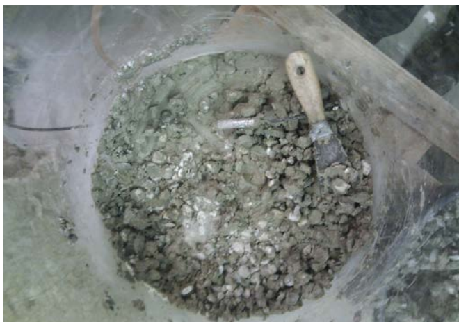
Figure 2-18. Excavation of the Room2 test. The picture show the pellets layer closest to the net. Also here was found relatively dry pellets in places.
