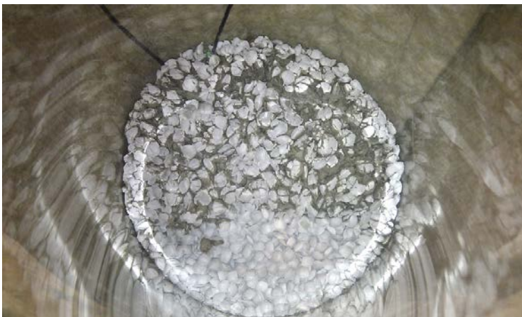
Figure 2-14. A straight front of condensation propagated across the pellets during the course of the Room2 test. Picture taken after approximately 6 days of testing.
