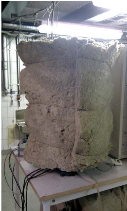
Figure 2-11. The insulated set-up of Room2 test. The system is open at the top (no lid).
