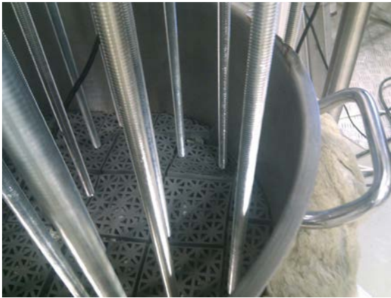
Figure 2-24. The plastic mat on top of the pellets filling in Room4 test. Also visible are the supporting rods which kept the pellets slot in place during the test.
