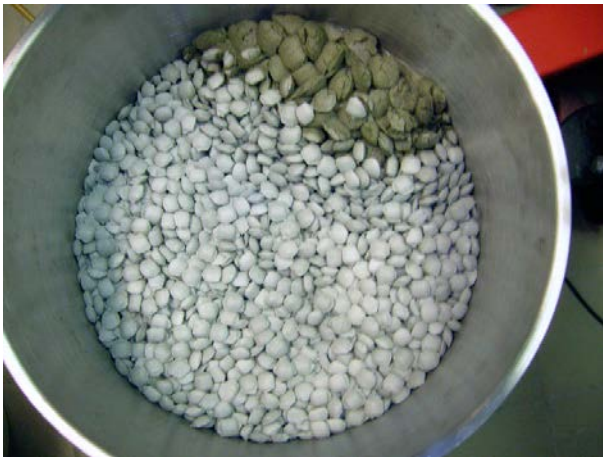
Figure 2-4. The pellets layer as seen from above after the isothermal test (Oven1).
