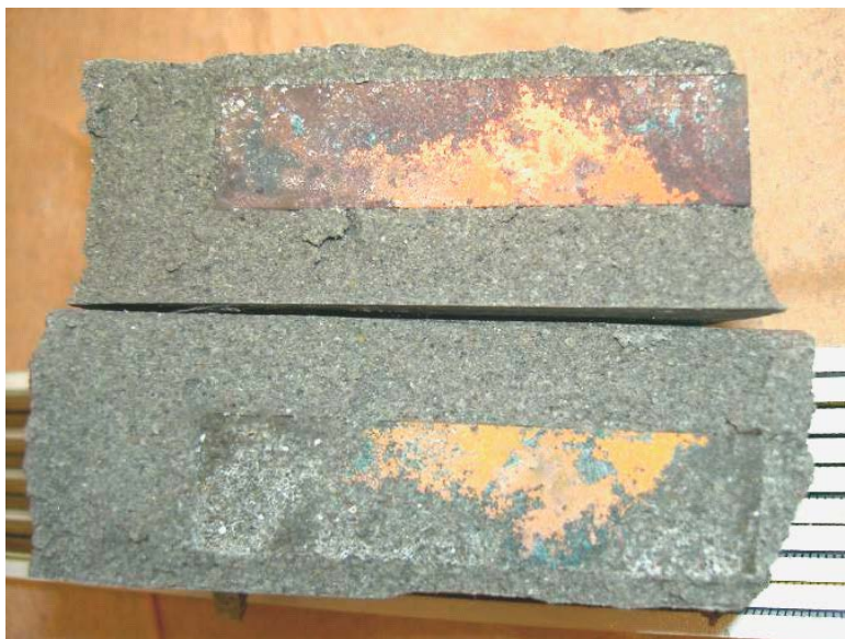
Figure 2-7. Corrosion products of Cu coupon (Karnland et al. 2009, Figure A3-1a). In upper part corrosion coupon is in place. Brownish corrosion product is cuprite (Cu 2 O).
