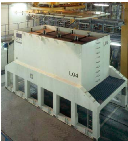
Figure 8-7. Swedish shielded transport container (Photo: Bengt O Nordin, SKB).
