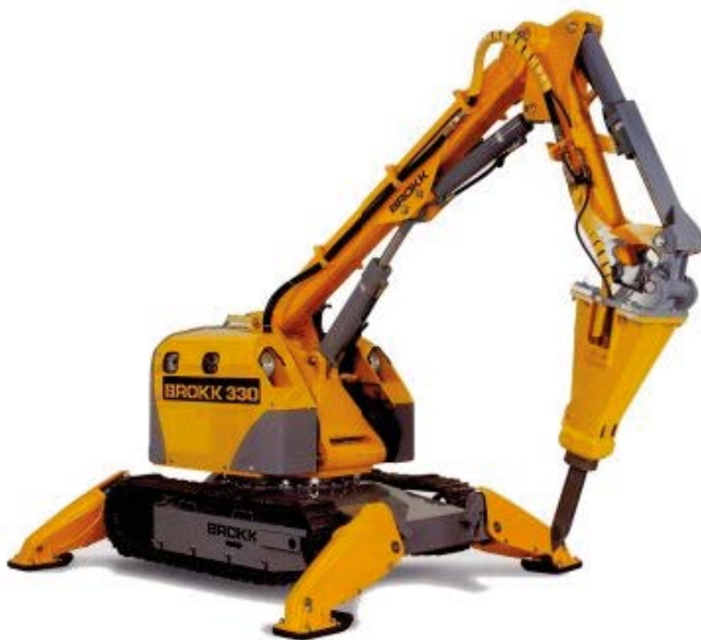
Figure 7-13. Demolition machine equipped for concrete breaking.
