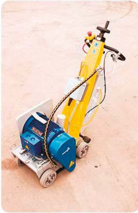
Figure 7-9. Floor Shaver and the resulting floor surface.
