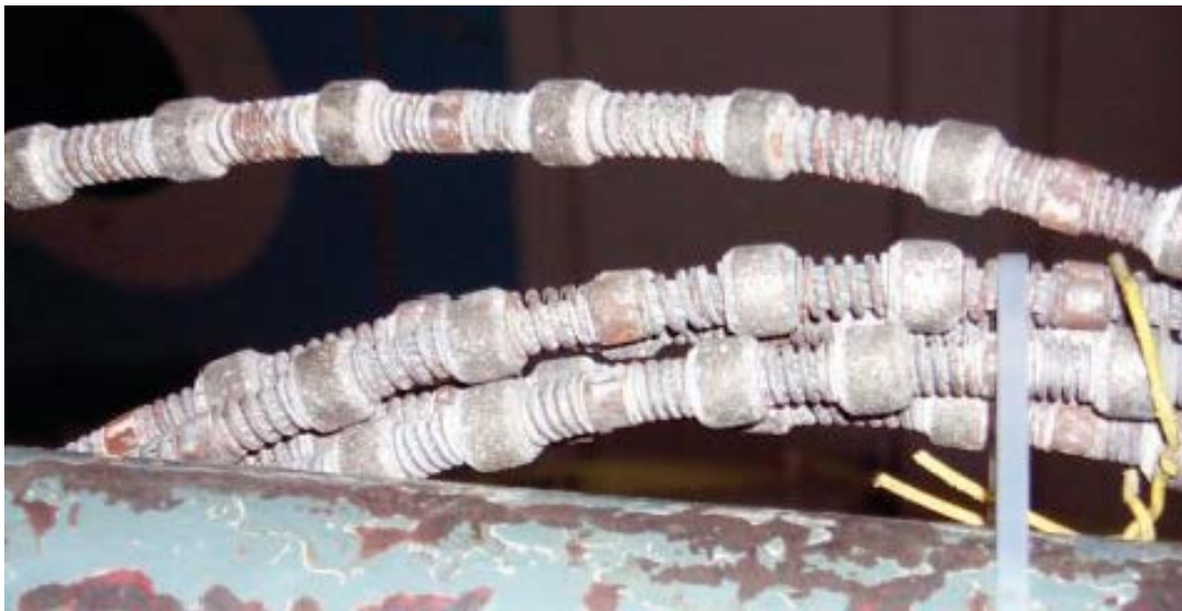
Figure 7-12. Close up of diamond wire saw blade.
