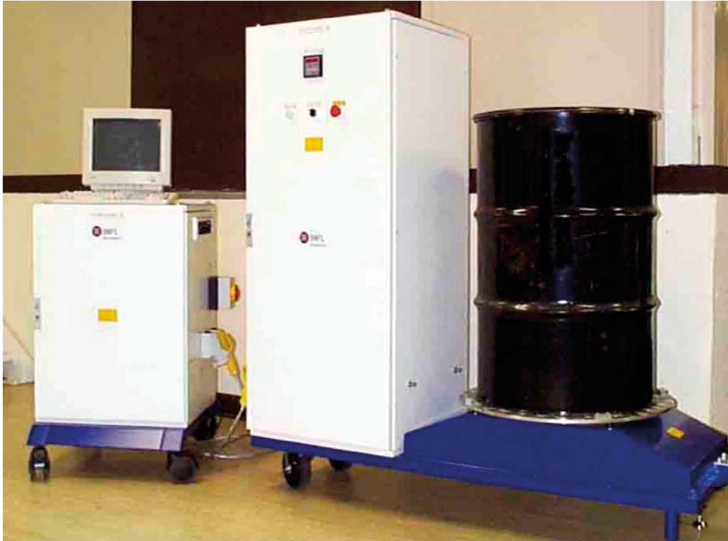
Figure A3-6. DrumScan LRGs Mk II Drum, Package and HEPA Filter Monitor.
