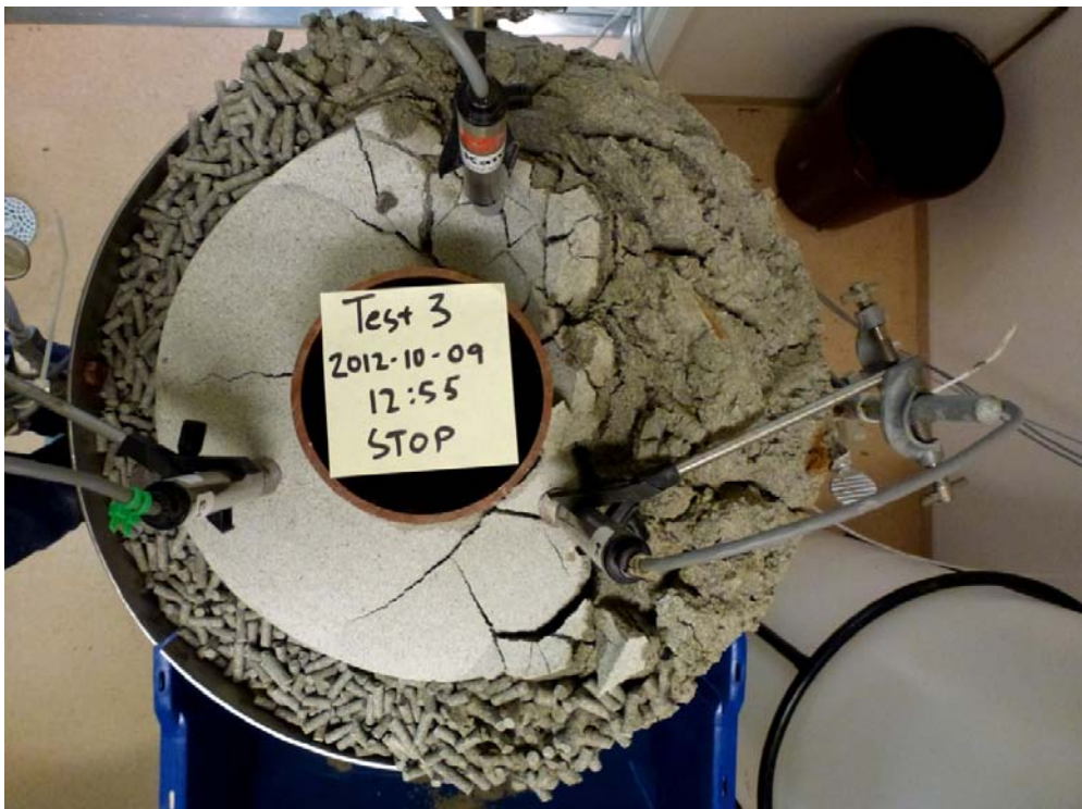
Figure A3-4. Photo showing the upper surface of the test just before the dismantling, about 165 hours after the start.
