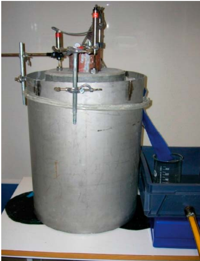
Figure 2-2. Photo of the test equipment used for testing the influence of water inflow to a deposition hole during the installation phase.
