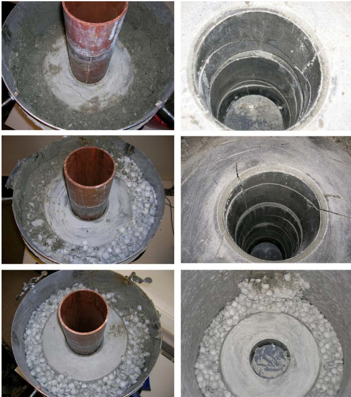
Figure 3-6. Photos taken during dismantling of the previous made tests with uniaxial compacted blocs and with roller compacted pellets at different inflow rates. Upper. 0.1 l/min: The whole pellet filling is wetted. Distinct cracks were observed in the blocks. Middle. 0.01 l/min: Half of the pellet filling is wetted. Also in this test distinct cracks can be seen in the blocks. Lower. 0.001 l/min: Only a small part of the filling is wetted. The water has ascended in a channel along the “rock” wall (Sandén and Börgesson 2010).
