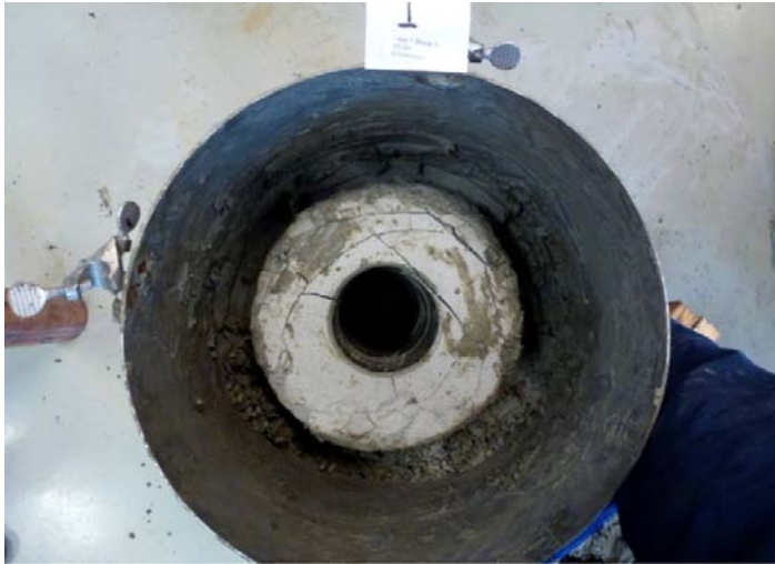
Figure 3-3. Photos taken at the dismantling of the tests made with extruded pellets. 0.01 l/min uniaxial compacted blocks.
