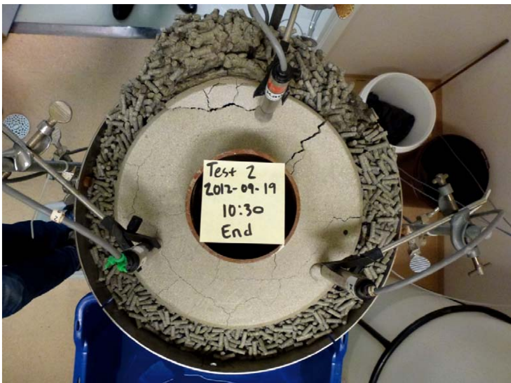
Figure A2-4. Photo showing the upper surface of the test just before the dismantling, about 165 hours after the start.
