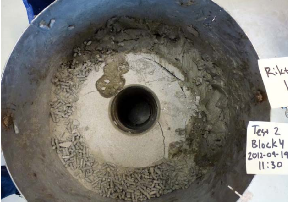
Figure A2-5. Photo showing the upper surface of a block at the dismantling.
