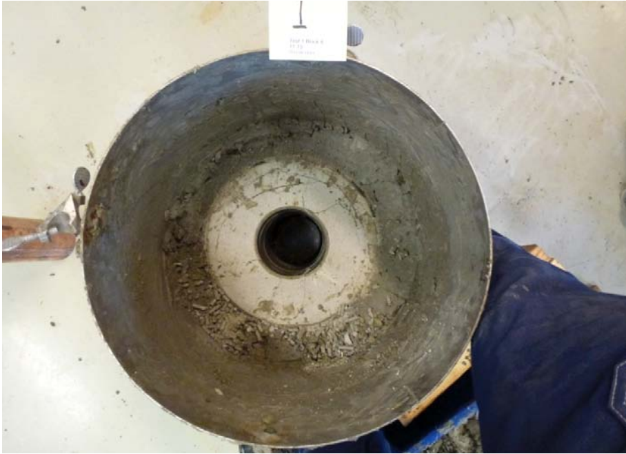
Figure A1-5. Photo showing the upper surface of a block at the dismantling.
