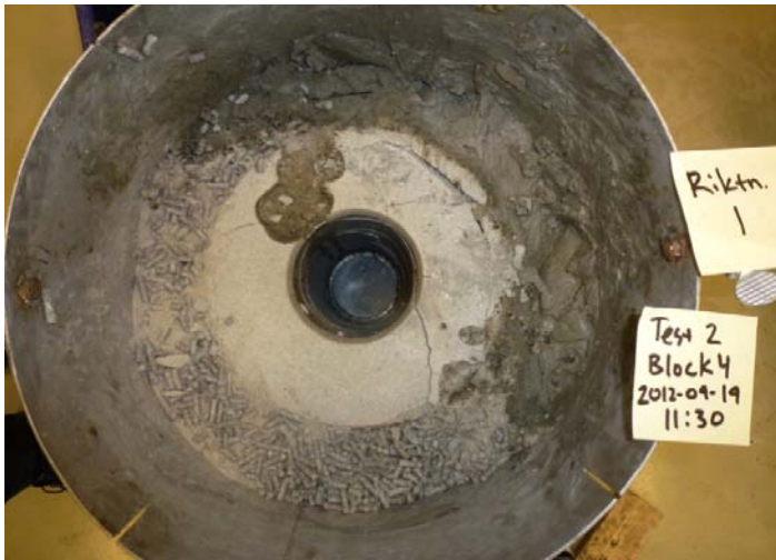
Figure 3-4. Photos taken at the dismantling of the tests made with extruded pellets. 0.00125 l/min uniaxial compacted blocks.
