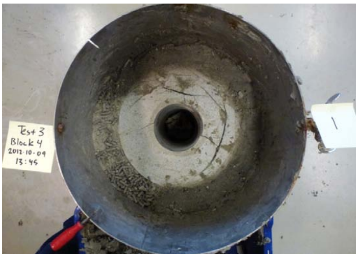
Figure 3-5. Photos taken at the dismantling of the tests made with extruded pellets. 0.01 l/min isostatic compacted blocks.
