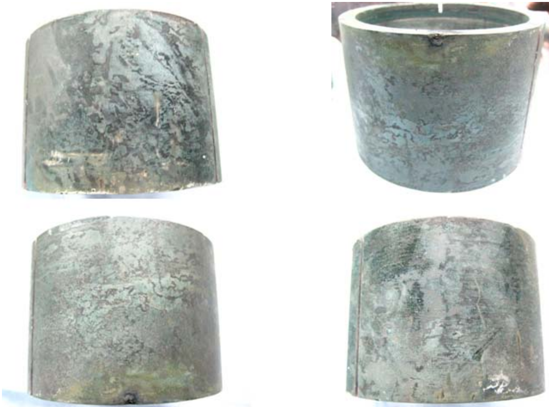
Figure 7-41. Appearance of outer surface of cast iron insert – top section (2).
