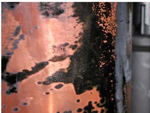
Figure 6-12. Appearance of the surface of the copper canister. The chain-like pattern on the surface at the top of the canister corresponds to the contact area with the strip of plastic insulator that was placed between the copper canister and the inner surface of the support cage.
