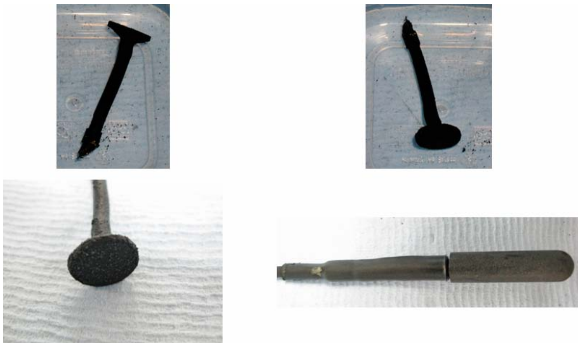
Figure 7-27. Appearance of silver-silver chloride electrodes and metal oxide E_h probe (bottom right hand corner) after removal from MiniCan Experiment 3. The top two photographs show the disc electrodes submerged in groundwater.
