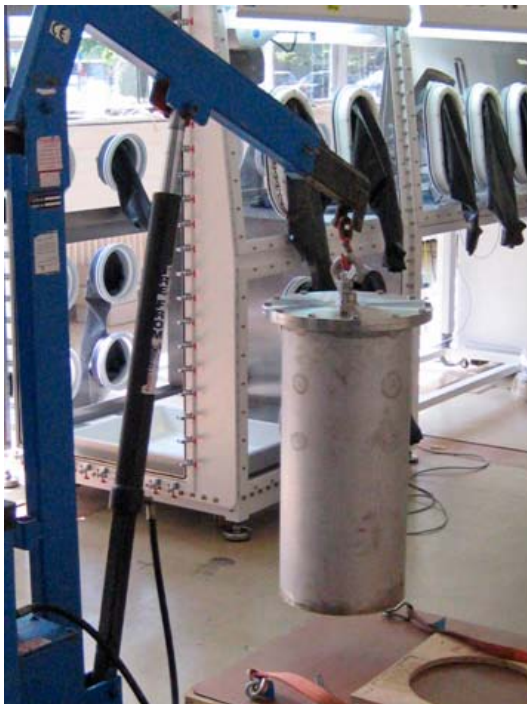
Figure 5-2. Transfer flask for MiniCan experiment being lifted into glovebox for dismantling and analysis. The right hand photograph shows the transfer flask inside the glovebox, the control for the lifting equipment and the sampling equipment for the microbial analyses in the background.
