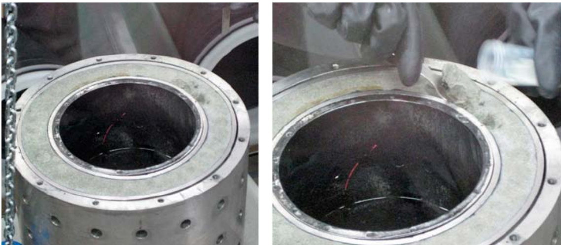
Figure 6-7. Photographs of the bentonite in the annulus of the support cage. The right hand photograph shows a sample of bentonite being taken for analysis by Microbial Analytics.
