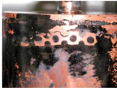
Figure 6-11. Appearance of copper canister after removal from support cage, showing condition of holes at top and bottom of the copper canister. Note that the surface had dried in the glovebox due to the very low humidity.
