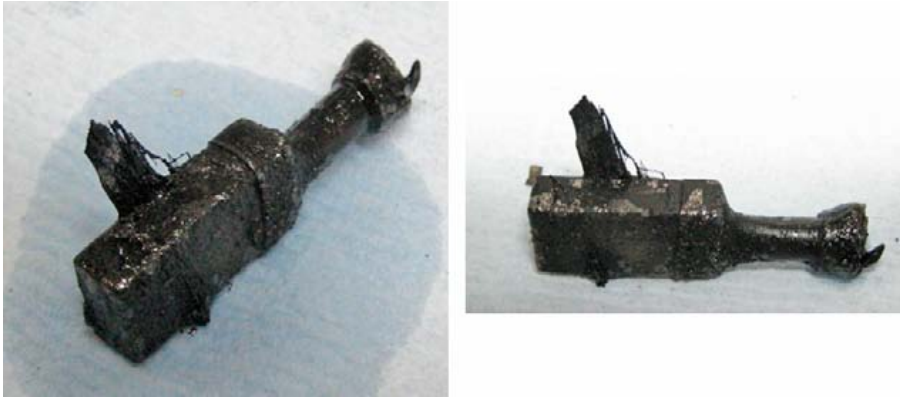
Figure 7-9. Iron electrode 2 from MiniCan Experiment 3, showing presence of whiskers of iron sulphide.
