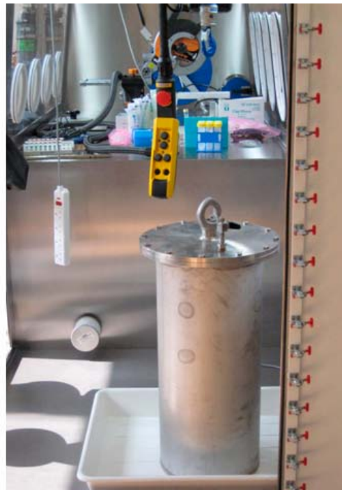
Figure 5-2. Transfer flask for MiniCan experiment being lifted into glovebox for dismantling and analysis. The right hand photograph shows the transfer flask inside the glovebox, the control for the lifting equipment and the sampling equipment for the microbial analyses in the background.
