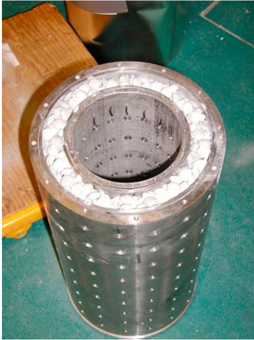
Figure 6-4. For comparison with later photographs, these photographs show the original condition of the support cage, bentonite pellets and copper canister in 2006 before the start of the experiment in the Äspö URL.
