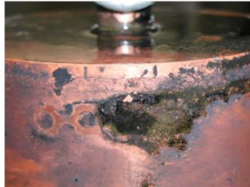
Figure 6-11. Appearance of copper canister after removal from support cage, showing condition of holes at top and bottom of the copper canister. Note that the surface had dried in the glovebox due to the very low humidity.
