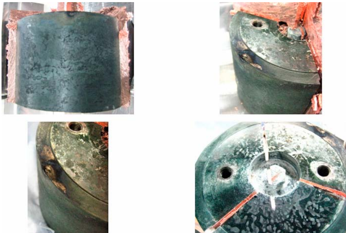
Figure 7-40. Appearance of outer surface of cast iron insert – top section (1).
