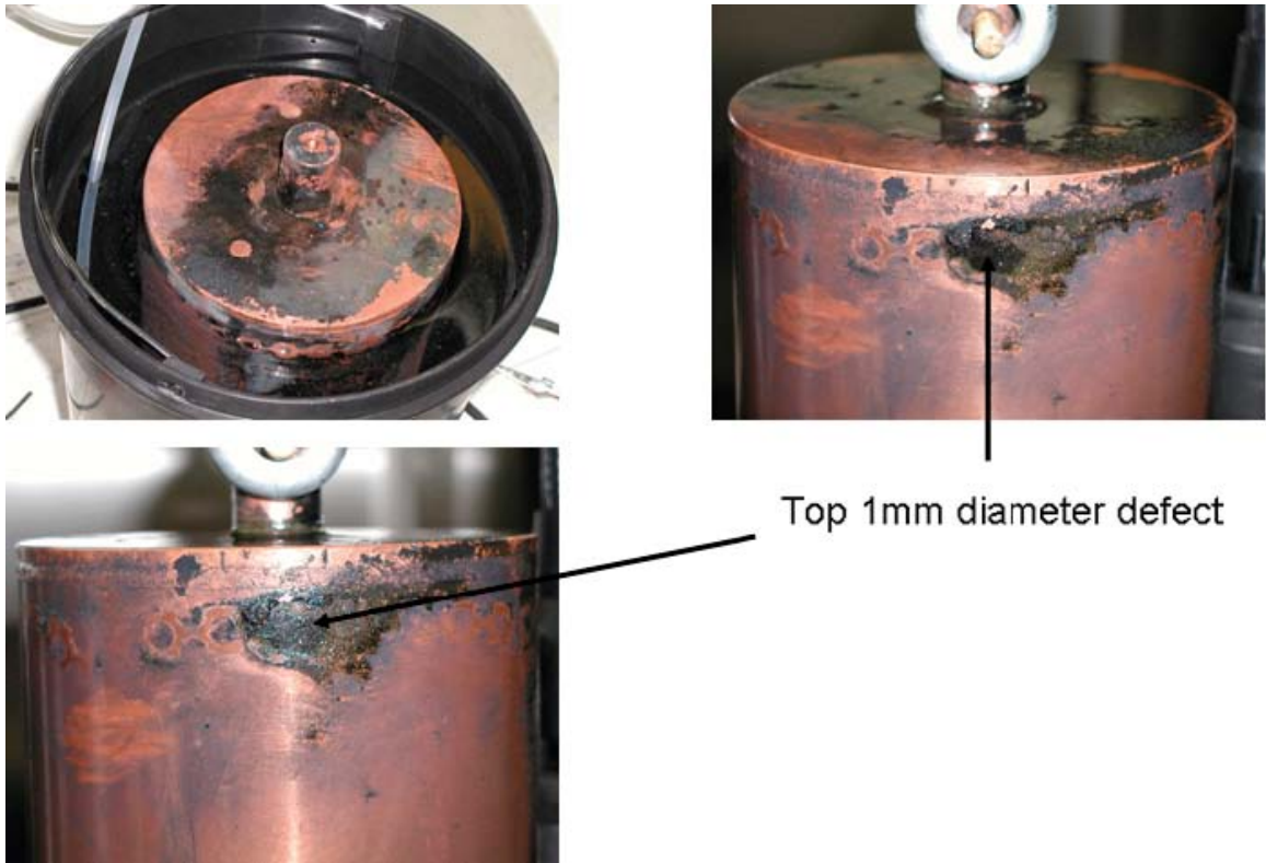
Figure 6-13. Appearance of the surface of the copper canister; showing location of defects at top of canister.
