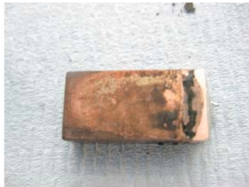
Figure 7-1. Copper electrode 1 in water, showing loose deposit that washed off electrode.
