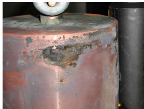
Figure 6-12. Appearance of the surface of the copper canister. The chain-like pattern on the surface at the top of the canister corresponds to the contact area with the strip of plastic insulator that was placed between the copper canister and the inner surface of the support cage.
