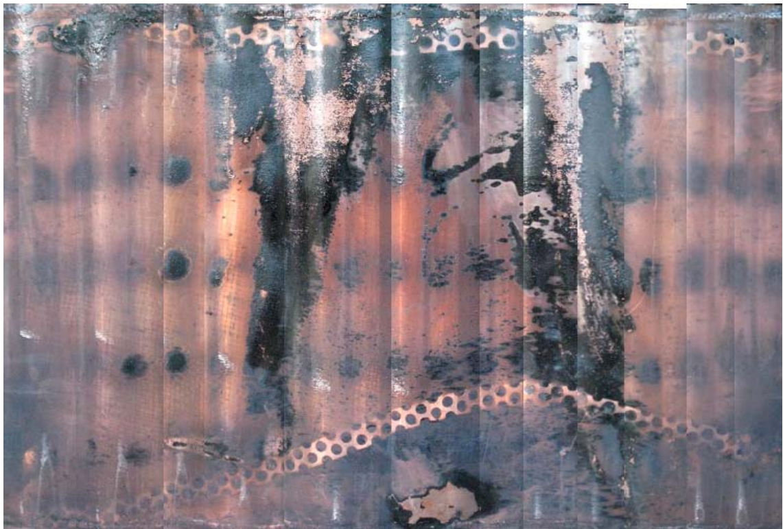
Figure 6-14. Panoramic photo-montage of surface of copper canister on removal from support cage.
