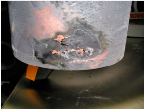
Figure 6-11. Appearance of copper canister after removal from support cage, showing condition of holes at top and bottom of the copper canister. Note that the surface had dried in the glovebox due to the very low humidity.
