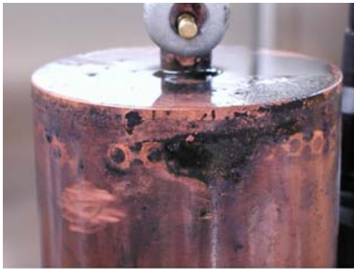
Figure 6-11. Appearance of copper canister after removal from support cage, showing condition of holes at top and bottom of the copper canister. Note that the surface had dried in the glovebox due to the very low humidity.
