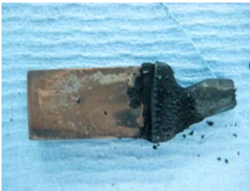
Figure 7-1. Copper electrode 1 in water, showing loose deposit that washed off electrode.
