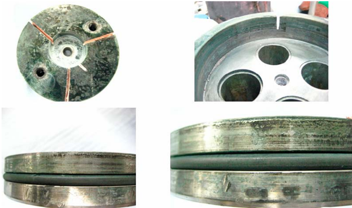
Figure 7-43. Lid of cast iron insert removed from Experiment 3 in an anoxic glovebox.
