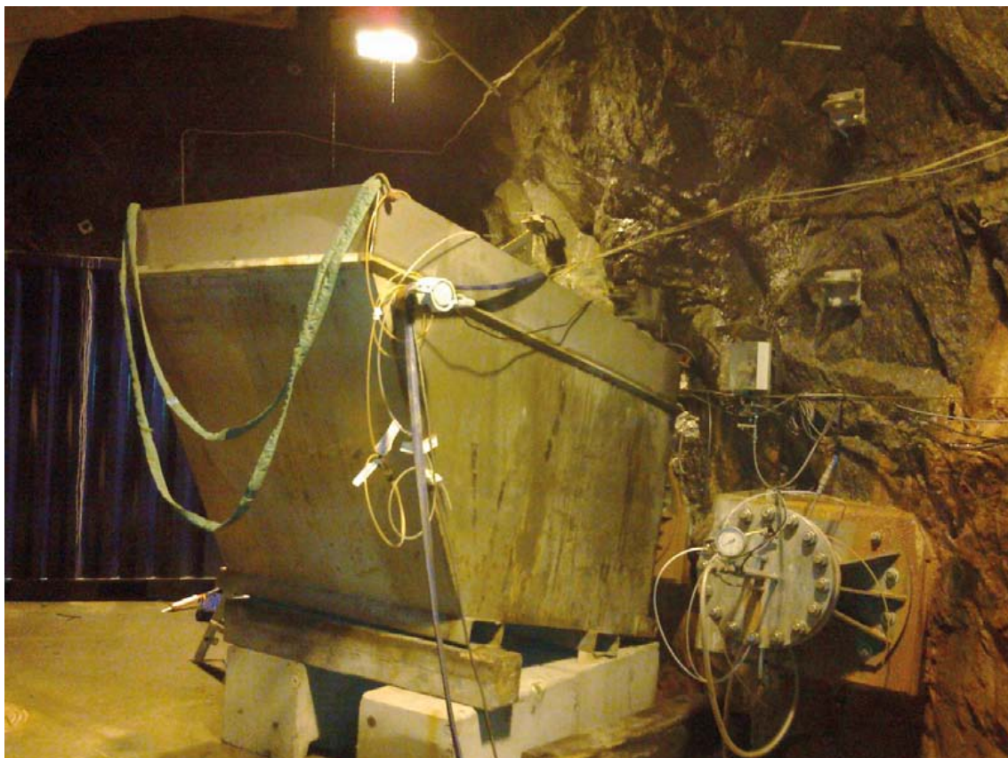
Figure 2-3. Photograph of transfer tank set up to enable MiniCan Experiment 3 to be removed and transferred into the transfer flask ready for transport without drying or exposure to air.
