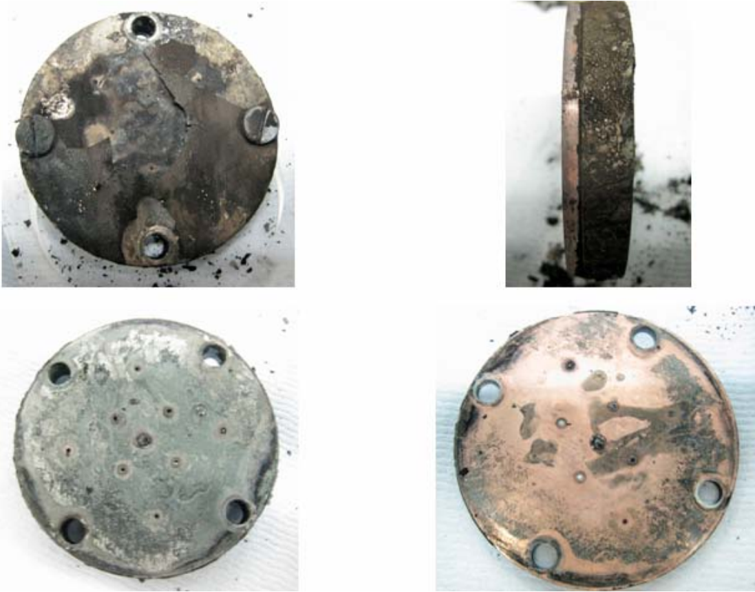
Figure 7-21. Appearance of sandwich specimen when removed from MiniCan Experiment 3. The lower two photographs show the interior surfaces of the specimen.
