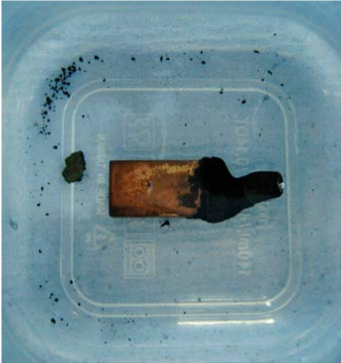
Figure 7-1. Copper electrode 1 in water, showing loose deposit that washed off electrode.
