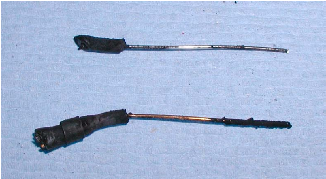
Figure 7-18. Platinum (top) and gold (bottom) electrodes removed from MiniCan Experiment 3. The insulating sheathing is still present at the left hand end of the wires.
