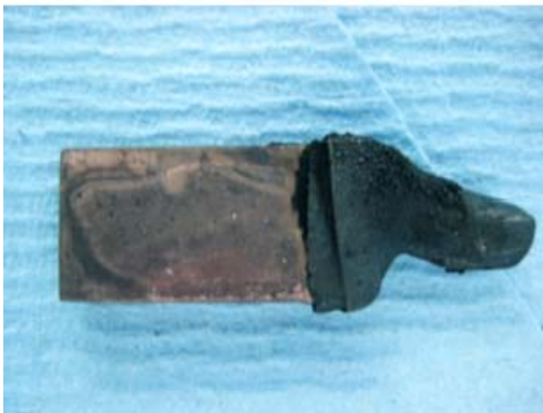
Figure 7-2. Copper electrode 1 showing both sides, before and after removal of sheathing. Note that the surface had dried out in the glovebox when these photographs were taken. The specimens were 10 mm wide.
