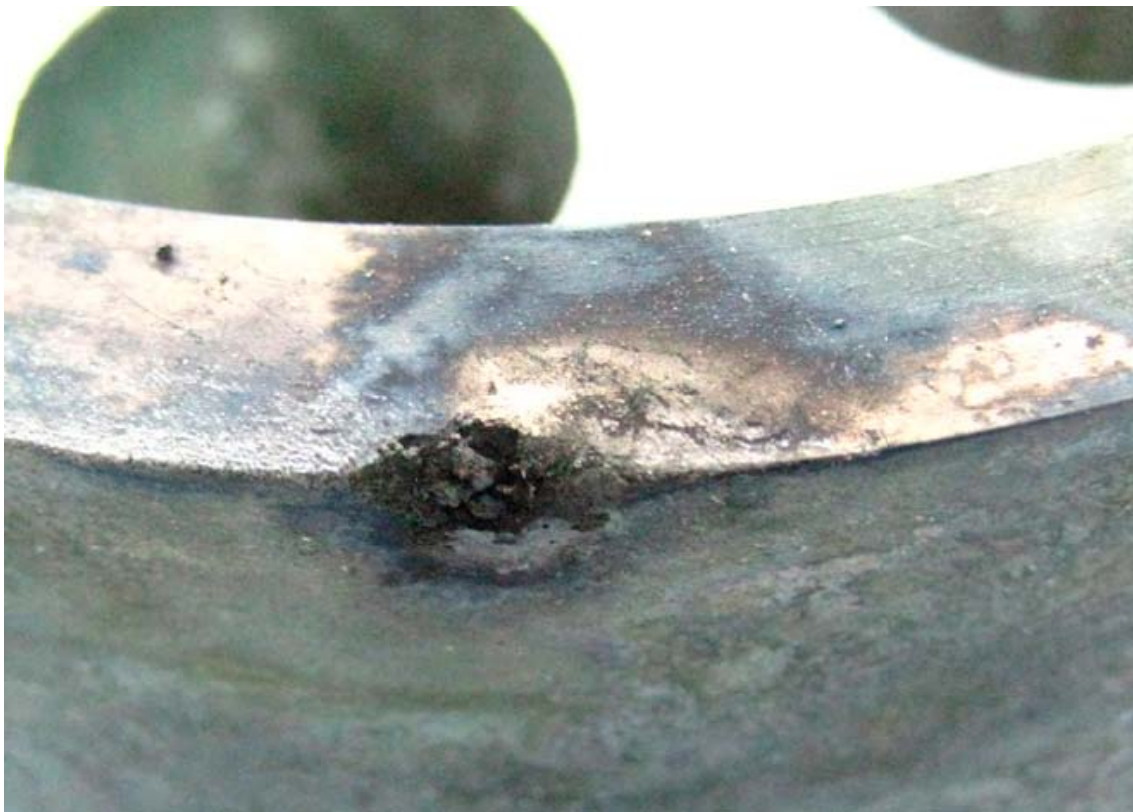
Figure 7-42. Top of cast iron insert showing attack of iron opposite defect in copper.
