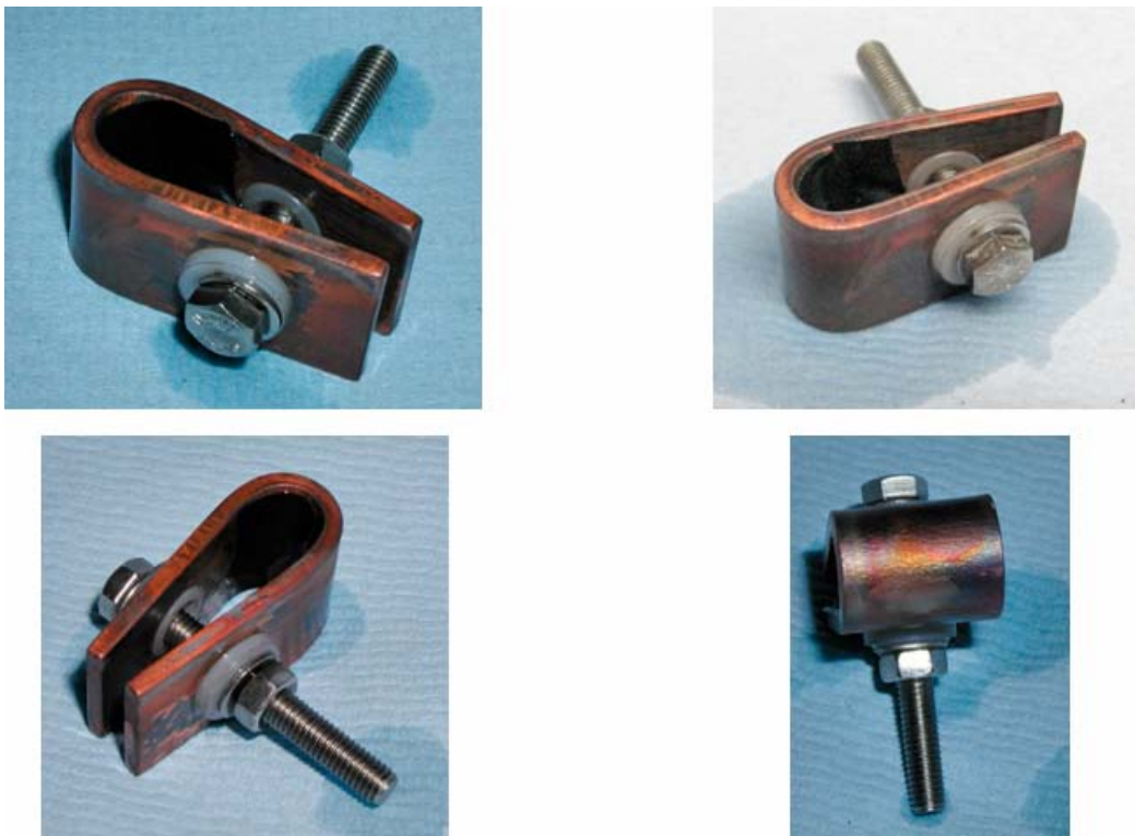
Figure 7-34. Photographs of U-bend SCC specimens from near the support cage removed from borehole Experiment 3.
