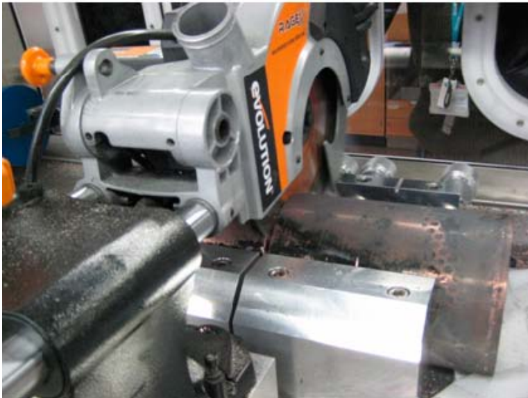
Figure 3-3. Photograph of lifting and cutting equipment inside glovebox.
