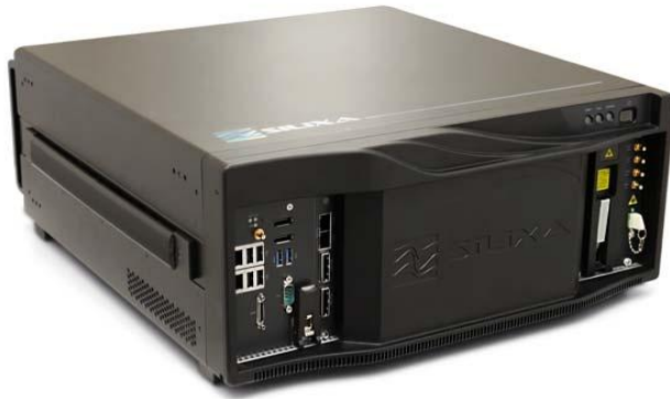
Figure 2-13 Silixa's Carina interrogator.
