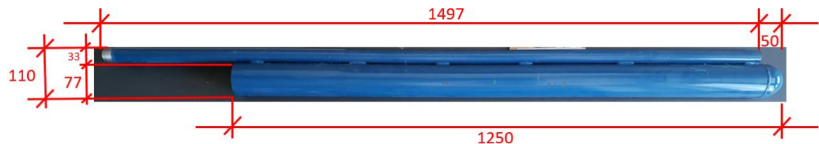
Figure 3-3 Bullnose welded at the first grouting pipe for protection of the downhole terminations of the fibre optic cables. Dimensions in mm.
