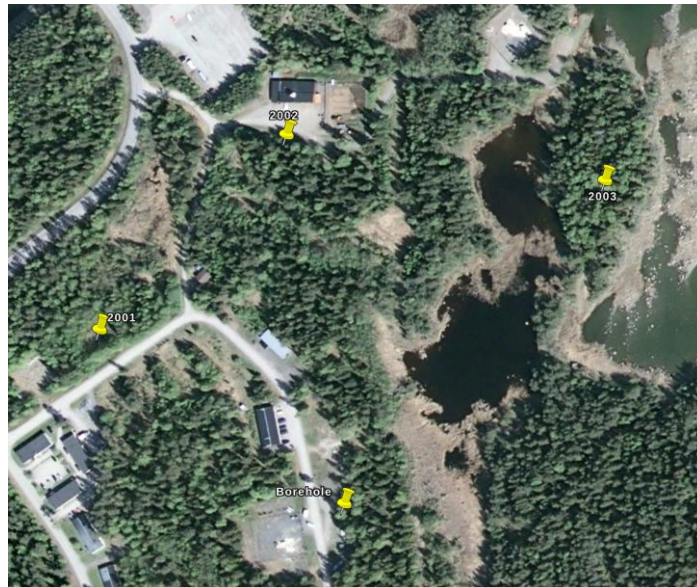
Figure 4-8: Location of the borehole and the 3 source sites (2001, 2002, 2003) where weight drops were performed in order to determine the orientation of the borehole geophones.
