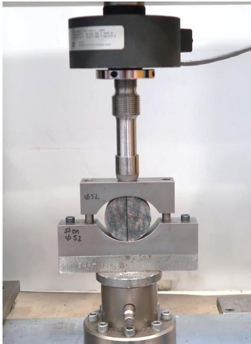
Figure 4-1. Test-set up for the indirect tensile strength test. The load cell is visible in the top and the curved bearing blocks are seen below that.
