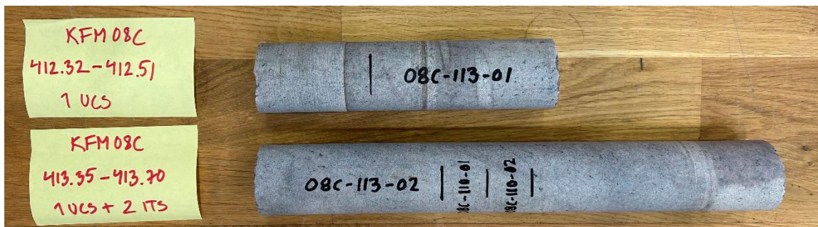
Figure 3-5. Specimen layout for cutting the test specimens on core sections from KFM08C (borehole length 412–413 m).
