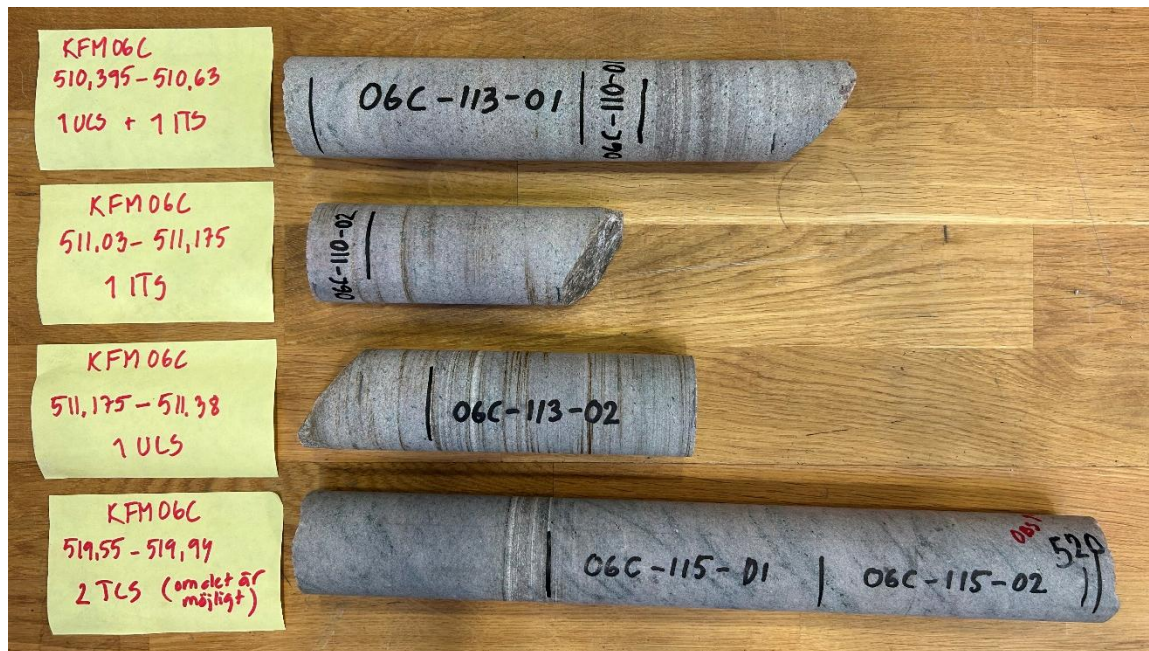
Figure 3-1. Specimen layout for cutting the test specimens on core sections from KFM06C (borehole length 510–520 m).
