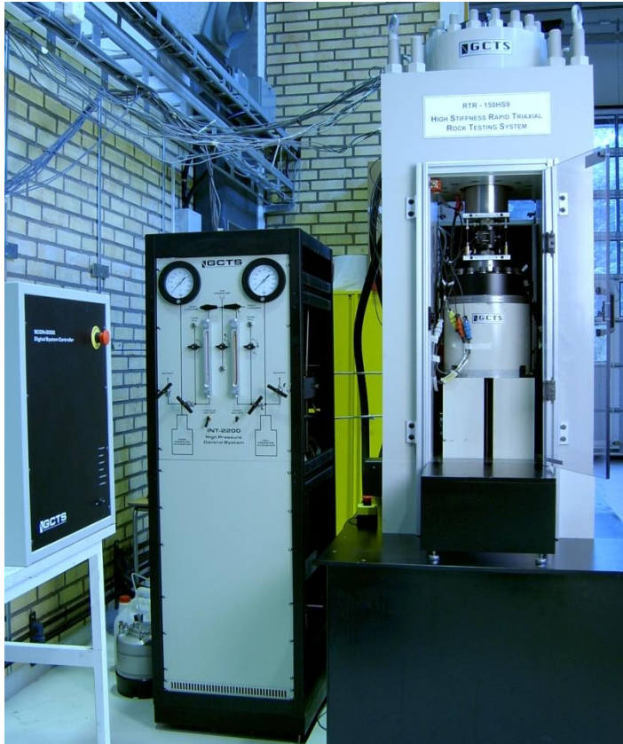
Figure 4-2. Rock testing system. From left: Digital controller unit, pressure cabinet (used for triaxial tests) and load frame. The PC with the test software (not shown in the picture) is placed on the left hand side of the controller unit.
