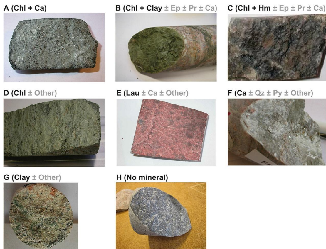
Figure 10-1. Typical fracture surfaces of Forsmark drill core samples illustrating identified fracture types. Mineral abbreviations: chlorite (Chl), calcite (Ca), epidote (Ep), hematite (Hm), laumontite (Lau), prehnite (Pr), pyrite (Py), quartz (Qz). Figure taken from Crawford and Löfgren (2019).
