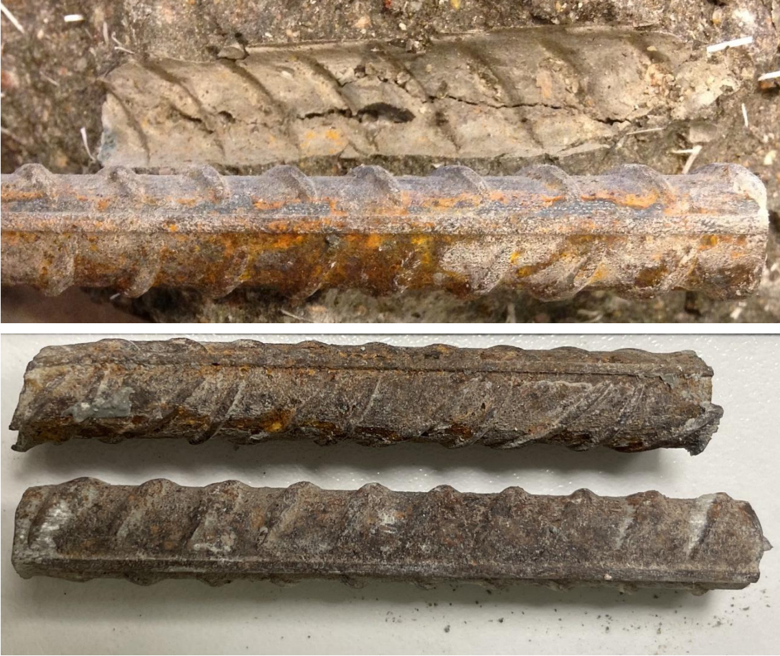
Figure 8-1. Photograph of carbon-steel objects 5YW-CS (with concrete imprint) (top) and 15YD-CS (bottom).
