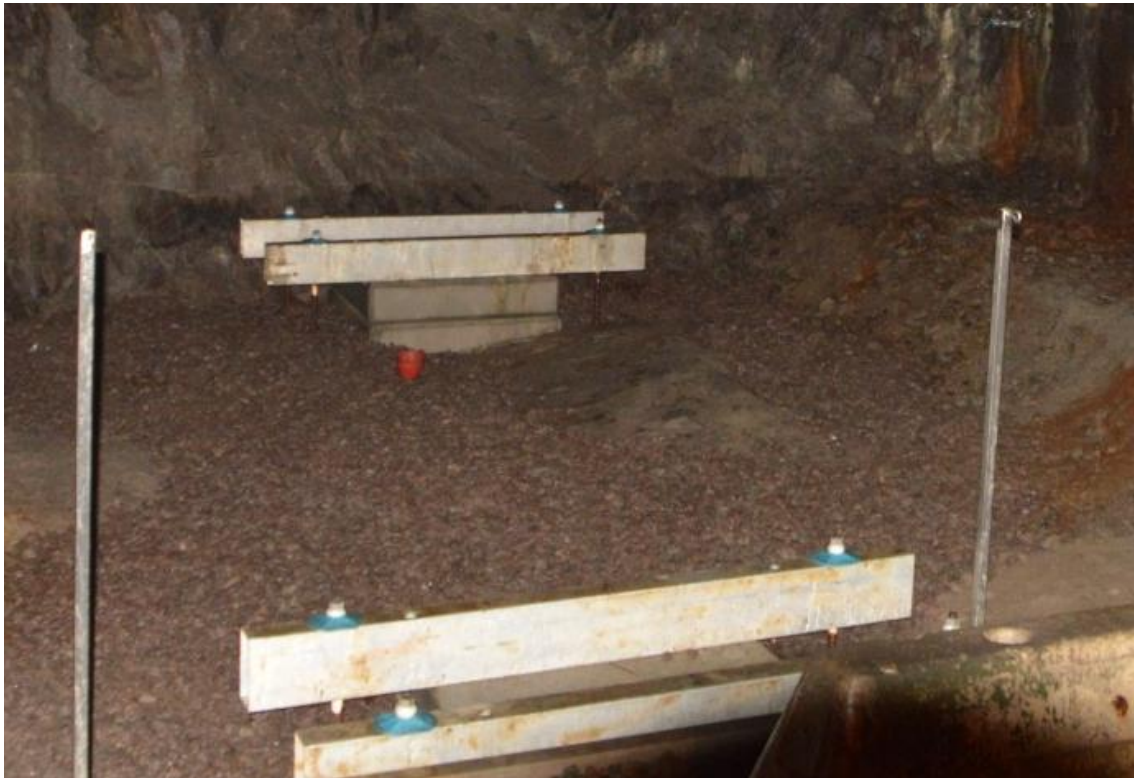
Figure 3-6. Installation of the long-term corrosion experiments in TASR completed
