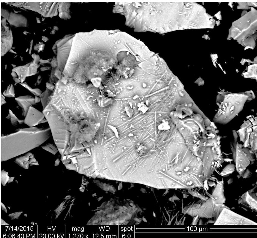
Figure 6-5. A single grain used to analyse the chemical composition of the grains identified on the surface of the zinc object, SEM/BSE detector. (Kalinowski 2015)
