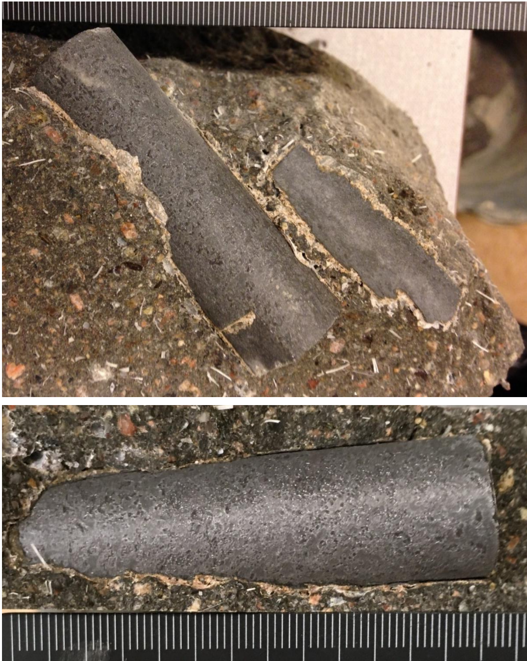
Figure 7-1. Surface of the aluminium object 5YW-Al (top) and 10YW-Al (bottom).
