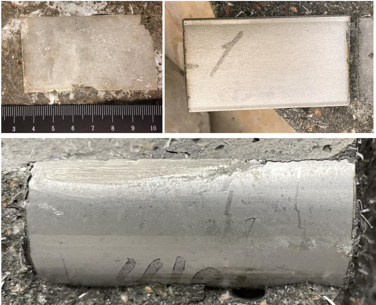
Figure 9-1. Surface of the stainless-steel objects from samples 5YW-SS (top left), 10YW-SS (top right) and 15YD-SS (lower).
