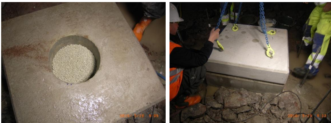
Figure 3-5. Sealing and closure of a long-term corrosion experiment.
