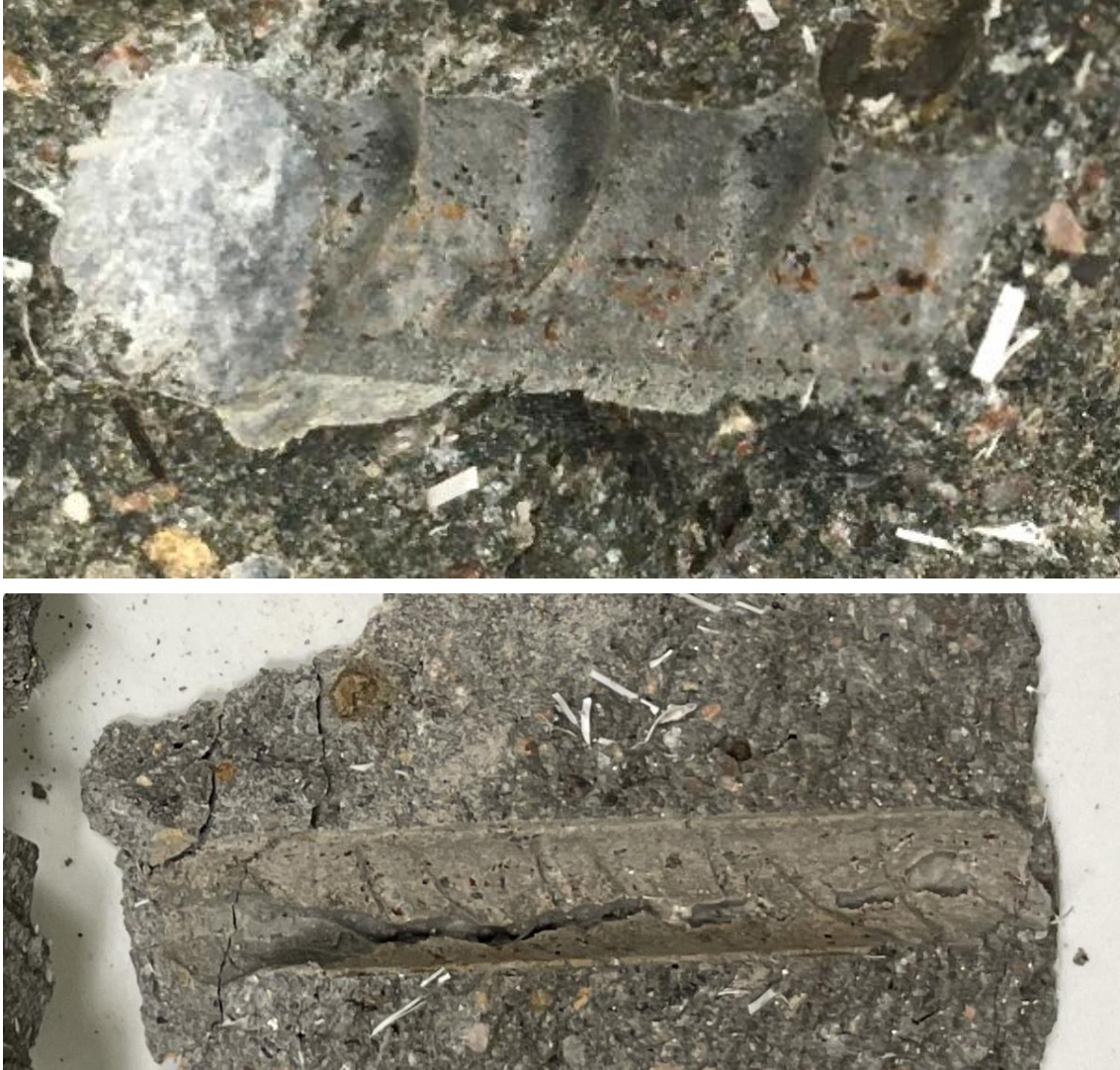
Figure 8-2. Concrete imprints of carbon-steel objects for samples 10YW-CS (top) and 15YD-CS (bottom).
