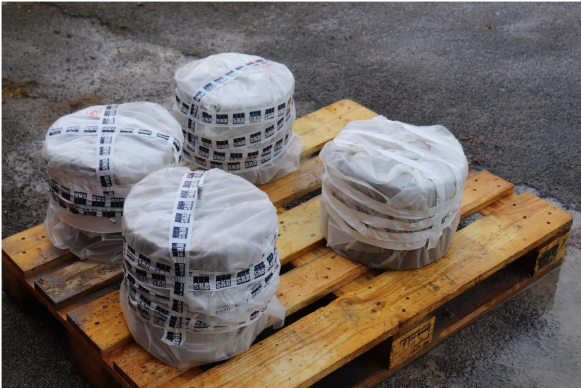
Figure 4-7. The four parts of a concrete cylinder after sectioning and packaging.
