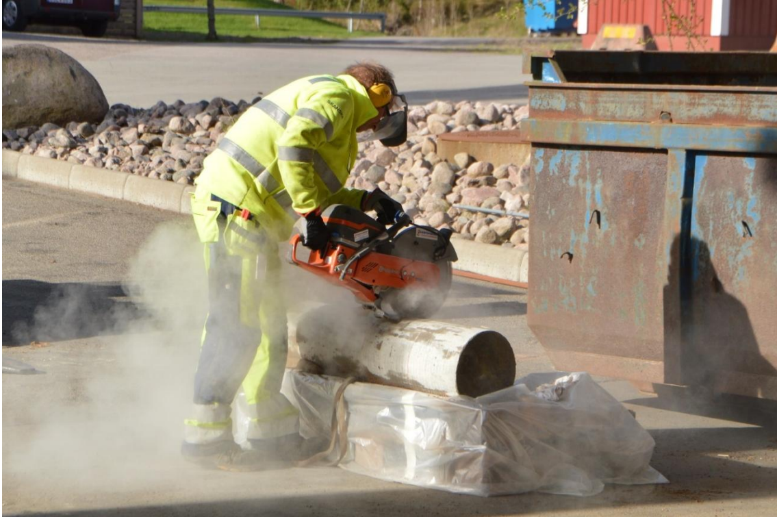
Figure 4-6. Sectioning of a concrete cylinder
