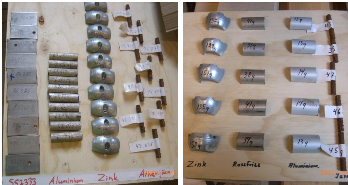
Figure 3-2. Metal objects used in the long-term corrosion studies. Metal objects for concrete cylinders installed in TASR and NASA2821A to the left and right respectively.
