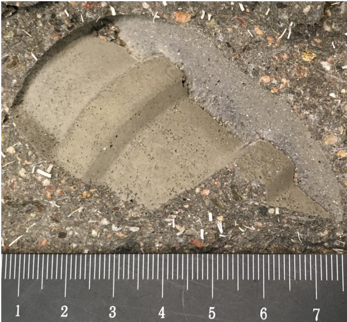
Figure 6-2. A concrete imprint of a zinc object from sample 10YW-Zn.
