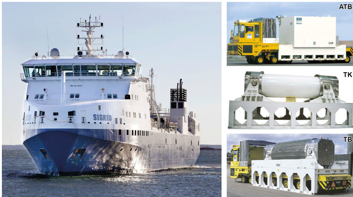
Figure 2-8. SKB's transport system currently consists of a ship ( m/s Sigrid ), terminal vehicles, and transport casks for short-lived radioactive waste (ATB), core components (TK), and spent nuclear fuel (TB).
