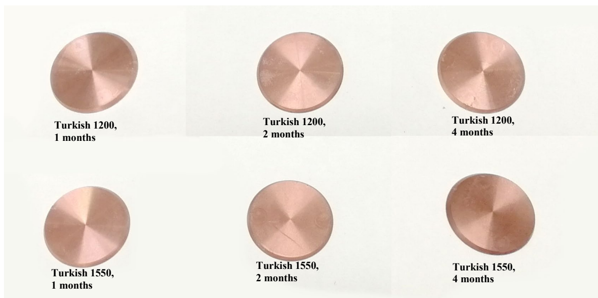
Figure 3-23. Copper discs from every test cell with Turkish bentonite after 1, 2 and 4 months.
