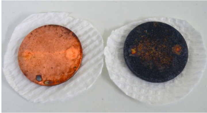
Figure 1-1. Copper surfaces from test cell 3 on the right and test cell 8 on the left analysed in a report by Bengtsson et al. (2015). Test cell 3 at saturated density of 1750 \text{ kg m}^{-3} and added SRB had 1598 kBq surface activity after 47 days. Test cell 8 at a saturated density of 2000 \text{ kg m}^{-3} and added SRB after 0.2 days had 0.2 kBq surface activity.
