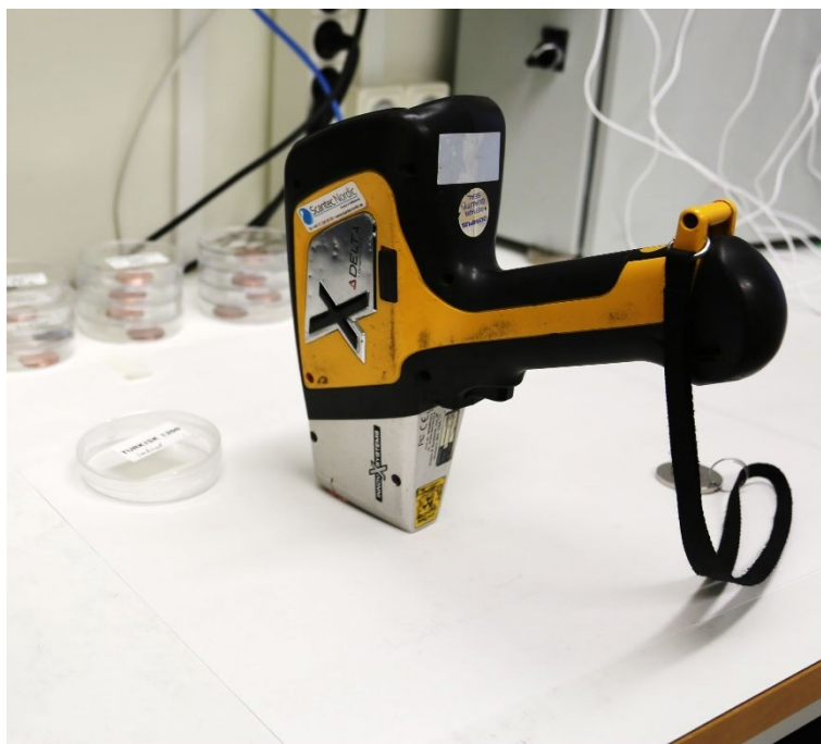
Figure 2-5. Analysis of sulphur on the copper disc with the Delta XRF analyser.
