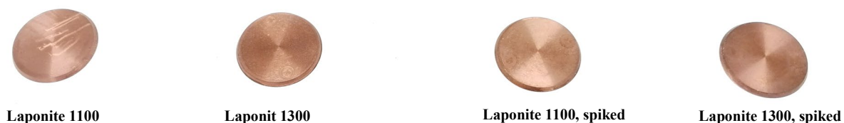
Figure 3-26. Copper discs from every test cell with Laponite, after 4 months.
