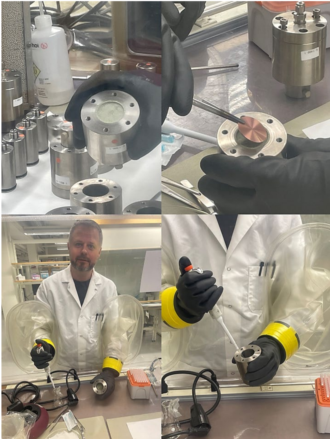
Figure 2-4. Addition of copper discs and lactate to the test cells in an anaerobic box.
