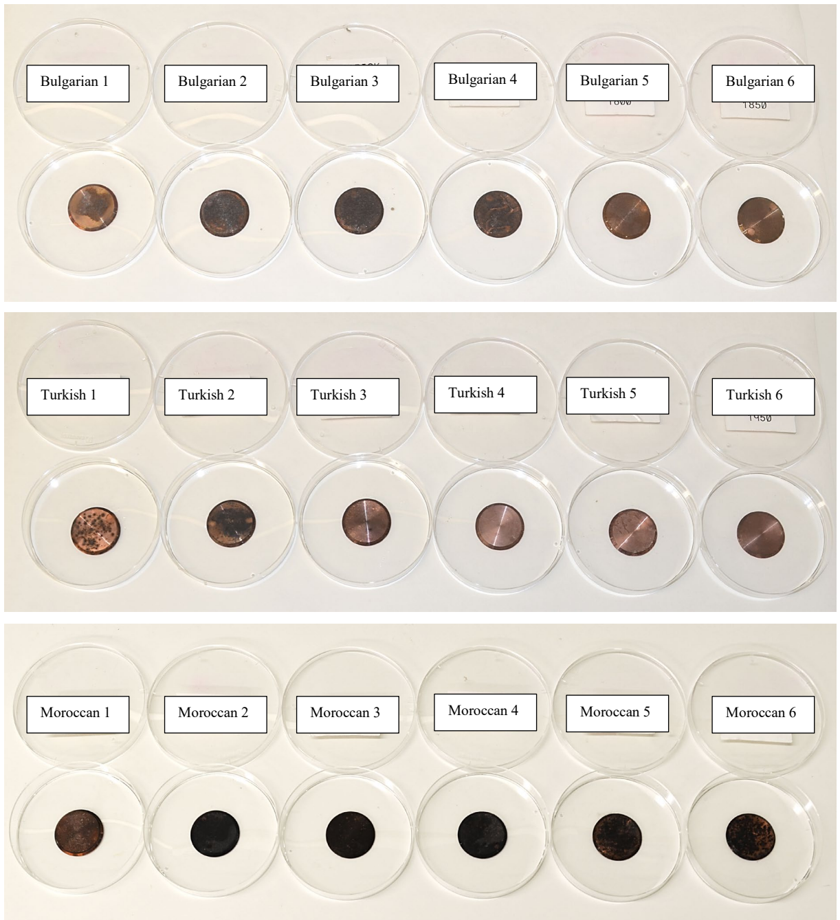
Figure 3-1. Copper discs from every test cell after 50 days.
