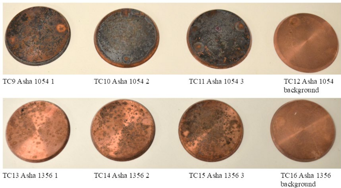
Figure 3-30. Copper discs from TC9 – 16. Numbers show dry density.
