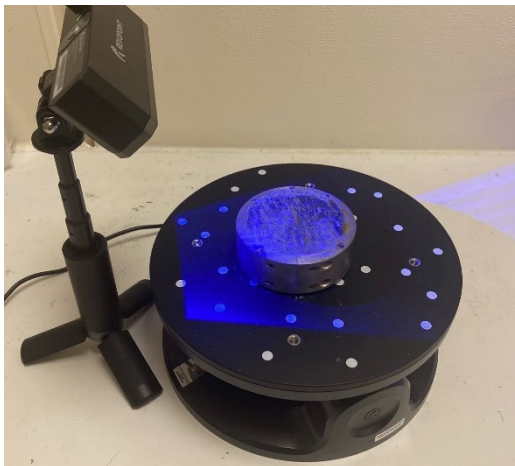
Figure 2-7. Laser scanning of fracture surfaces using a Revopoint MINI 3D Scanner.
