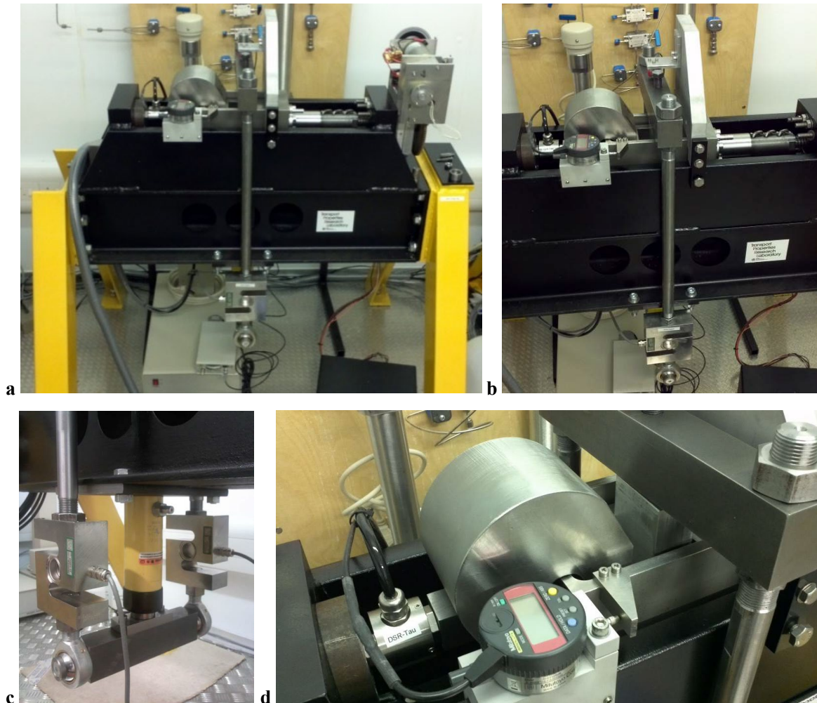
Figure 2-2. Components of the Direct Shear Rig. a) Photo of the complete apparatus; b) Loading frame with normal load cells at the bottom; c) normal load ram (yellow); d) sample assembly, shear load cell and Mitutoyo Digimatic Indicator (note the Mitutoyo device was replaced with a LVDT for this study).
