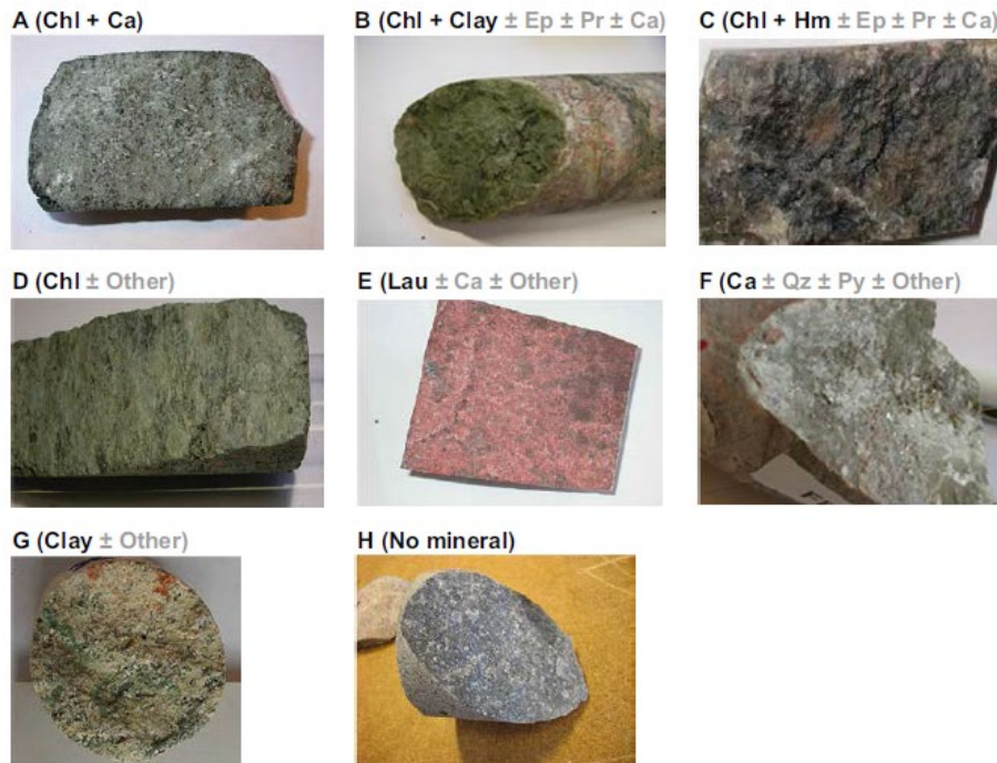
Figure 4-1. Typical fracture surfaces of Forsmark drill core samples. Mineral abbreviations are as follows: chlorite (Chl), calcite (Ca), epidote (Ep), hematite (Hm), laumontite (Lau), prehnite (Pr), pyrite (Py), quartz (Qz). Reproduced from Crawford and Löfgren (2019, Figure 4-3).
