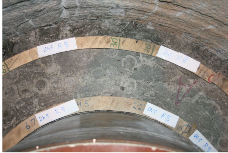
Figure 3-5. Graduated rulers were placed towards the canister and the rock surface to facilitate the determination of the sample positions. (Johannesson 2014).
