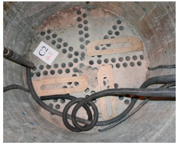
Figure 3-1. Left: The core drilling machines standing on the tunnel floor. Right: Holes from cores taken from a buffer block. (Johannesson 2014).
