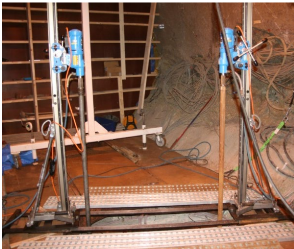
Figure 3-1. Left: The core drilling machines standing on the tunnel floor. Right: Holes from cores taken from a buffer block. (Johannesson 2014).
