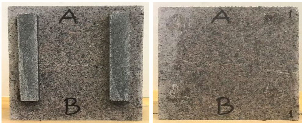
Figure 2-3. Sample for hydromechanically coupled flow test with support for transport (left), and without support (right).
