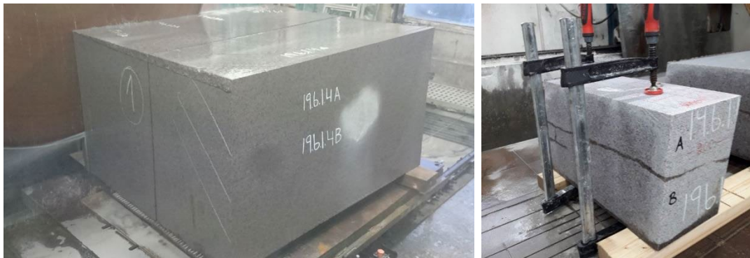
Figure 2-2. (left) Block 19.6.1.4 from which the sample is cut. (right) Slab of 19.6.1.4 block from which the 200 x 200 x 250 mm 3 is cut from.
