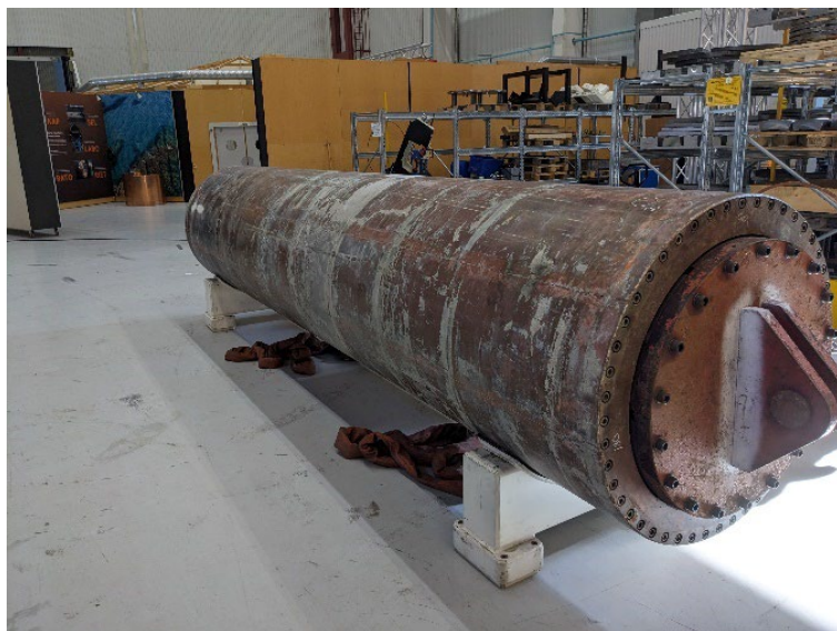
Figure 2. Copper canister from which exposed samples were obtained.
