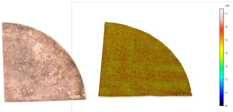
*Figure 7-84. Surface characterization of exposed and pickled sample C7-1 (bottom side).*
