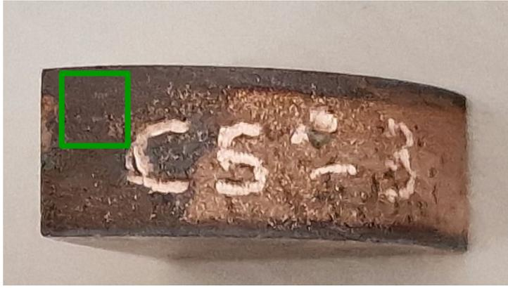
**Figure 3-1.** Blackened edge observed on sample C5-3.
