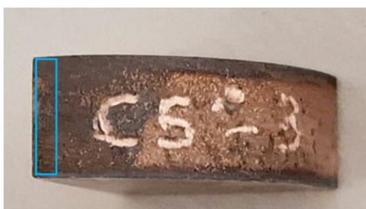
**Figure 3-14.** Side of specimen C5-3. The blue rectangle indicates the area where infrared spectroscopy measurements were performed.
