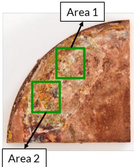
*Figure 7-161. Sample C8-3. The marked areas correspond to approximately the examined sites using SEM/EDS.*
