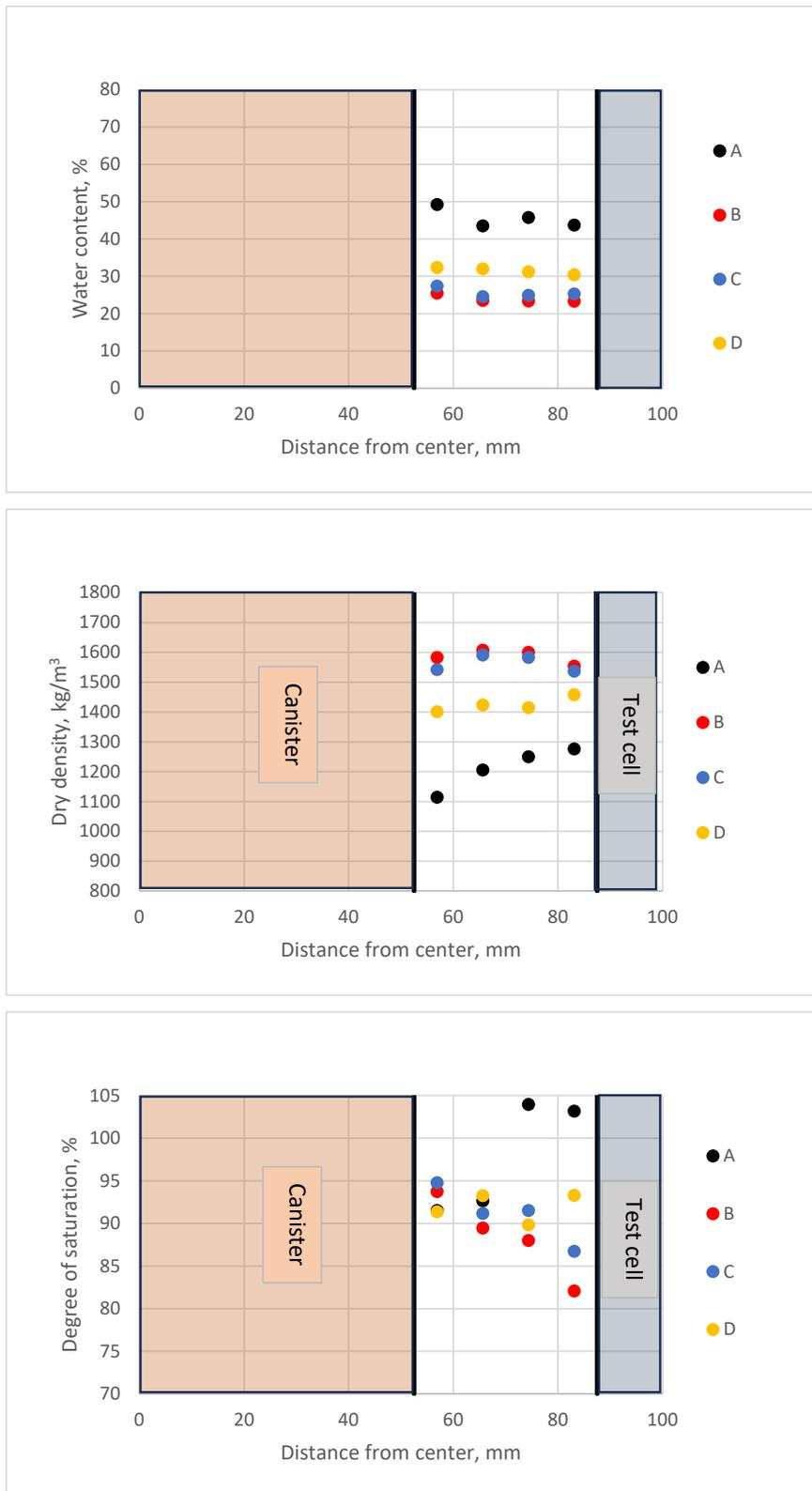
**Figure 6-14.** Results from measurements in sample section L2 (along canister) in Test 2. Upper: Water content plotted versus distance from the centre. Middle: Dry density plotted versus distance from the centre. Lower: Degree of saturation plotted versus distance from the centre.
