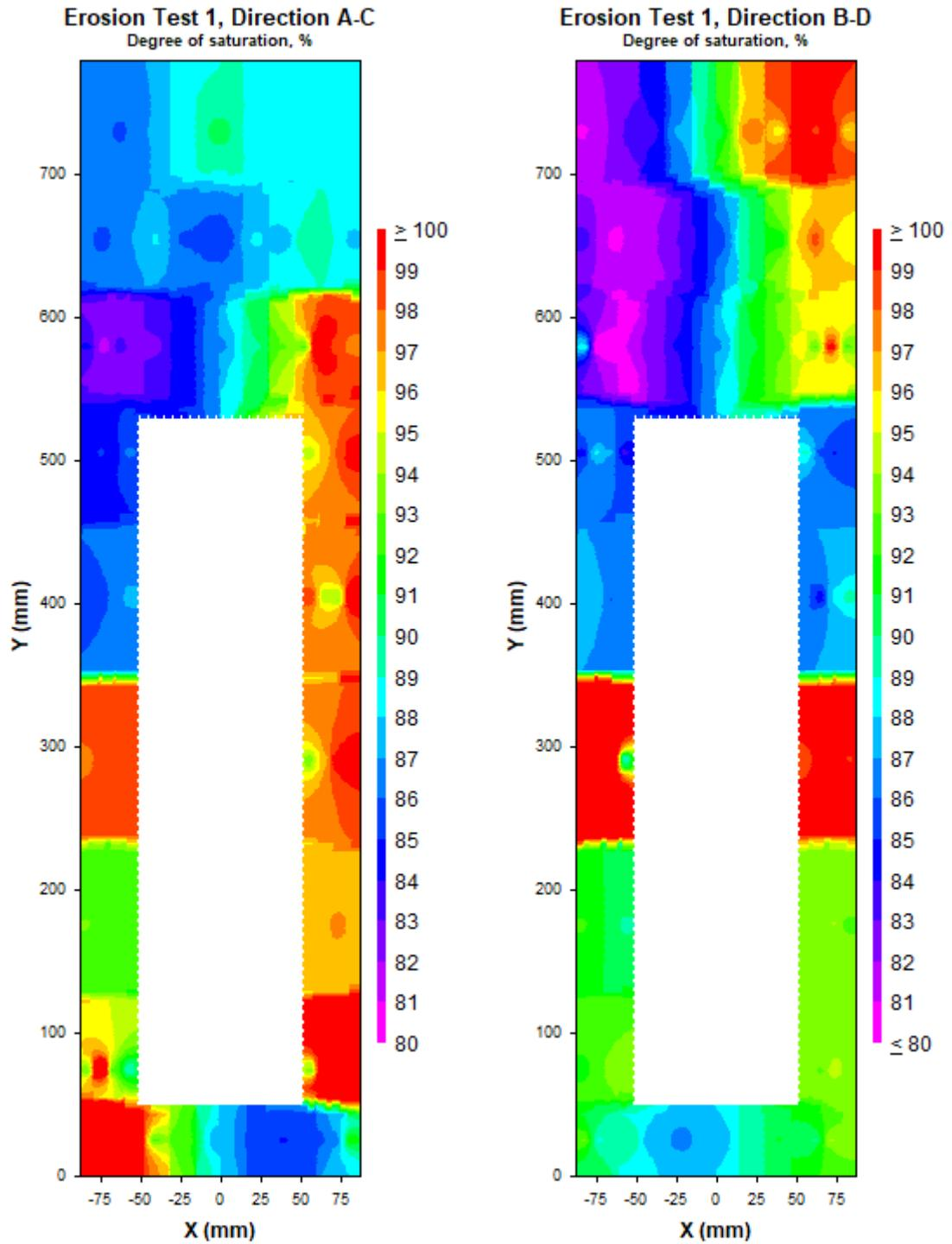
**Figure 5-30.** Contour plots showing the degree of saturation distribution in the four sampled directions (A, B, C, and D) of the deposition hole in Test 1.
