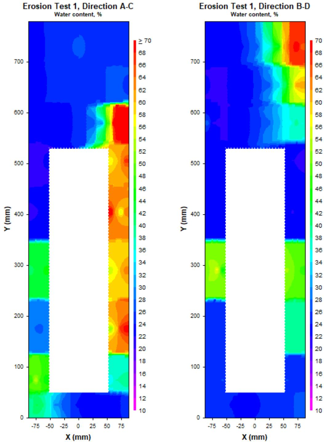
**Figure 5-28.** Contour plots showing the water content distribution in the four sampled directions (A, B, C, and D) of the deposition hole in Test 1.
