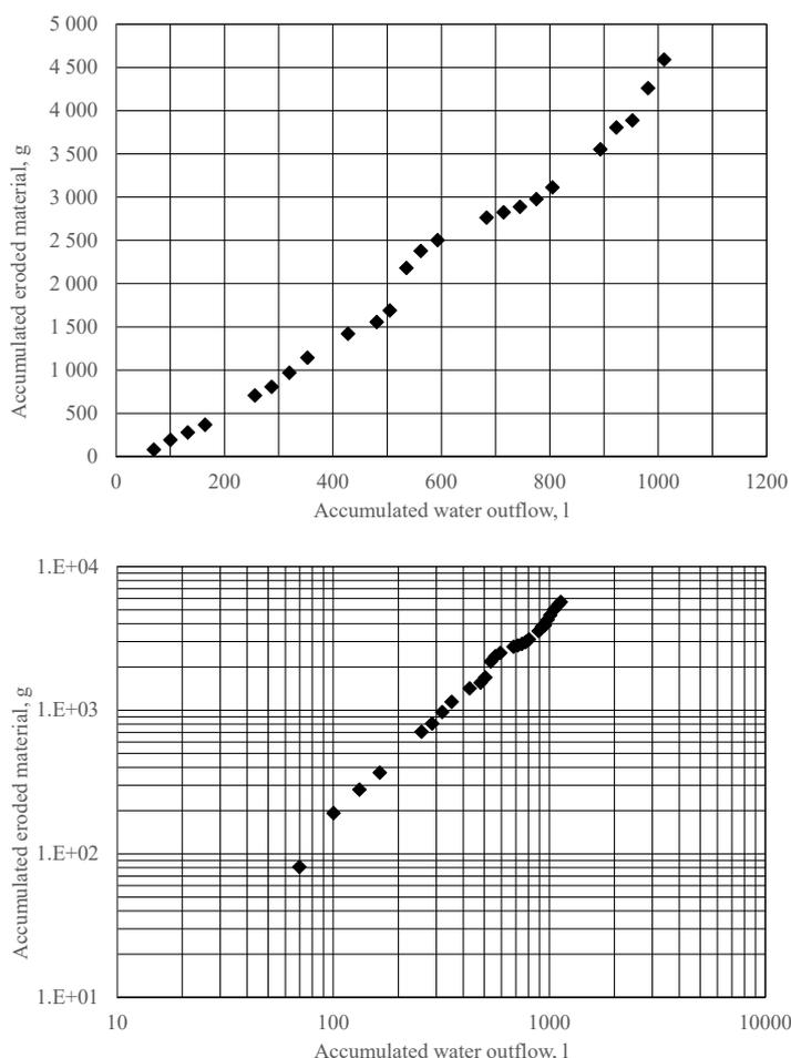
**Figure 6-3.** The accumulated eroded material plotted versus the accumulated water outflow for Test 2. Upper: The results presented in a lin-lin graph. Lower: The results presented in a log-log graph.
