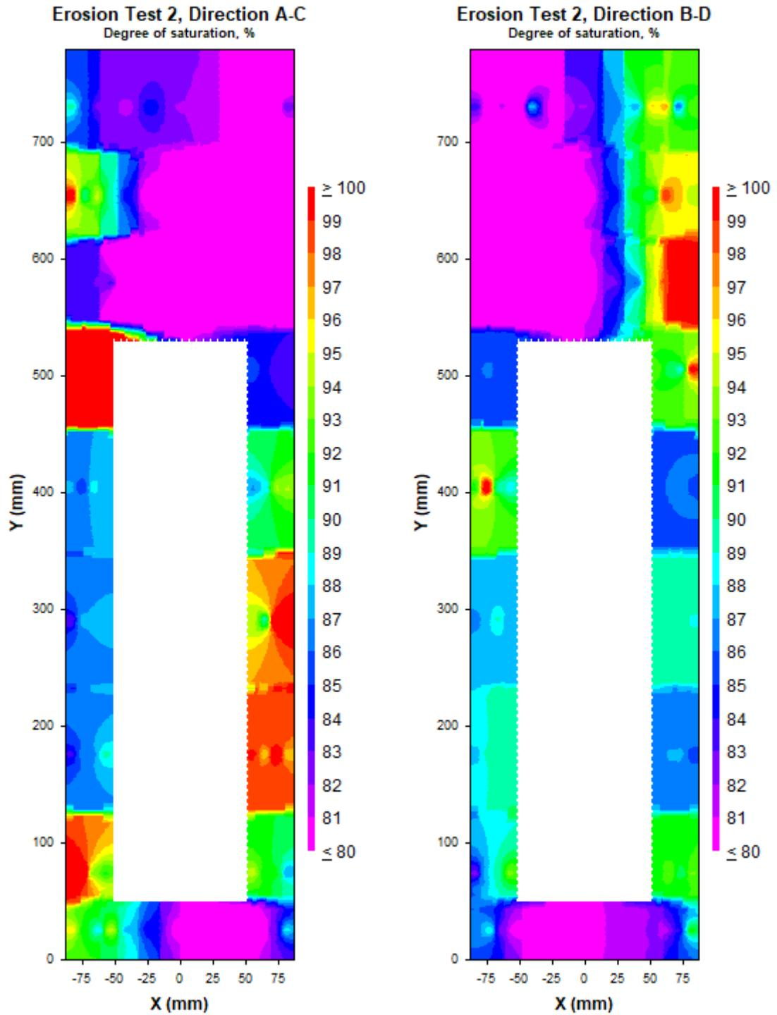
**Figure 6-24.** Contour plots showing the degree of saturation distribution in the four sampled directions (A, B, C, and D) of the deposition hole in Test 2.
