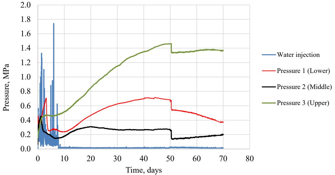
**Figure 5-7.** Applied water injection pressure (blue line) and radial total pressure for Test 1, registered at three levels in the deposition hole (red, black and green lines) plotted versus time.
