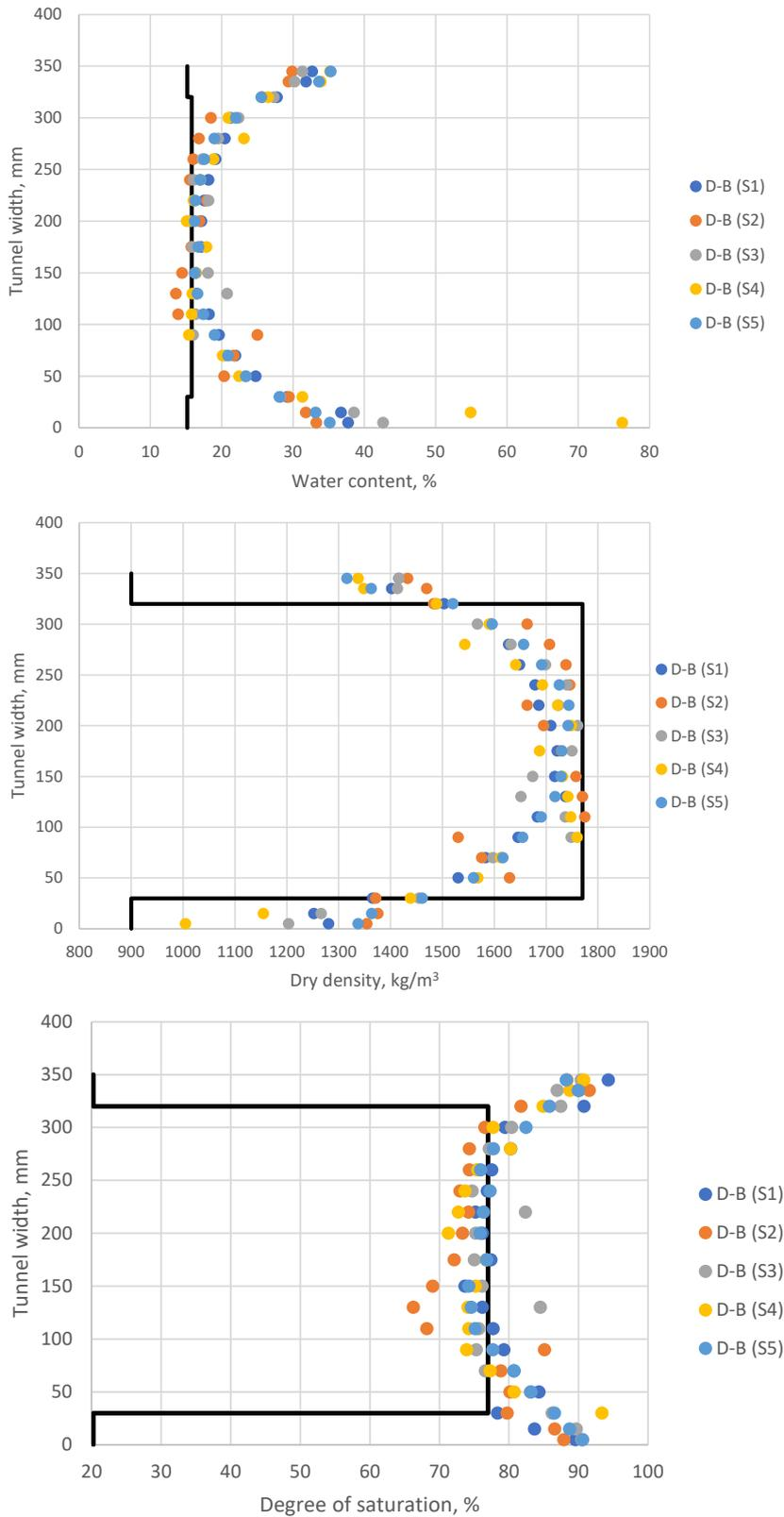
**Figure 6-10.** Water content (upper), dry density (middle), and degree of saturation (lower) along a horizontal line, positioned at the mid-height of the tunnel, at five different sections in Test 2, see Figure 5-8 and Figure 5-9. The black lines indicate the initial values. Sampling direction B upwards.
