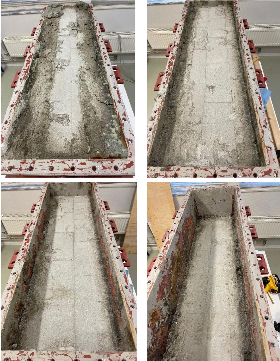
**Figure 6-8.** Test 2. Upper left: The top lid has been removed. Upper right: The first block layer has been removed. Lower left: The second block layer has been removed. Lower right: The bottom block layer.
