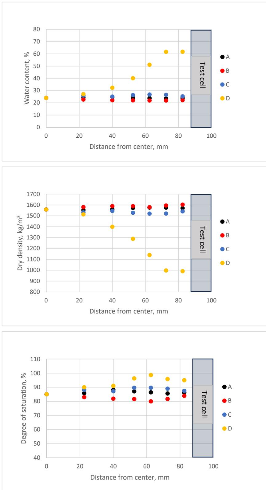
**Figure 5-26.** Results from measurements in sample section L8 (above canister) in Test 1. Upper: Water content plotted versus distance from the centre. Middle: Dry density plotted versus distance from the centre. Lower: Degree of saturation plotted versus distance from the centre.
