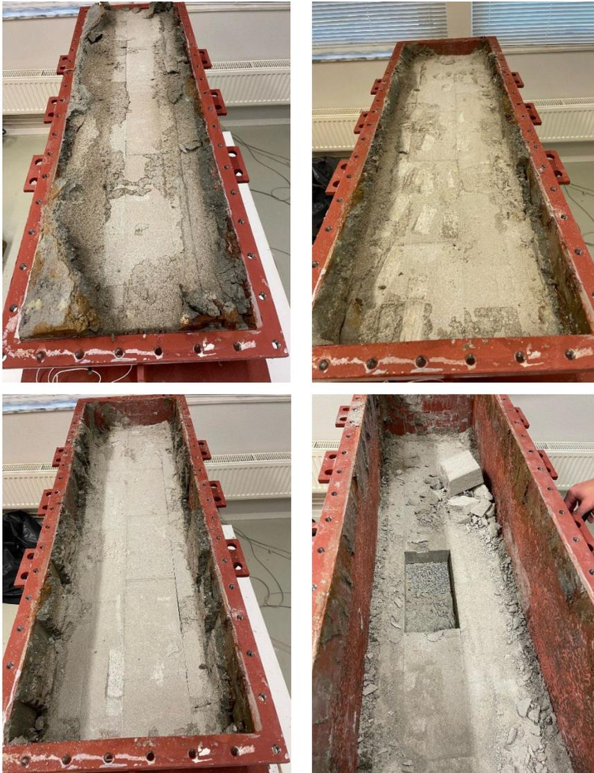
**Figure 5-13.** Test 1. Upper left: The top lid has been removed. Upper right: The first block layer has been removed. Lower left: The second block layer has been removed. Lower right: The bottom block layer. One block has been removed exposing the bottom pellet layer.
