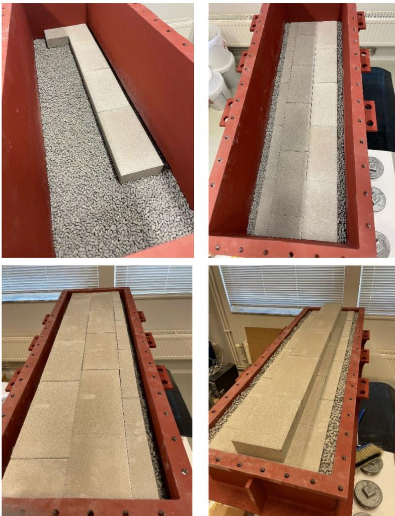
**Figure 5-2.** Photos taken in conjunction with the backfill installation. Upper left: The bottom pellet layer has been installed together with the first blocks. Upper right: The third block layer has been installed. Lower left: The sixth block layer have been completed. Lower right: The seventh block layer has been installed.
