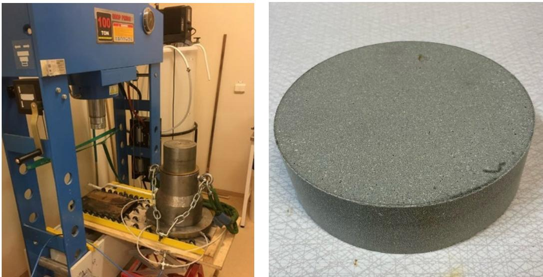
*Figure 4-1 Left: Manufacturing of blocks with an outer diameter of 175/173 mm using the 100-ton press at Clay Technology, Lund. Right: Photo showing a manufactured block.*
