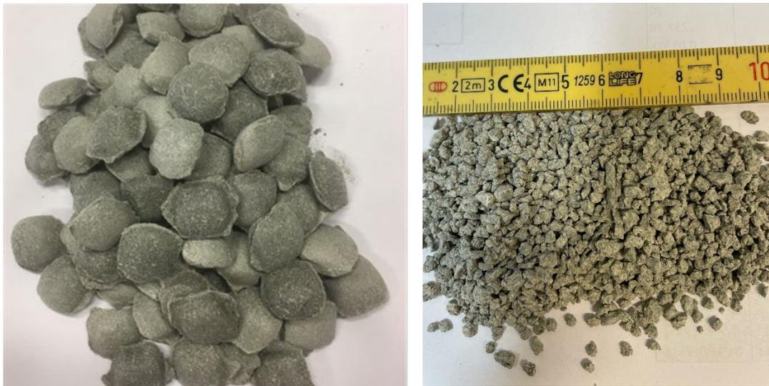
*Figure 4-3. Left: Photo showing compacted pellets. Right: Photo showing the compacted pellets after crushing.*
