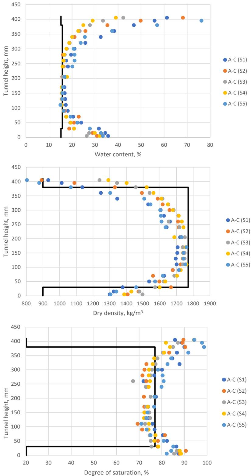
**Figure 6-9.** Water content (upper), dry density (middle), and degree of saturation (lower) along central vertical lines at five different sections in Test 2, see Figure 5-8 and Figure 5-9. The black lines indicate the initial values. Sampling direction A upwards.
