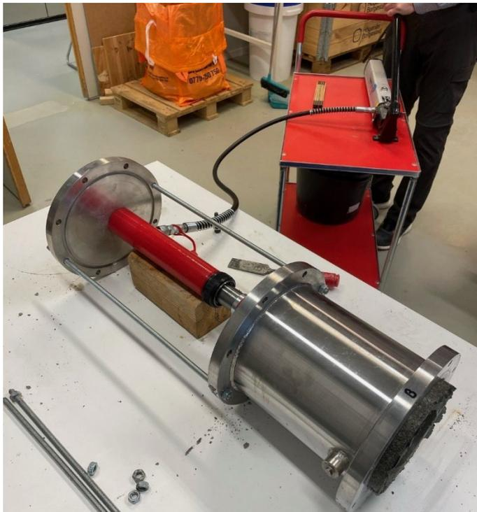
*Figure 5-18. The buffer was pushed out from the steel tube using a hydraulic piston. The photo shows the removal of the buffer in the section above the canister.*
