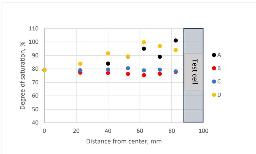
**Figure 6-20.** Results from measurements in sample section L8 (above canister) in Test 2. Upper: Water content plotted versus distance from the centre. Middle: Dry density plotted versus distance from the centre. Lower: Degree of saturation plotted versus distance from the centre.
