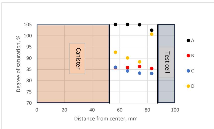
**Figure 6-18.** Results from measurements in sample section L6 (along canister) in Test 2. Upper: Water content plotted versus distance from the centre. Middle: Dry density plotted versus distance from the centre. Lower: Degree of saturation plotted versus distance from the centre.
