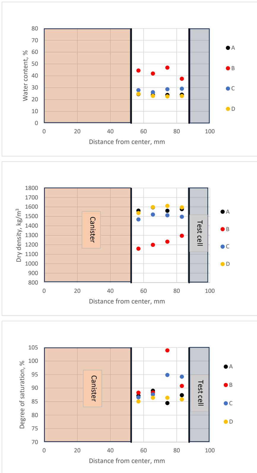
**Figure 6-17.** Results from measurements in sample section L5 (along canister) in Test 2. Upper: Water content plotted versus distance from the centre. Middle: Dry density plotted versus distance from the centre. Lower: Degree of saturation plotted versus distance from the centre.
