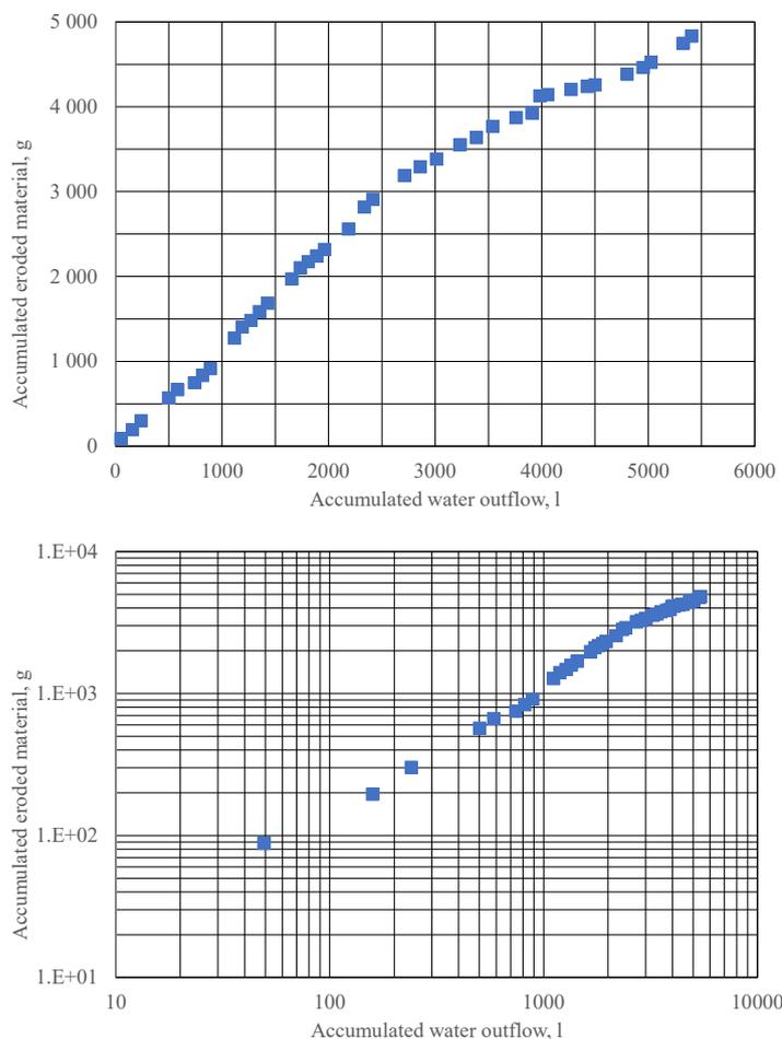
**Figure 5-5.** The accumulated eroded material plotted versus the accumulated water outflow for Test 1. Upper: The results presented in a lin-lin graph. Lower: The results presented in a log-log graph.
