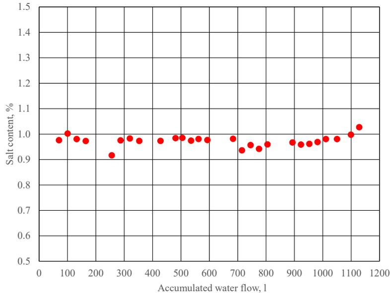
**Figure 6-2.** Results from measurements of the salt content plotted versus the accumulated water flow for Test 2.
