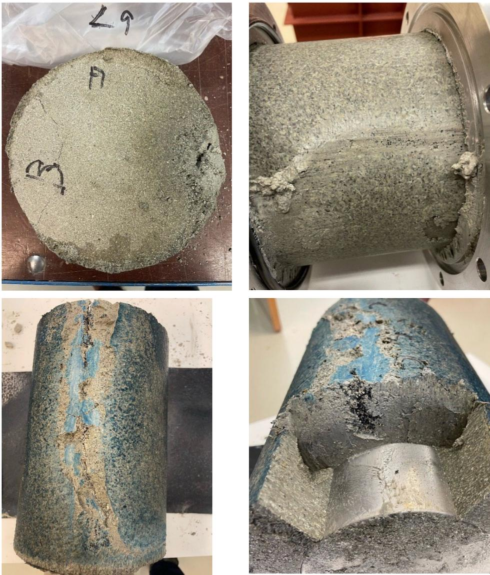
**Figure 5-16.** Test 1. Upper left: Photo showing the block including sampling section L9. The most wetted part was clearly in direction D. Upper right: Erosion channel on the buffer surface (approximately sampling section L8). Lower left: Erosion channel along the buffer (canister section). Note that the outer surface of the buffer has been discoloured by the rubber mat. Lower right: Cross-section of the erosion channel along the canister.
