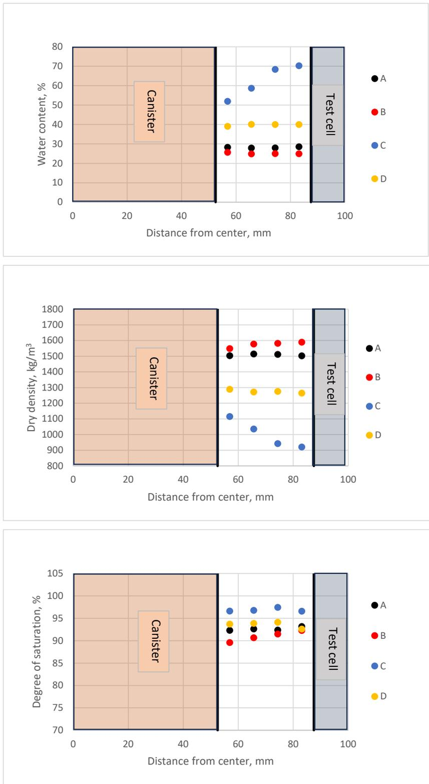
**Figure 5-21.** Results from measurements in sample section L3 (along canister) in Test 1. Upper: Water content plotted versus distance from the centre. Middle: Dry density plotted versus distance from the centre. Lower: Degree of saturation plotted versus distance from the centre.
