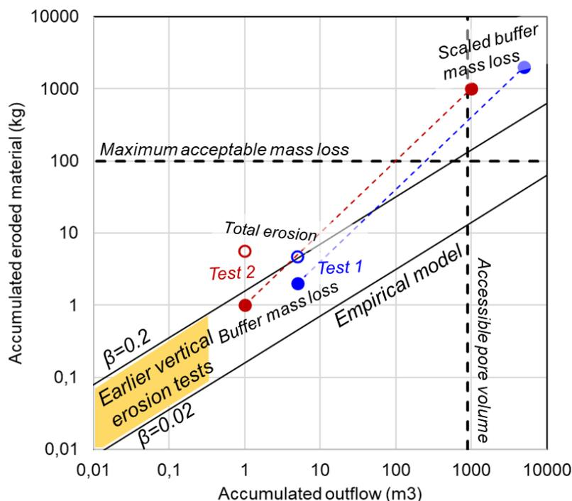
**Figure 7-2.** Estimation of buffer mass loss from a deposition hole which acts as the sole inflow point in an entire deposition tunnel: i) with empirical model, i.e. through extrapolation of data from earlier erosion tests; and ii) through scaling of experimental data from test presented in this study; Test 1 (blue) and Test 2 (red).
