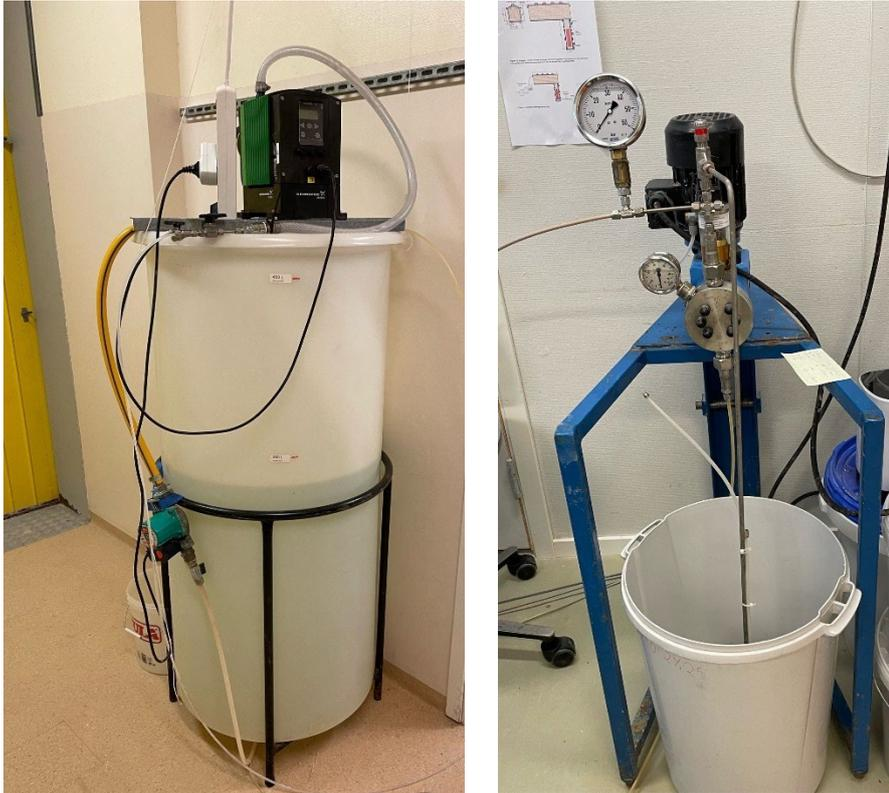
**Figure 3-4.** Left: Photo showing the dose pump positioned above the vessel with water. Right: Photo showing the high-pressure pump.
