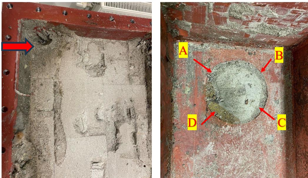
**Figure 5-12.** Left: Photo showing the corner where water flowing from the deposition hole have reached the upper corner of the tunnel in Test 1 (see corresponding photo of the tunnel ceiling in the photo above). Right: After removal of all the backfill, the upper part of the buffer in the deposition hole was exposed. The red arrows show the sampling directions of the buffer (direction A is almost at the same direction as the inflow point and also close to the pressure measurements).
