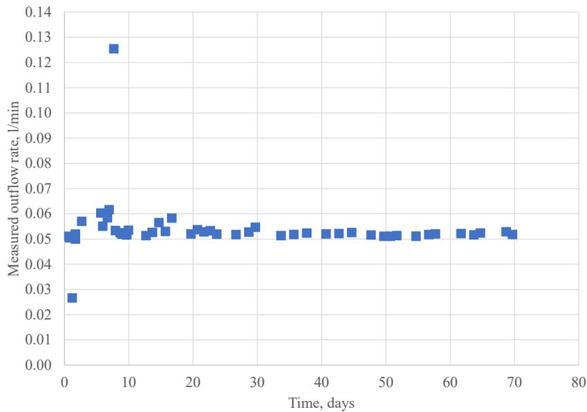
**Figure 5-3.** The measured outflow rate plotted versus time for Test 1. The inflow rate was set to 0.05 l/min.
