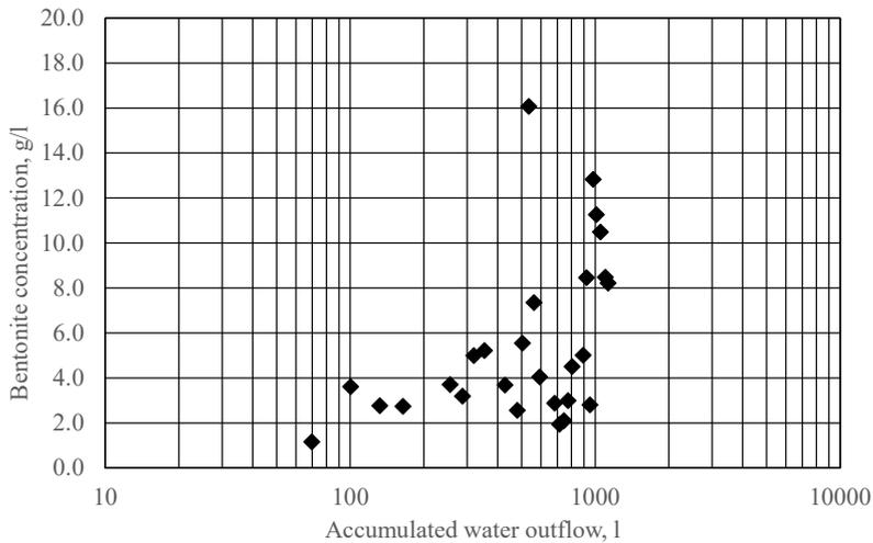
**Figure 6-4.** The bentonite concentration plotted versus the accumulated water outflow for Test 2.
