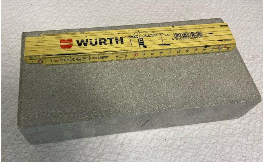
*Figure 4-2. Photo showing one of the backfill blocks used in the tests.*
