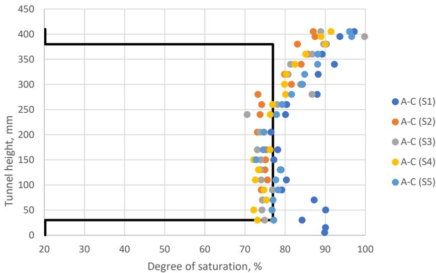
**Figure 5-14.** Water content (upper), dry density (middle), and degree of saturation (lower) along central vertical lines at five different sections in Test 1, see Figure 5-8 and Figure 5-9. The black lines indicate the initial values. Sampling direction A upwards.
