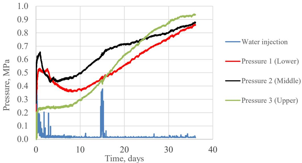
**Figure 6-5.** Applied water injection pressure (blue line) and radial total pressure for Test 2, registered at three levels in the deposition hole (red, black and green lines) plotted versus time.
