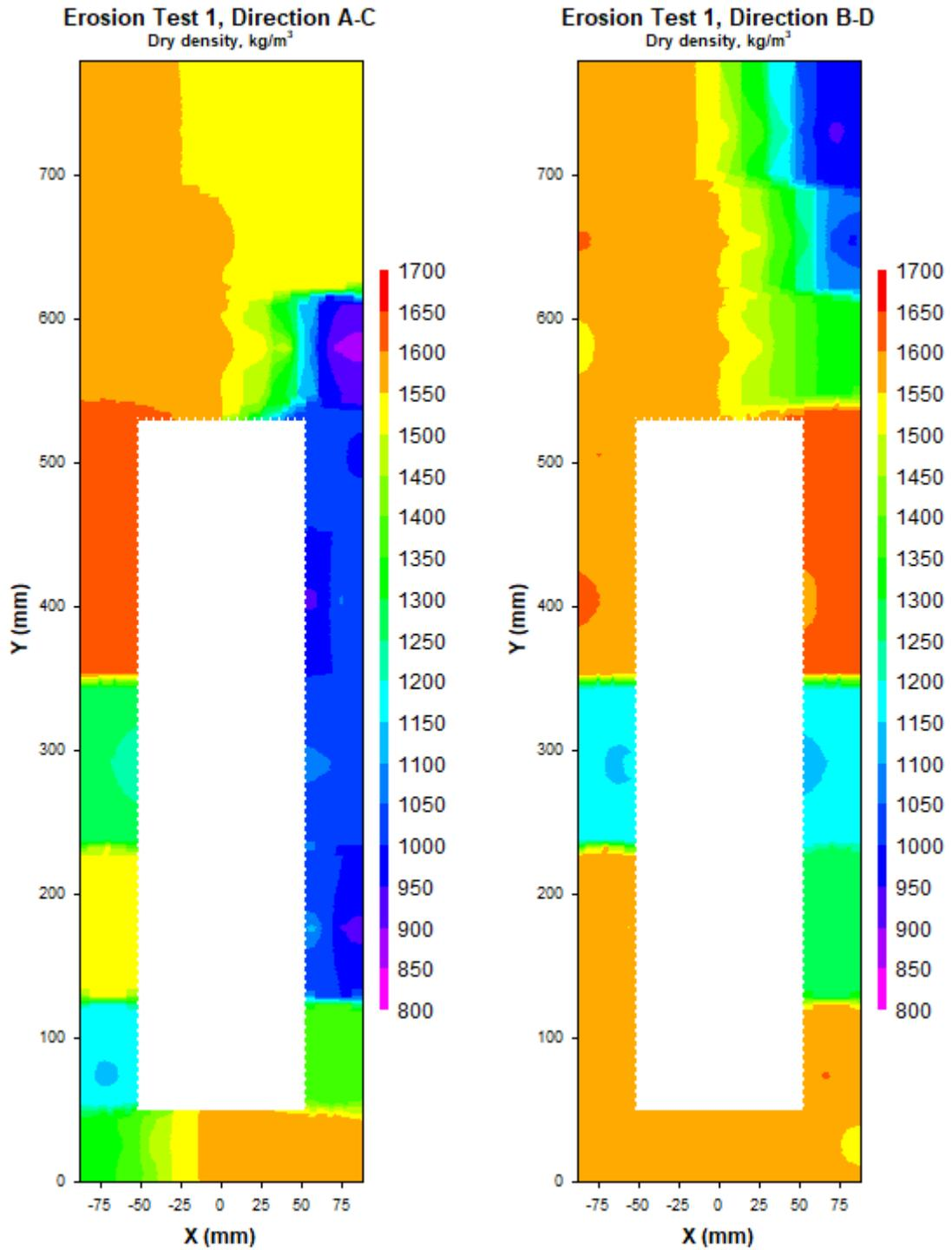
**Figure 5-29.** Contour plots showing the dry density distribution in the four sampled directions (A, B, C, and D) of the deposition hole in Test 1.
