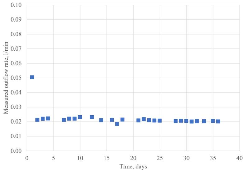
**Figure 6-1.** The measured outflow rate plotted versus time for Test 2. The inflow rate was at test start 0.05 l/min but was after 23 hours test duration decreased to 0.02 l/min.
