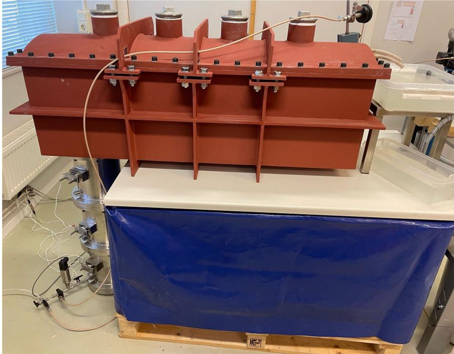
*Figure 3-3. Photo showing the test arrangement. The deposition tunnel was placed on a bench and the deposition hole was standing on the floor below (to the left in the photo). The sedimentation vessels can be seen to the right in the photo.*
