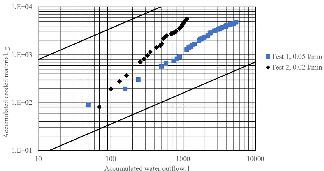
**Figure 7-1.** The accumulated eroded material plotted versus the accumulated outflow. The straight black lines describe a model of expected maximum and minimum accumulated eroded material (Sandén et al, 2008).
