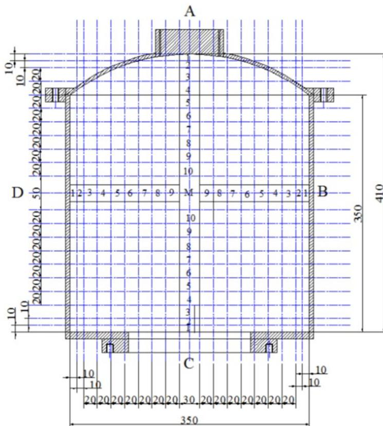
Figure 5-9. Planned sampling of the backfill. The picture shows the planned sampling in each of the cross-sections.
