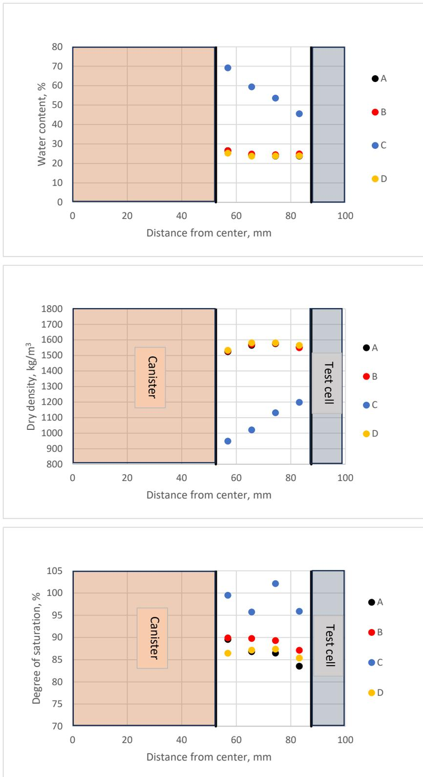
**Figure 6-15.** Results from measurements in sample section L3 (along canister) in Test 2. Upper: Water content plotted versus distance from the centre. Middle: Dry density plotted versus distance from the centre. Lower: Degree of saturation plotted versus distance from the centre.
