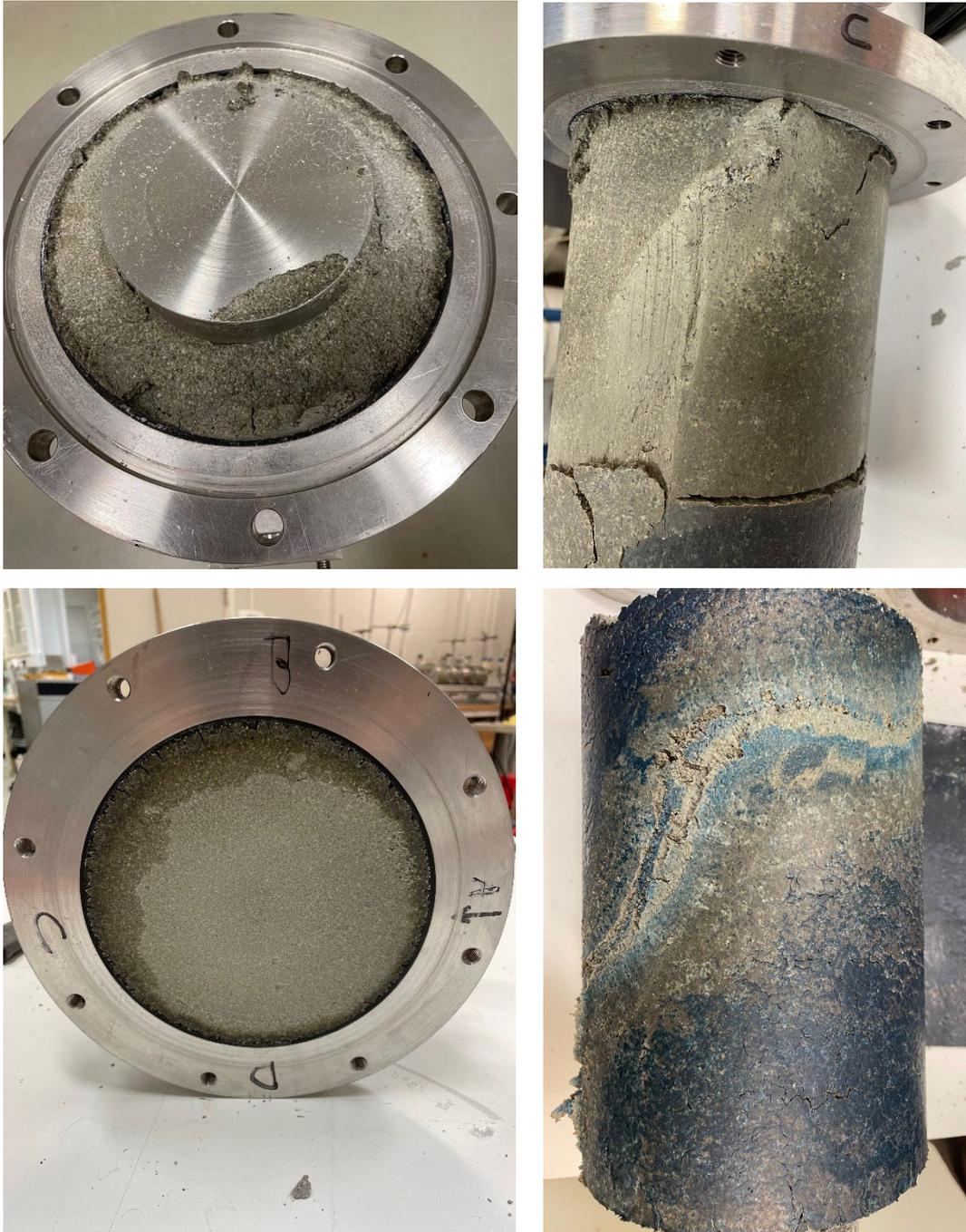
**Figure 6-11.** Test 2. Upper left: Photo showing the top of the canister. The wettest part can be seen as a dark field (between direction A and D). Upper right: Erosion channel on the buffer surface along the lower part of the canister. Lower left: Photo showing the bottom block from below. Lower right: Erosion channel along the upper part of the canister. Note that the outer surface of the buffer has been discoloured by the rubber mat.
