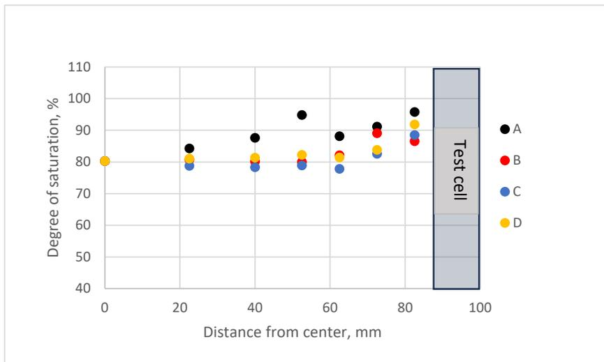
**Figure 6-13.** Results from measurements in sample section L1 (bottom block) in Test 2. Upper: Water content plotted versus distance from the centre. Middle: Dry density plotted versus distance from the centre. Lower: Degree of saturation plotted versus distance from the centre.
