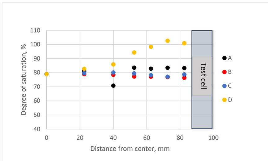
**Figure 6-19.** Results from measurements in sample section L7 (above canister) in Test 2. Upper: Water content plotted versus distance from the centre. Middle: Dry density plotted versus distance from the centre. Lower: Degree of saturation plotted versus distance from the centre.
