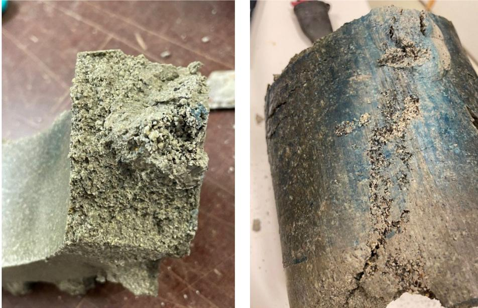
**Figure 6-12.** Photos showing close-ups of the erosion channel in Test 2. The finest clay particles have eroded away leaving the coarser grains left in the channel.
