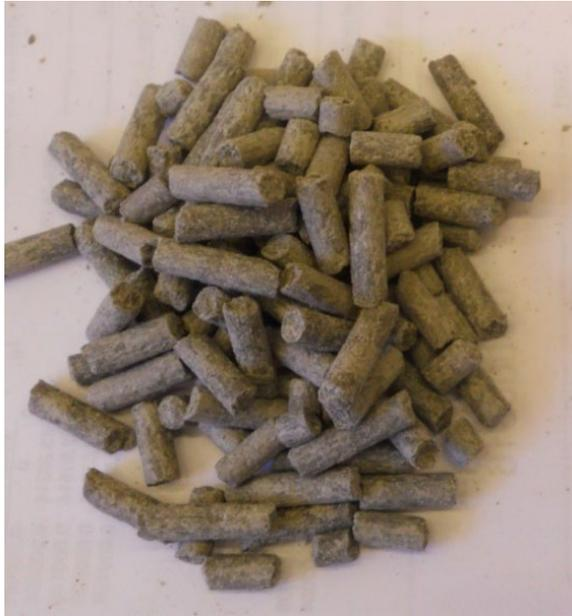
*Figure 4-4. Photo showing pellets manufactured by extrusion.*
