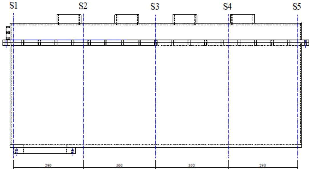
Figure 5-8. Planned sampling of the backfill. The sampling was made in five cross-sections, S1 to S5.
