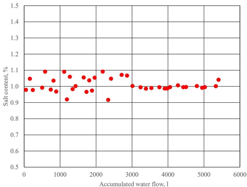
**Figure 5-4.** Results from measurements of the salt content plotted versus the accumulated water flow in Test 1.
