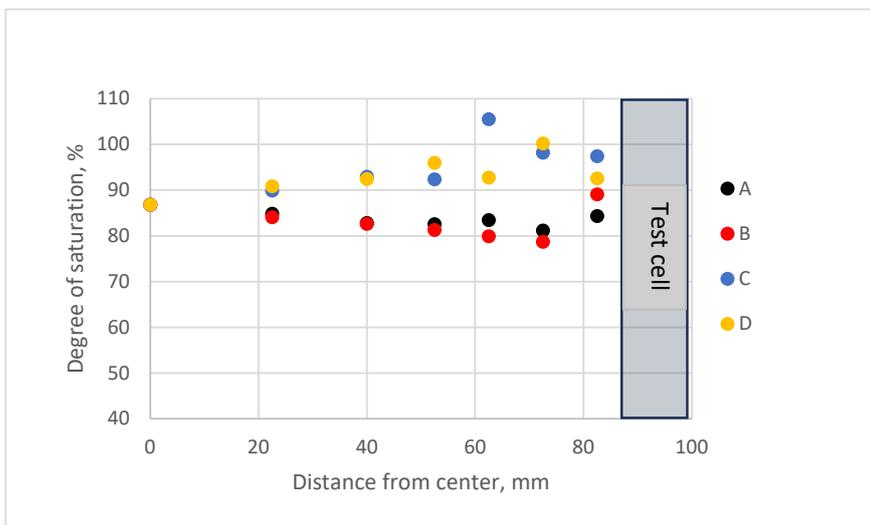
**Figure 5-25.** Results from measurements in sample section L7 (above canister) in Test 1. Upper: Water content plotted versus distance from the centre. Middle: Dry density plotted versus distance from the centre. Lower: Degree of saturation plotted versus distance from the centre.
