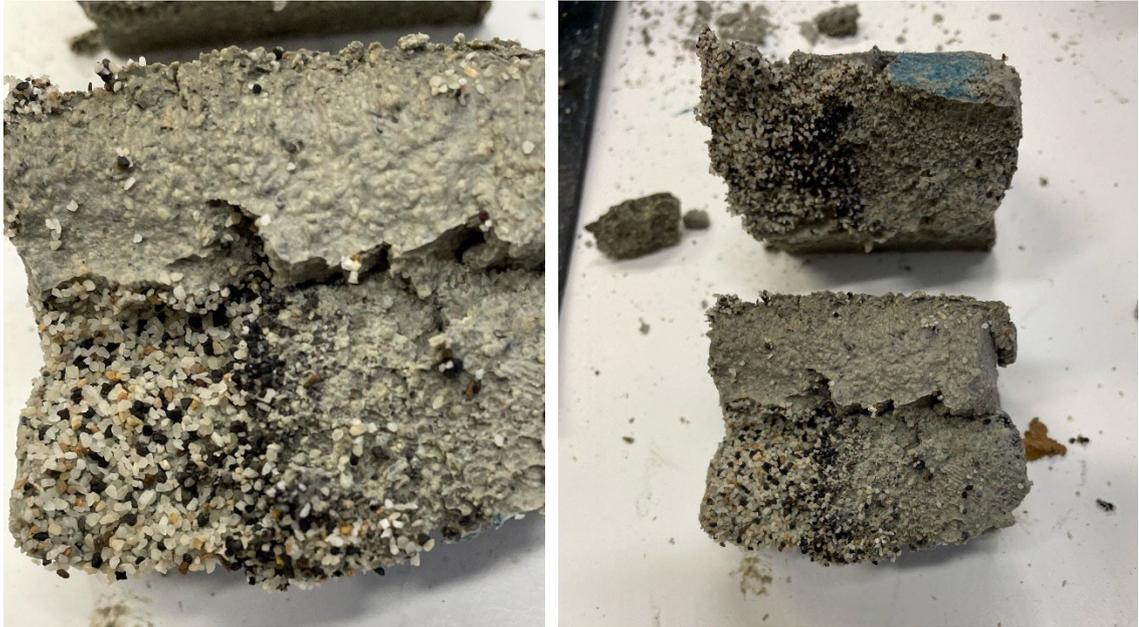
*Figure 5-17. Photos showing close-ups of the erosion channel in Test 1. The finest clay particles have eroded away leaving the coarser grains left in the channel.*
