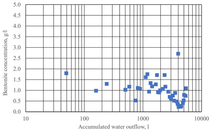
**Figure 5-6.** The bentonite concentration plotted versus the accumulated water outflow for Test 1.
