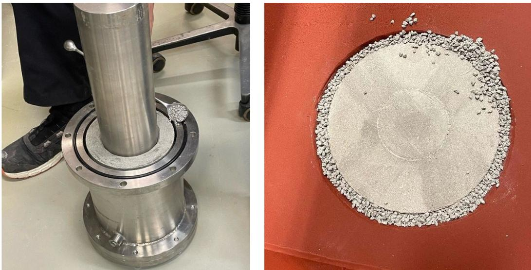
**Figure 5-1.** Photos taken in conjunction with the preparation of the deposition hole. Left: Installation of pellets around a ring-shaped block. Right: The deposition hole has been attached to the tunnel floor and the last buffer block has been installed together with the pellets.
