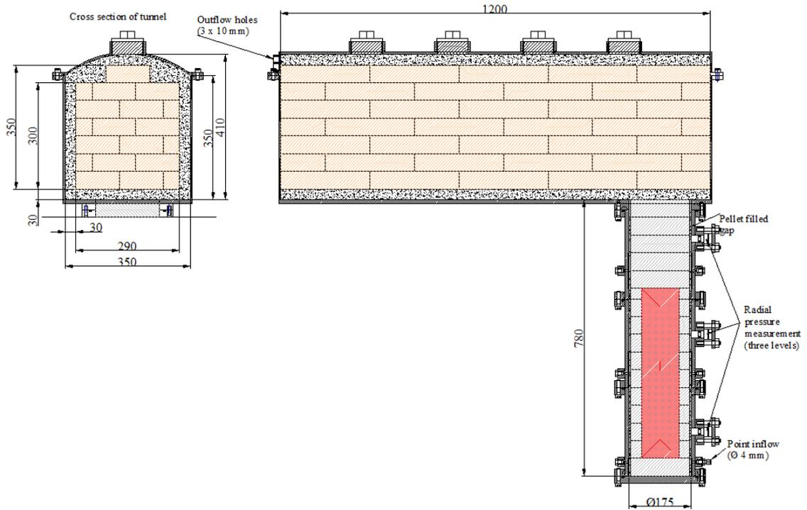
**Figure 3-1.** Schematic overview showing the design of the test equipment. The drawing up to the left shows a cross section of the deposition tunnel and shows also the backfill block stacking pattern.
