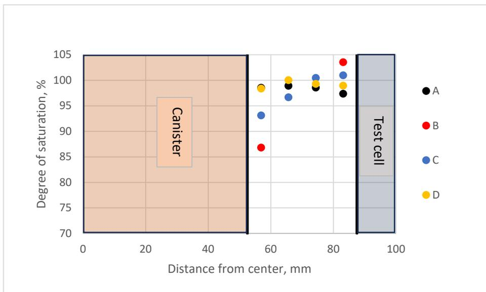
**Figure 5-22.** Results from measurements in sample section L4 (along canister) in Test 1. Upper: Water content plotted versus distance from the centre. Middle: Dry density plotted versus distance from the centre. Lower: Degree of saturation plotted versus distance from the centre.
