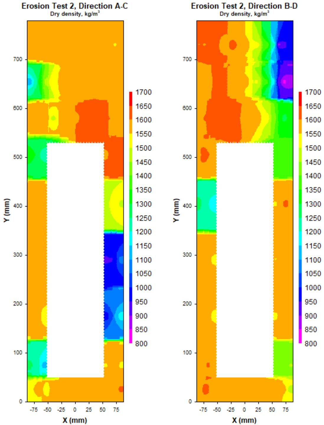
**Figure 6-23.** Contour plots showing the dry density distribution in the four sampled directions (A, B, C, and D) of the deposition hole in Test 2.
