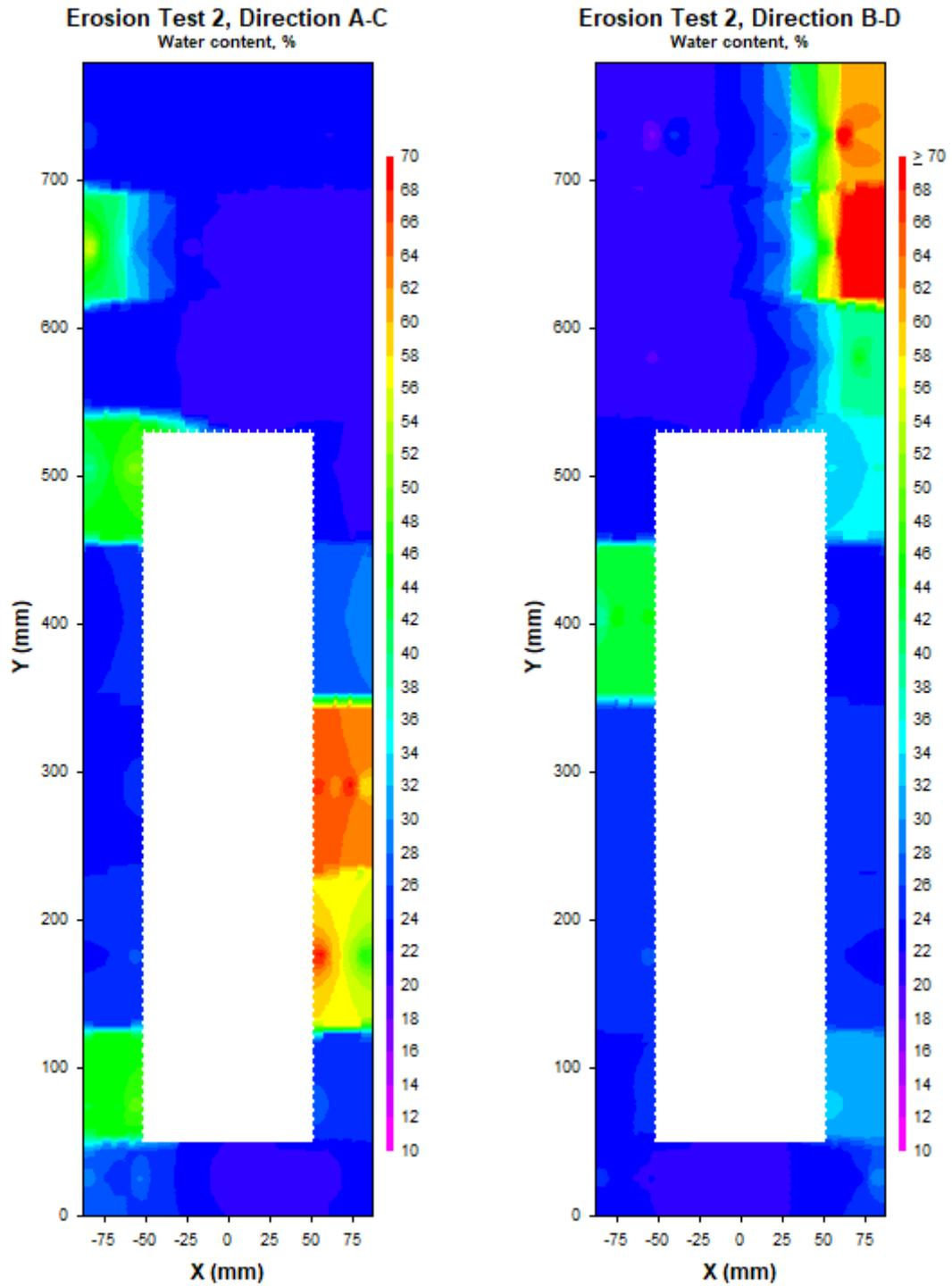
*Figure 6-22. Contour plots showing the water content distribution in the four sampled directions (A, B, C, and D) of the deposition hole in Test 2.*
