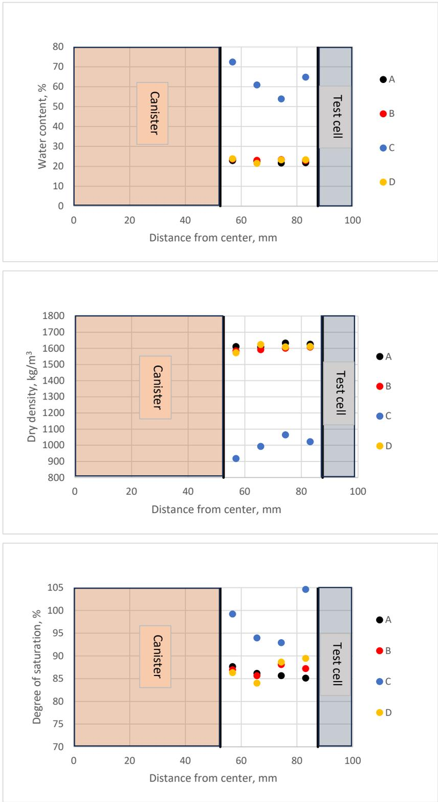
**Figure 5-23.** Results from measurements in sample section L5 (along canister) in Test 1. Upper: Water content plotted versus distance from the centre. Middle: Dry density plotted versus distance from the centre. Lower: Degree of saturation plotted versus distance from the centre.
