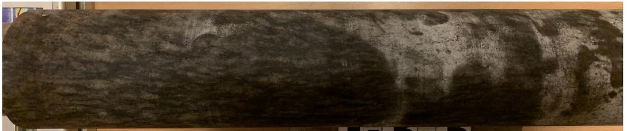
*Figure A1-13. Photo of overcore sample 1:3:3 taken at position of strain rosette 2.*
