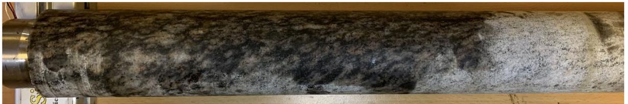
*Figure A1-18. Photo of overcore sample 1:4:4 taken at position of strain rosette 1.*
