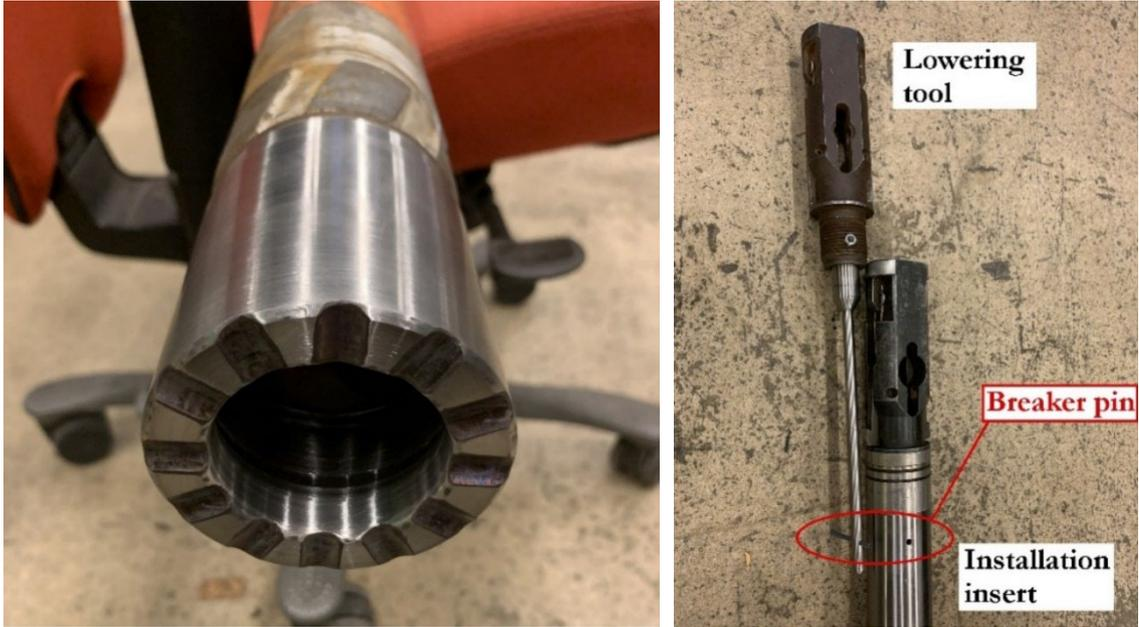
**Figure 2-3.** Left: Drill bit adapter for the CORAC core barrel. Right: The lowering tool for the installation insert. Once the installation insert has latched in the core barrel, the retrieval of the lowering tool requires pulling off a breaker pin, thus providing an indication that the installation insert is correctly installed in the core barrel.
