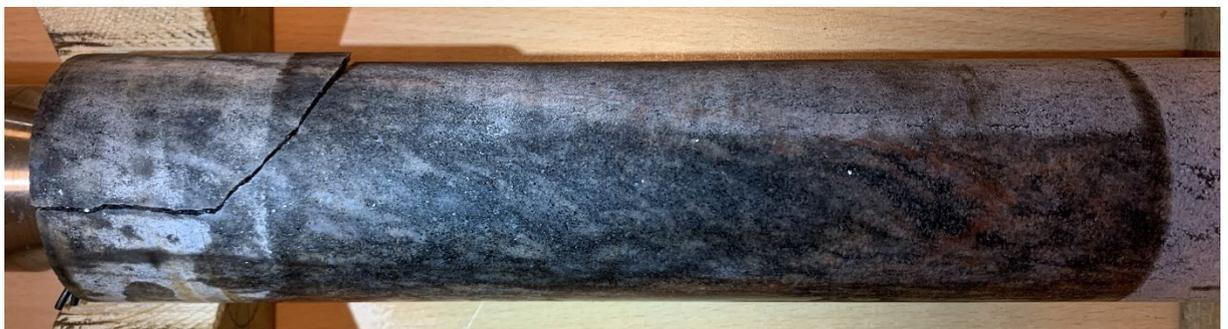
*Figure A1-6. Photo of overcore sample 1:2:2 taken at position of strain rosette 1.*
