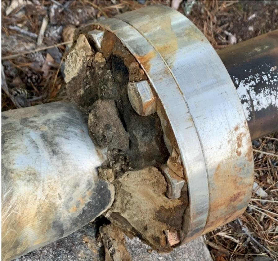
*Figure 1-3. Mud cake visible on the cone, placed in the intersection between the slim and large diameter parts of the borehole. Based on the traces along the cone assembly, a mud cake extending at least 2.1 m above the bottom plate was clearly visible.*
