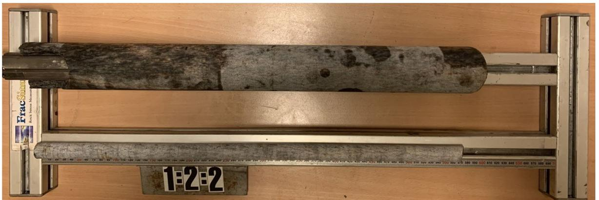
*Figure A1-5. Pilot 1:2:2 drilled between 563.18-563.90 mbl and overcore sample drilled between 563.18-563.81 mbl.*
