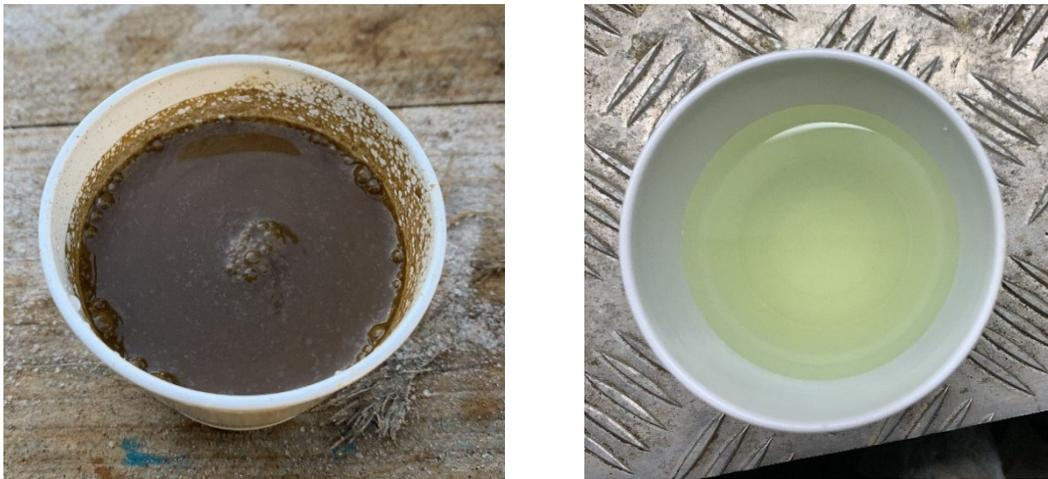
*Figure 1-2. Water sample taken before and after the cleaning operations in borehole KFM24.*
