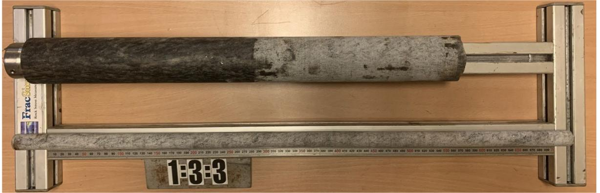
*Figure A1-11. Pilot 1:3:3 drilled between 563.94-564.69 mbl and overcore sample drilled between 563.97-564.59 mbl.*
