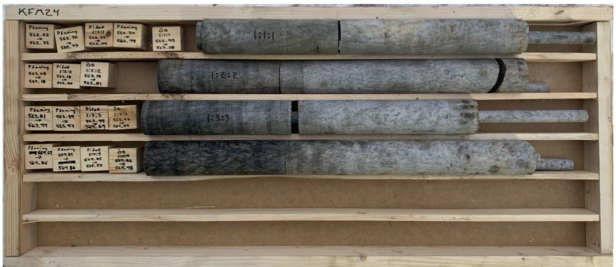
Figure A1-22. Core box after completed drilling in borehole KFM24.
