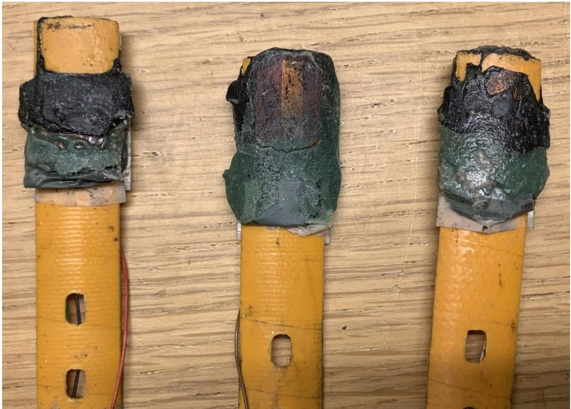
*Figure A1-9. Strain gauge assembly from Test 1:2:2, 563.32 mbl.*
