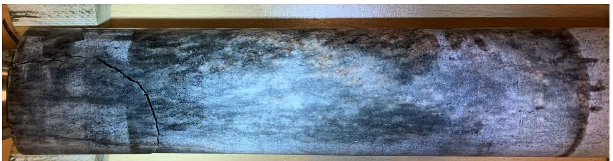
*Figure A1-7. Photo of overcore sample 1:2:2 taken at position of strain rosette 2.*
