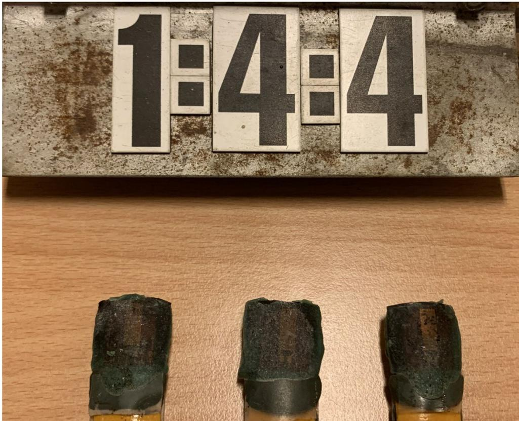
Figure A1-21. Strain gauge assembly from Test 1:4:4, 565.02 mbl.
