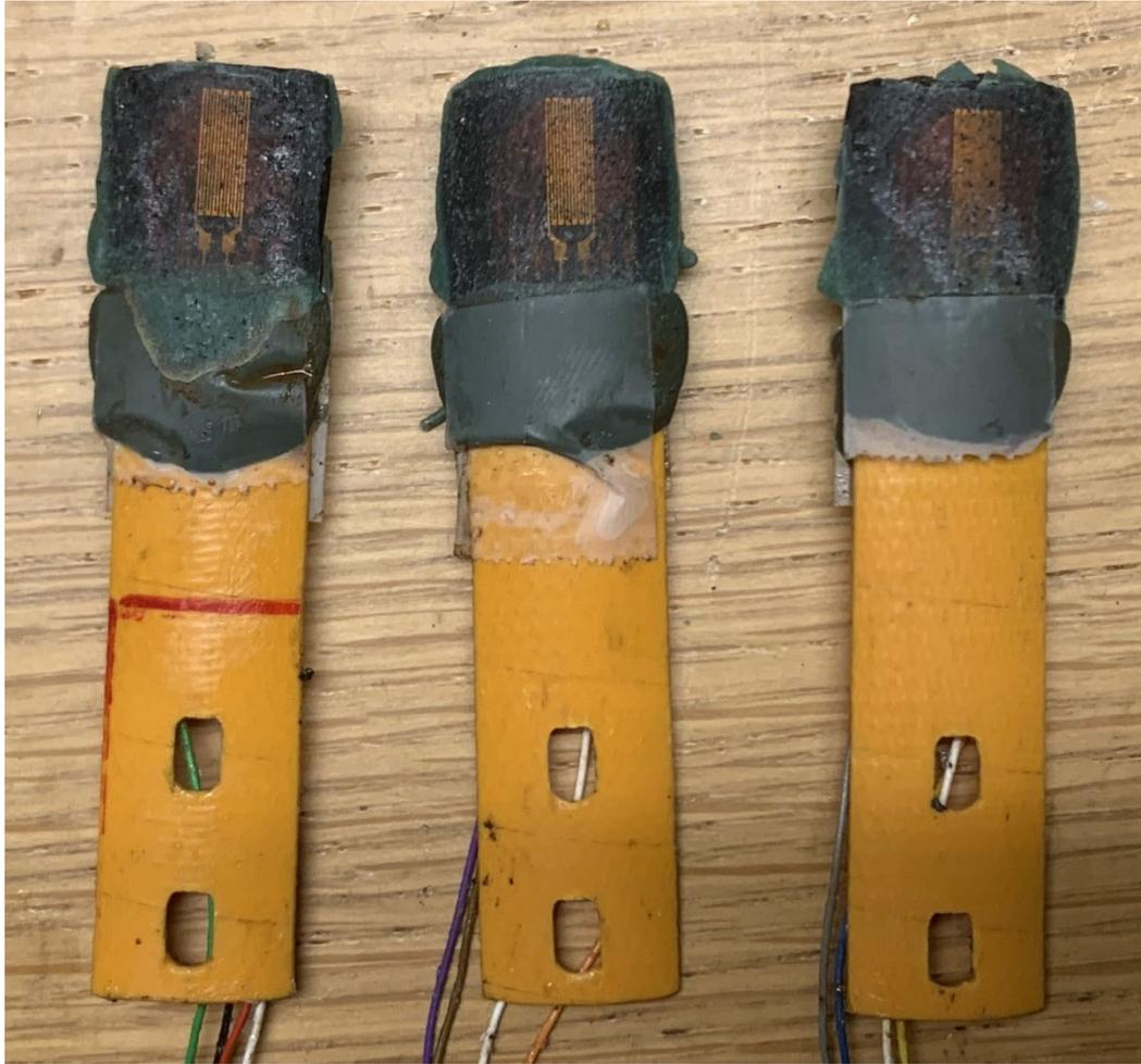
*Figure A1-15. Strain gauge assembly from Test 1:3:3, 564.13 mbl.*
