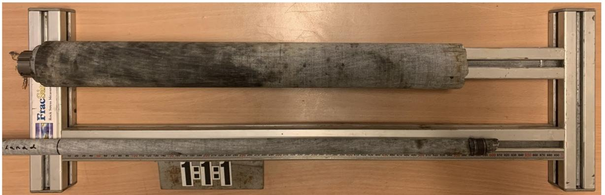
*Figure A1-2. Pilot 1:1:1 drilled between 562.37-563.09 mbl and overcore sample drilled between 562.49-563.08 mbl.*
