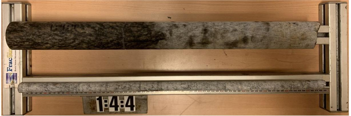
*Figure A1-17. Pilot 1:4:4 drilled between 564.86-565.57 mbl and overcore sample drilled between 564.86-565.48 mbl.*
