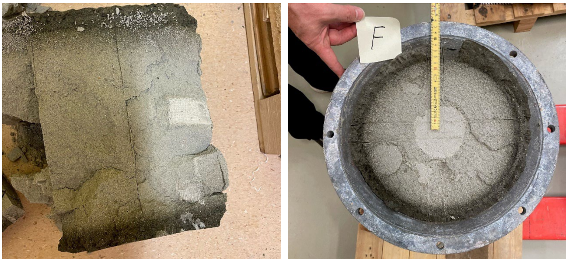
Figure 4-16. Photos taken in conjunction with the dismantling of Test 1. Left: Interface between two blocks in between cross section F and G (a shadow is covering the left block). Right: Cross section F.
