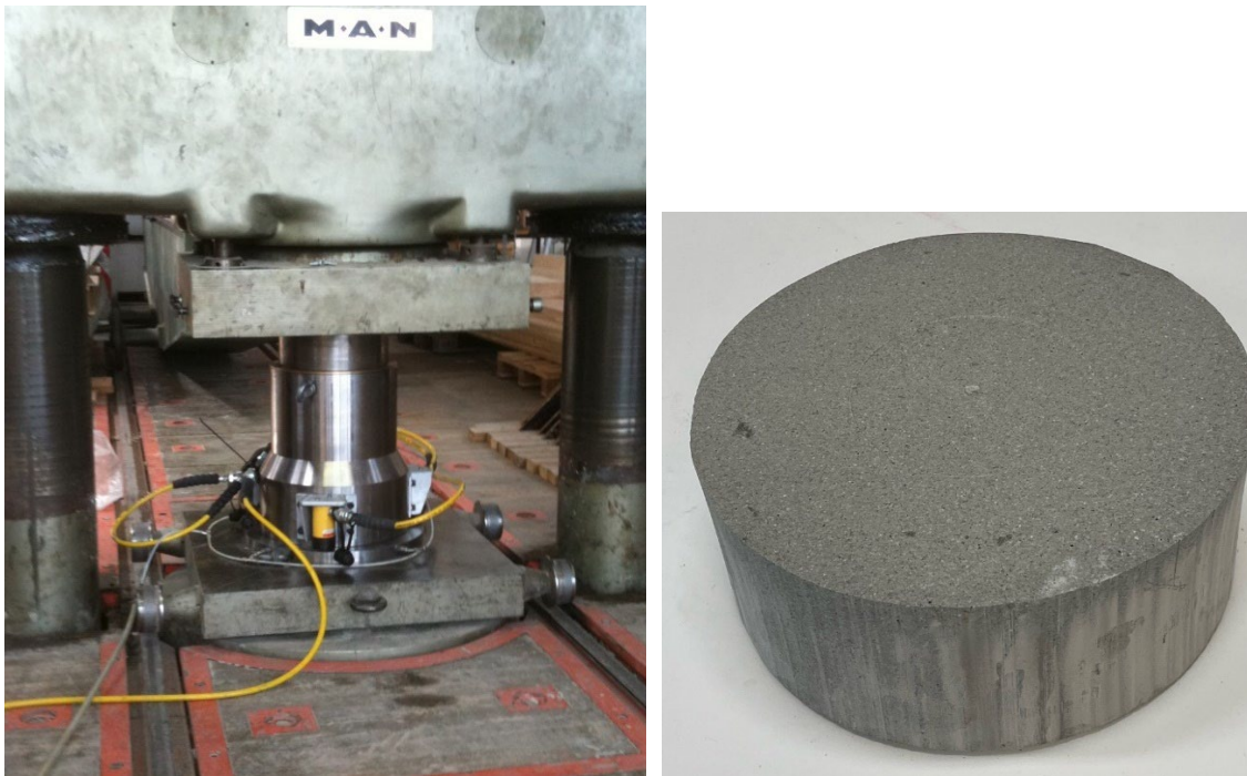
Figure 3-1 Left: Manufacturing of blocks with an outer diameter of 275/280 mm using the 1000-ton press at LTH Lund. Right: Photo showing a manufactured block after adjustment of the diameter.
