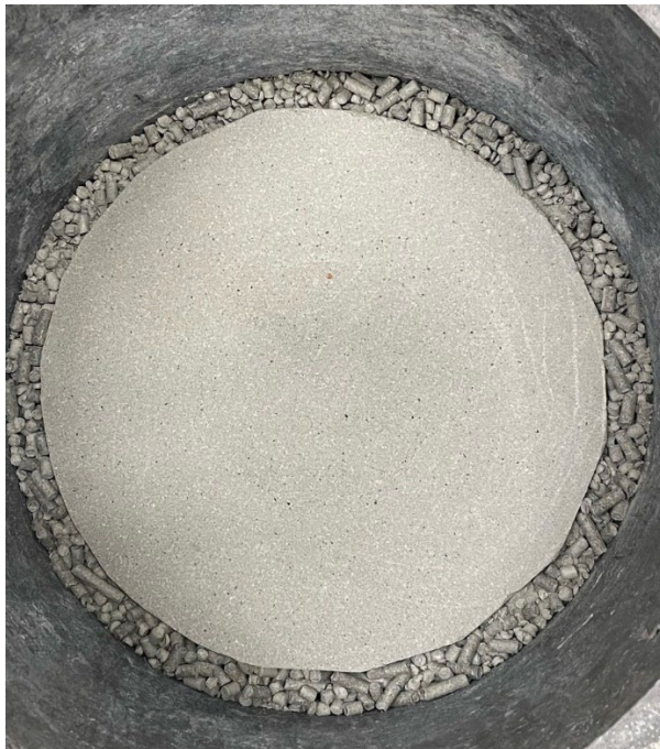
Figure 4-1 Blocks and pellets have been installed.
