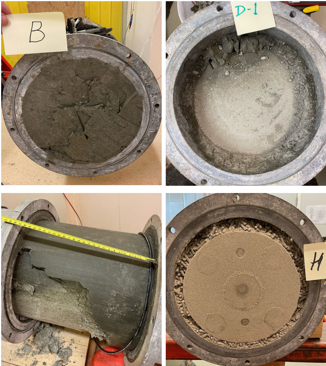
Figure 5-3 Photos taken in conjunction with the dismantling of Test 2. Upper left: Test section B before sampling. The bentonite was clearly wetted. Upper right: The photo shows a cross-section one block before sample section D, where the former pellet filling and parts of the block was wetted. Lower left: The photo shows the wetted upper part between cross-sections D (to the right) and E. Lower right: The photo shows the last cross-section (H) which looked unaffected by the inflowing water. The pellets in the gap also looked unaffected and was easily removed.
