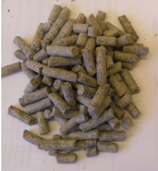
Figure 3-2 Photo showing pellets manufactured by extrusion.
