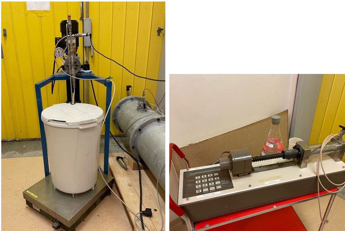
Figure 2-2. Left: Photo showing the pump system used in Test 1 to inject water with high pressure, 4 MPa. Right: Photo showing the GDS APVC (Advanced Pressure/Volume Controller) used to apply a constant flow rate of 0.2 mL/min in Test 2.
