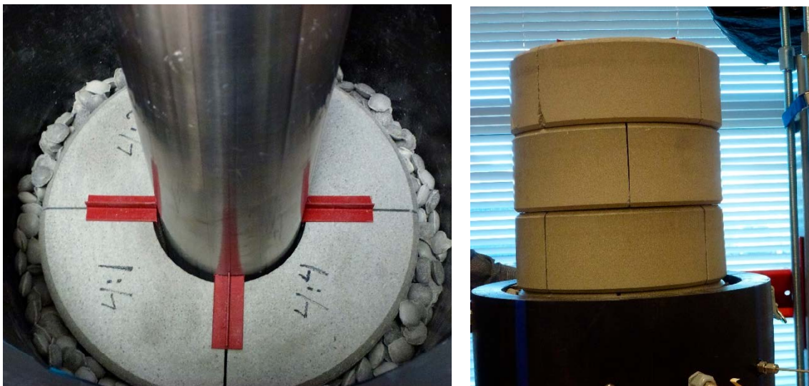
Figure 3-20. Left: Special spacers were used to achieve the same distances between the different block parts. Right: The blocks were positioned as a masonry bond to avoid vertical channels.
