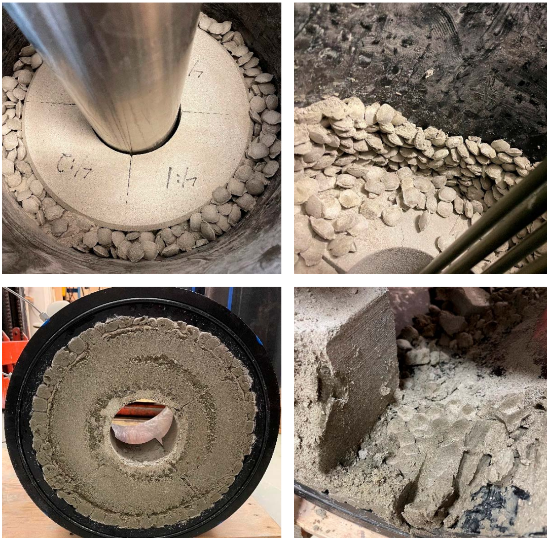
Figure 3-27. Photos taken in conjunction with dismantling of the blocks around the heater, Scale test 2. Upper left: Block 4. The block parts had moved closer to each other, and the radial gaps between the block parts had almost disappeared. Upper right: The pellet filling around Block 2 was partly wetted and some of the individual pellets had glued together. Lower left: The bottom block seen from below. The bottom surface and the lower part of the pellet filling was clearly wetted. The block had swelled and was stuck in the tube. Lower right: Dismantling of the bottom block. The block and the pellet filling have swelled together.
