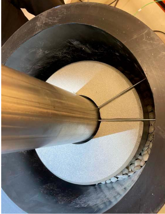
Figure 3-4. Left: Two thermocouples positioned on the surface of block no 5. One thermocouple was positioned against the heater, and one was positioned at the edge of the inner block surface. Right: The first section (0.6 m) has been installed.
