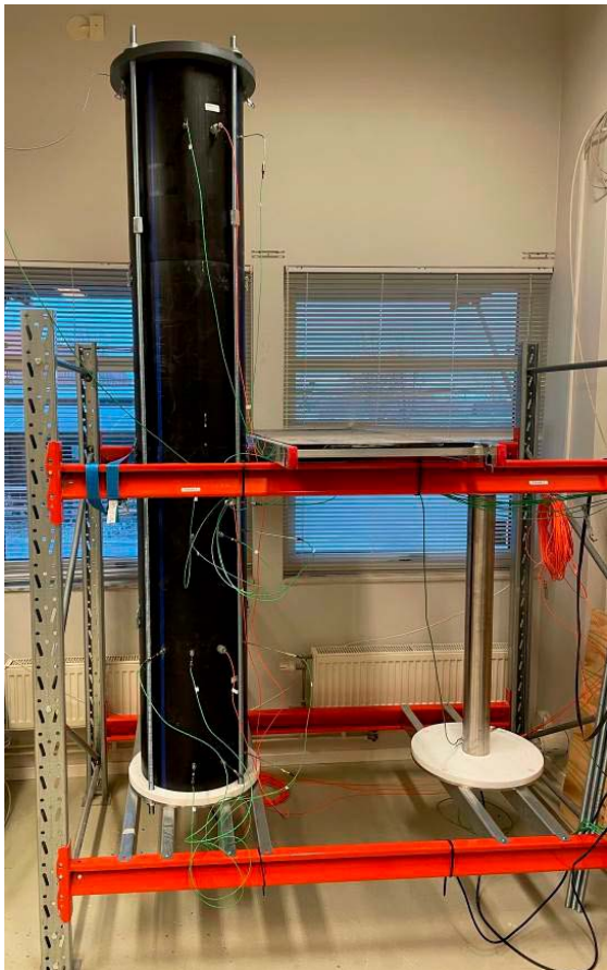
Figure 3-5. Left: The assembly of all parts have been successfully finished. Right: The test has been covered with insulation. The heater and bottom plate for the second test can be seen to the right in the photos.
