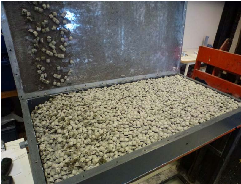
Figure 4-6. The alumina plate on the cold side of Gap test 1 have been removed. Pellets at the upper part of the test box were clearly wet.
