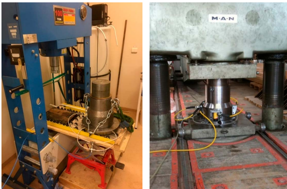
Figure 2-1. Left: Block manufacturing at Clay Technology. Right: Block manufacturing of blocks with an outer diameter of 275/280 mm using the 1000-ton press at LTH Lund.
