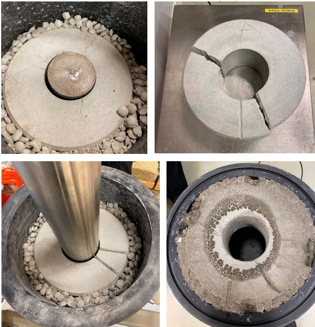
Figure 3-14. Photos taken in conjunction with dismantling of the blocks around the heater; Scale test 1. Upper left: Block 10. Some radial fractures can be seen on the block surface. Note the attachment point for the thermocouple on top of the heater. Upper right: Block 9. Two radial fractures. The block was divided in two pieces when it was removed. Lower left: Block 5. A few radial fractures could be seen. Lower right: The bottom block, Block 1, seen from below. The bottom surface and the lower part of the pellet filling was clearly wetted. The block had swelled and was stuck in the tube.
