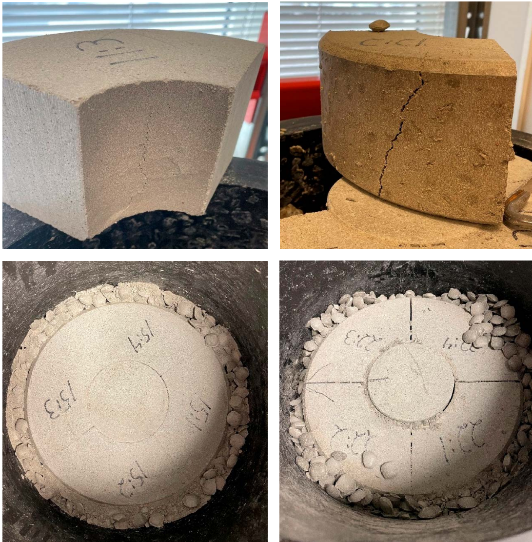
Figure 3-28. Photos taken in conjunction with the dismantling of the blocks above the heater, Scale test 2. Upper left: Some minor fractures could be seen in the parts of Block 11. Upper right: Block 12. Fracture in one of the block parts. Some of the pellets were almost glued against the block surface, see dark spots on the surface. Lower left: Block 15. The block parts have swelled, and the initial radial gaps have almost disappeared. Lower right: Block 22. The block was almost unaffected.
