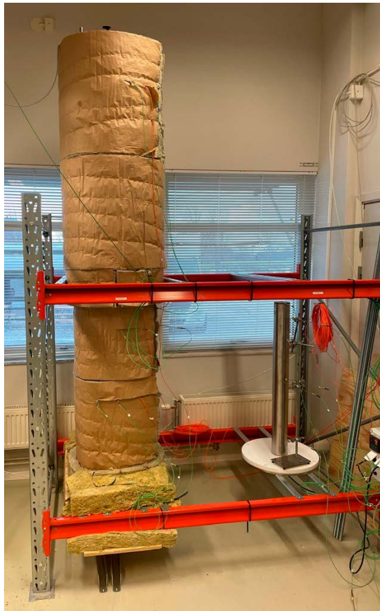
Figure 3-5. Left: The assembly of all parts have been successfully finished. Right: The test has been covered with insulation. The heater and bottom plate for the second test can be seen to the right in the photos.
