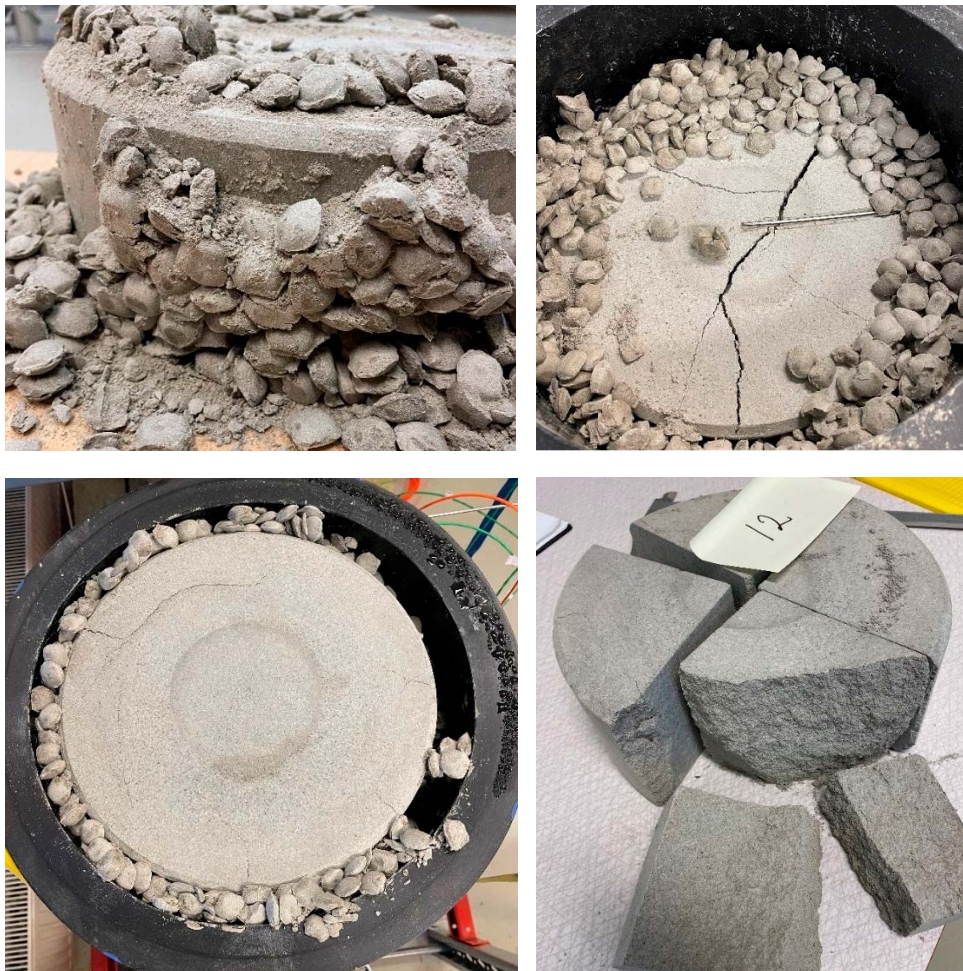
Figure 3-15. Photos taken in conjunction with the dismantling of the blocks above the heater, Scale test 1. Upper left: The pellet filling had locally a higher water content around Block 16 in direction A. Upper right: Block 11. This block had dehydrated, and radial fractures were formed in several directions. Lower left: Block 12. Some fractures were found in the block. There was also a locally empty pocket in the pellet filling. Lower right: Block 12 after sawing. Pieces fell off along the fractures.
