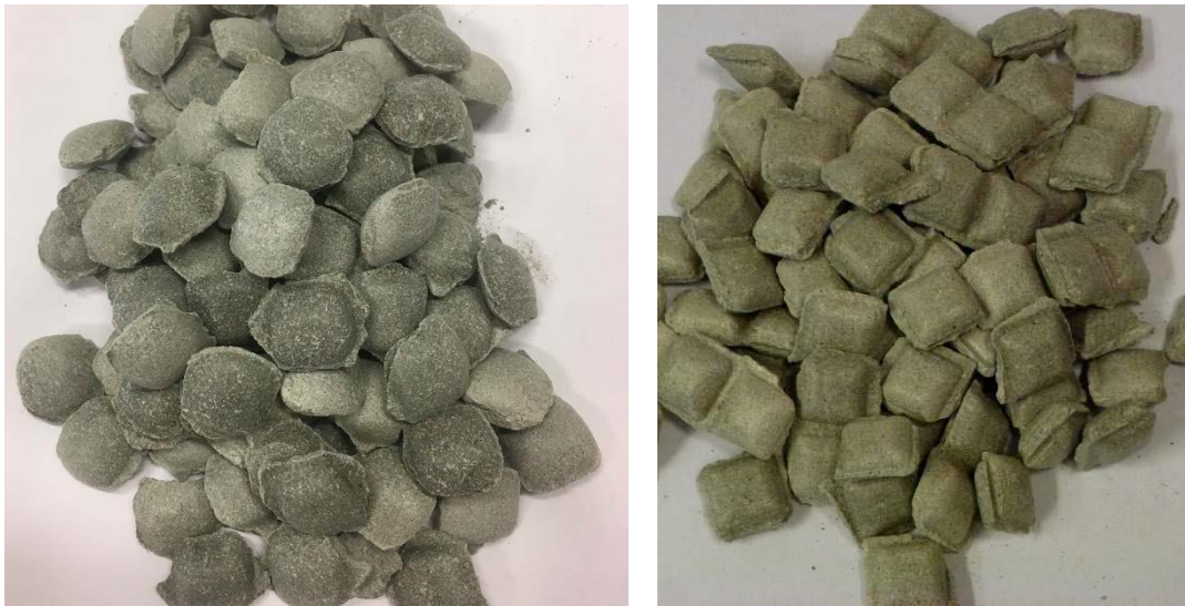
Figure 2-2. Photo showing the pellets used in the tests. Left photo: Pellets used in the scale tests. Right photo: Pellets used in the gap test.
