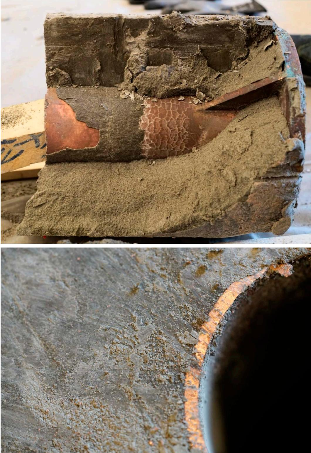
*Figure 1-5. Sampling of a LOT-experiment. Top: gypsum was sometimes seen as a web like white precipitate in the bentonite innermost to the heater. Bottom: a cross cut of the copper tube. Photos by D. Svensson.*
