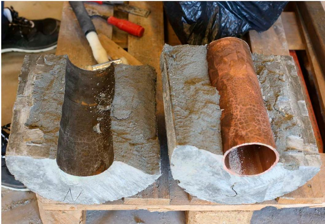
**Figure 1-4.** Sampling of a LOT-experiment. Top: sawing and cutting of the heater. All handling was documented by continuous filming. Bottom: example of how bentonite and copper surfaces and interfaces looked.
