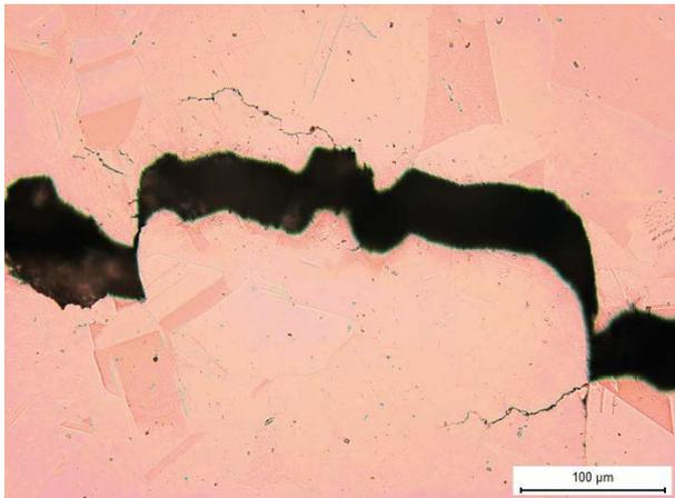
**Figure 1-5.** Optical image of the middle part of the pre-crack of WOL sample M4 4:1 from MiniCan 4, showing smaller fractures emanating from the pre-crack (Figure 4-7 in Gordon et al. (2017)).
