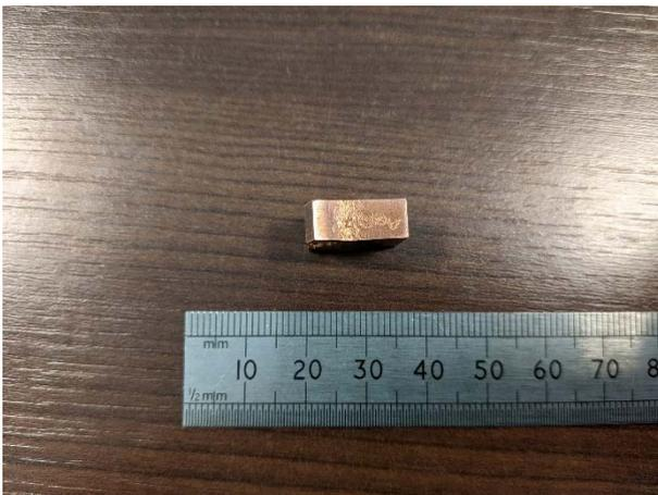
*Figure C-2. Top view of overloaded WOL specimen.*
