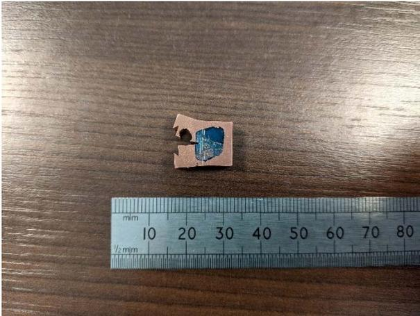
*Figure C-1. Side view of overloaded WOL specimen.*
