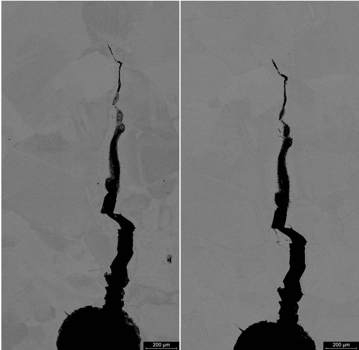
**Figure 3-1.** SEM micrographs of the WOL specimen BBG01 pre-etch (left) and post-etch (right) that was pre-cracked by fatigue but was not exposed to a corrosive environment prior to metallographic analysis. Some features appear more clearly after etching the specimen surface.
