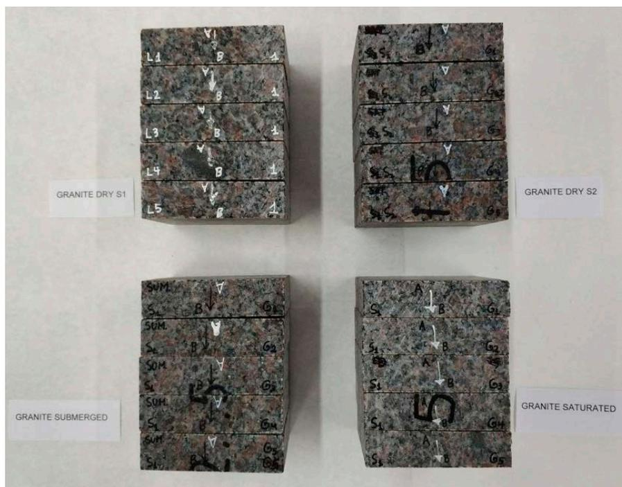
*Figure 3-24. Granite specimens for tilt-tests.*
