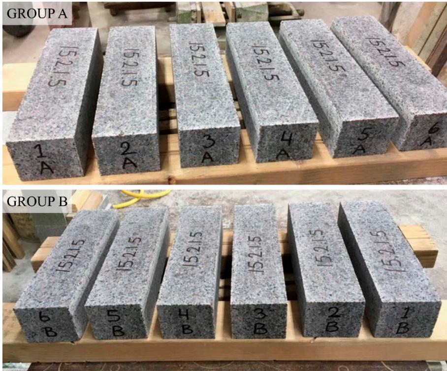
**Figure 3-22.** Sized slabs from Block 15.2.1.5 (300 mm × 80 mm × 70 mm) categorised as Groups A and B, for further preparation of tilt-test specimens at the University of Vigo (Spain).
