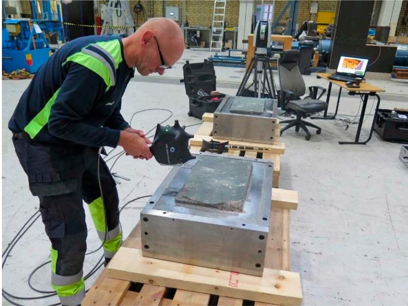
**Figure 4-9.** Contactless 3D scanning of a fracture surface using the Leica Absolute Scanner LAS with the Leica Absolute Tracker AT960 in the background.
