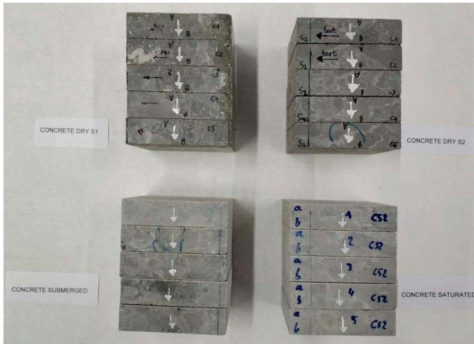
Figure 3-27. Concrete specimens for tilt-tests.
