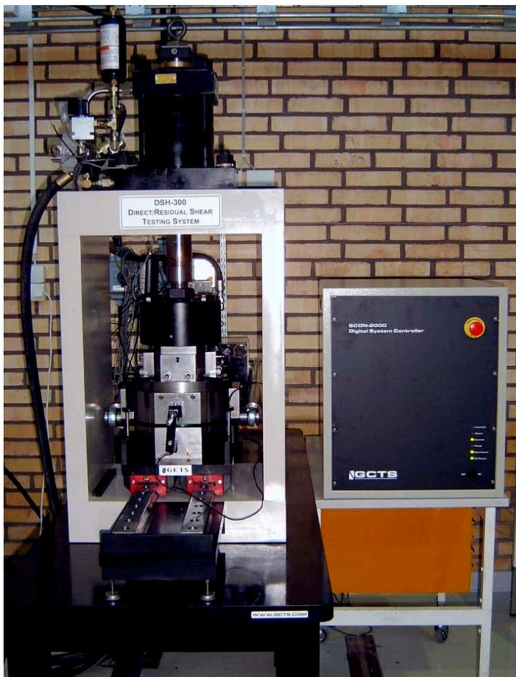
Figure 5-8. Equipment for direct shear tests and digital controller unit.
