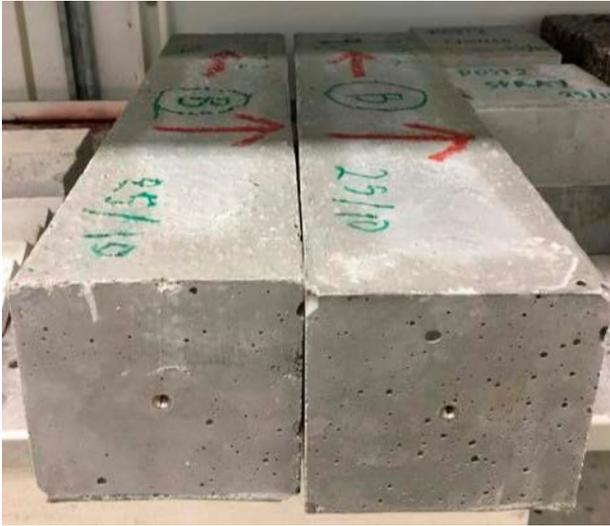
**Figure 3-25. Specimens with end studs for shrinkage measurements.**
