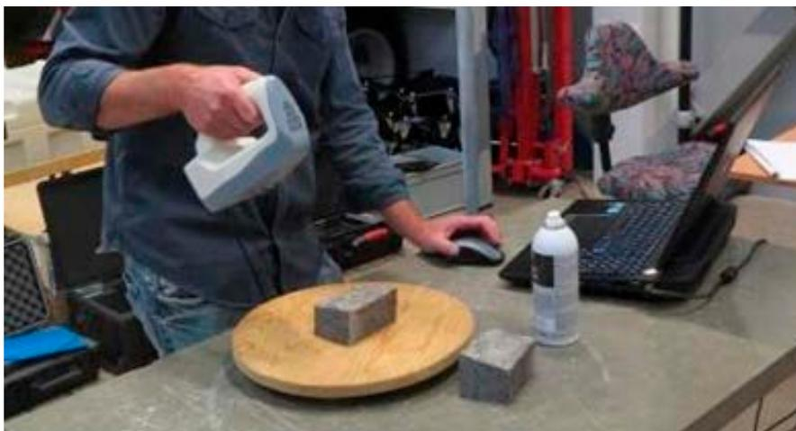
**Figure 4-11.** Scanning the fracture surface (not cast in formwork) on a turning table using an *Artec Spider* scanner.
