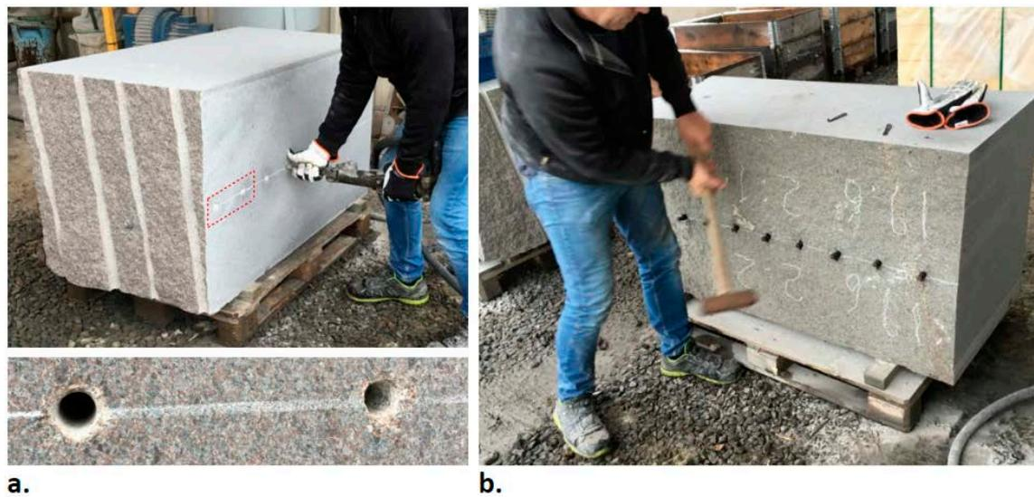
Figure 3-6. Block 19.6.2 (TI) a. Overview of drilling process (17 mm diameter drill, and centre depth of 80 mm); b. Overview of splitting process by means of wedge-driving with a sledgehammer.
