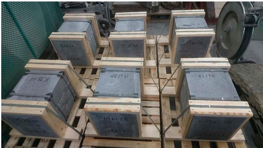
**Figure 3-11.** Photo of the 300 mm × 500 mm × 350 mm specimens with natural cracks, fixed with steel belts and pieces of wood with screw fractures to maintain the fractures in original position during transportation.
