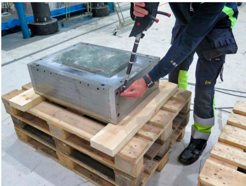
**Figure 4-8.** Tactile measurements using the T-probe for alignment of the casting box to the nominal CAD model.
