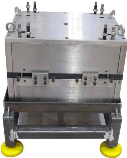
*Figure 5-2. Specimen holder standing on a table with the two halves in a fixed relative position.*
