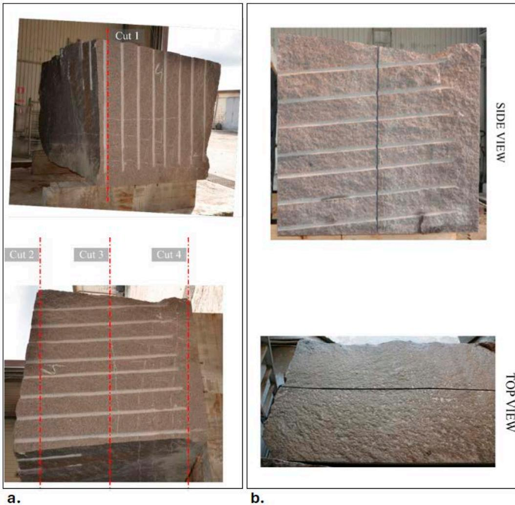
**Figure 3-4.** Block 19.6. a. Cut 1 (producing a thin side slab, subsequently denoted 19.6.0 (N)) and Cuts 2–4 producing two large slabs (Block 19.6–slab (1) and Block 19.6–slab (2)) plus two thin end slabs; b. Side and top view of Block 19.6 after the cuts.
