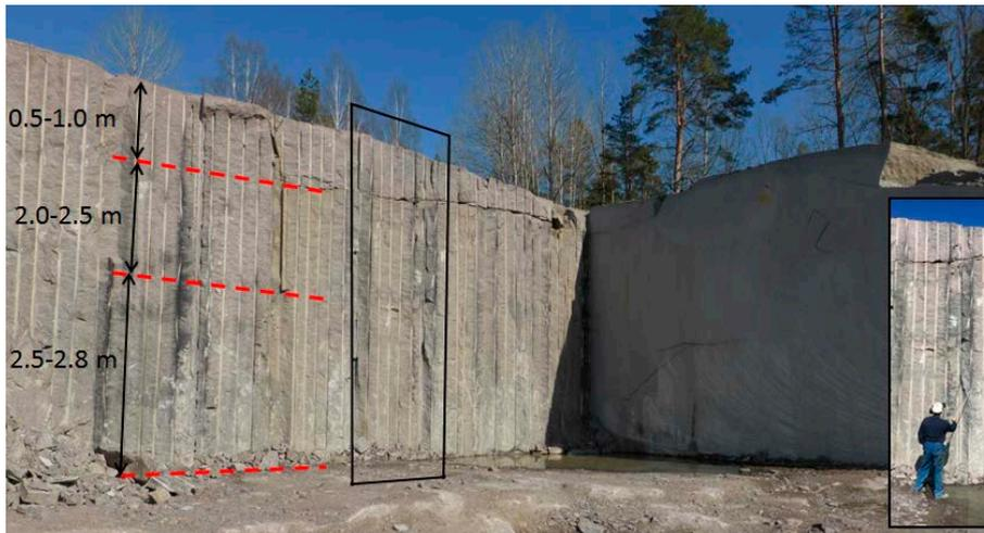
**Figure 3-2.** Location in the quarry where the blocks were extracted. The red lines show horizontal exfoliation fractures, and the small picture on the right-hand side of the photo illustrates the height of the wall. The vertical wall having drill holes (blasted surface) corresponds to the hardway plane (one of the granite cleavage orientation planes associated with the genesis of this rock), and the perpendicular plane with smooth wire cut would correspond to the grain plain.
