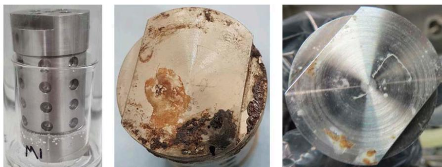
**Figure 4-2.** Images of the white crystals formed on M1 (left), and of the corrosion of the stainless steel sample holder bases of L1 (middle) and L2 (right).
