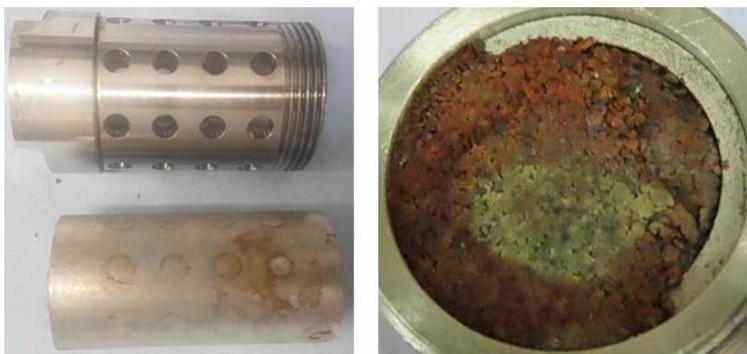
**Figure 4-1.** Images of the stainless steel sample holder (upper left) and steel filter (lower left) and the bentonite (right) from tipped glass cell S3 (0.20 L, 0 %  $\text{O}_2$ , 249 days, NaCl contaminated).
