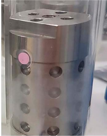
**Figure 2-3.** Close up image of one of the glass cells showing the location of an oxygen sensing spot (pink). The spot is attached to the inside of the glass using silicone rubber.
