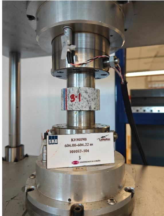
Figure A2-33. Measurement of ultrasonic velocities of sample KFM09B (3-1)
