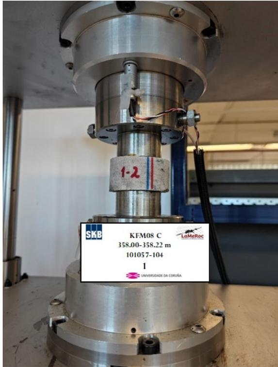
Figure A2-5. Measurement of ultrasonic velocities of sample KFM08C (1-2)
