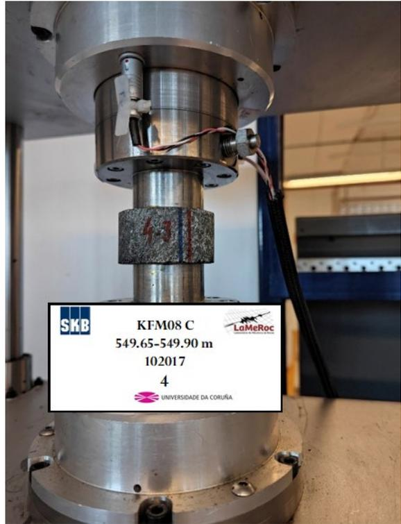
Figure A2-57. Measurement of ultrasonic velocities of sample KFM08C (4-3)
