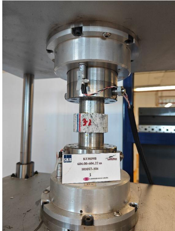
Figure A2-37. Measurement of ultrasonic velocities of sample KFM09B (3-2)
