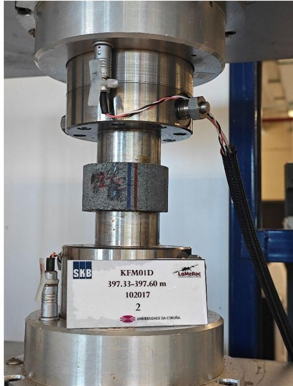
Figure A2-29. Measurement of ultrasonic velocities of sample KFM01D (2-4)
