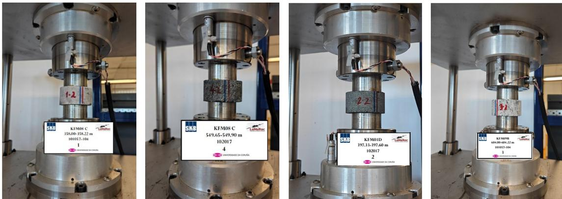
**Figure 2-7** Platens and load frame used to perform the ultrasonic pulse velocity determinations of the Forsmark site borehole specimens.
