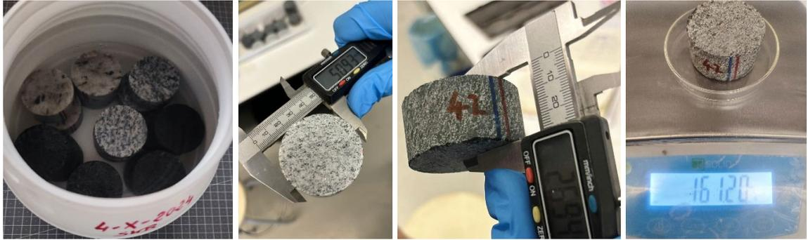
**Figure 2-3** Sliced specimens while immersed in tap water (left) and measurement of their corresponding geometric dimensions and weight (right)
