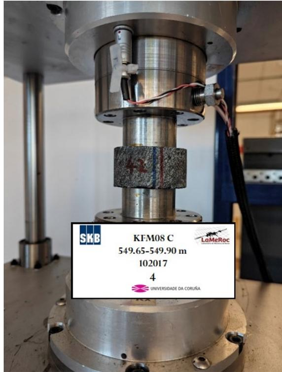
Figure A2-53. Measurement of ultrasonic velocities of sample KFM08C (4-2)
