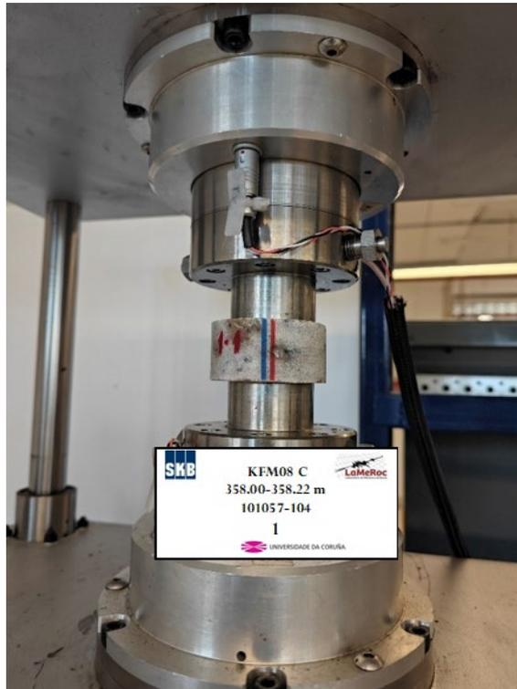
Figure A2-1. Measurement of ultrasonic velocities of sample KFM08C (1-1)
