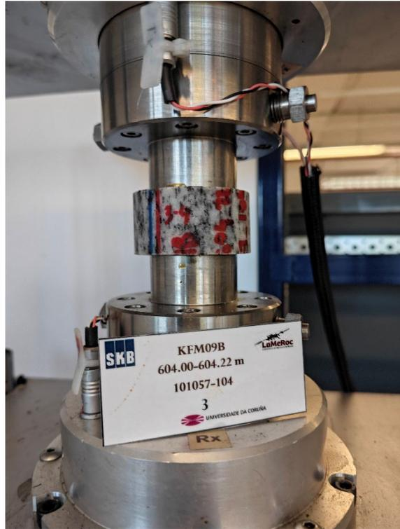
Figure A2-45. Measurement of ultrasonic velocities of sample KFM09B (3-4)
