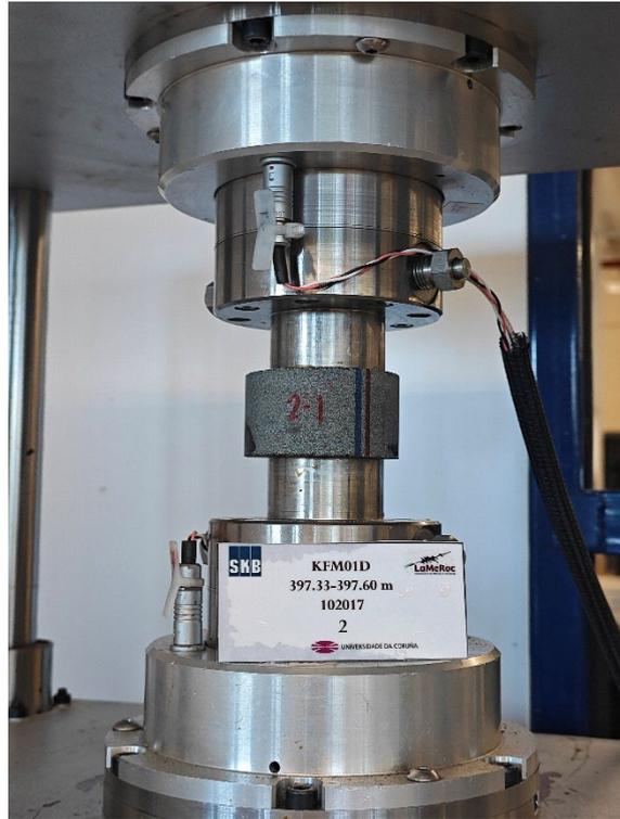
Figure A2-17. Measurement of ultrasonic velocities of sample KFM01D (2-1)
