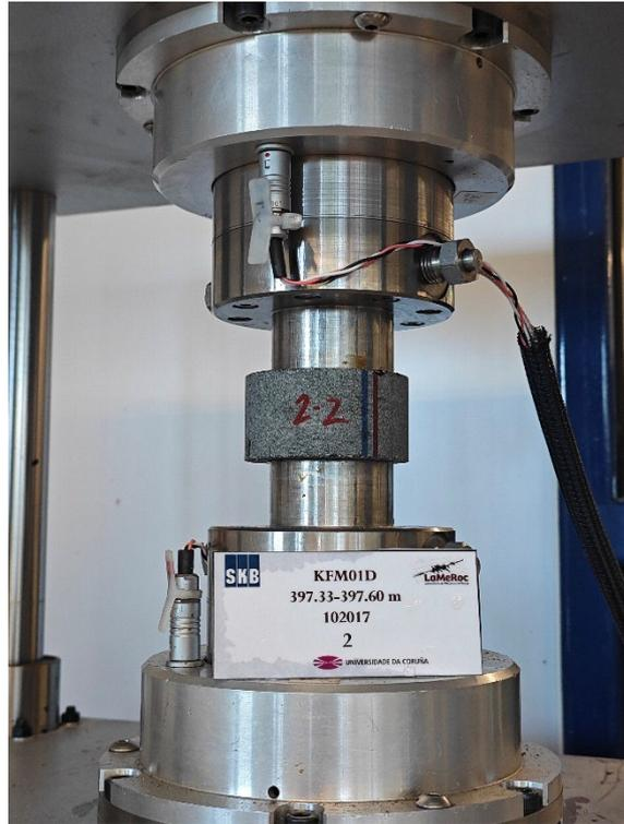
Figure A2-21. Measurement of ultrasonic velocities of sample KFM01D (2-2)
