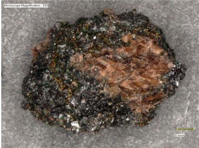
**Figure H-11.** Sample LL-1381 (LKAB 384-1137), potentially oxidised pyrite as indicated by the rust brown colouring of the sample. Scale bar bottom right.
