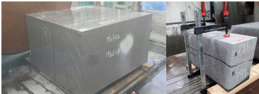
Figure 2-1. Block 19.6.1.4 from which the sample is cut (left) and Slab of 19.6.1.4 block from which the 200 \times 200 \times 250 \text{ mm}^3 is cut (right). Figure taken from Bruines (unpublished) 2 .
