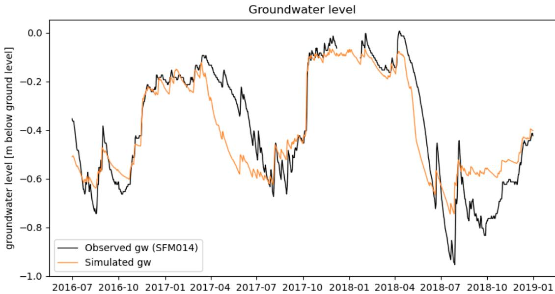
**Figure 3-22.** Simulated groundwater level (orange line) and observed groundwater level (black line) for evaluation period A.
