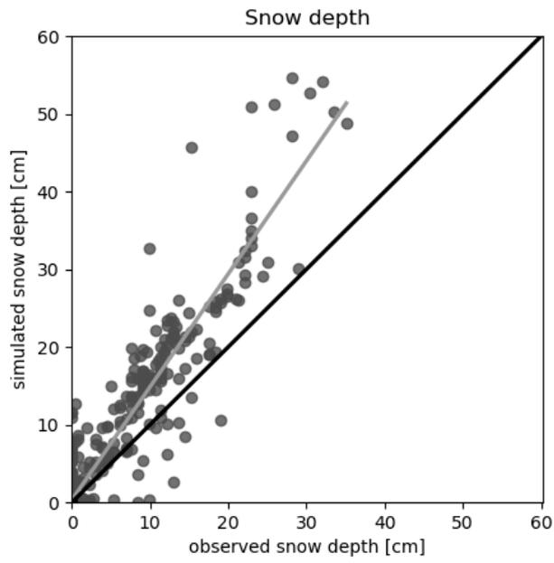
**Figure D-25.** Linear regression of simulated and observed snow depth for evaluation period B. The grey line shows the linear regression, the black line shows what would be a 1:1 relationship.
