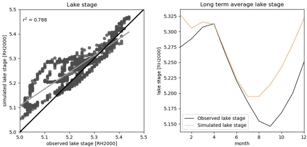
**Figure D-7.** Left: linear regression of simulated and observed lake stage for Eckarfjärden for calibration period B. The grey line shows the linear regression, the black line shows what would be a 1:1 relationship. Right: Lake Eckarfjärden monthly average lake stage for calibration period B. Both simulated (orange line) and observed (black line) lake stage are shown.
