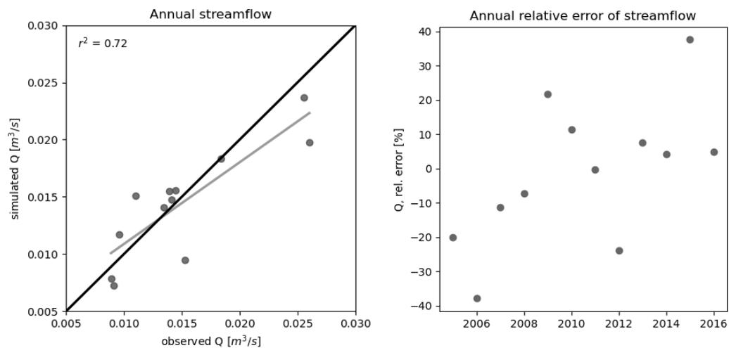
**Figure 3-5.** Left: linear regression of simulated and observed annual streamflow for calibration period A. The grey line shows the linear regression, the black line shows what would be a 1:1 relationship. Right: Relative error [%] of simulated and observed annual streamflow for the calibration period A.
