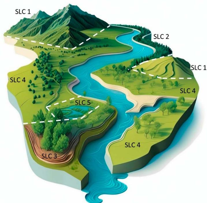
**Figure 1-1.** Example of a hydrological drainage basin in HYPE with Soil type Land use Combinations (SLCs) represented. Modified from image generated with OpenArt.ai.
