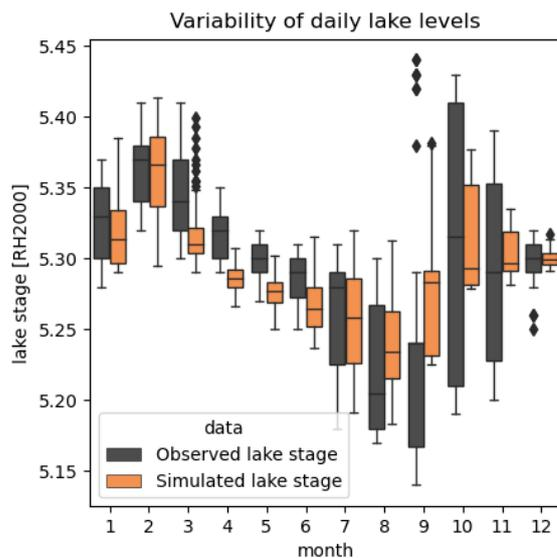
**Figure 3-8.** Eckarfjärden daily lake stage for calibration period A, for each month of the year. Simulated lake stage is shown in orange and observed lake stage is shown in grey.
