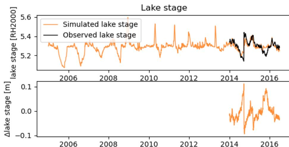
**Figure 3-6.** Model performance for calibration period A. Top: Simulated lake stage of Eckarfjärden (orange line) and observed lake stage of Eckarfjärden (black line). Bottom: error in estimated lake stage (observed – simulated).
