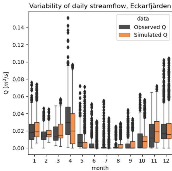
**Figure D-4.** Daily streamflow for the calibration period B, for each month of the year. Simulated streamflow is shown in orange and observed streamflow is shown in grey.
