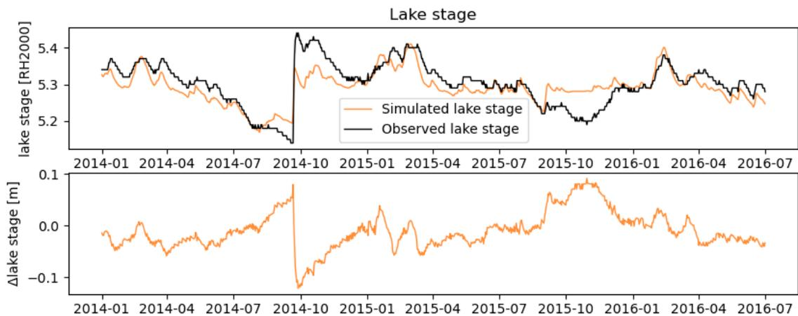
**Figure D-18 Model performance for evaluation period B.** Top: Simulated lake stage of Eckarfjärden (orange line) and observed lake stage of Eckarfjärden (black line). Bottom: error in estimated lake stage (observed – simulated).
