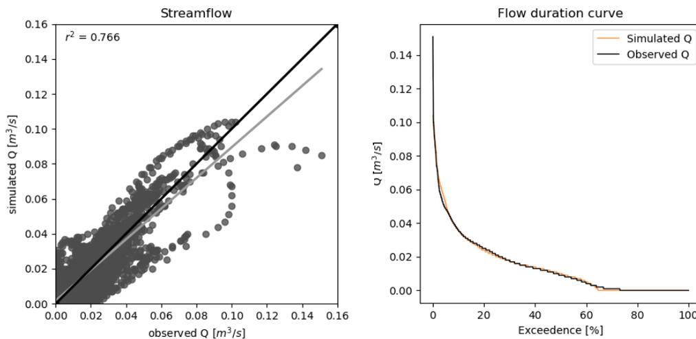
Figure D-2. Left: linear regression of simulated and observed streamflow for calibration period B. The grey line shows the linear regression, the black line shows what would be a 1:1 relationship. Right: Flow duration curve of simulated (orange line) and observed (black line) streamflow for calibration period B.
