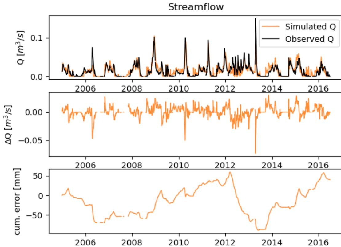
**Figure 3-1.** Model performance for calibration period A. Top: Simulated streamflow (orange line) and observed streamflow (black line). Mid: error in streamflow estimations ( $R_{\text{observed}} - R_{\text{simulated}}$ ). Bottom: cumulative error of runoff [mm].
