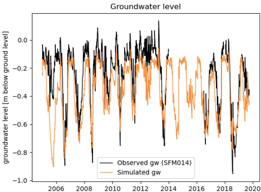
**Figure D-10.** Simulated groundwater level (orange line) and observed groundwater level (black line) for calibration period B.
