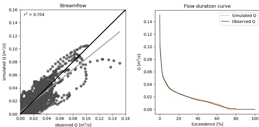
**Figure 3-2.** Left: linear regression of simulated and observed streamflow for calibration period A. The grey line shows the linear regression, the black line shows what would be a 1:1 relationship. Right: Flow duration curve of simulated (orange line) and observed (black line) streamflow for calibration period A.
