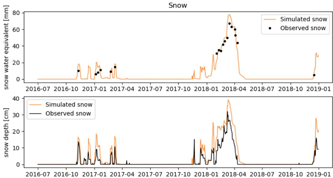
**Figure 3-24.** Snow time series data. Top: Simulated snow water equivalent (orange line) and observed snow water equivalent (black line) for evaluation period A. Bottom: Simulated snow depth (orange line) and observed snow depth (black line) for evaluation period A.
