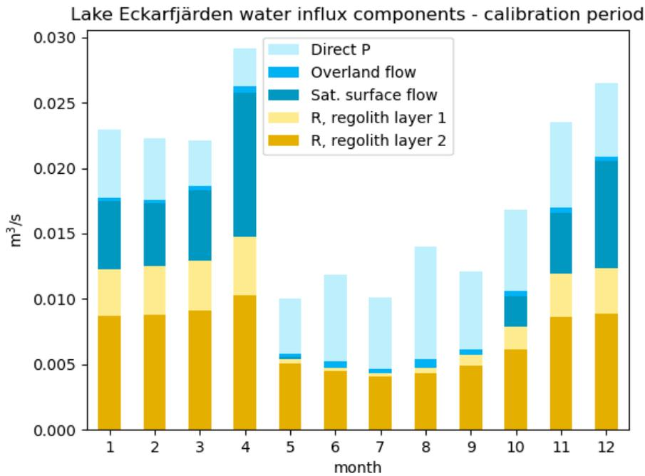
**Figure D-9.** Water influxes to Lake Eckarfjärden for calibration period B. “Overland flow” is excess precipitation and snowmelt, “Sat. surface flow” occurs when the groundwater level is higher than the ground level, “R, soil layer 1” and “2” are groundwater contributions from the upper two soil layers. “Soil layer 3” does not contribute to runoff in this model realization.
