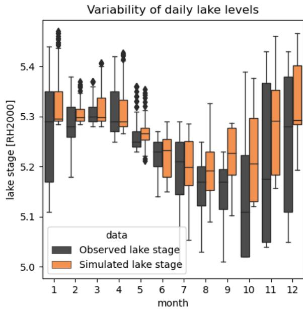
**Figure D-8.** Eckarfjärden daily lake stage for calibration period B, for each month of the year. Simulated lake stage is shown in orange and observed lake stage is shown in grey.
