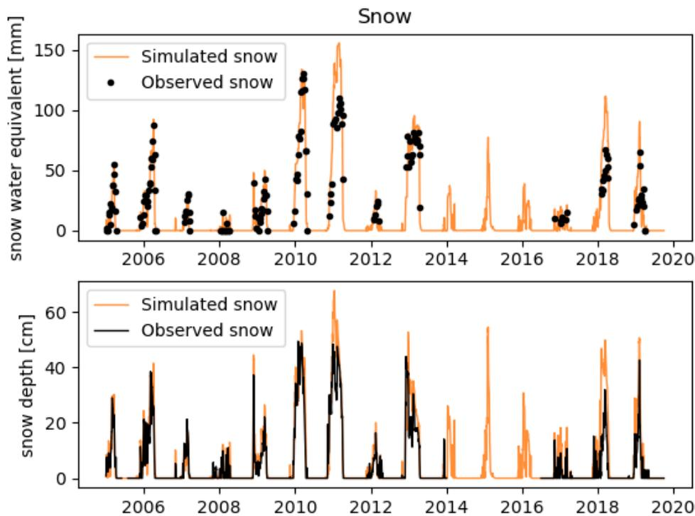
**Figure D-12.** Snow time series data. Top: Simulated snow water equivalent (orange line) and observed snow water equivalent (black line) for calibration period B. Bottom: Simulated snow depth (orange line) and observed snow depth (black line) for calibration period B.
