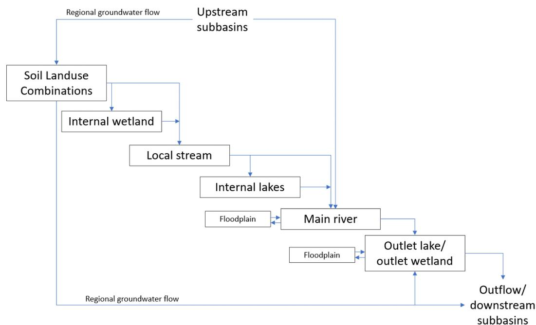
**Figure 1-3.** Routing of water flow through HYPE. Lakes, wetlands, floodplains, and regional groundwater flow are optional. All flows between storages are surface water flows unless otherwise specified. All storages are subjected to precipitation and evapotranspiration. Figure based on figure(s) presented on the HYPE wiki pages ([hype.smhi.net/wiki](http://hype.smhi.net/wiki)).
