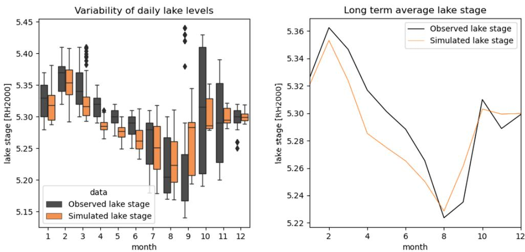
**Figure D-20.** Left: Eckarfjärden daily lake stage for evaluation period B, for each month of the year. Simulated lake stage is shown in orange and observed lake stage is shown in grey. Right: Lake Eckarfjärden monthly average lake stage for evaluation period B. Both simulated (orange line) and observed (black line) lake stage are shown.
