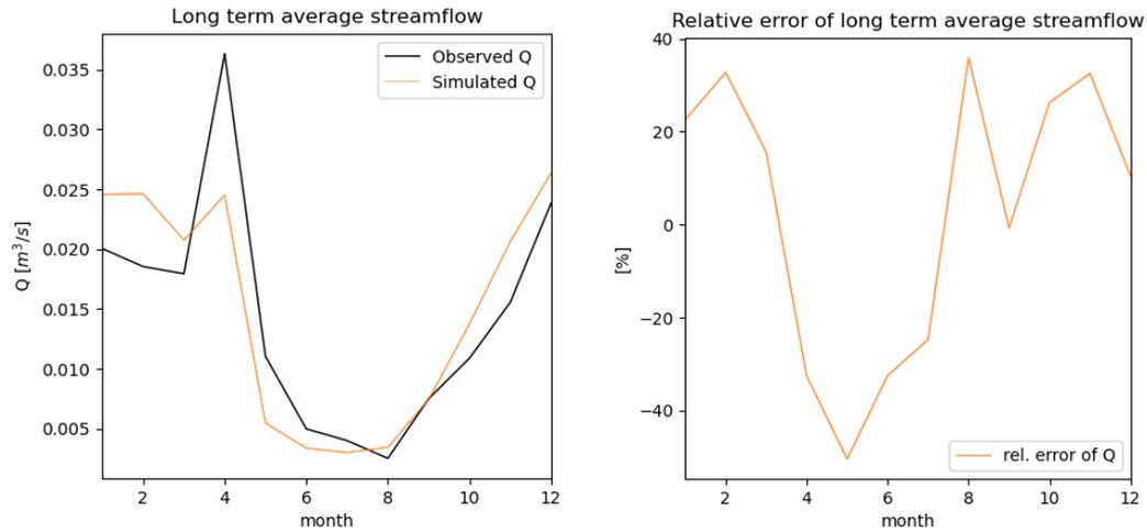
**Figure 3-3.** Left: Monthly average streamflow for calibration period A. Both simulated (orange line) and observed (black line) streamflow is shown. Right: Relative error  $((Q_{\text{simulated}} - Q_{\text{observed}})/Q_{\text{observed}})$  of monthly average streamflow for calibration period A.
