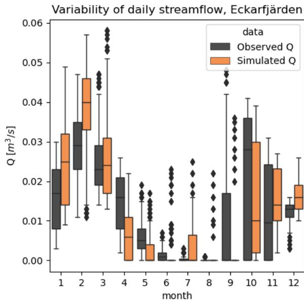
**Figure D-17.** Daily streamflow for the evaluation period B, for each month of the year. Simulated streamflow is shown in orange and observed streamflow is shown in grey.
