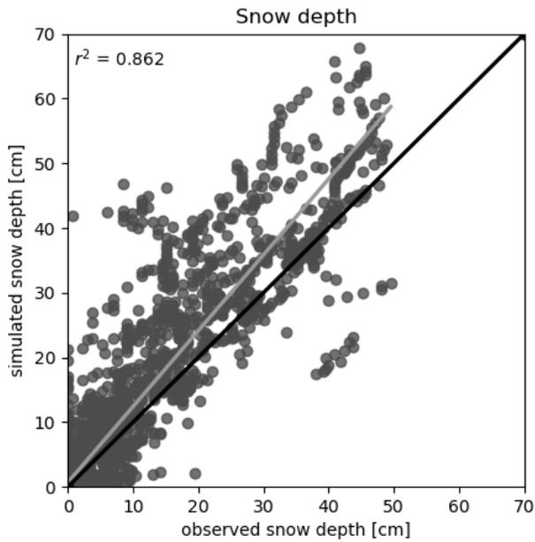
**Figure D-13.** Linear regression of simulated and observed snow depth for calibration period B. The grey line shows the linear regression, the black line shows what would be a 1:1 relationship.
