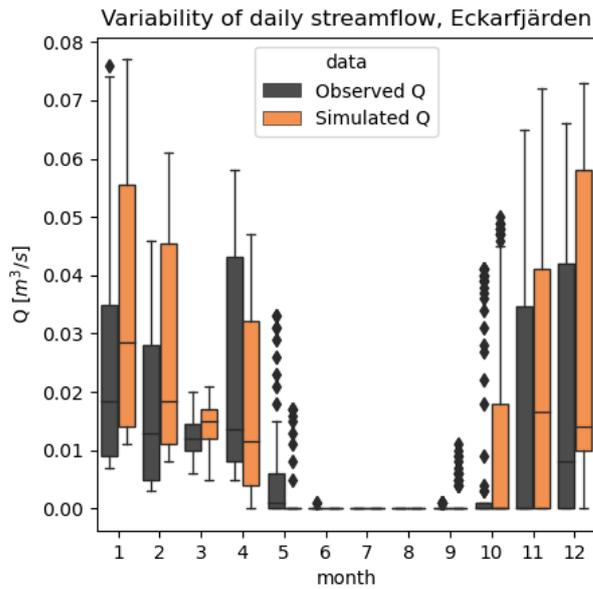
**Figure 3-17.** Daily streamflow for the evaluation period A, for each month of the year. Simulated streamflow is shown in orange and observed streamflow is shown in grey.
