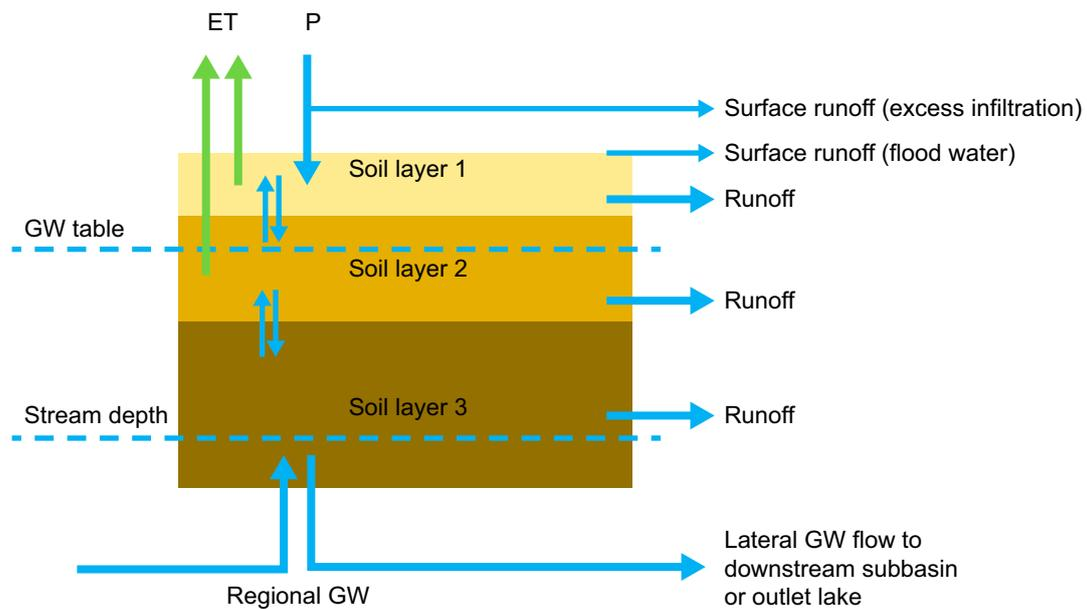
**Figure A-1.** Water fluxes in an SLC when the module for regional groundwater flow is enabled. GW is groundwater; P is precipitation and ET is evapotranspiration (modified from smhi wiki).
