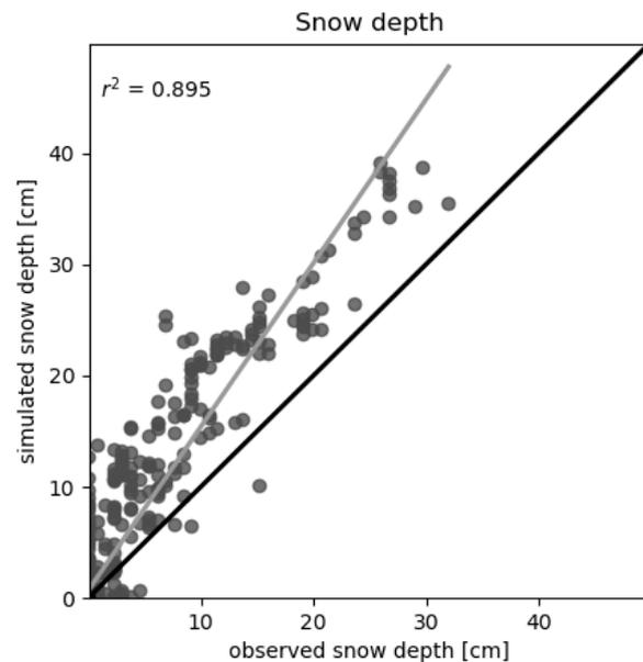
**Figure 3-25.** Linear regression of simulated and observed snow depth for evaluation period A. The grey line shows the linear regression, the black line shows what would be a 1:1 relationship.
