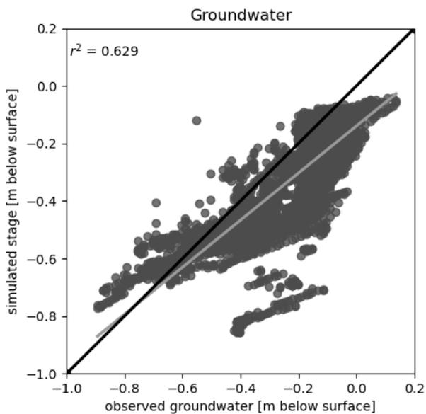
**Figure 3-11.** Linear regression of simulated and observed groundwater level for calibration period A. The grey line shows the linear regression, the black line shows what would be a 1:1 relationship.
