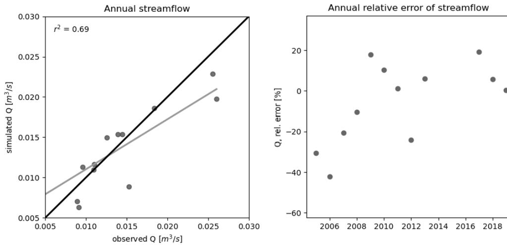
**Figure D-5.** Left: linear regression of simulated and observed annual streamflow for calibration period B. The grey line shows the linear regression, the black line shows what would be a 1:1 relationship. Right: Relative error [%] of simulated and observed annual streamflow for the calibration period B.
