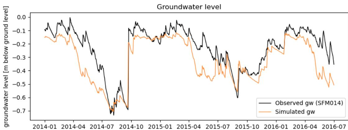
**Figure D-22.** Simulated groundwater level (orange line) and observed groundwater level (black line) for evaluation period B.
