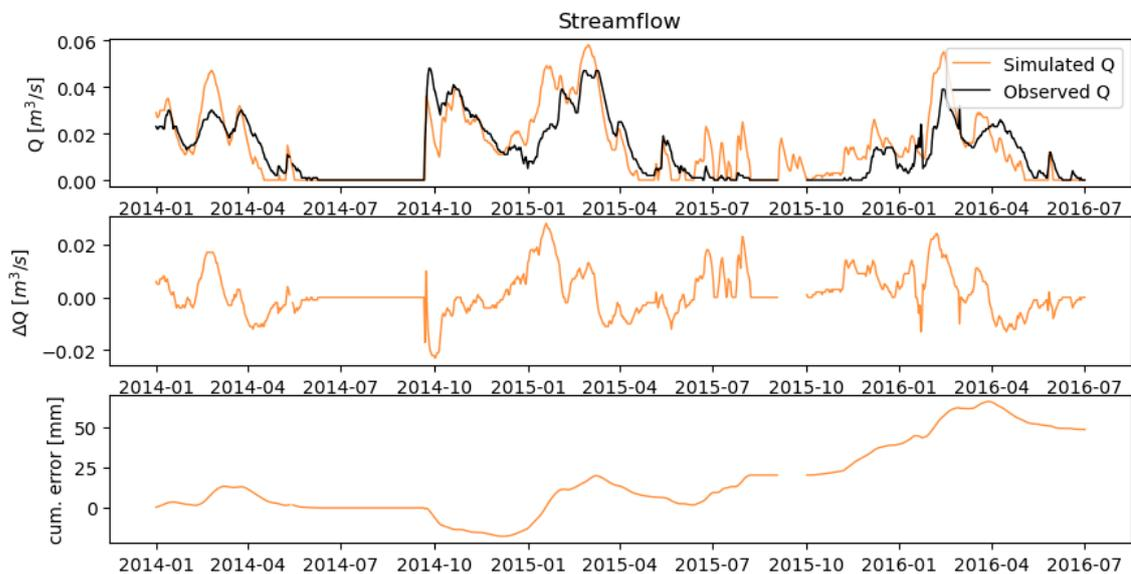
**Figure D-14.** Model performance for evaluation period B. Top: Simulated streamflow (orange line) and observed streamflow (black line). Mid: error in streamflow estimations ( $R_{observed} - R_{simulated}$ ). Bottom: cumulative error of runoff [mm].
