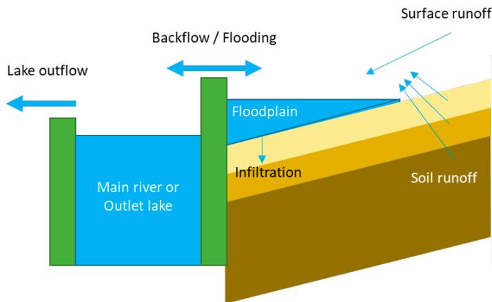
**Figure A-2.** Visualization of the floodplain model in HYPE when using the floodplain soil routine.
