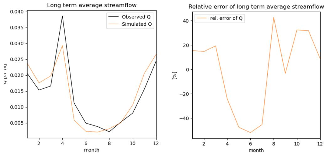
**Figure D-3.** Left: Monthly average streamflow for calibration period B. Both simulated (orange line) and observed (black line) streamflow is shown. Right: Relative error  $((Q_{\text{simulated}} - Q_{\text{observed}})/Q_{\text{observed}})$  of monthly average streamflow for calibration period B.
