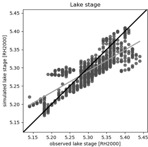
**Figure D-19.** Linear regression of simulated and observed lake stage for Eckarfjärden for evaluation period B. The grey line shows the linear regression, the black line shows what would be a 1:1 relationship.
