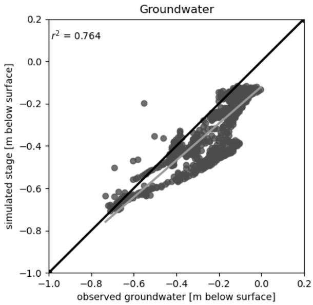
**Figure D-23.** Linear regression of simulated and observed groundwater level for evaluation period B. The grey line shows the linear regression, the black line shows what would be a 1:1 relationship.
