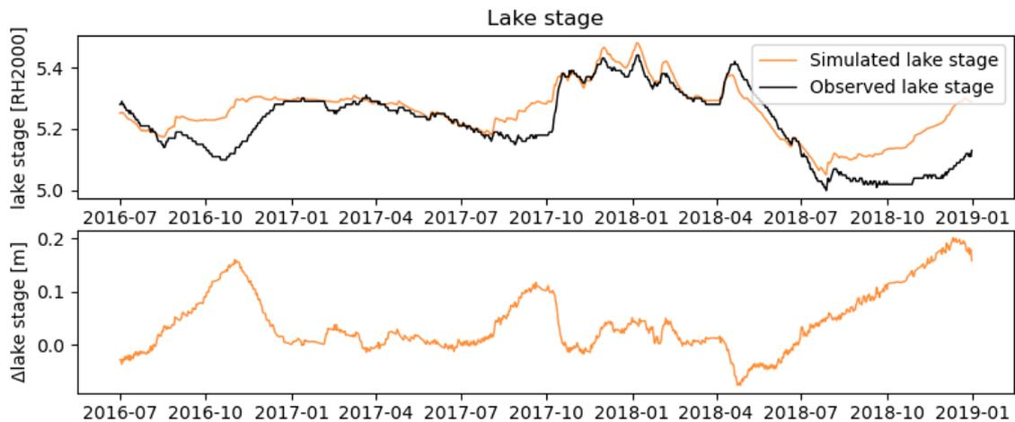
**Figure 3-18.** Model performance for evaluation period A. Top: Simulated lake stage of Eckarfjärden (orange line) and observed lake stage of Eckarfjärden (black line). Bottom: error in estimated lake stage (observed – simulated).
