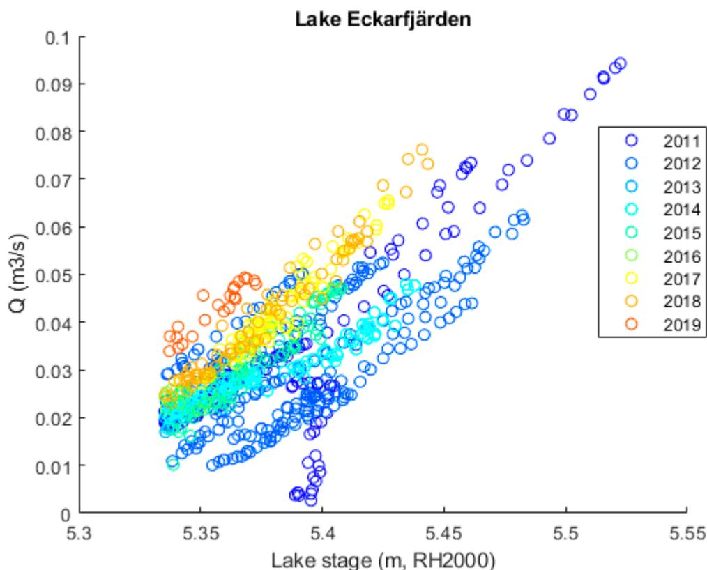
**Figure 2-4.** Lake stage and lake outlet discharge relationship at the outlet of Lake Eckarfjärden. The colors correspond to the year of the measurement point.
