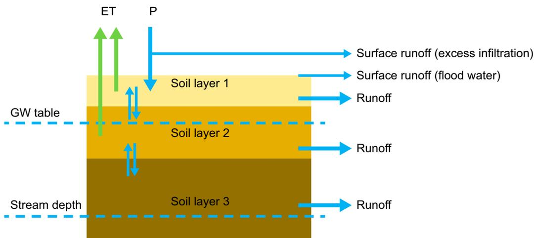
**Figure 1-2.** Water fluxes and runoff generation in an SLC for the model setup. GW is groundwater, P is precipitation and ET is evapotranspiration (modified from [www.smhi.net/hype/wiki](http://www.smhi.net/hype/wiki)).
