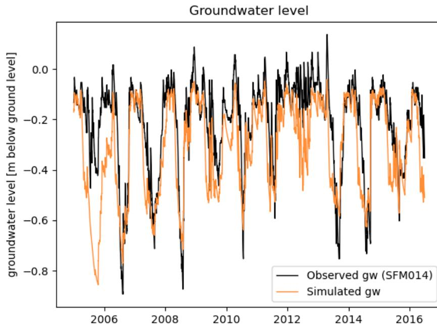
**Figure 3-10.** Simulated groundwater level (orange line) and observed groundwater level (black line) for calibration period A.
