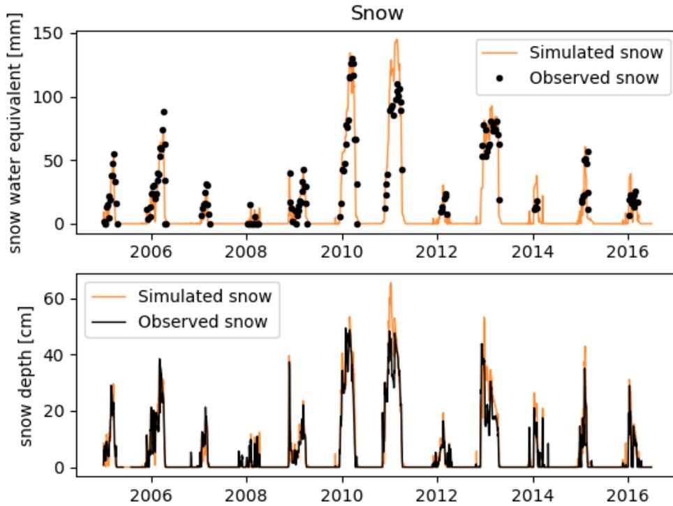
**Figure 3-12.** Snow time series data. Top: Simulated snow water equivalent (orange line) and observed snow water equivalent (black line) for calibration period A. Bottom: Simulated snow depth (orange line) and observed snow depth (black line) for calibration period A.
