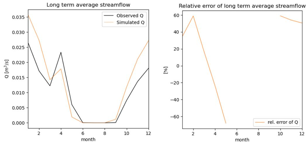
**Figure 3-16.** Left: Monthly average streamflow for evaluation period A. Both simulated (orange line) and observed (black line) streamflow is shown. Right: Relative error  $((Q_{\text{simulated}} - Q_{\text{observed}})/Q_{\text{observed}})$  of monthly average streamflow for months with streamflow during evaluation period A.
