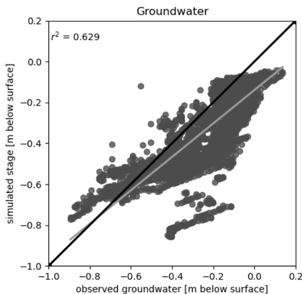
**Figure 3-23.** Linear regression of simulated and observed groundwater level for evaluation period A. The grey line shows the linear regression, the black line shows what would be a 1:1 relationship.
