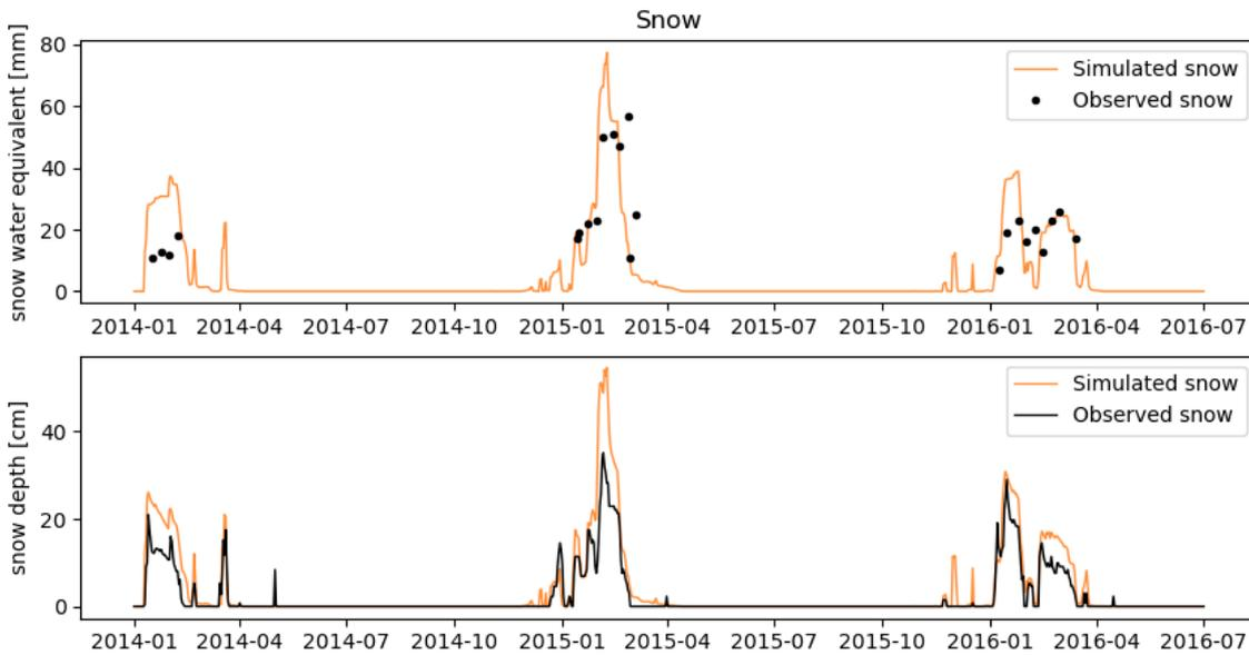
**Figure D-24.** Snow time series data. Top: Simulated snow water equivalent (orange line) and observed snow water equivalent (black line) for evaluation period B. Bottom: Simulated snow depth (orange line) and observed snow depth (black line) for evaluation period B.
