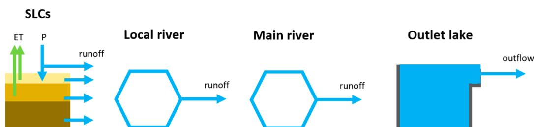
**Figure 2-1.** Schematic representation of runoff generation in HYPE model implemented for this study. Runoff generated from all SLCs are first routed through a single conceptual representation of local rivers and then through a main river. The main river feeds an outlet lake where the outflow from the drainage basin is generated.
