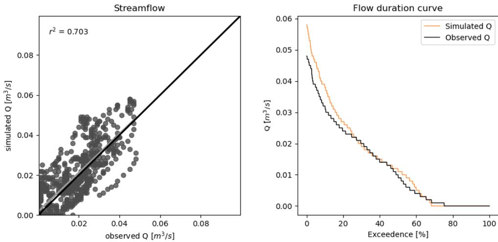
**Figure D-15.** Left: linear regression of simulated and observed streamflow for evaluation period B. The grey line shows the linear regression, the black line shows what would be a 1:1 relationship. Right: Flow duration curve of simulated (orange line) and observed (black line) streamflow for evaluation period B.
