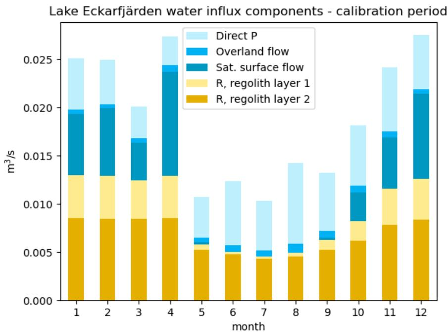
**Figure 3-21.** Water influxes to Lake Eckarfjärden for evaluation period A. “Overland flow” is excess precipitation and snowmelt, “Sat. surface flow” occurs when the groundwater level is higher than the ground level, “R, soil layer 1” and “2” are groundwater contributions from the upper two soil layers. “Soil layer 3” does not contribute to runoff in this model realization.
