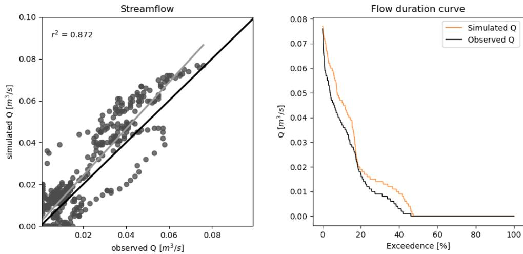
**Figure 3-15.** Left: linear regression of simulated and observed streamflow for evaluation period A. The grey line shows the linear regression, the black line shows what would be a 1:1 relationship. Right: Flow duration curve of simulated (orange line) and observed (black line) streamflow for evaluation period A.
