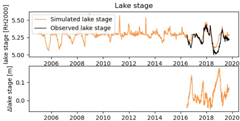
**Figure D-6.** Model performance for calibration period B. Top: Simulated lake stage of Eckarfjärden (orange line) and observed lake stage of Eckarfjärden (black line). Bottom: error in estimated lake stage (observed – simulated).
