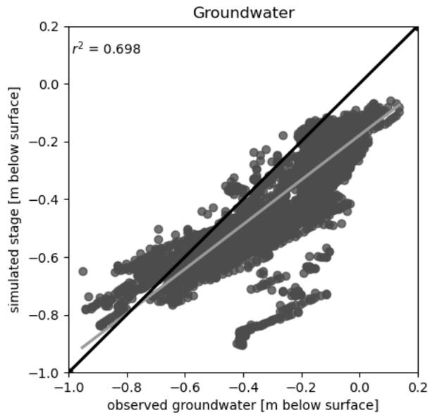
**Figure D-11.** Linear regression of simulated and observed groundwater level for calibration period B. The grey line shows the linear regression, the black line shows what would be a 1:1 relationship.
