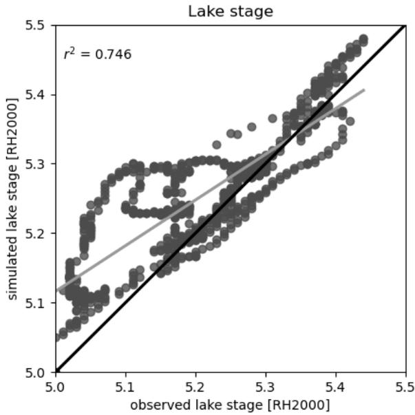
**Figure 3-19.** Linear regression of simulated and observed lake stage for Eckarfjärden for evaluation period A. The grey line shows the linear regression, the black line shows what would be a 1:1 relationship.
