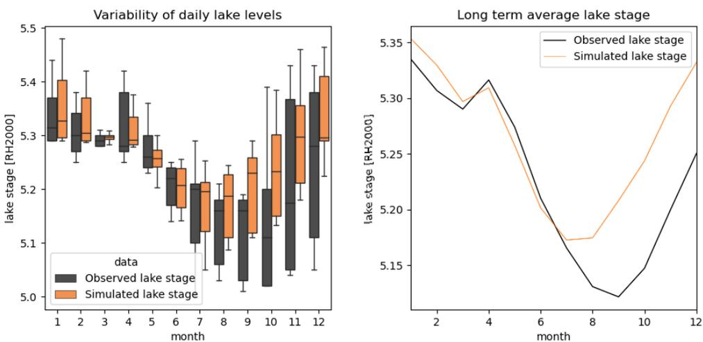
**Figure 3-20.** Left: Eckarfjärden daily lake stage for evaluation period A, for each month of the year. Simulated lake stage is shown in orange and observed lake stage is shown in grey. Right: Lake Eckarfjärden monthly average lake stage for evaluation period A. Both simulated (orange line) and observed (black line) lake stage are shown.
