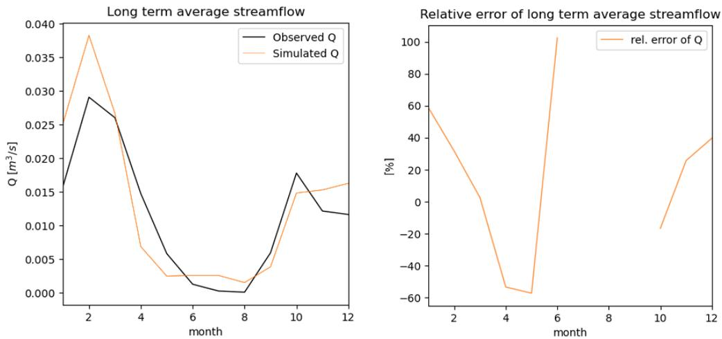
**Figure D-16.** Left: Monthly average streamflow for evaluation period B. Both simulated (orange line) and observed (black line) streamflow is shown. Right: Relative error  $((Q_{\text{simulated}} - Q_{\text{observed}})/Q_{\text{observed}})$  of monthly average streamflow for months with streamflow during evaluation period B.
