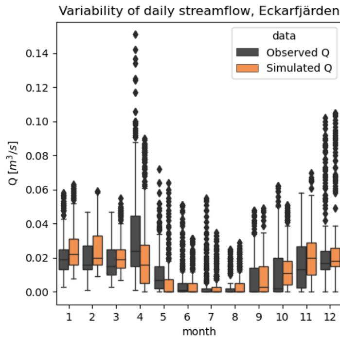
**Figure 3-4.** Daily streamflow for the calibration period A, for each month of the year. Simulated streamflow is shown in orange and observed streamflow is shown in grey.
