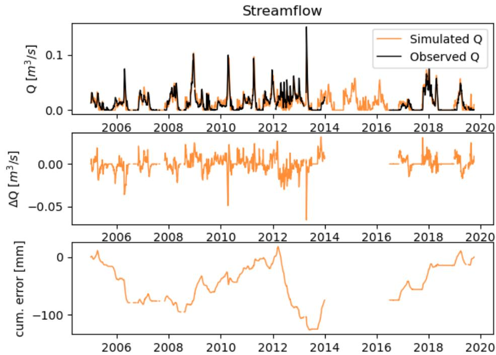
Figure D-1. Model performance for calibration period B. Top: Simulated streamflow (orange line) and observed streamflow (black line). Mid: error in streamflow estimations ( $R_{observed} - R_{simulated}$ ). Bottom: cumulative error of runoff [mm].
