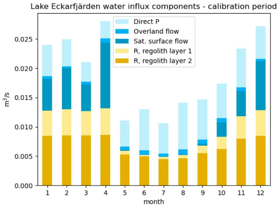
**Figure 3-9.** Water influxes to Lake Eckarfjärden for calibration period A. “Overland flow” is infiltration excess of rainfall and snowmelt, “Sat. surface flow” occurs when the groundwater level is higher than the ground level, “R, soil layer 1” and “2” are groundwater contributions from the upper two soil layers. “Soil layer 3” does not contribute to runoff in this model realization.
