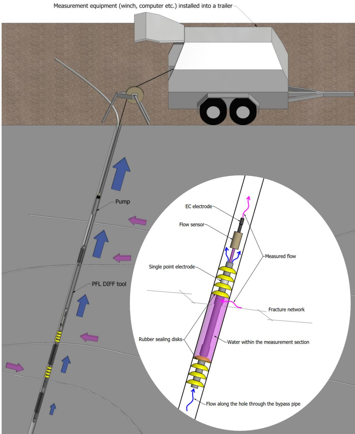
**Figure 3-2** Schematic of the PFL DIFF probe used in a ground-level borehole. In a sub-horizontal tunnel borehole, the probe operation is similar; only the borehole pressure is controlled with a borehole sealing mechanism instead of a submersible pump.
