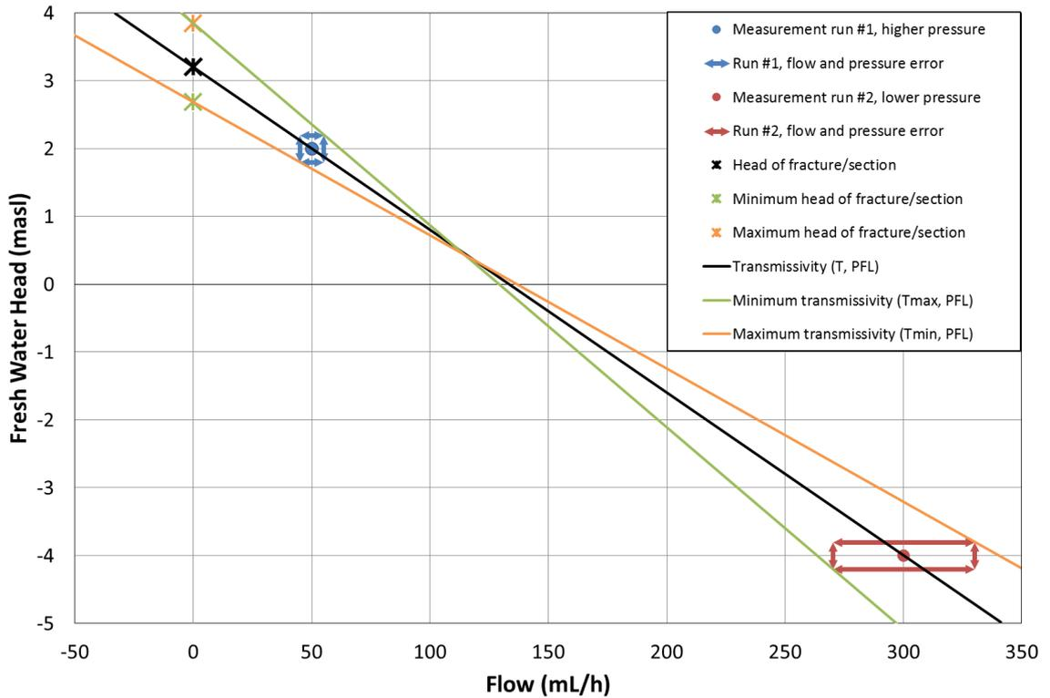
**Figure 6-1** Demonstrative plot how measurement accuracy of flow rate and pressure affects derivation of transmissivity and fracture head.
