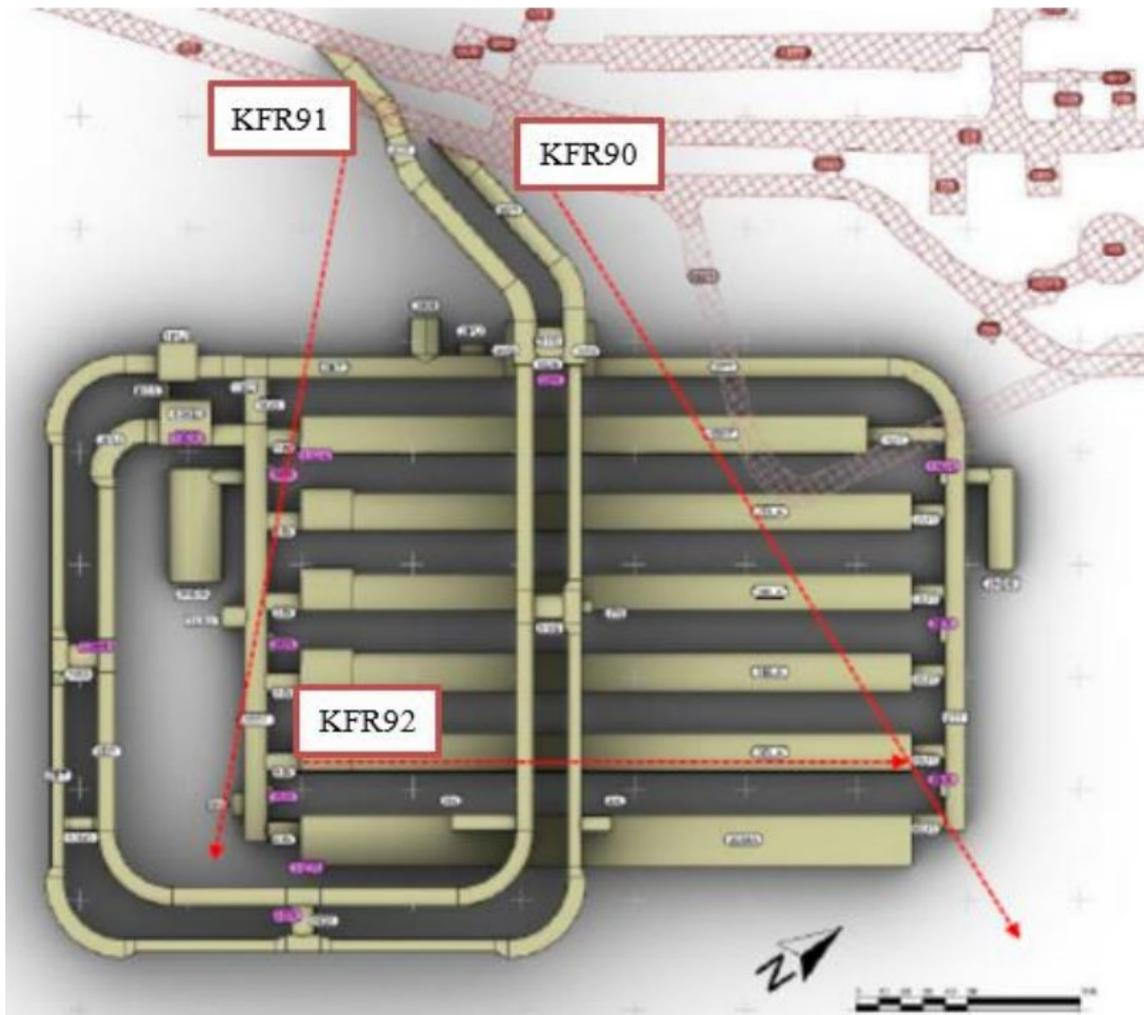
**Figure 1-1** Locations and drilling directions of boreholes KFR90 and KFR91 in one of the SFR access tunnels. The hatched area is the existing tunnel system, and the green area is the extended tunnel system to be constructed. KFR92 is a planned borehole.
