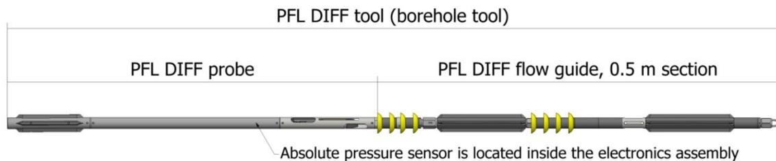
**Figure 3-1** Technical illustration of the PFL DIFF probe with 0.5 m measurement section length.
