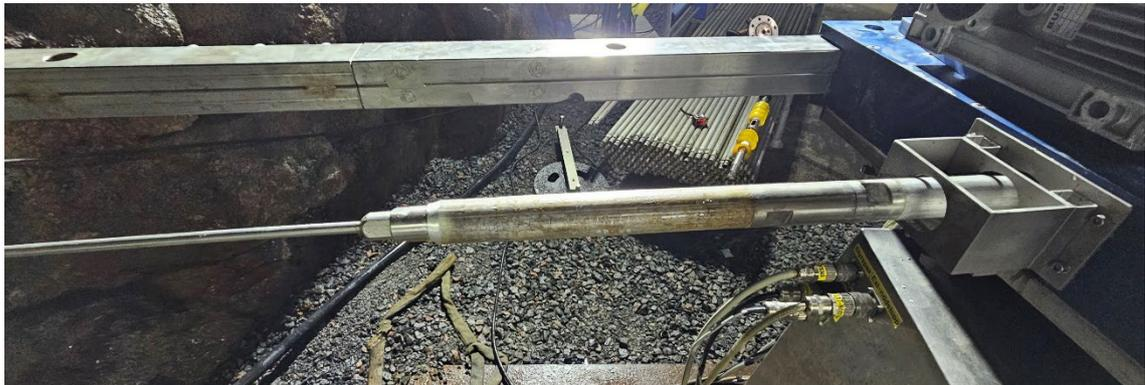
**Figure 4-4** Pushing rod with adapter for PFL DIFF probe.
