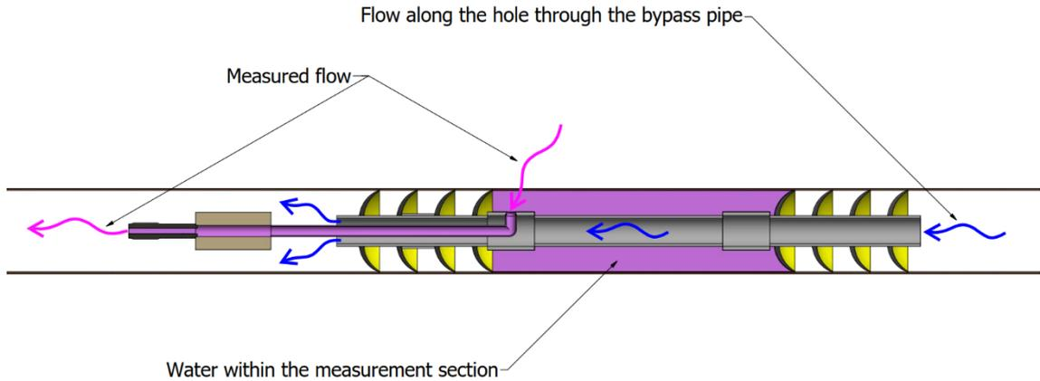
**Figure 3-3** Schematic of a cross-section of the PFL DIFF probe.
