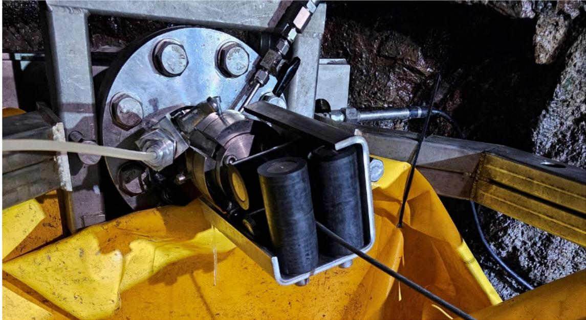
**Figure 4-1** Borehole sealing mechanism attached to the casing pipe at the opening of the borehole. A cable guide extends onwards from the sealing mechanism.
