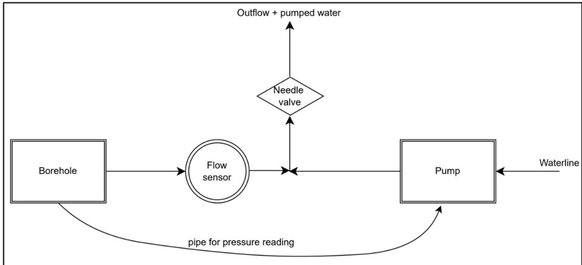
**Figure 4-3** Borehole pressure control during flow logging.
