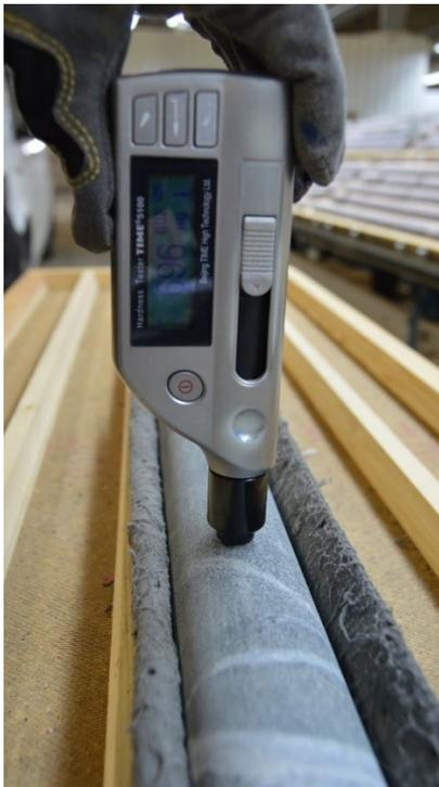
*Figure 5-1. The instrument for Leeb hardness test.*
