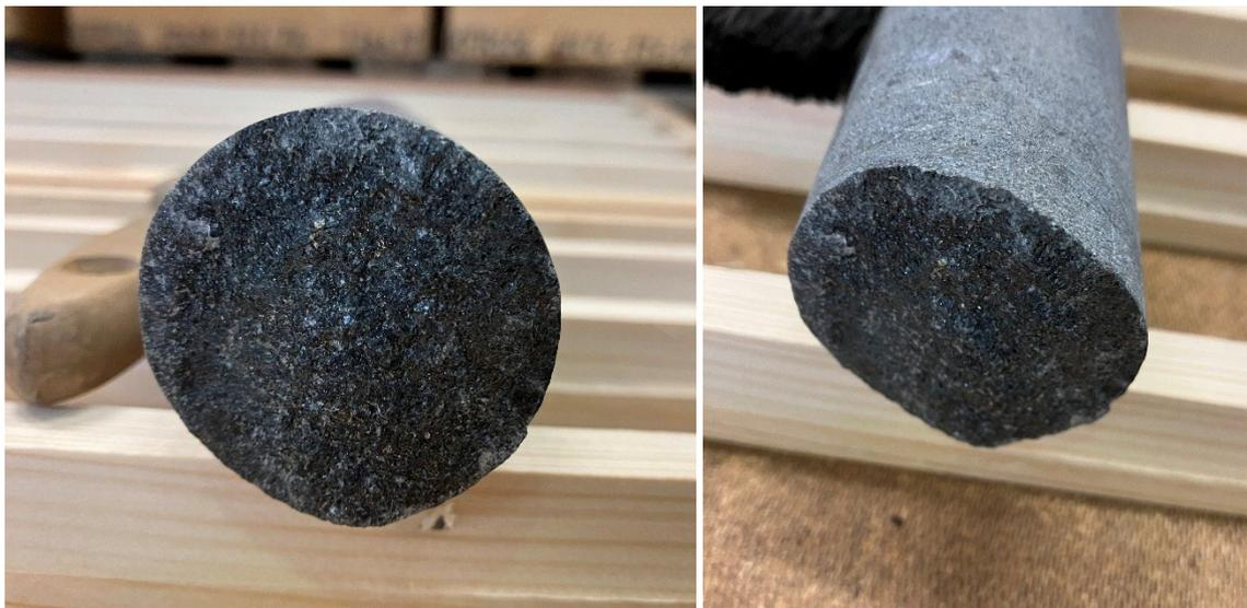
**Figure 5-5.** Fresh rough cross-section of an artificially broken amphibolite rock core (front and perspective views shown in the left and right figures, respectively).
