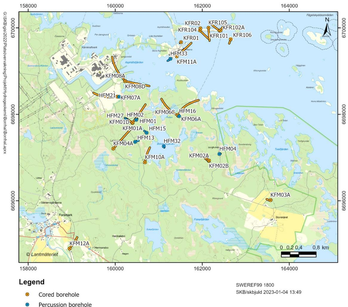
**Figure 3-1.** The location of most of the cored boreholes and percussion drilled boreholes. In this study data from boreholes KFM01A, KFM01D, KFM02A, KFM02B, KFM04A, KFM05A (not shown), KFM08C, KFM08D, KFM10A and KFM11A are used.
