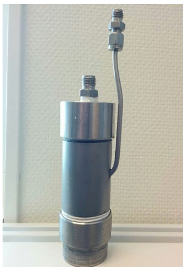
Figure 2-5. The docking unit, which is used together with the pump (GEOPUMP UV-45). Instead of using the mini-packer to isolate the lower part of the standpipe with the pump, the unit is tightly fitted to the tube in the bottom of the standpipe. The photo shows the docking unit used in normally equipped boreholes. The one used in KFM08D is modified to match with the special equipment in PEEK but is very similar to the one in the photo.
