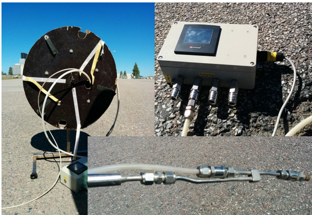
Figure 2-6. The equipment used for gas-lift pumping. To the left, the tubing lowered down the standpipe (the narrower tube for sample water and the wider for gas) on a bobbin to simplify the lowering. To the upper right the control unit for the pumping/gas supply and lower right the end of the gas-lift pump.
