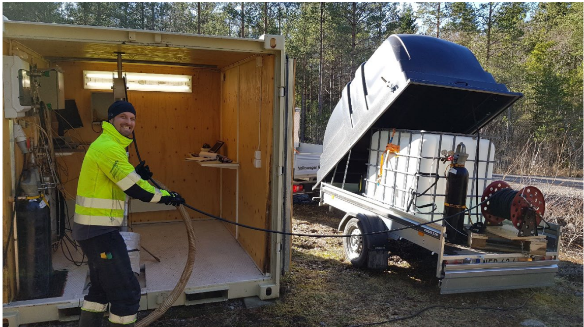
Figure 2-3. Cleaning equipment used to clean the standpipes prior to pumping and sampling.
