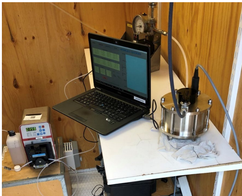
Figure 3-4. All equipment during injection. Pump for tracer injection to the left, circulation unit in the back, fluorescence detector in the front connected to the logger under the bench. The logger is connected to the computer during injection, which makes it possible to follow the concentration in real time.
