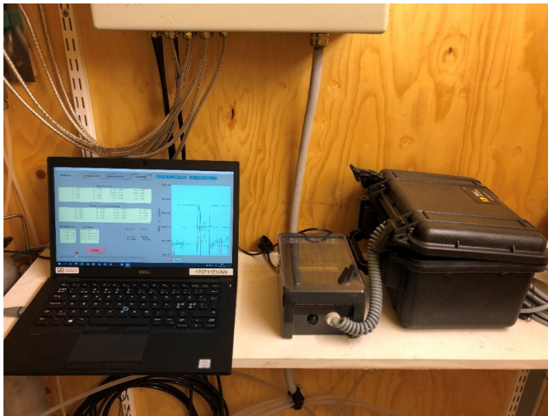
Figure 3-6. Data logger with transportation box and computer with ongoing measurements in the FLUO program.
