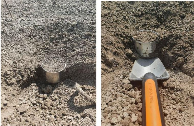
*Figure 5-6. Sampling of soil physical properties using steel cylinders. The cylinder was pressed down into the soil without disturbing the soil within the cylinder and then taken out carefully by digging around the cylinder.*
