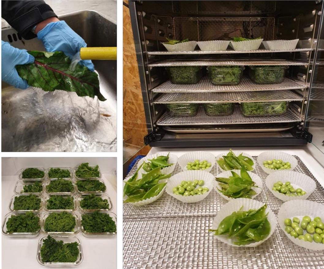
*Figure 5-11. Sample preparation of crops. Upper left picture shows rinsing of crops using tap water, lower left picture shows rinsed crops ready for drying and the right-hand picture crops in the oven ready for drying.*
