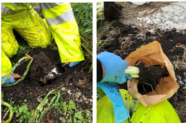
*Figure 5-7. Pictures showing the sampling of root soils. The roots and the soil close to the roots were collected using two small spades. The root soil zone was cleaned from the excess soil by hand, and the soil closest to the roots was sampled into a paper bag by shaking the roots.*
