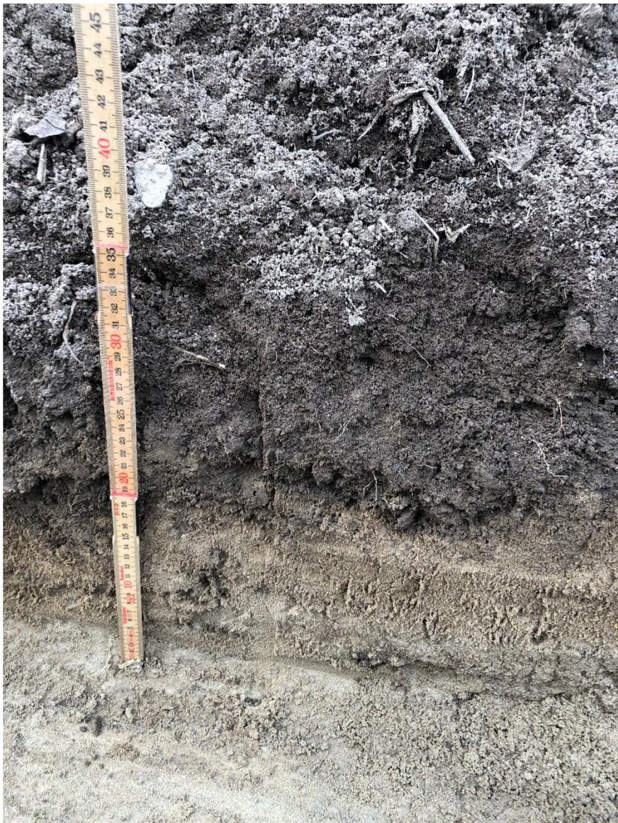
*Figure 5-8. Soil profile at site PBY004. The brown cultivated soil with higher organic matter content is overlaying a sandier soil layer under the ploughing depth.*
