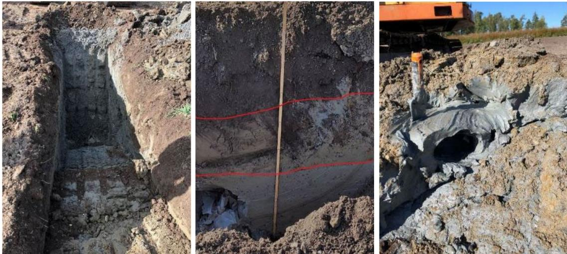
*Figure 4-3. One of the shafts (left). The middle panel shows the different layers and the picture to the right shows sampling of the glacial clay.*
