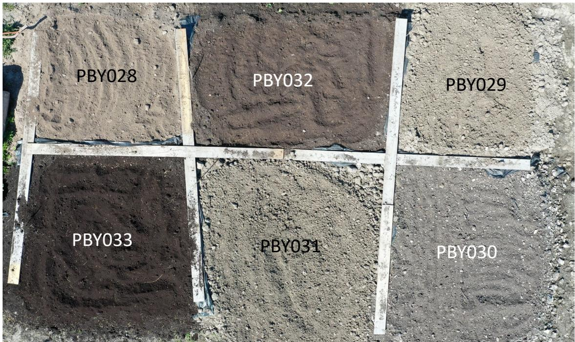
**Figure 5-2. Cultivation plots constructed in 2021 with soil from Lohärad in the vicinity of the Byle site. According to the soil map PBY028 represents moraine clay, PBY029 and PBY033 silty clay, and PBY030, PBY032 and PBY033 represent organic soils.**
