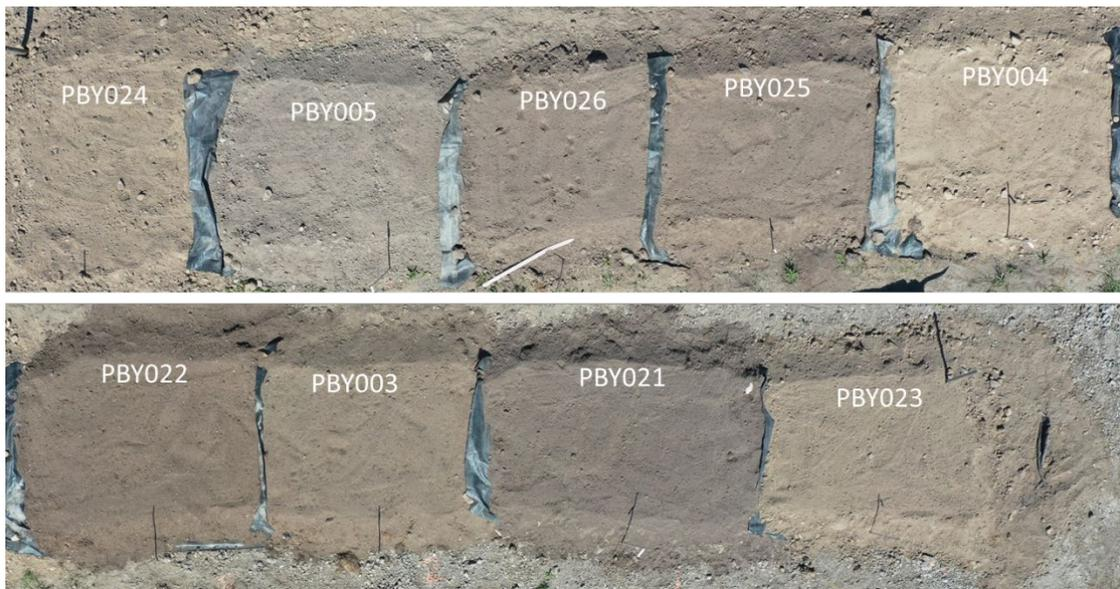
*Figure 5-1. Cultivation plots for soils used in the cultivation experiment in 2020. According to the soil map they represent gyttja clay (PBY022, 003, 021), glacial clay (PBY005, 026, 025) and clayey till (PBY024, 004, 023).*
