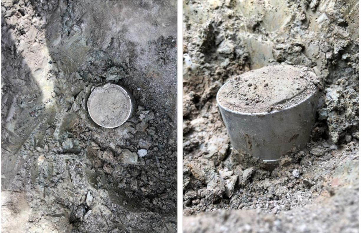
*Figure 5-9. Cylinder for measuring soil density and porosity was placed at the bottom of the pit below ploughing depth. Pictures from site PBY029.*
