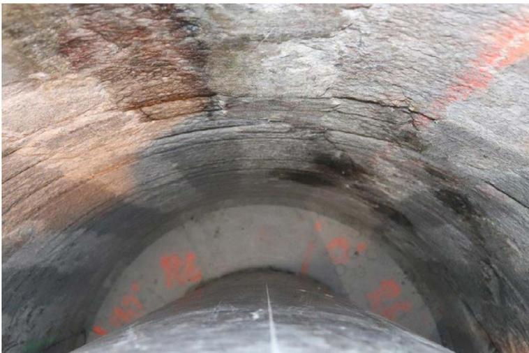
**Figure 5-13.** Sampling of layer R-16 between the canister and the rock surface.
