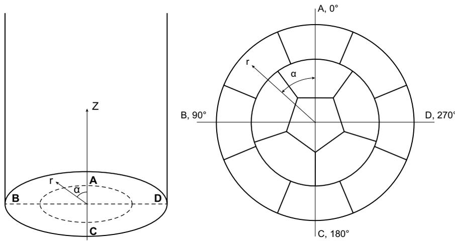
**Figure 3-2.** Coordinate system used when describing the positions of the installed sensors or samples. A, 0 degrees are pointing towards the end of the tunnel and C, 180 degrees towards the tunnel mouth.
