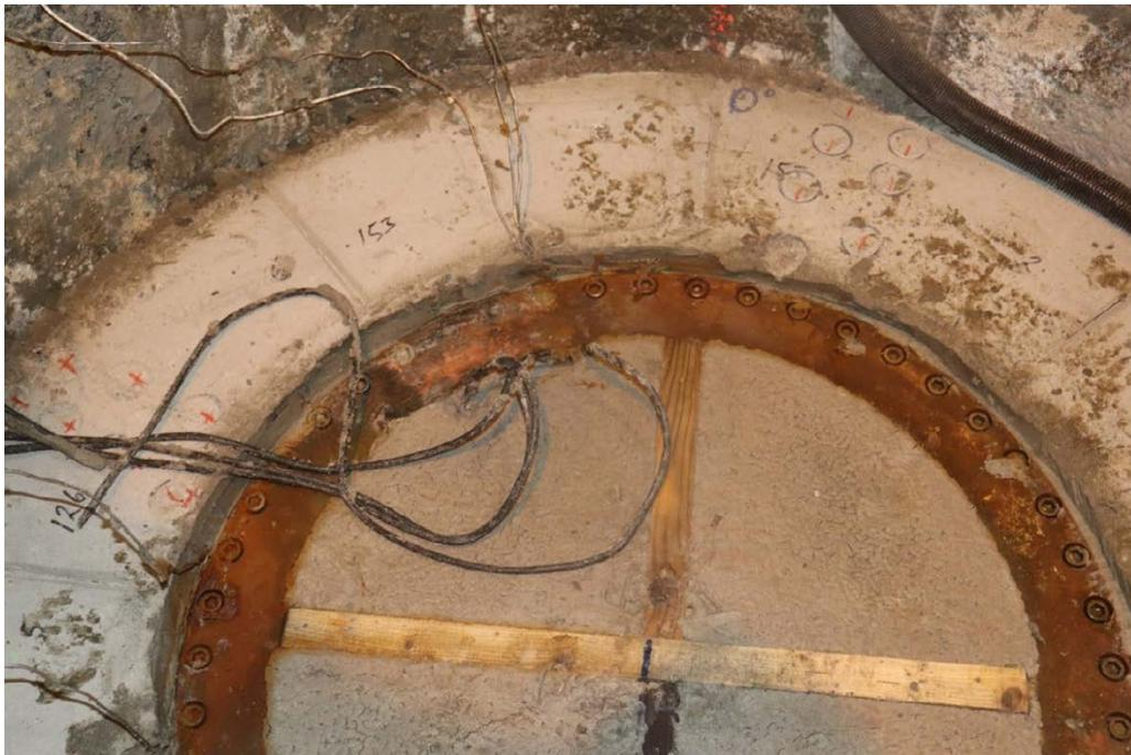
***Figure 4-19.*** The canister was exposed after the removal of layer C3. The top of the canister is treated differently in this test than it will be in the repository due to the handling of sensor cables, for examples the small planks will not be used in real operation.
