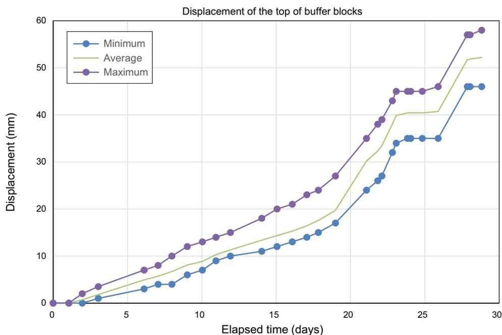
Figure 5-8. Minimum, maximum and average displacement of the top buffer blocks.
