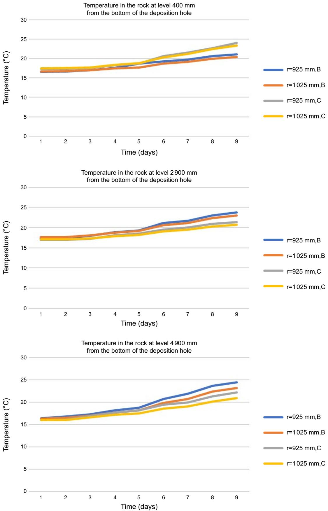
**Figure 4-12.** The temperature evolution in the surrounding rock at three levels in the deposition hole. Top graph: 400 mm, middle graph: 2900 mm and bottom graph: 4900 mm, all from the bottom.
