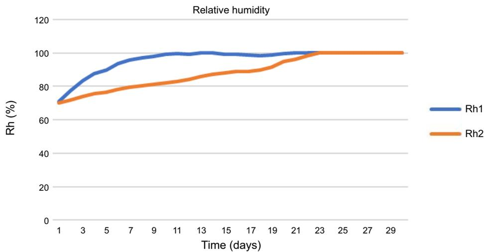
Figure 5-7. The evolution of relative humidity in the buffer layer R20.
