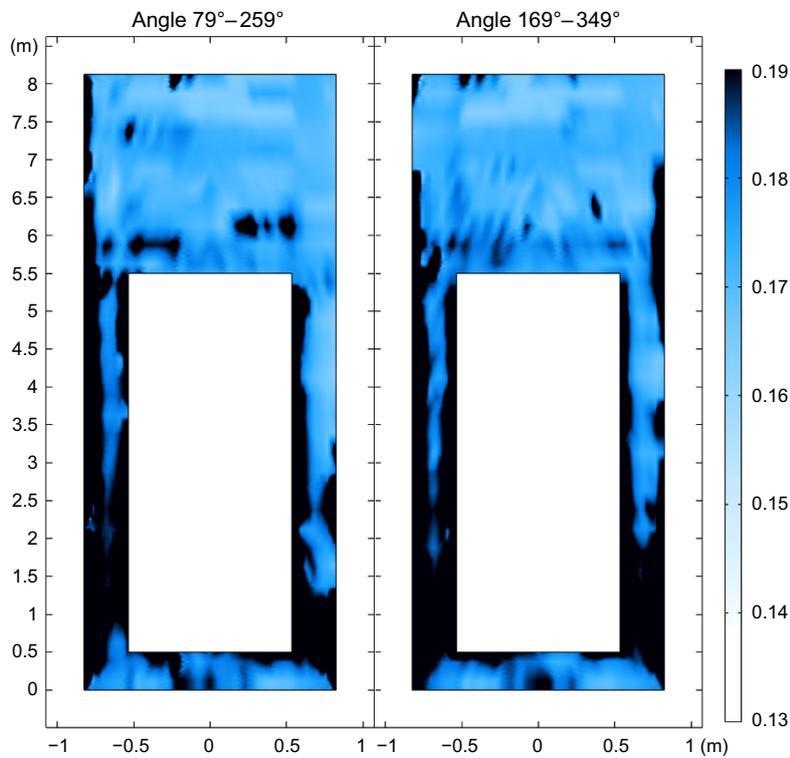
**Figure 6-8.** Water content in the buffer blocks in Test\_Seg\_0.1 with segmented blocks and an artificial inflow of 0.1 l/min. The scale has been cut of at 13 % and 19 % to be able to see the wetted areas.
