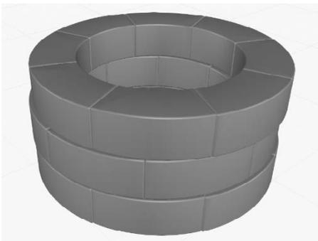
*Figure 4-1. Principle how the block joints are displaced relative to each other.*
