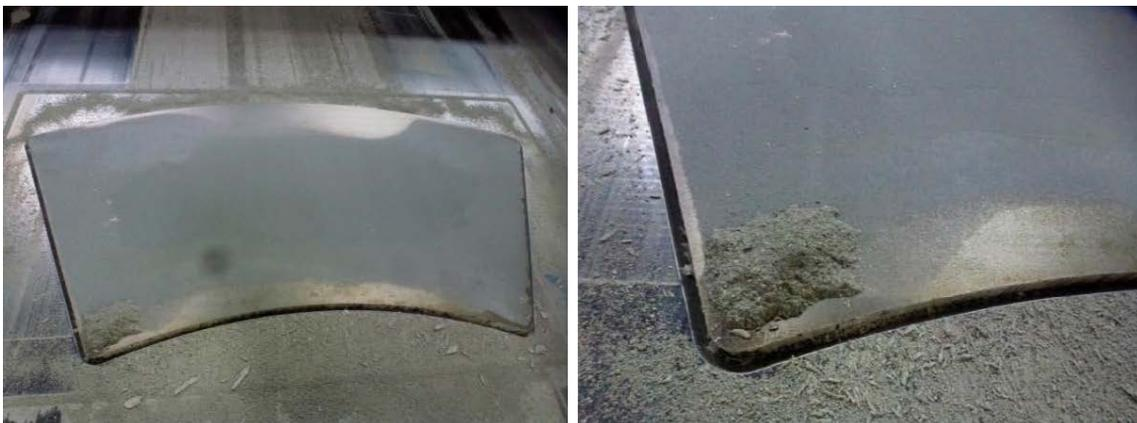
*Figure 2-6. Bottom mould plate with material build-up.*
