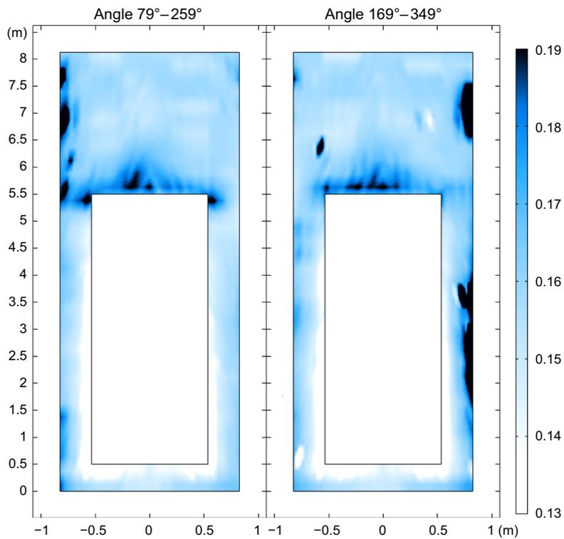
**Figure 6-6.** Water content in the buffer blocks in Test\_Seg\_N with segmented blocks and a natural inflow. The scale has been cut of at 13 % and 19 % to be able to see the wetted areas.
