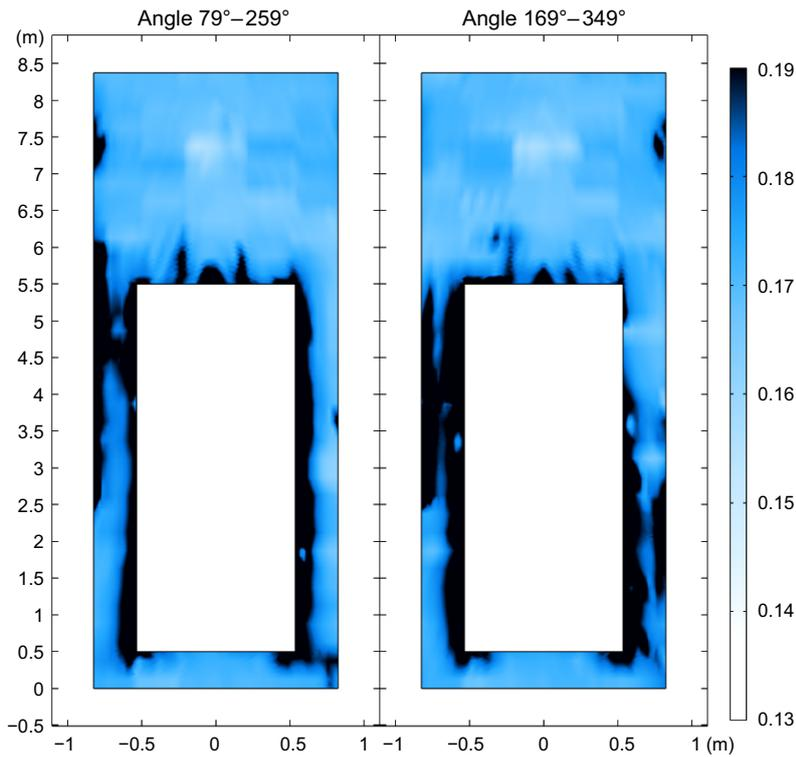
**Figure 6-7.** Water content in the buffer blocks in Test\_Seg\_0.01 with segmented blocks and an artificial inflow of 0.01 l/min. The scale has been cut of at 13 % and 19 % to be able to see the wetted areas.
