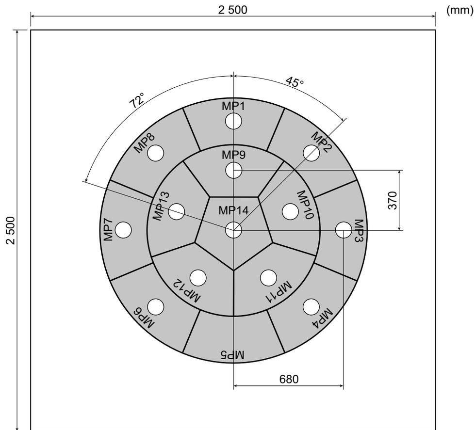
**Figure 3-4.** Protective lid with openings for measuring block displacement. The openings are named measurement points, MP:s.
