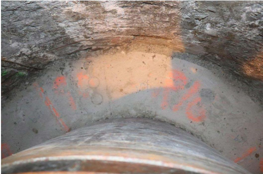
**Figure 6-1.** The inner gap is closed since water entered the gap and caused the bentonite to swell.
