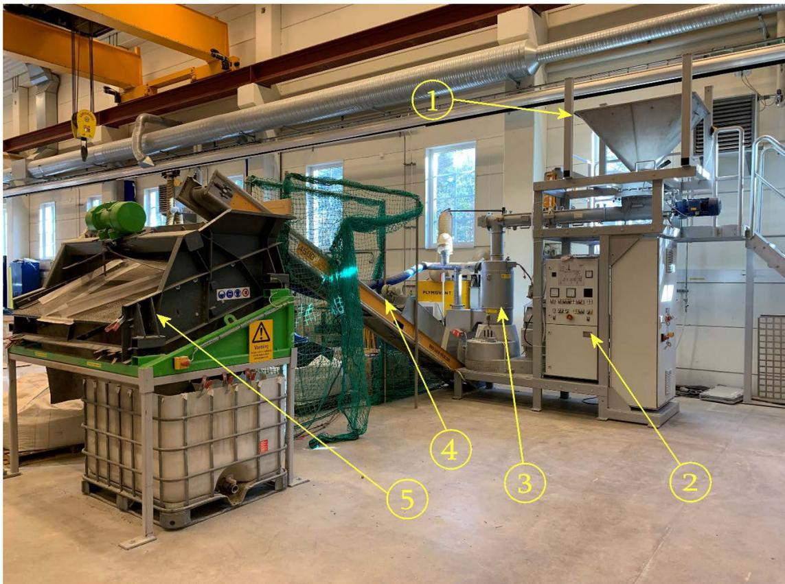
**Figure 2-7.** The setup for the production line. 1) Material container, 2) Control unit, 3) Extrusion unit, 4) Belt transporter unit, 5) Shaker table.
