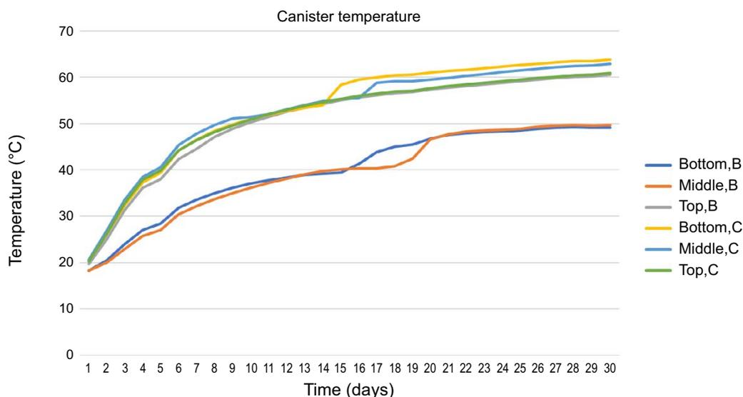
**Figure 5-5.** The temperature evolution on the canister surface as function of time. The thermocouples are placed at the bottom, at mid height and at the top of the canister in two directions B and C.
