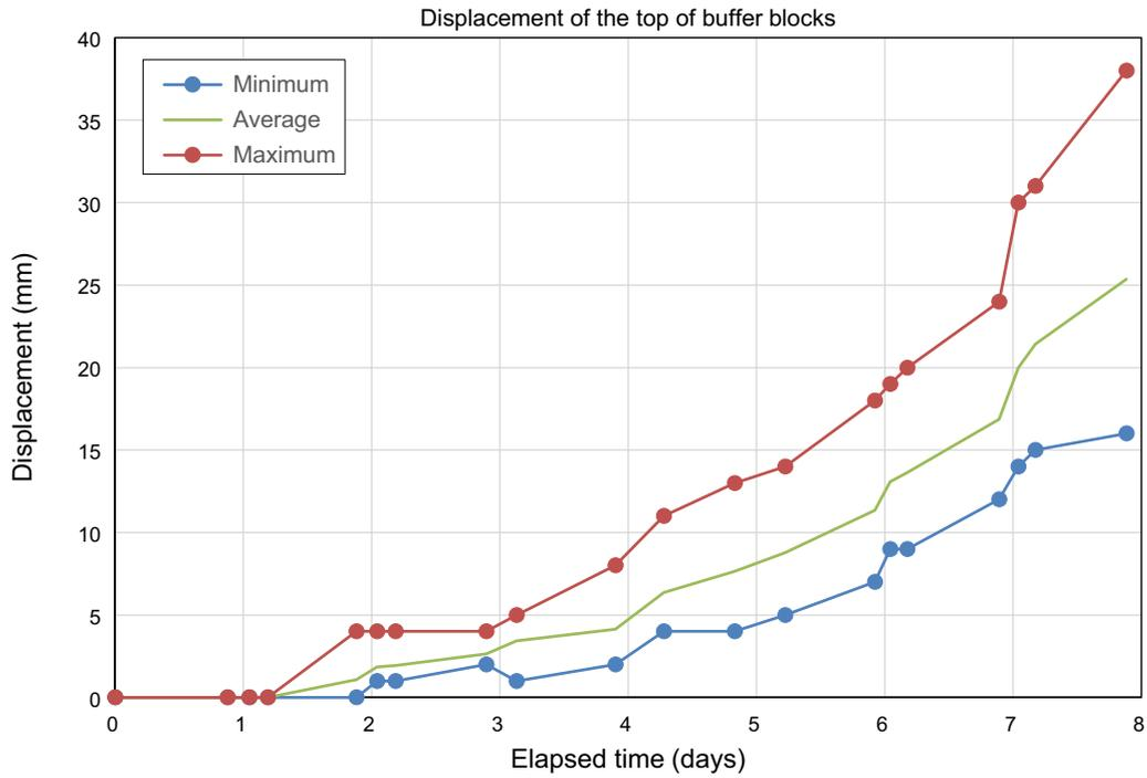
Figure 4-14. Minimum, maximum and average displacement of the top buffer blocks.
