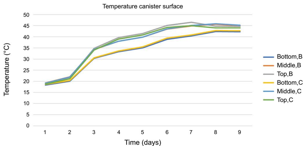
**Figure 4-11.** The temperature evolution on the canister surface as function of time. The thermocouples are placed at the bottom, at mid height and at the top of the canister in two directions B and C.
