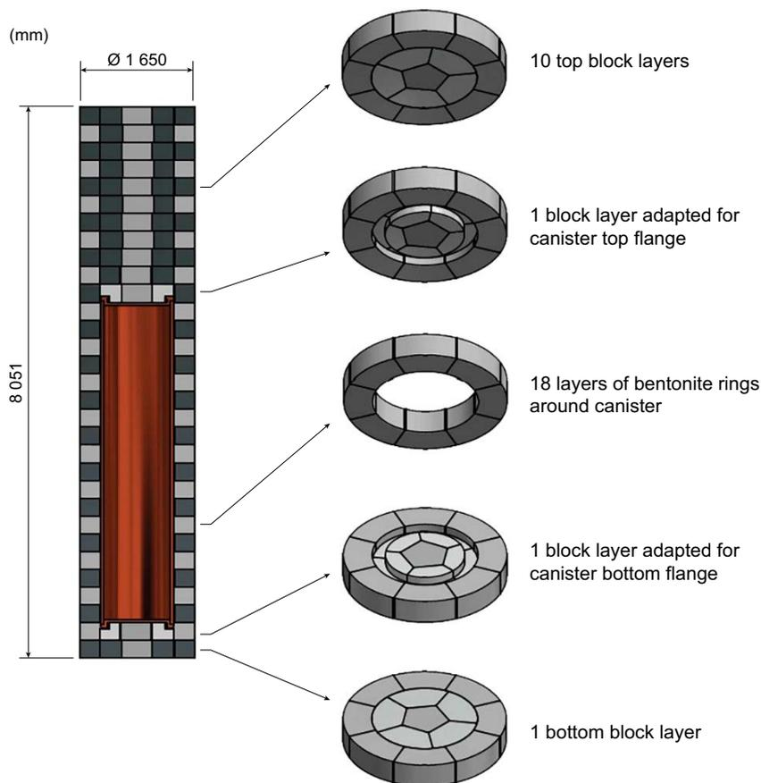
*Figure 1-1. Design of a segmented buffer.*
