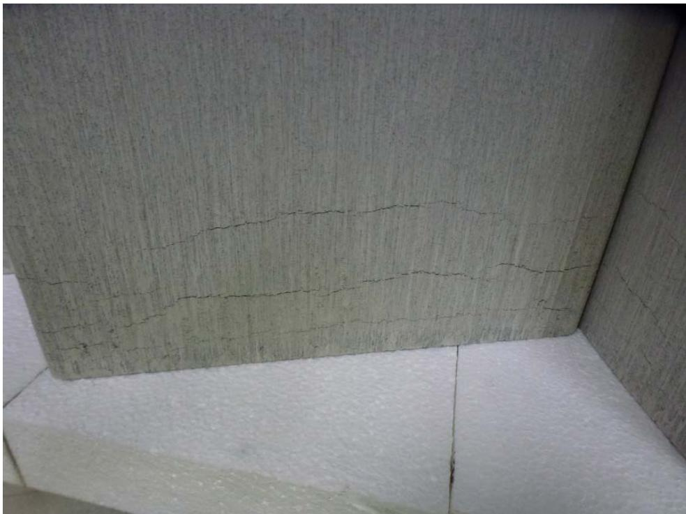
*Figure 2-5. Euro-pallet with blocks. Small horizontal cracks can be seen on the lower half of the blocks.*
