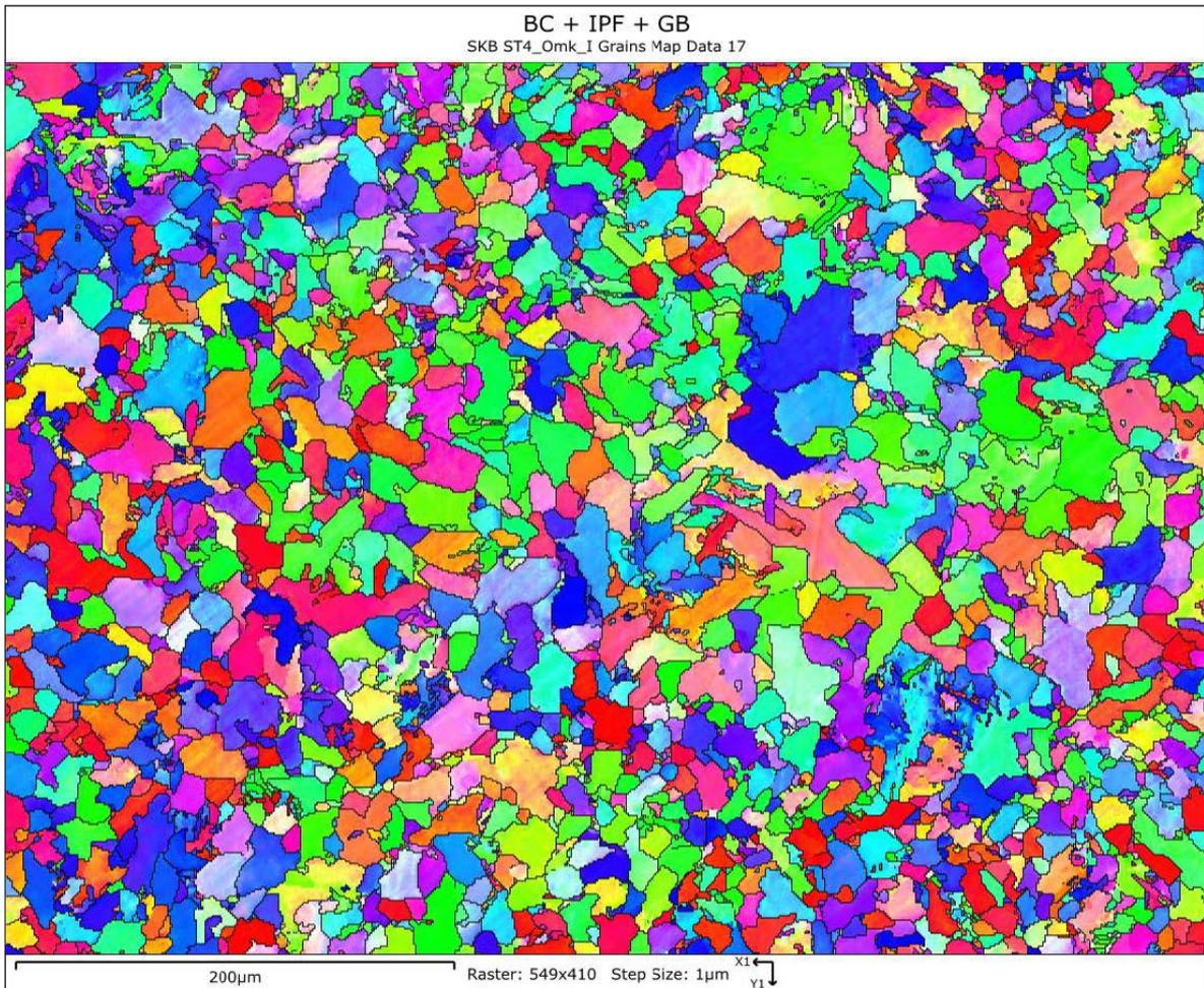
**Figure A-37.** Specimen ST4 in circumferential direction. Close to inner surface. Lower magnification EBSD analysis showing the grain structure.
