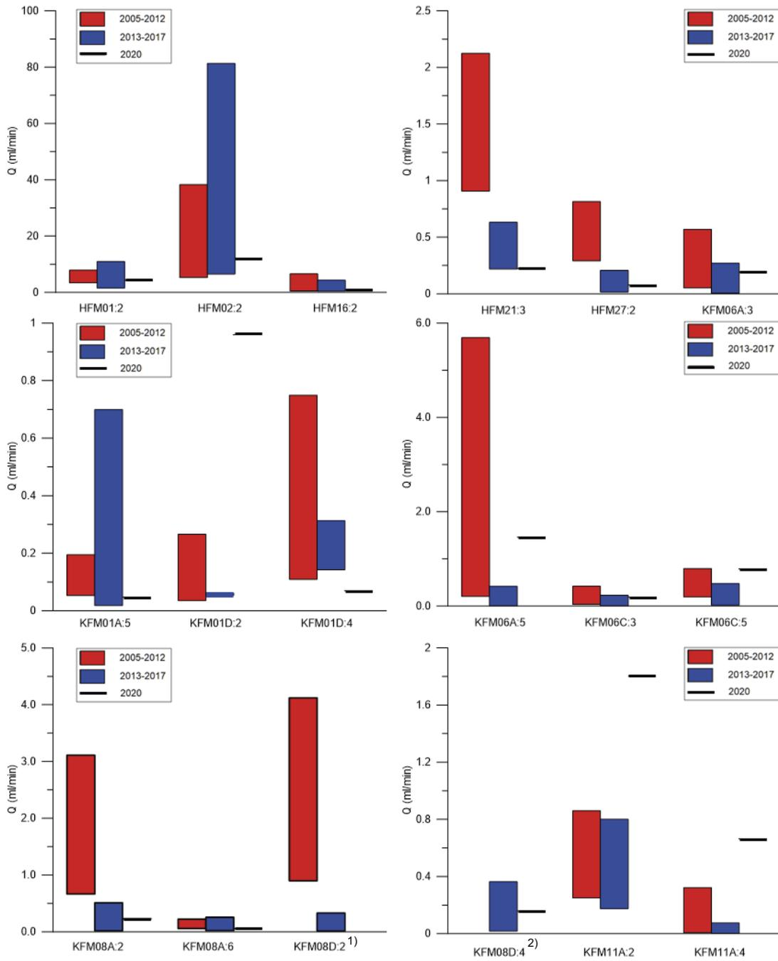
**Figure 5-4.** Summarized results from groundwater flow measurements in 2005–2020. HFM33 was measured the first time in 2020 and is excluded from the figure. 1) In KFM08D:2 no flow was obtained in 2020. 2) For KFM08D:4 the leakage influenced flow from 2005–2012 is excluded in the figure.
