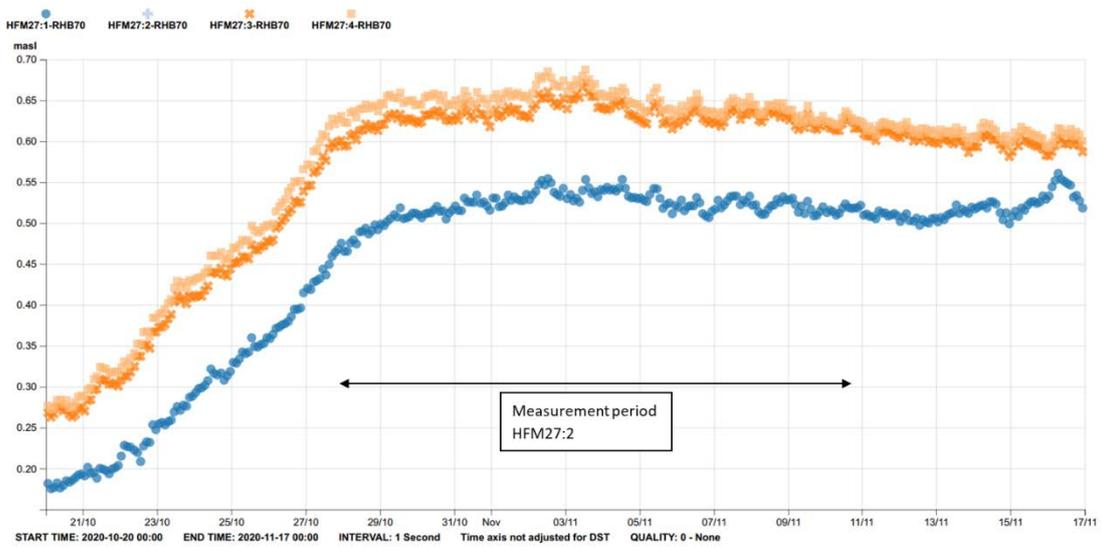
**Figure A2-13.** Measured section: HFM27:2. Unfortunately, data is missing for section 2 due to malfunctioning monitoring equipment. However, the level in section 2 usually follows about 5 centimeters below sections 3 and 4.
