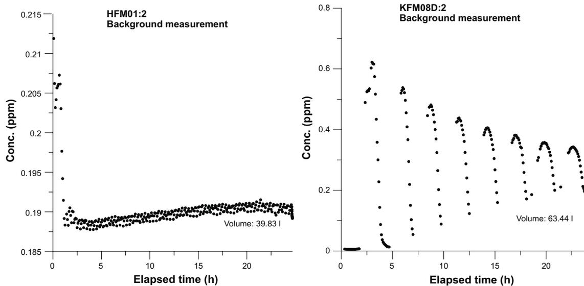
**Figure 4-2.** Background concentrations measured during the day before tracer injection. Percussion borehole section HFM01:2 (left) and cored borehole section KFM08D:2 (right).
