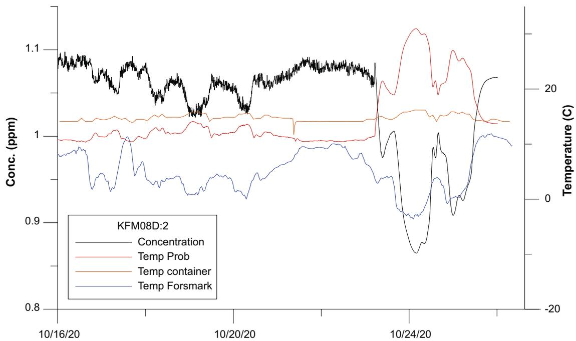
Figure 5-3. Measured concentration in KFM08D:2 and water temperature in the measuring probe, the temperature in the container and outside temperature in Forsmark. The pump stop probably occurred during the morning hours of 23rd October as indicated by the large increase in water temperature inside the detector due to stagnant water heated by the detector lamp.
