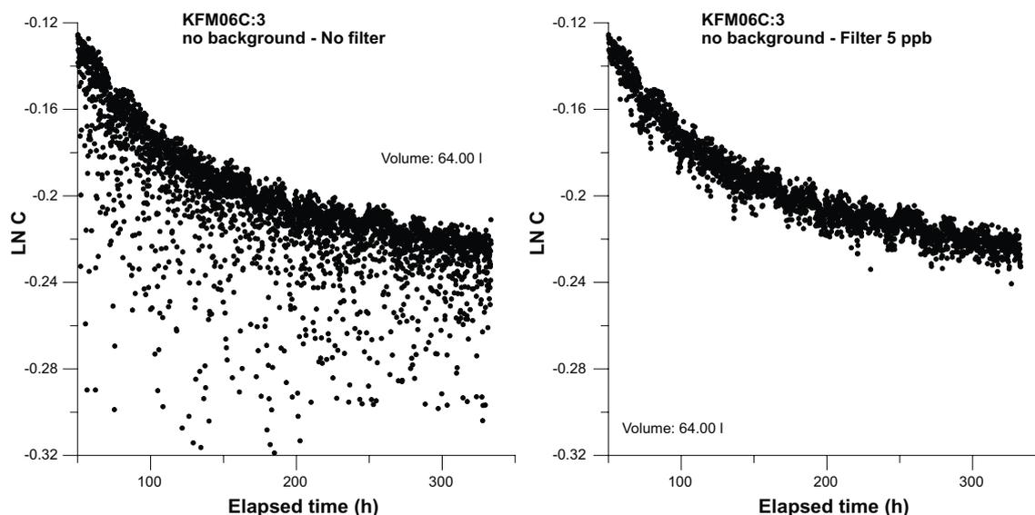
Figure 4-1. Unfiltered and filtered data. Fluctuations are due to gas bubbles.
