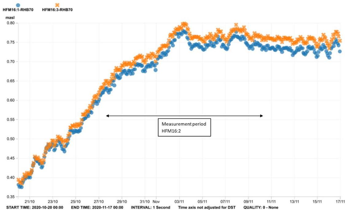
Figure A2-11. Measured section: HFM16:2. Unfortunately, data is missing for section 2 due to malfunctioning monitoring equipment. However, the level in section 2 usually follows the two other sections within some centimeter.
