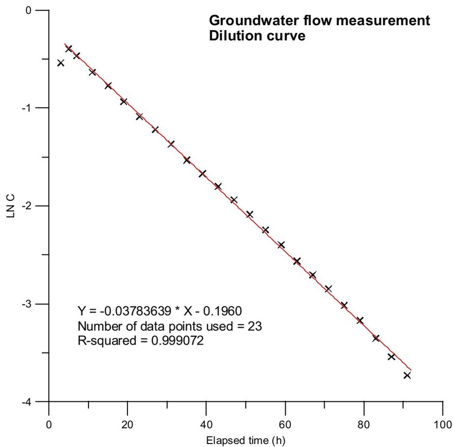
**Figure 3-7.** Example of a tracer dilution graph (logarithm of concentration versus time), including straight-line fit. The used interval is chosen by eye assessment as the injection and start-up effects varies from section to section (Andersson et al. 2018).
