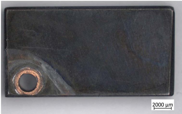
**Figure 5-10.** The surface appearance of the coupon sample (no straining) after sulphide test 1.
