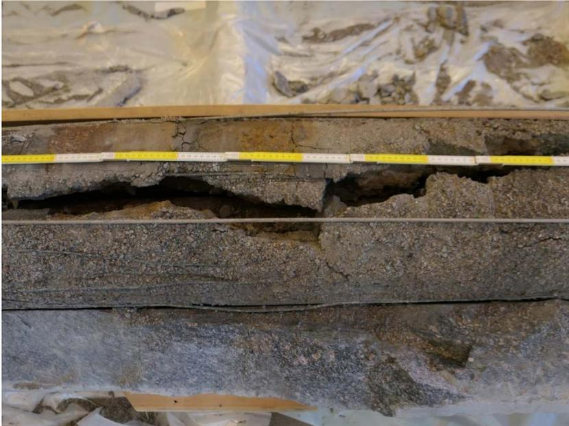
**Figure 5-13.** Large fractures in the bentonite were present along the complete test package. The photo shows the situation for block no. 20 (left) to block no. 11 (right).
