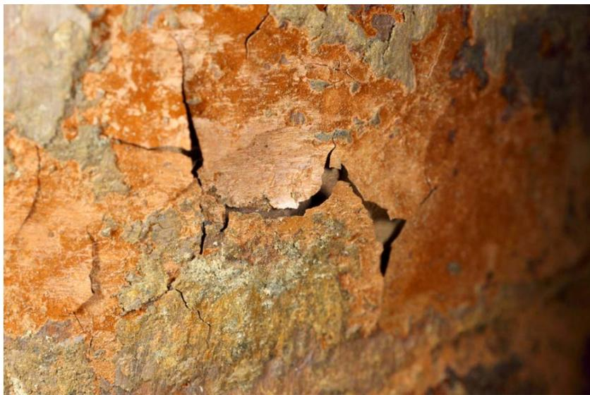
**Figure 6-23.** ABM2 Febex block 9. A crust on the surface of the iron heater.
