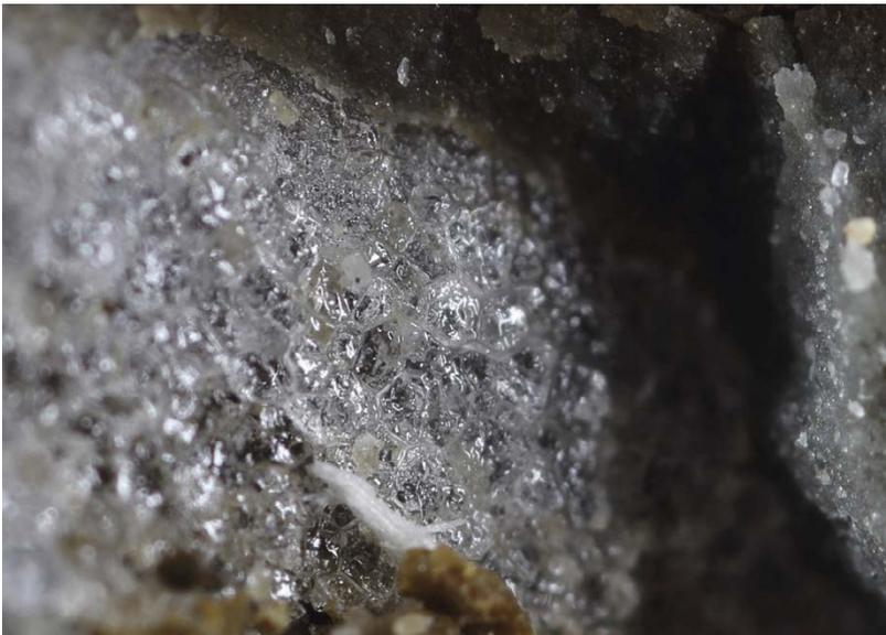
*Figure 6-19. ABM2. A highly glassy halite present in lenses of approximately 8 × 4 mm size (Kunigel #22).*
