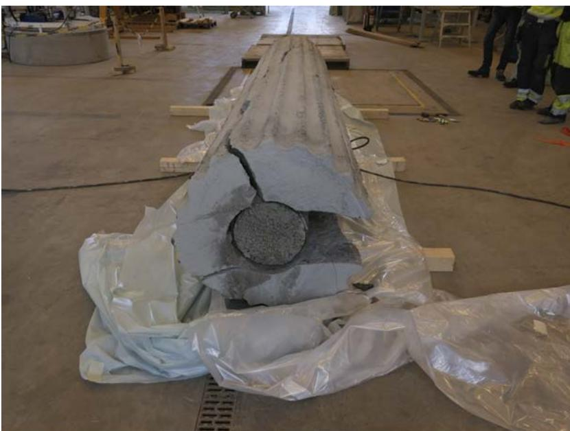
*Figure 5-12. The bottom of the test package. A minor rock piece fell off during the uplift.*
