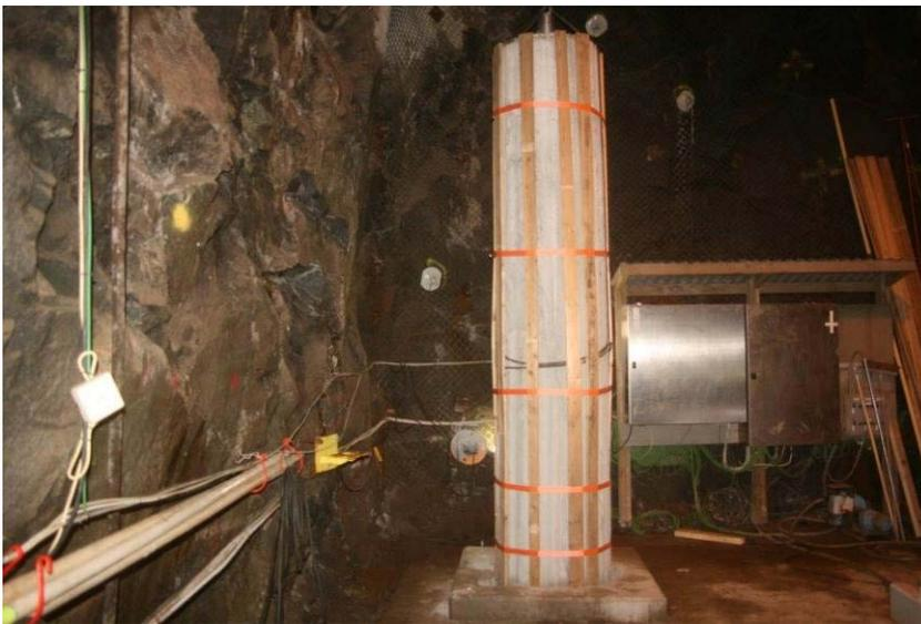
*Figure 5-9. Photo showing the released test package during the uplift.*
