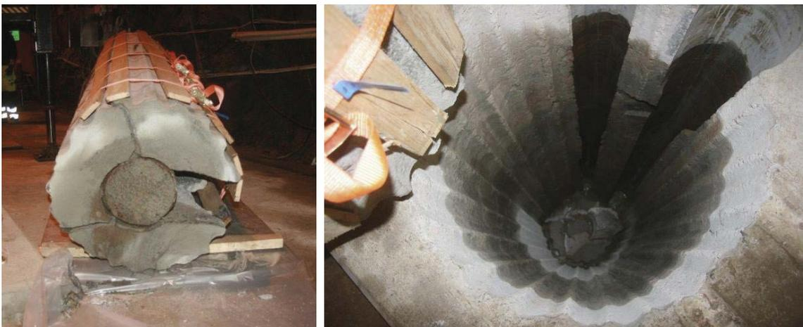
*Figure 5-10. Left: The test package was lifted up almost in one piece. A minor rock piece close to the bottom fell off during the uplift. Right: Photo showing the rock after retrieval of the test package.*
