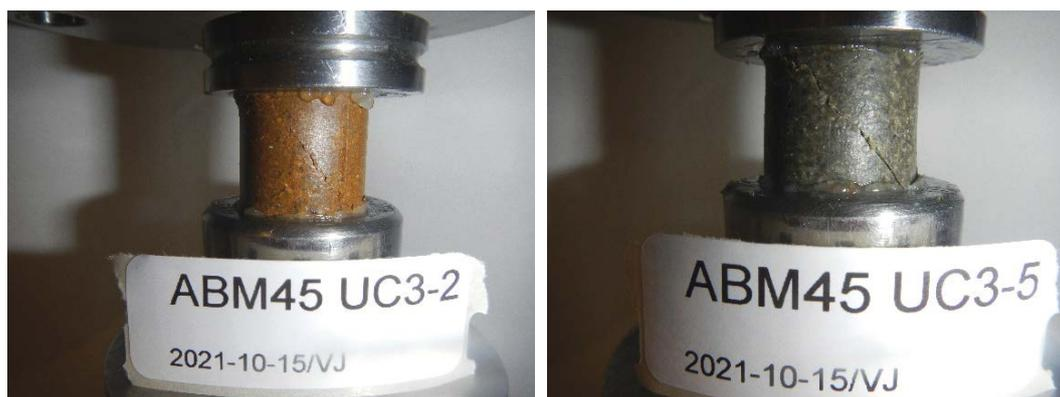
**Figure A2-9.** Photo after unconfined compression tests on ion-exchanged specimens of Asha 505 and MX-80 with dry densities  $1550 \text{ kg/m}^3$  and  $1490 \text{ kg/m}^3$  respectively.
