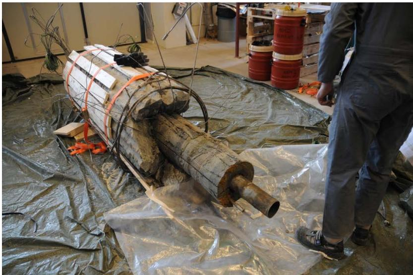
*Figure 4-15. The bottom plate has been cut off from the steel tube and some of the blocks have been removed.*
