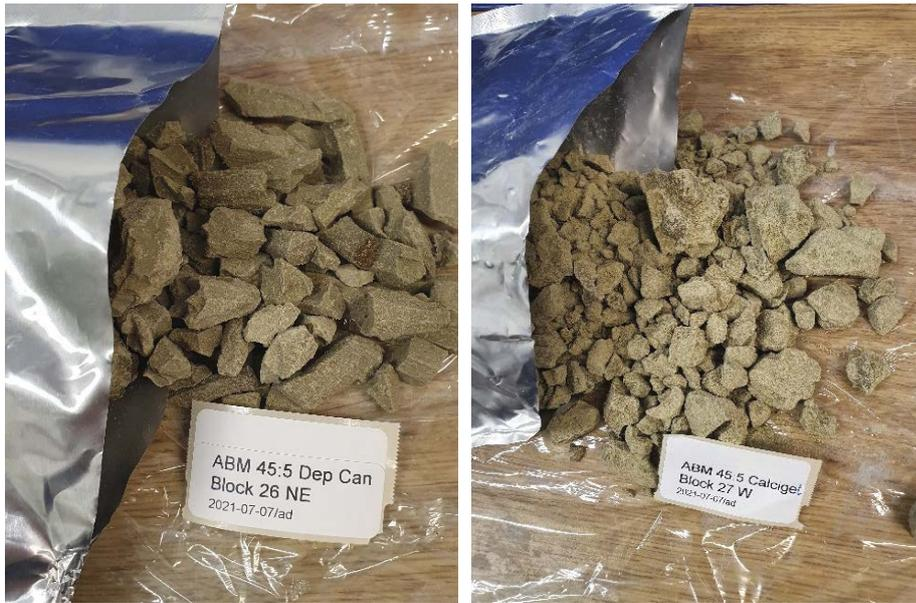
**Figure A1-3.** Samples from ABM 5 for the analyses; Deponit CA-N (to the left) and Calcigel (to the right). The samples were taken from block number 26 and 27, respectively.
