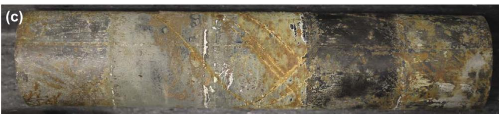
**Figure 4-16.** In the ABM2 (a) the rock was locally highly fractured, (b) some of the blocks were very fragile and fell into parts when the rock cover was removed, and (c) the iron heater was showing a different corrosion pattern in contact with different bentonites.
