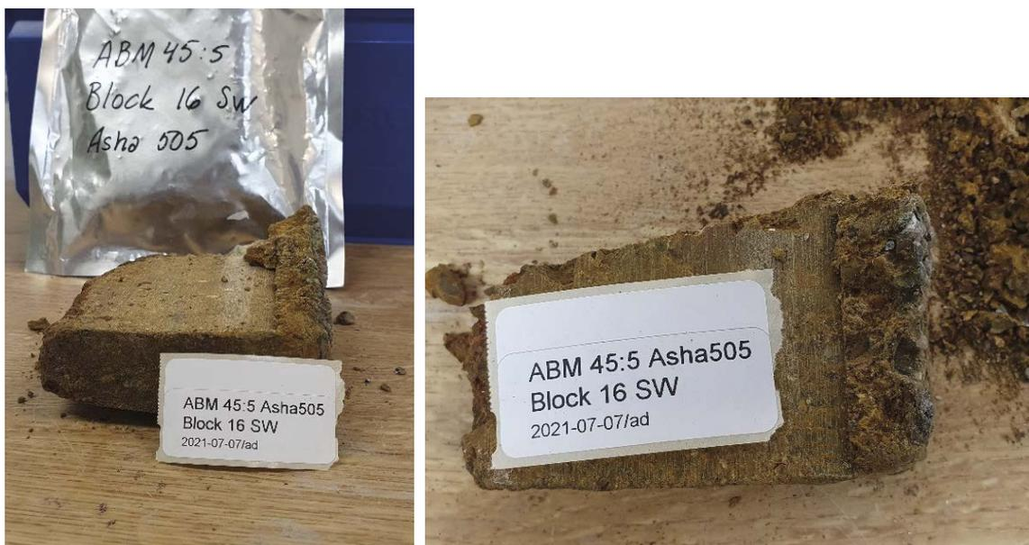
*Figure A1-2. Asha505 samples from ABM 5 used for the analyses. Samples were taken from block number 16.*
