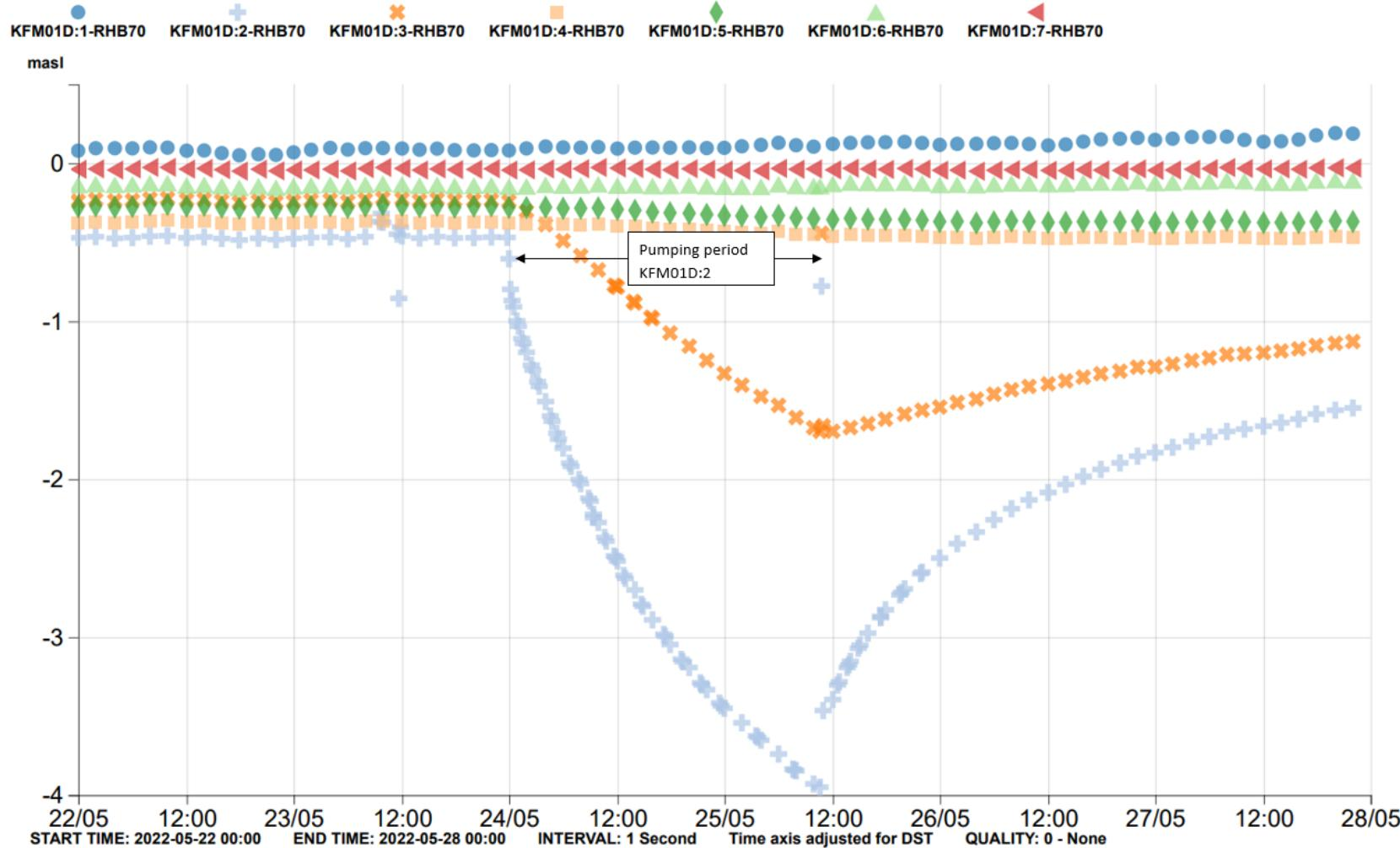
**Figure A5-2.** Pumping and drawdown in KFM01D:2 in May 2022. Sections KFM01D:3, KFM01D:4 and KFM01D:5 were affected by the pumping in KFM01D:2.
