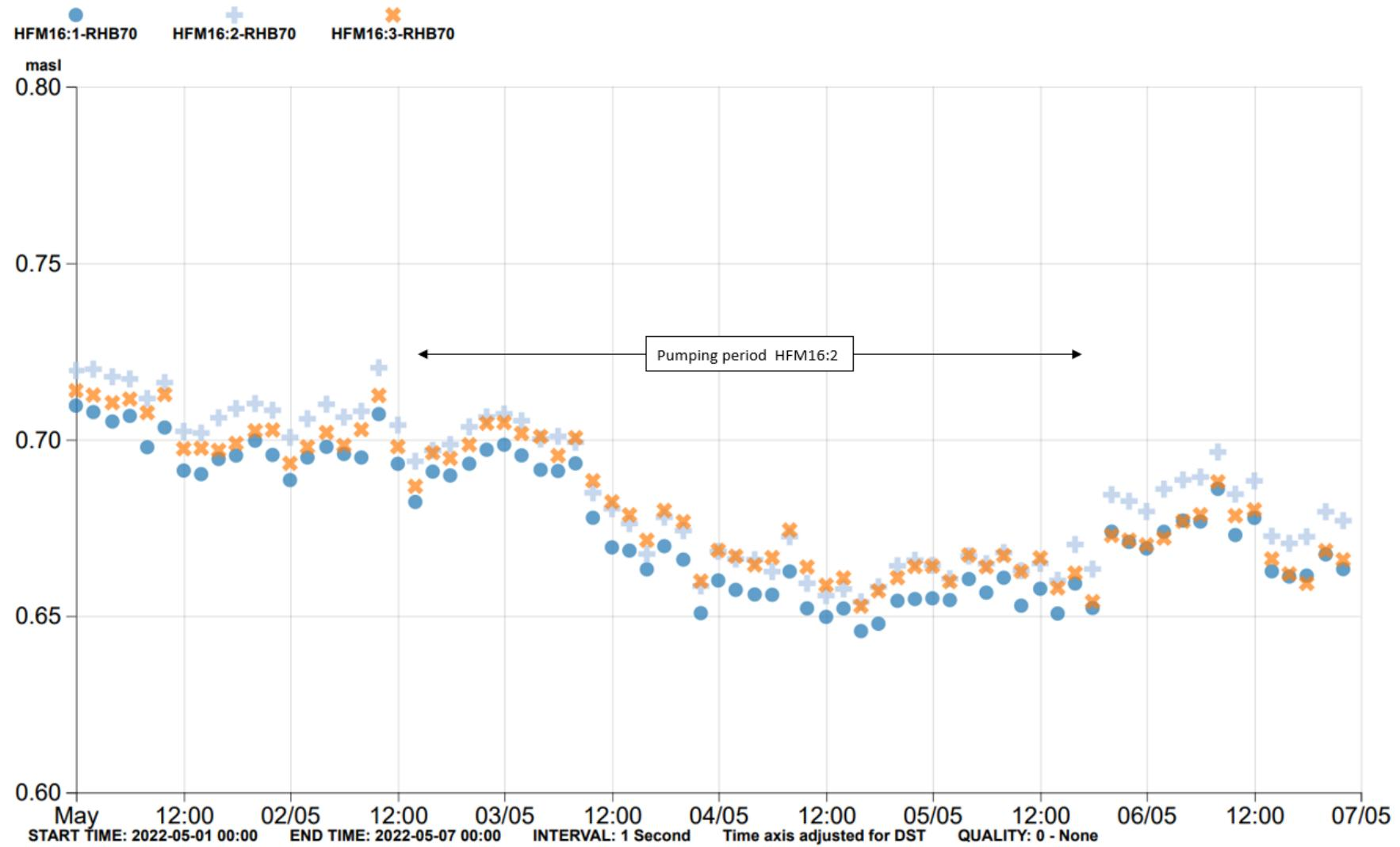
**Figure A5-20.** Pumping in HFM16:2 in May 2022. No significant drawdown was observed in any of the borehole sections.
