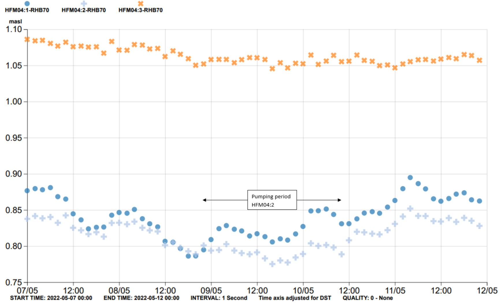
Figure A5-17. Pumping in HFM04:2 in May 2022. No significant drawdown was observed in any of the borehole sections.
