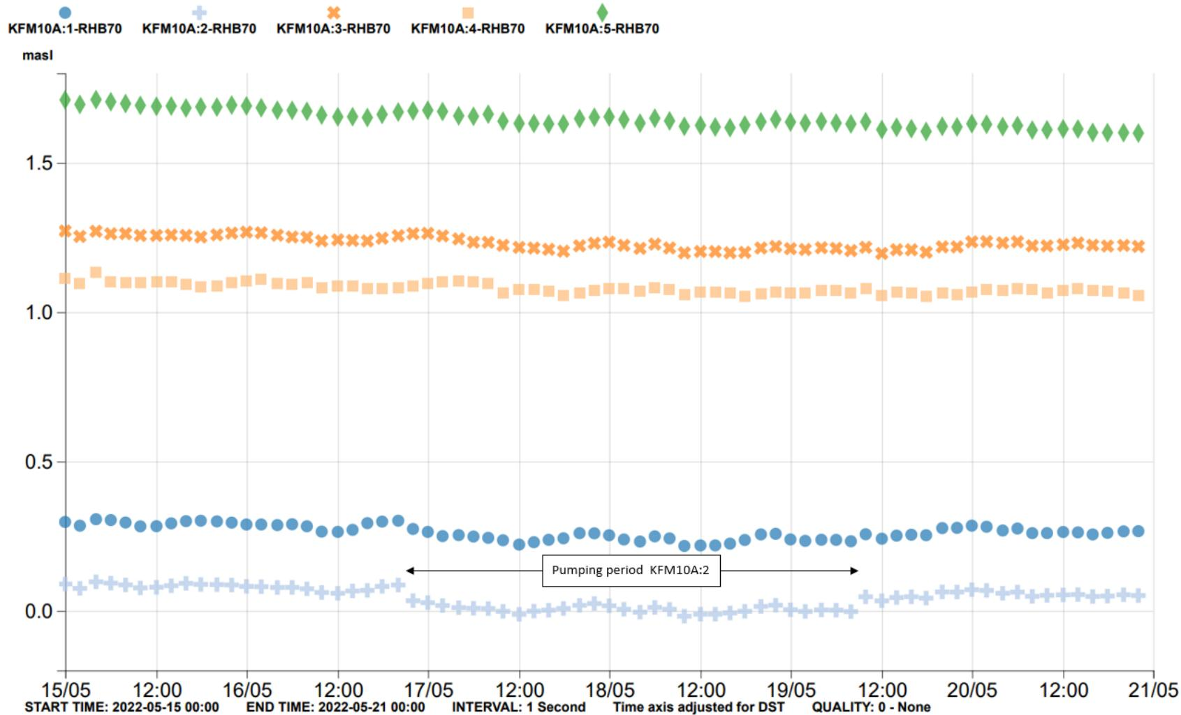
Figure A5-13. Detailed plot of pumping and drawdown in KFM10A:2 in May 2022. No (?) sections were significantly affected by the pumping.
