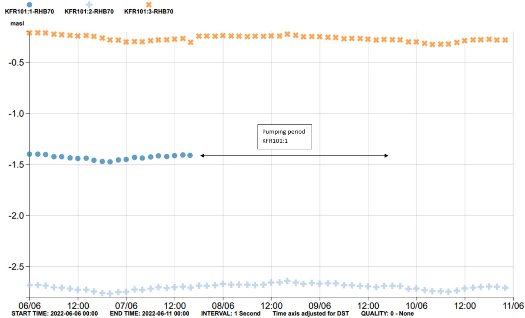
*Figure A5-25.* Pumping in KFR101:1 in June 2022. The pressure transducer in KFR101:1 was removed during the pumping. No significant drawdown was noted in any other section.
