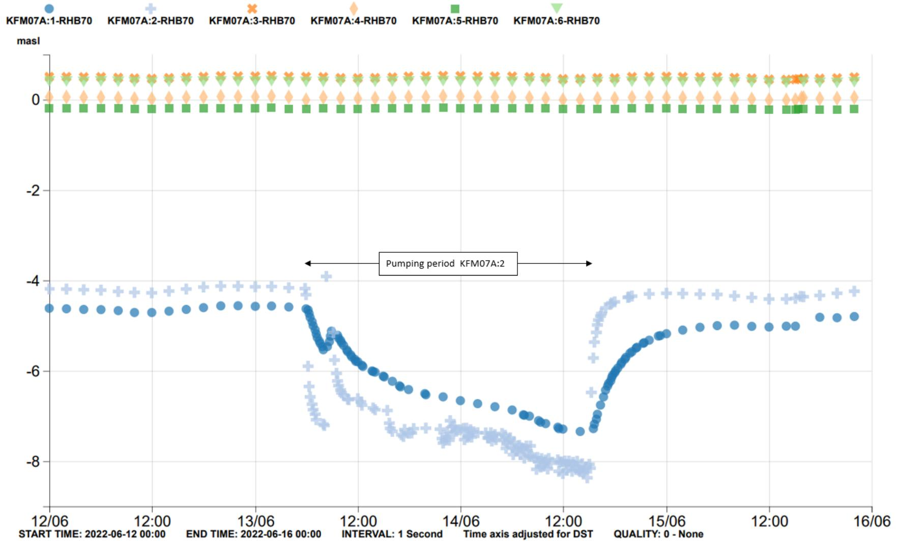
**Figure A5-10.** Detailed plot of pumping and drawdown in KFM07A:2 in June 2022. The pumping in section KFM07A:2 caused a response in KFM07A:1.
