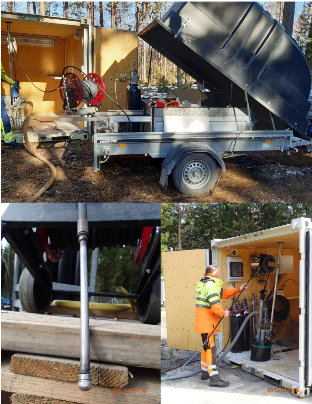
*Figure 2-2. Cleaning equipment used to clean the standpipes prior to pumping and sampling.*
