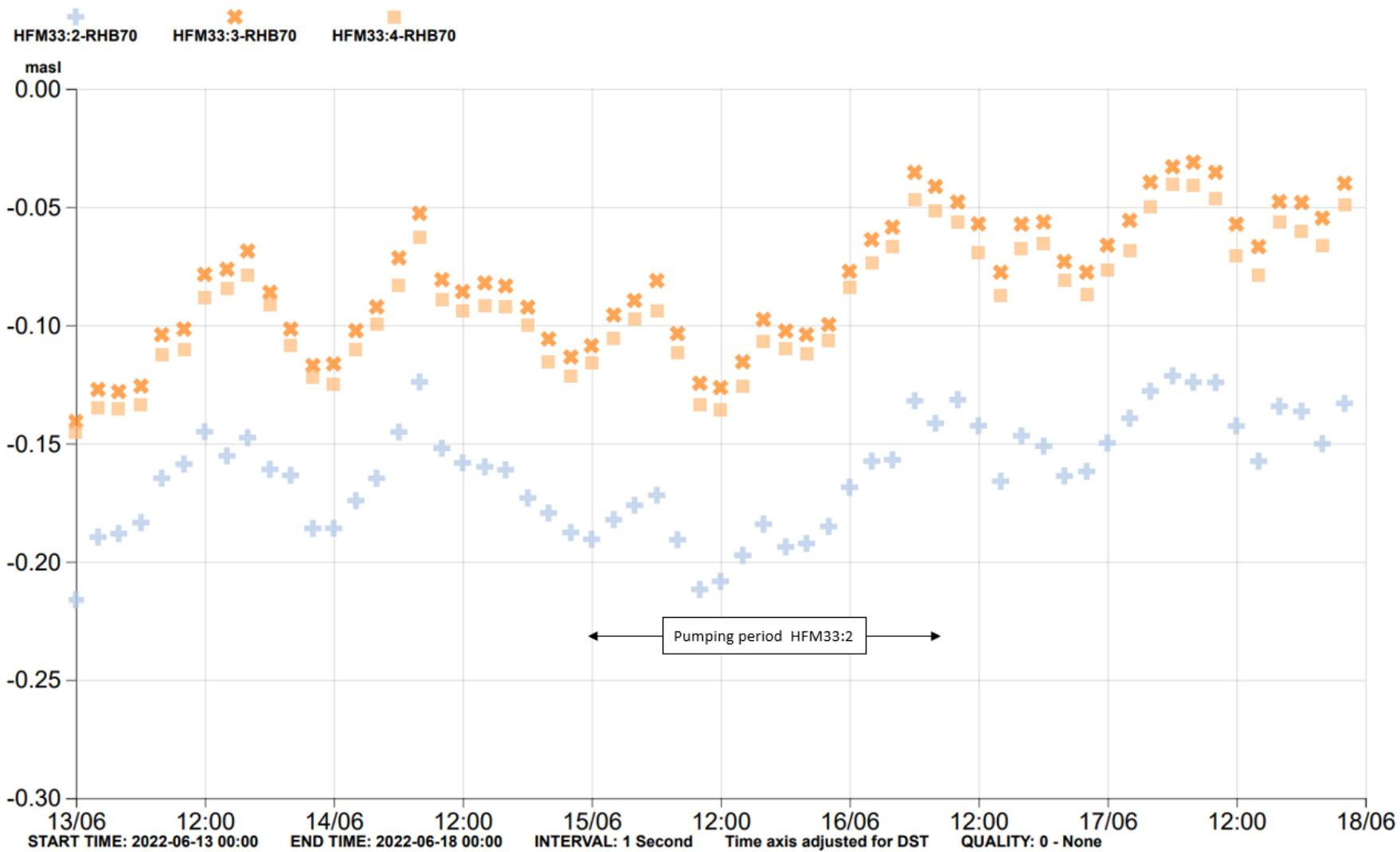
**Figure A5-24.** Pumping in HFM33:2 in June 2022. No significant responses were observed.
