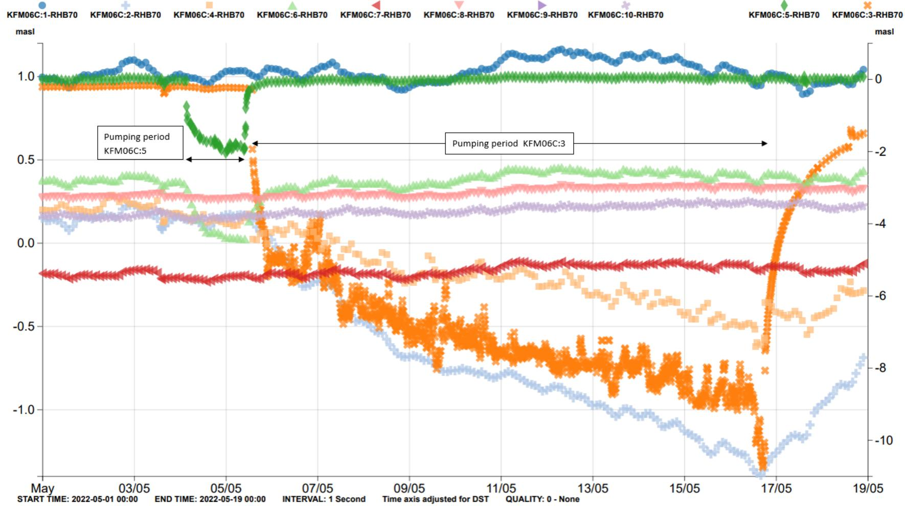
**Figure A5-9.** Pumping and drawdown in KFM06C:3 and KFM06C:5 in May 2022. Sections KFM06C:2 and KFM06C:4 were affected by the pumping in section KFM06C:3. The pumping in section KFM06C:5 caused a response in KFM06C:6.
