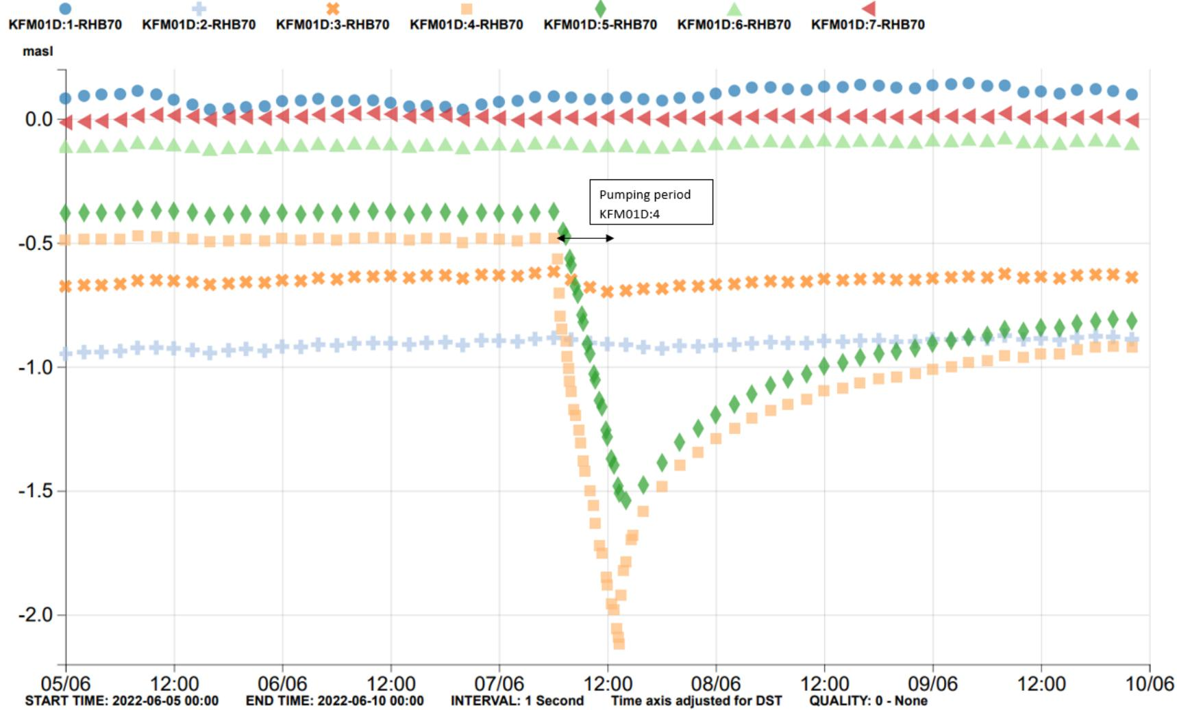
Figure A5-3. Pumping and drawdown in KFM01D:4 in June 2022. Sections KFM01D:3 and KFM01D:5 were affected by the pumping in KFM01D:4.
