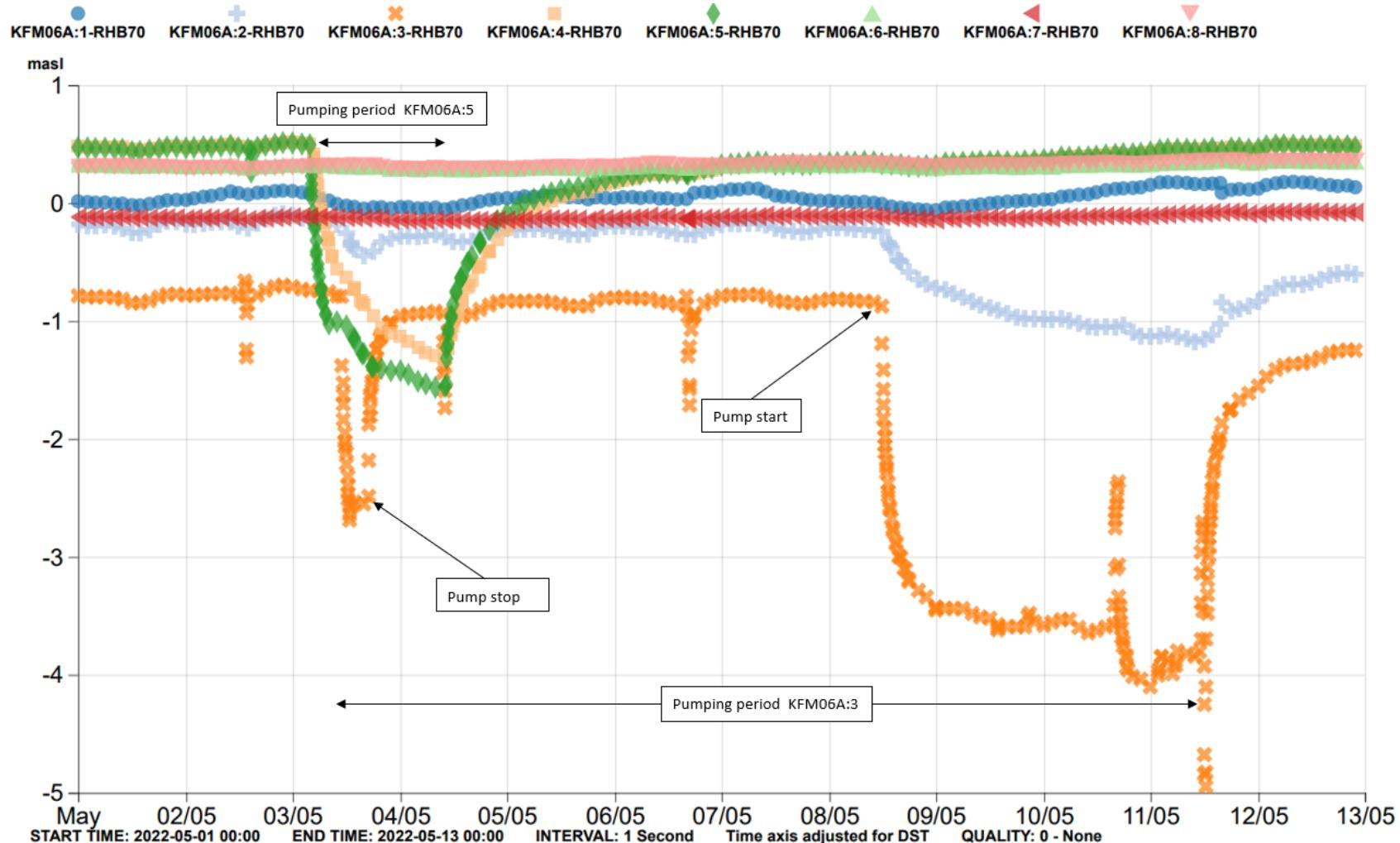
**Figure A5-8.** Pumping and drawdown in KFM06A:3 and KFM06A:5 in May 2022. Section KFM06A:2 was affected by the pumping in KFM06A:3. KFM06A:4 was affected by the pumping in section KFM06A:5. During the pumping period for KFM06A:3 a pump stop occurred.
