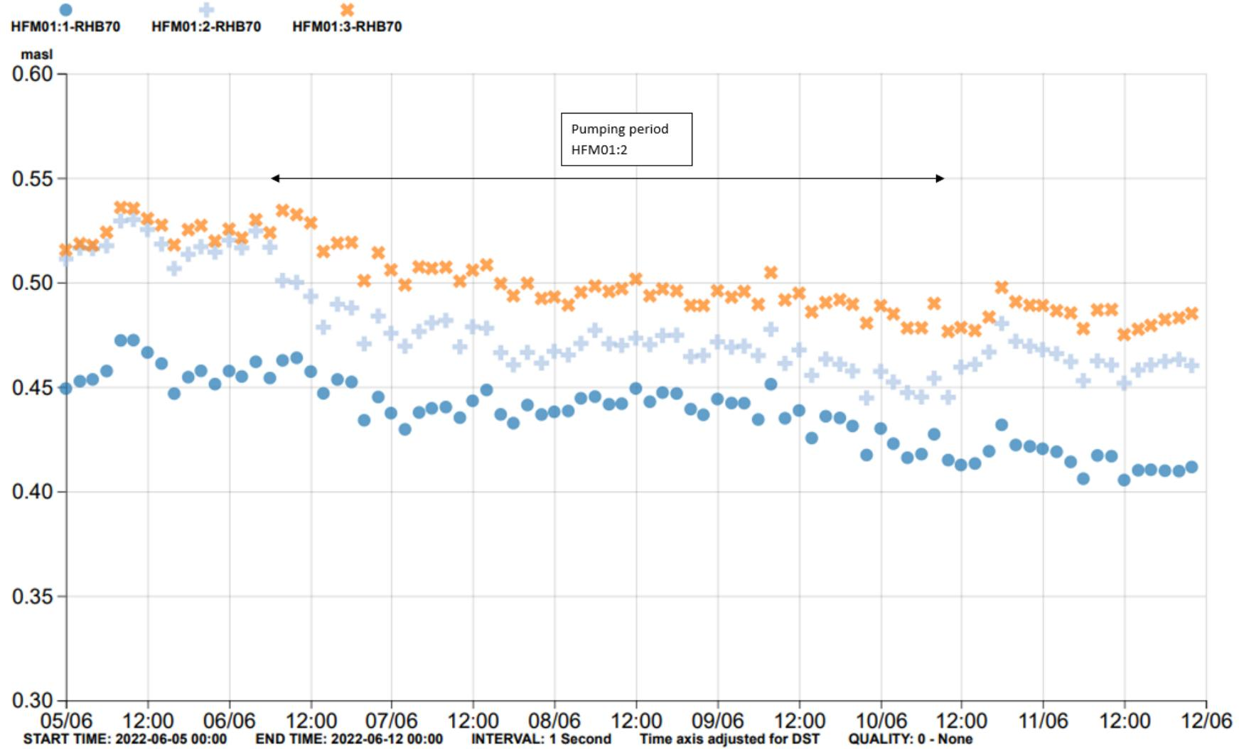
Figure A5-15. Pumping and drawdown in HFM01:2 in June 2022. No (?) sections were significantly affected by the pumping.
