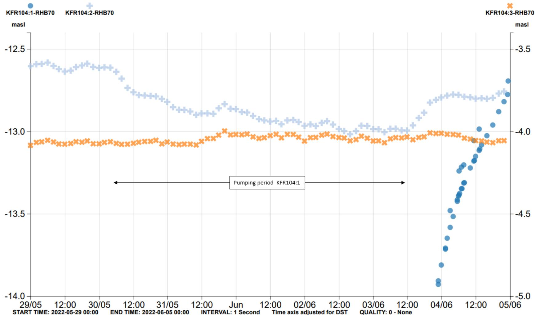
**Figure A5-26.** Pumping in KFR104:1 in May and June 2022. The pressure transducer in KFR104:1 was removed during the pumping. A response can be seen in section KFR104:2. Note the different scales for the respective borehole sections.
