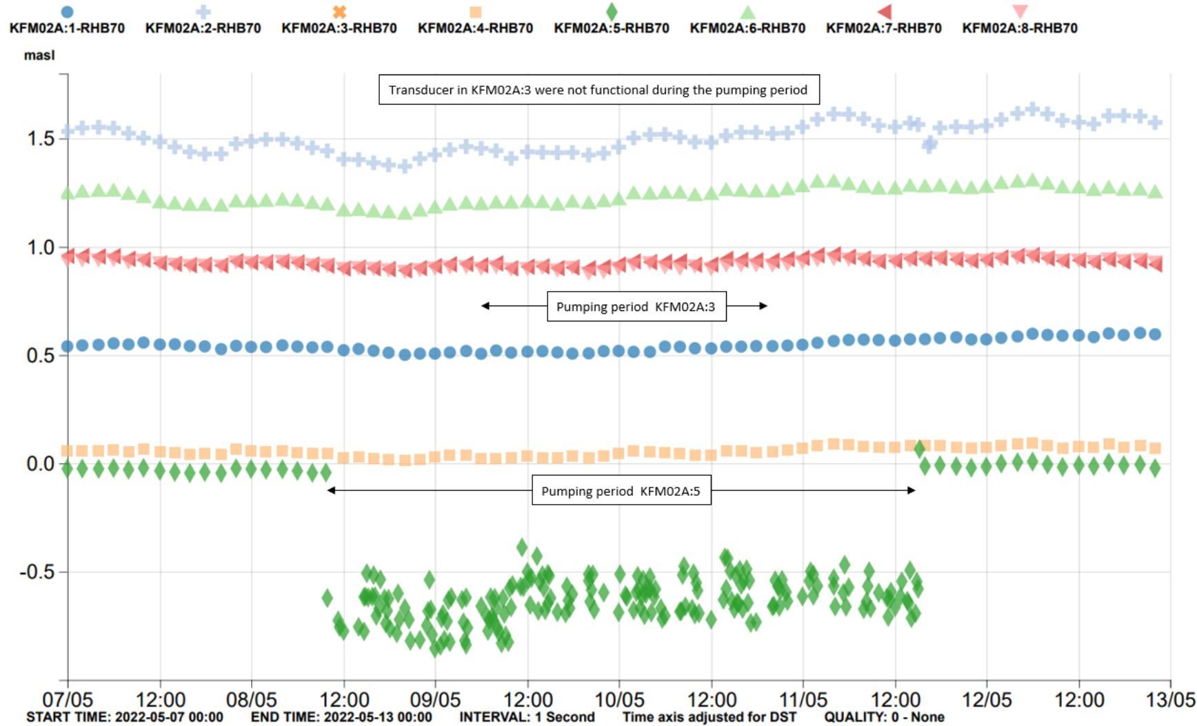
Figure A5-4. Pumping and drawdown in KFM02A:3 and KFM02A:5 in May 2022. No other sections were affected.
