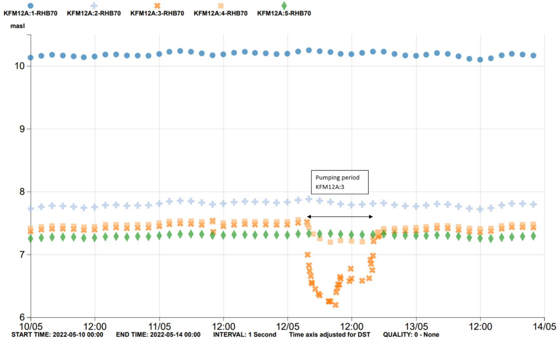
Figure A5-14. Pumping and drawdown in KFM12A:3 in May 2022. The pumping in section KFM12A:3 caused a response in KFM12A:4.
