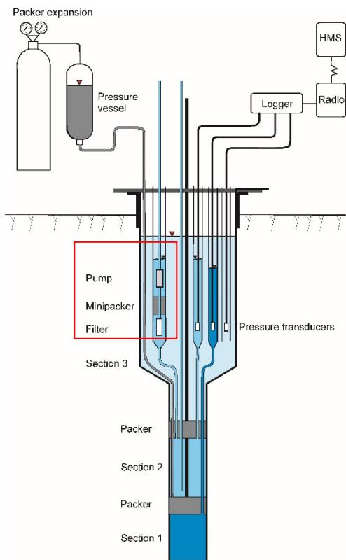
**Figure 2-1.** Installations in a borehole test section with connected standpipes and monitoring equipment. The installation is permanent in the borehole, except for the pump and filter (marked with the red box), which are used in the standpipe at the pumping/sampling occasions.
