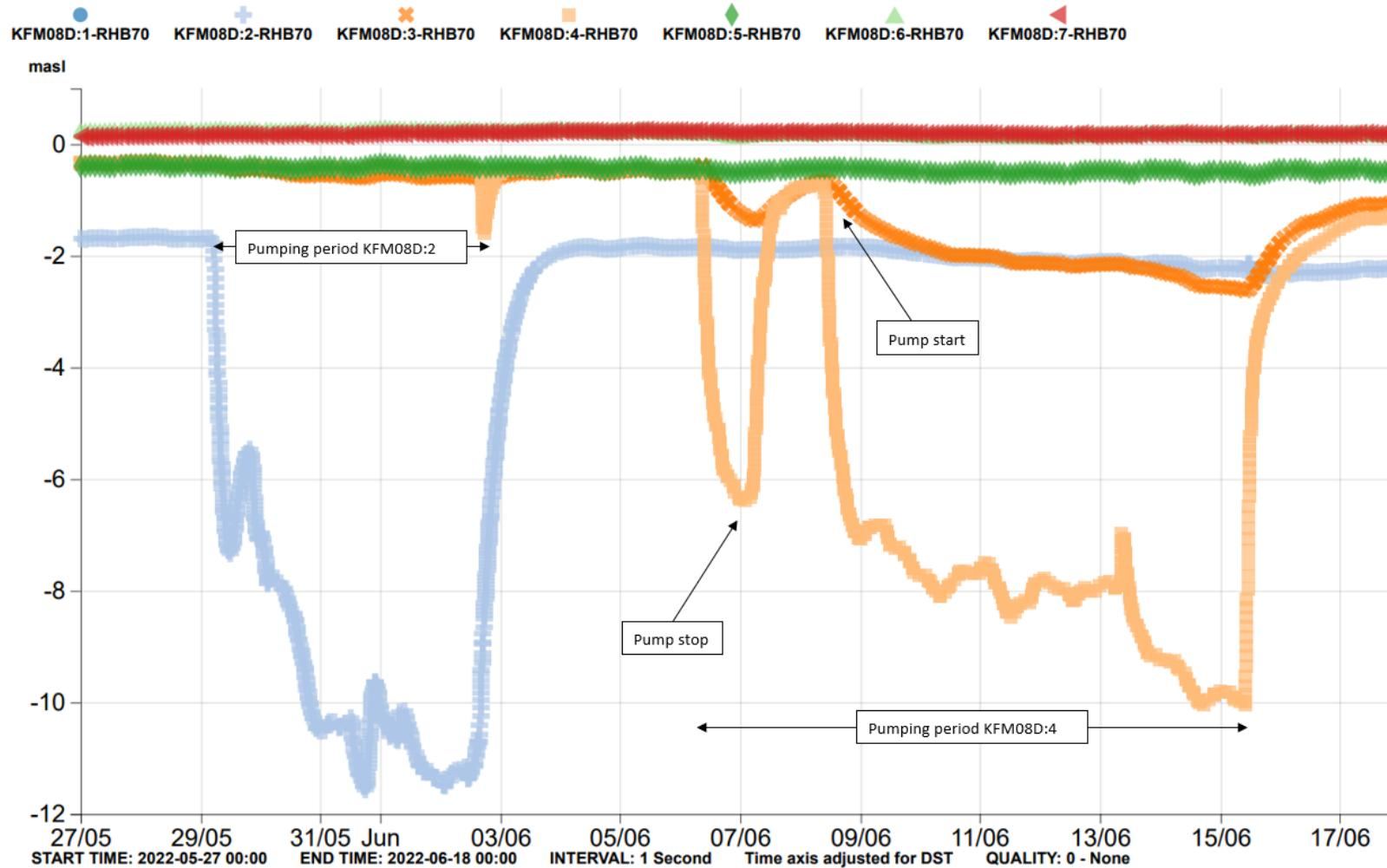
**Figure A5-12.** Detailed plot of pumping and drawdown in KFM08D:2 and KFM08D:4 in May and June 2022. Pumping in KFM08D:2 caused a small response in KFM08D:3. The pumping in section KFM08D:4 causes a response in KFM08D:3 and KFM08D:2. The pumping rate in both sections had to be adjusted several times which could be seen in the graph.
