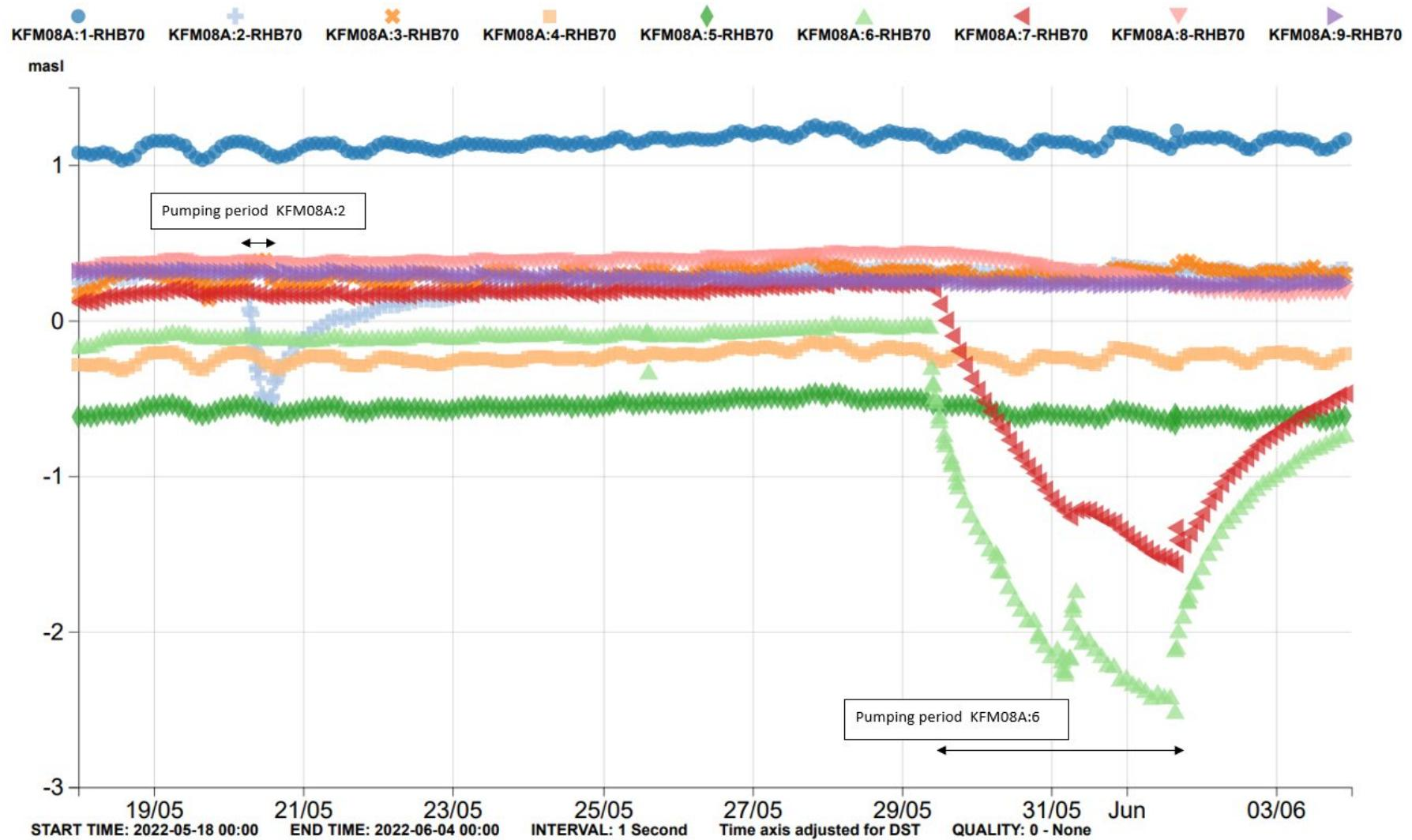
Figure A5-11. Detailed plot of pumping and drawdown in KFM08A:2 and KFM08A:6 in May and June 2022. The pumping in section KFM08A:2 caused an inverted (increase in pressure) response in KFM08A:3. Pumping in section KFM08A:6 caused responses in KFM08A:7 and KFM08A:8.
