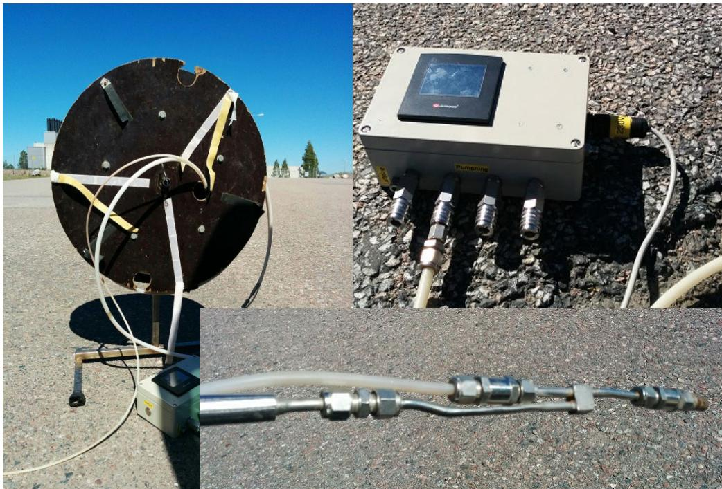
**Figure 2-5.** The equipment used for gas-lift pumping. To the left, the tubing lowered down the standpipe (the narrower tube for sample water and the wider for gas) on a bobbin to simplify the lowering. To the upper right the control unit for the pumping/gas supply and lower right the end of the gas-lift pump.
