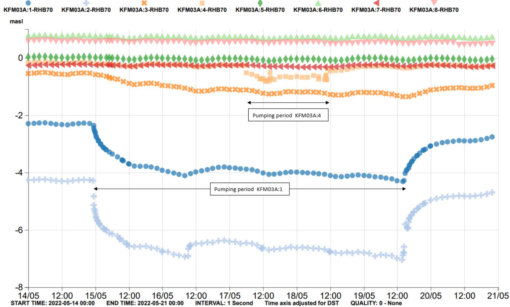
**Figure A5-6.** Pumping and drawdown in KFM03A:1 and KFM03A:4 in May 2022. The pressure response observed in KFM03A:2 during pumping in KFM03A:1 may be caused by a leaking connection in the equipment between sections KFM03A:1 and KFM03A:2 rather than a connected fracture system. A response to the pumping in KFM03A:1 was also seen in KFM03A:3.
