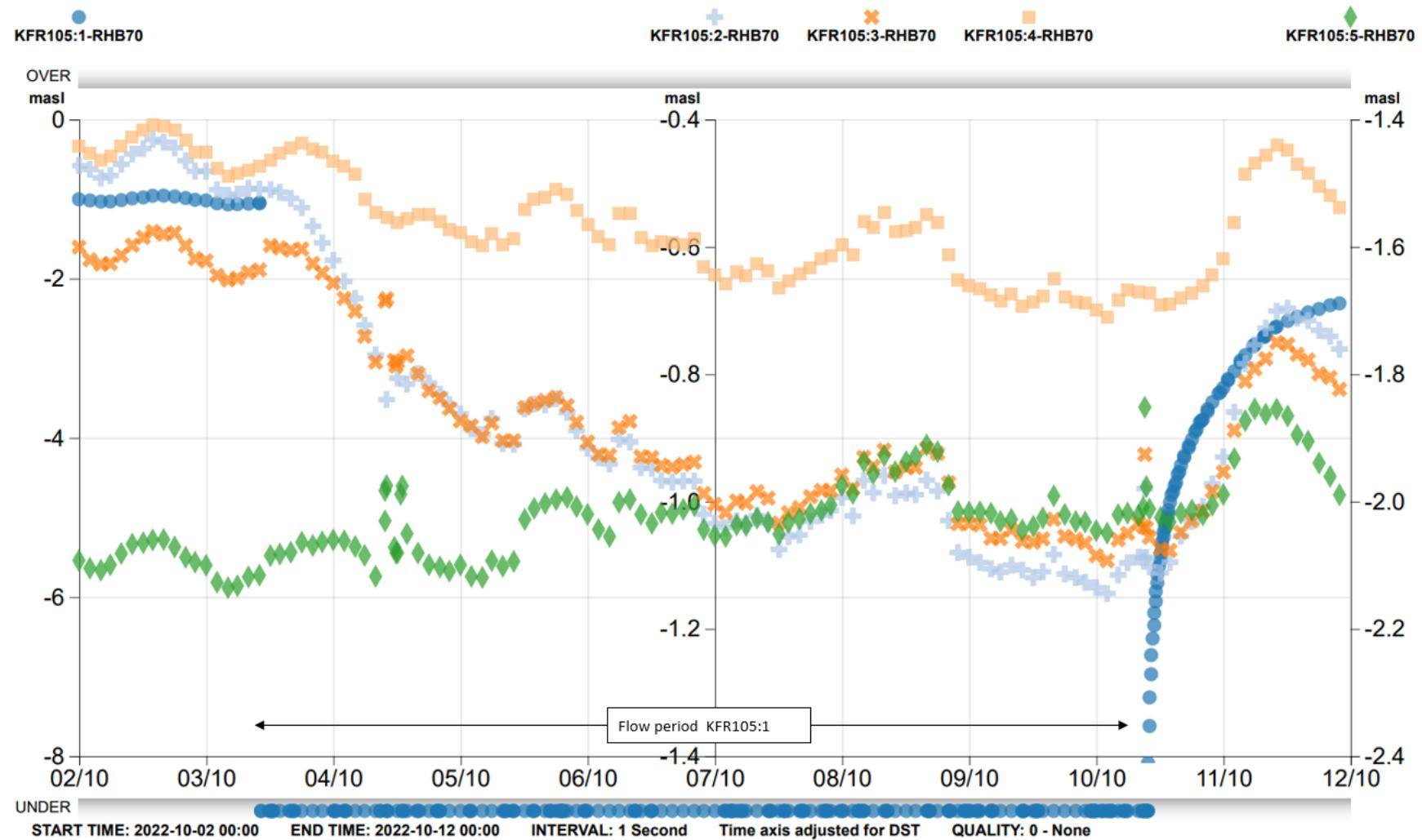
**Figure A5-27.** Flow period in KFR105:1 in October 2022. The efflux in KFR105:1 caused responses in KFR105:2, KFR105:3 and KFR105:4. Note the different scales for the respective borehole sections.
