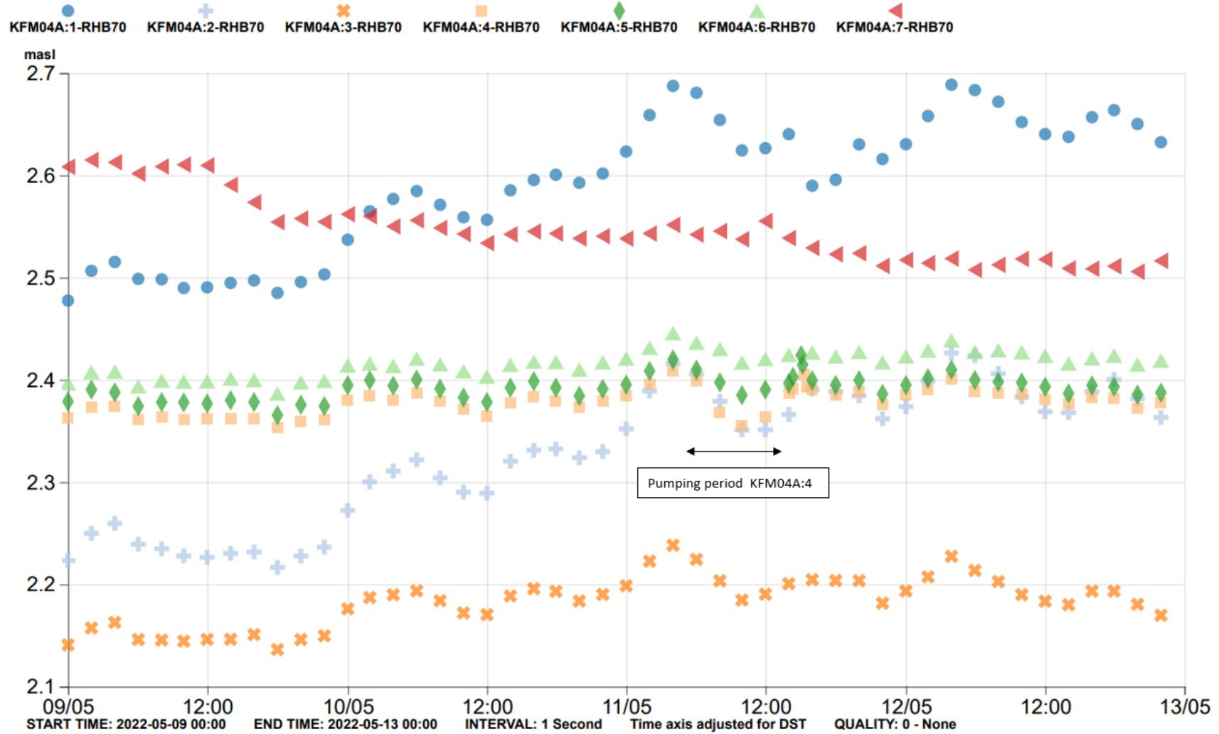
**Figure A5-7.** Pumping and drawdown in KFM04A:4 in May 2022. No (?) sections were significantly affected by the pumping.
