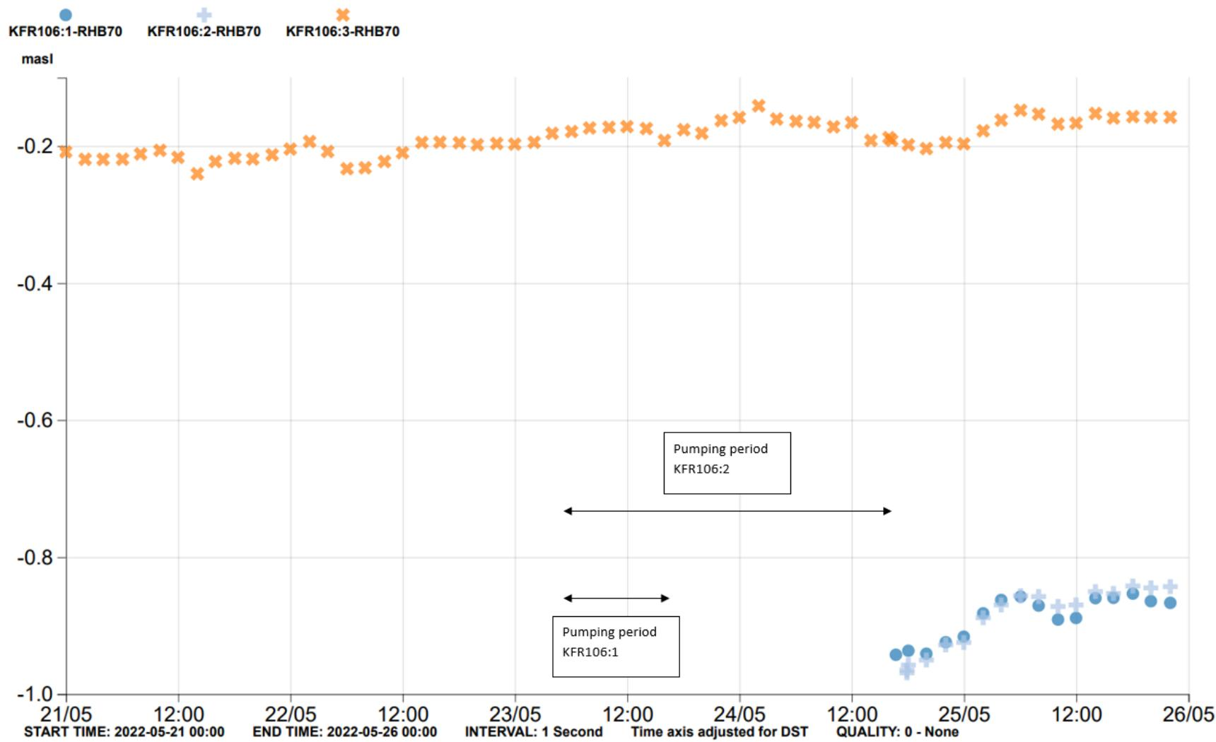
Figure A5-28. Pumping in KFR106:1 and KFR106:2 in May 2022. The pressure transducers in the pumped sections were removed during the pumping. KFR106:3 was not affected.
