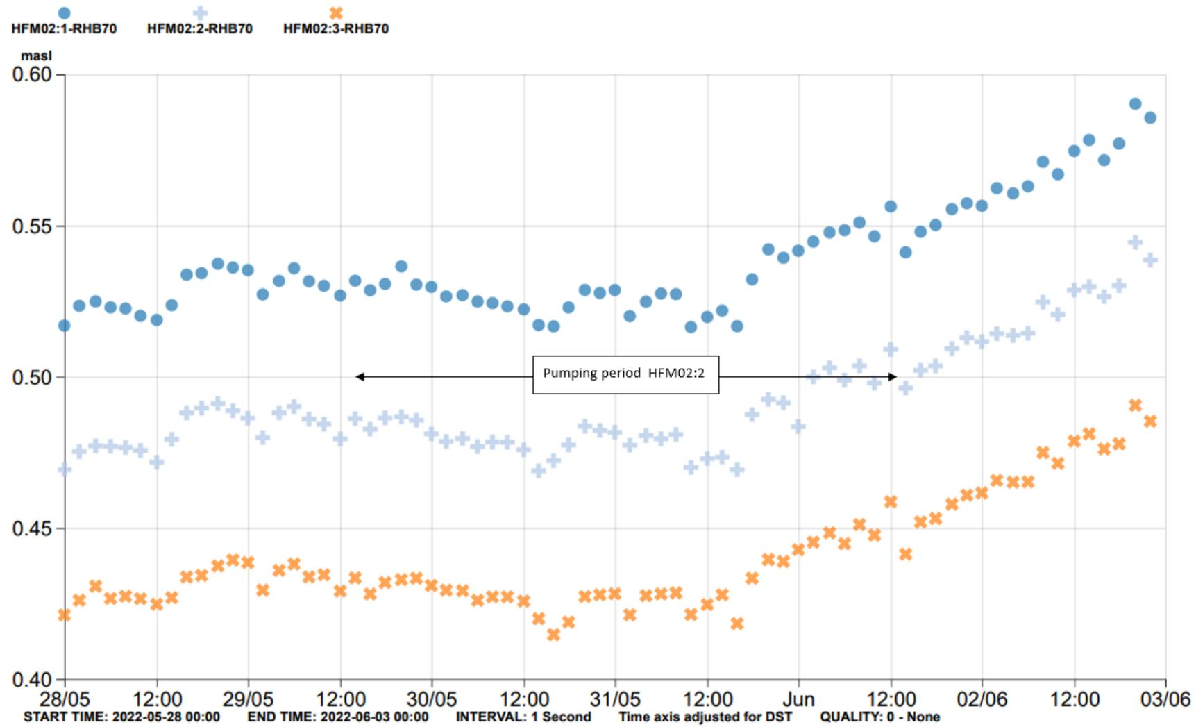
**Figure A5-16.** Pumping in HFM02:2 in May and June 2022. No significant drawdown was observed in any of the borehole sections.
