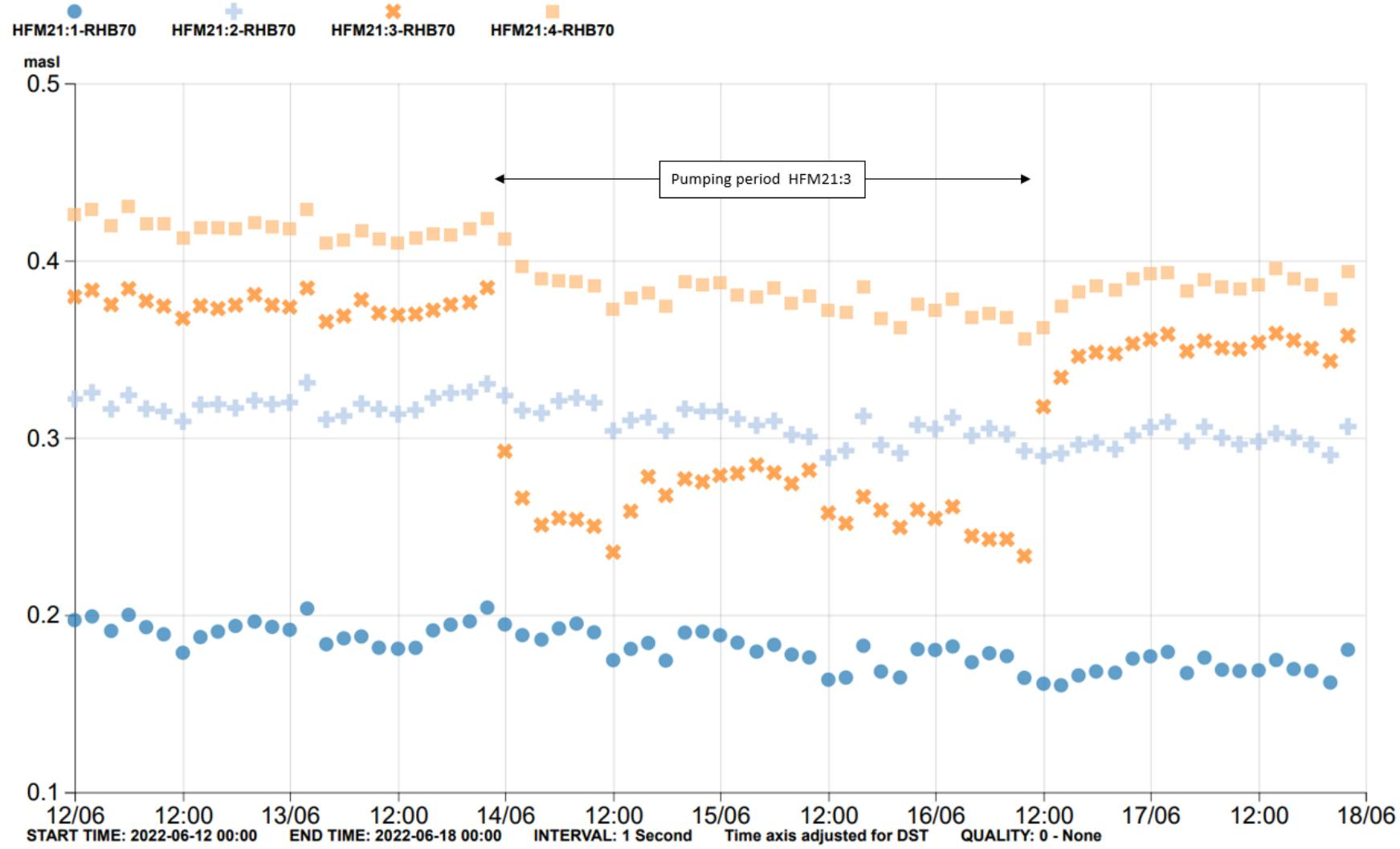
**Figure A5-21.** Pumping in HFM21:3 in June 2022. A small drawdown was observed in HFM21:4.
