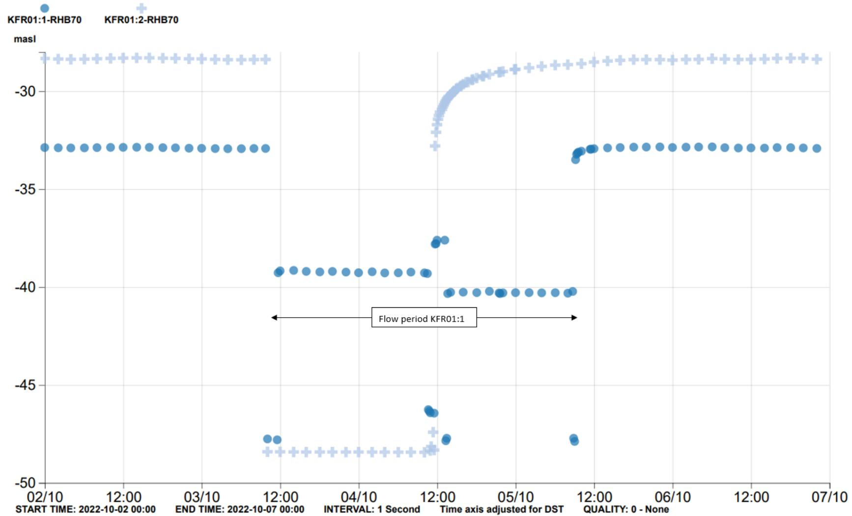
Figure A5-29. Flow period in KFR01:1 in October 2022. The response in KFR01:2 was affected due to the valve to the section being open 3/10-4/10 in another sampling campaign.
