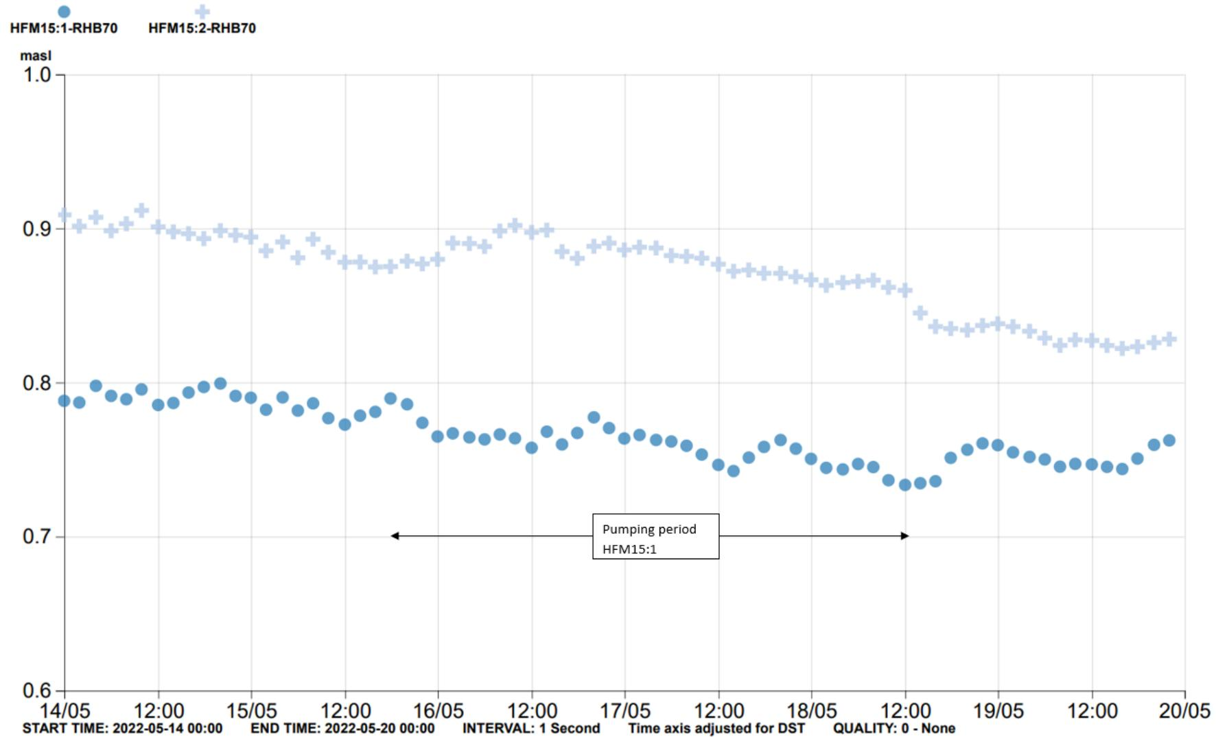
*Figure A5-19.* Pumping in HFM15:1 during May 2022. No significant drawdown was observed in any of the borehole sections.
