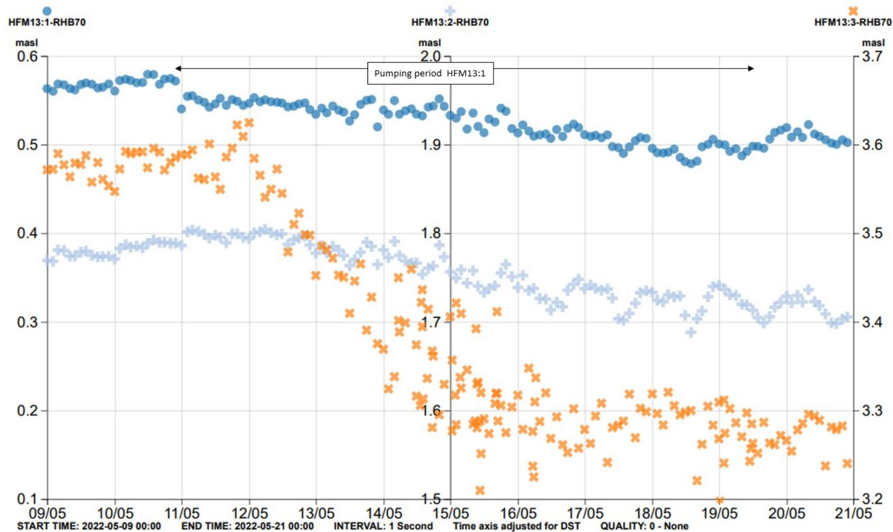
Figure A5-18. Pumping in HFM13:1 in May 2022. No (?) sections were significantly affected by the pumping. Note the different scales for the respective borehole sections.
