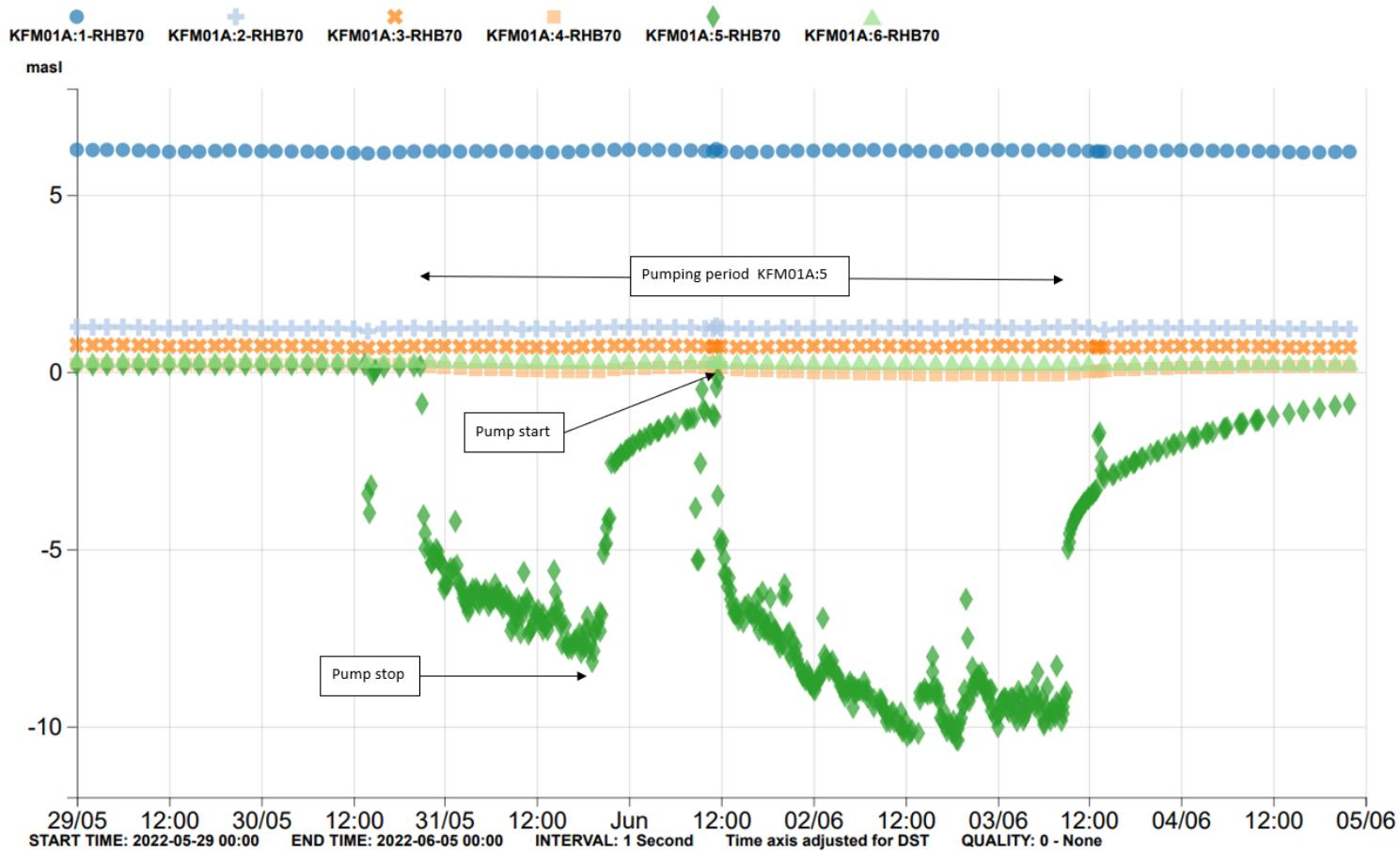
Figure A5-1. Pumping and drawdown in KFM01A:5 in May and June 2022. A small response was observed in 4. During the pump period a pump stop occurred.
