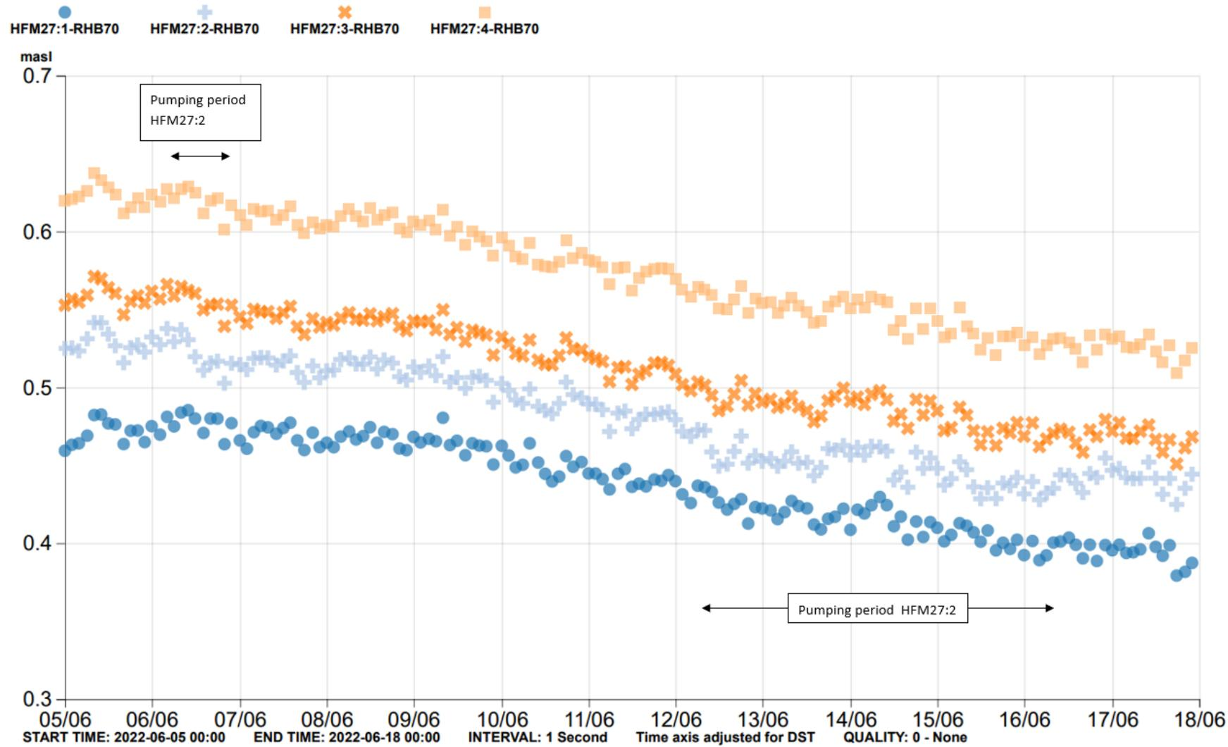
Figure A5-22. Pumping in HFM27:2 in June 2022. No significant drawdown was observed in any of the borehole sections.
