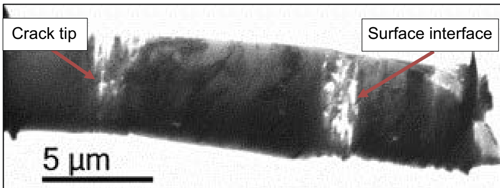
Figure A-12. High Resolution TEM image of lamella from Rod #4. The left side corresponds to the crack tip interface, while the right side corresponds to the surface interface between metallic copper and corrosion products.
