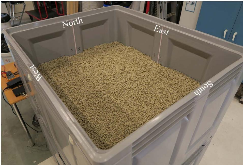
**Figure A-13.** Photographic images of test 06 at the end of the test after 40.0 hours. Wetting did not reach the top of the pellet surface during the test.
