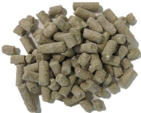
*Figure A-1. Extruded 6 mm rod-shaped Cebogel QSE pellets as received.*
