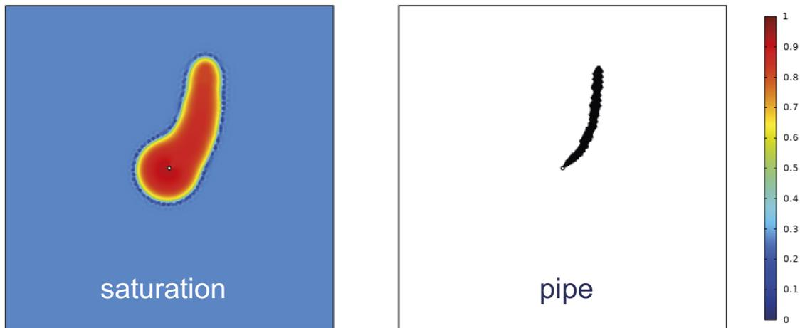
**Figure 4-8.** Total saturation and pipe state variable after 80 h in the piping channel formation test.
