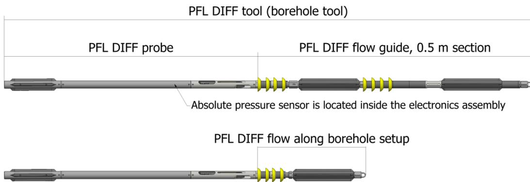
Figure 3-1. Technical illustration of the PFL DIFF probe in different setups.
