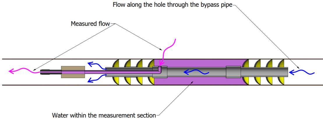
**Figure 3-3.** The absolute pressure sensor is located inside the electronics assembly and connected to the measurement section through a tube.
