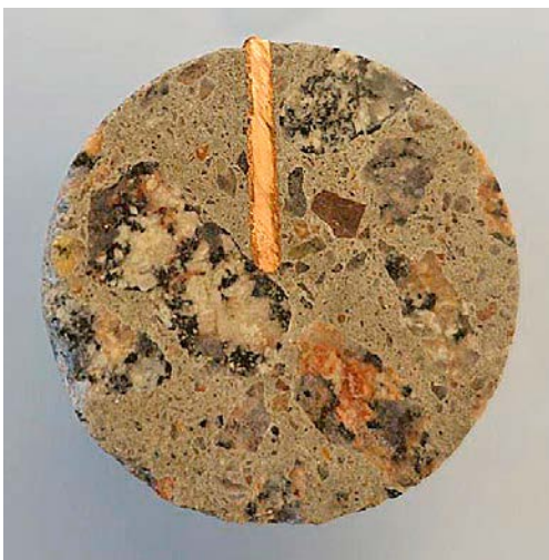
Figure 7-6. Core containing a joint seal. Note that it was not possible to prepare specimens where the 2 halves of the specimen were completely separated by the joint seal as this caused the specimen to split.
