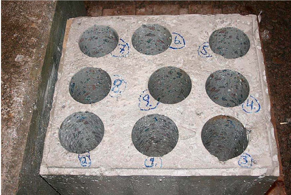
Figure 5-17. The small cube cast from concrete from truck #7 after drilling of cores for testing of compressive and tensile strength. Numbers refer to specimens numbers in Table 5-6 and 5-7.
