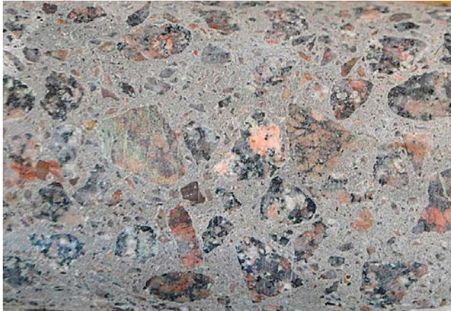
Figure 7-3. Particle distribution in the concrete from core TAS05_08. This image is from the inner part of the core, approximately 500 mm from the surface of the concrete structure.
