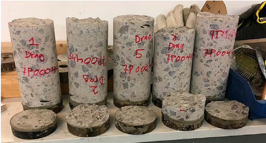
Figure 5-18. Cores used for measurements of tensile strength after testing.
