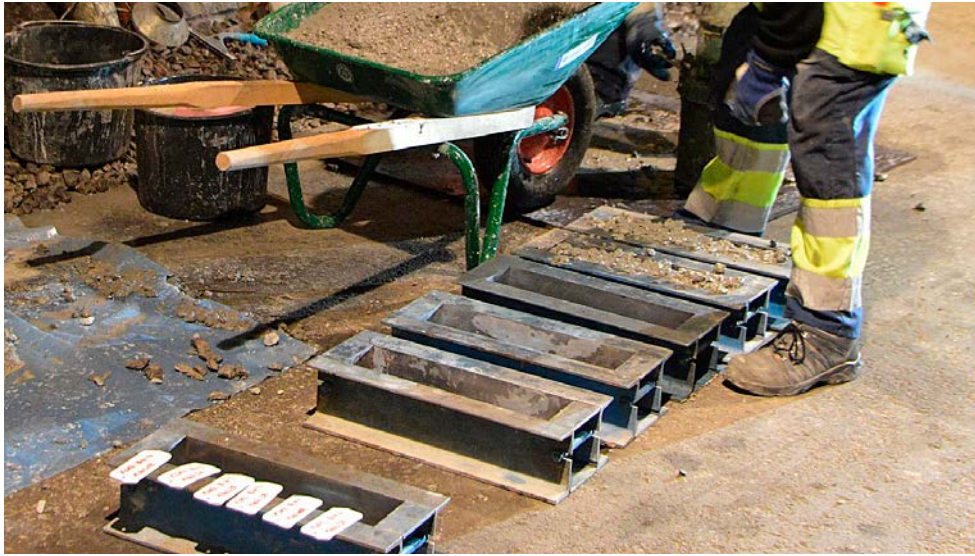
Figure 5-20. Casting of specimens for shrinkage measurements.
