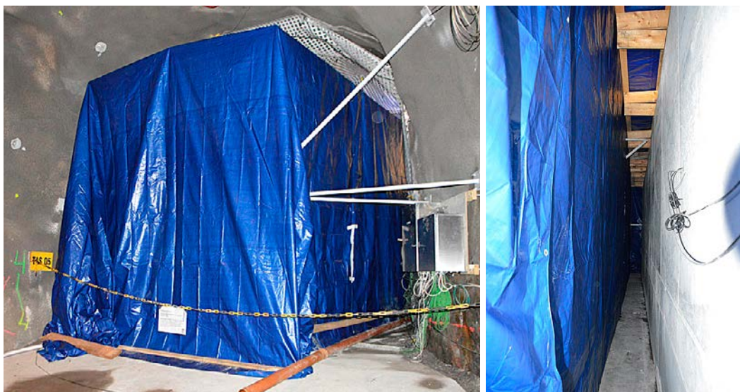
Figure 10-1. The tent covering the concrete structure during the stress test.
