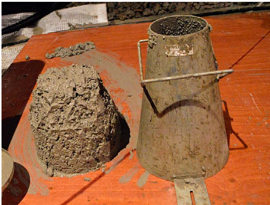
Figure 5-8. A typical example of a stiff concrete from one of the concrete trucks prior to adjustments.
