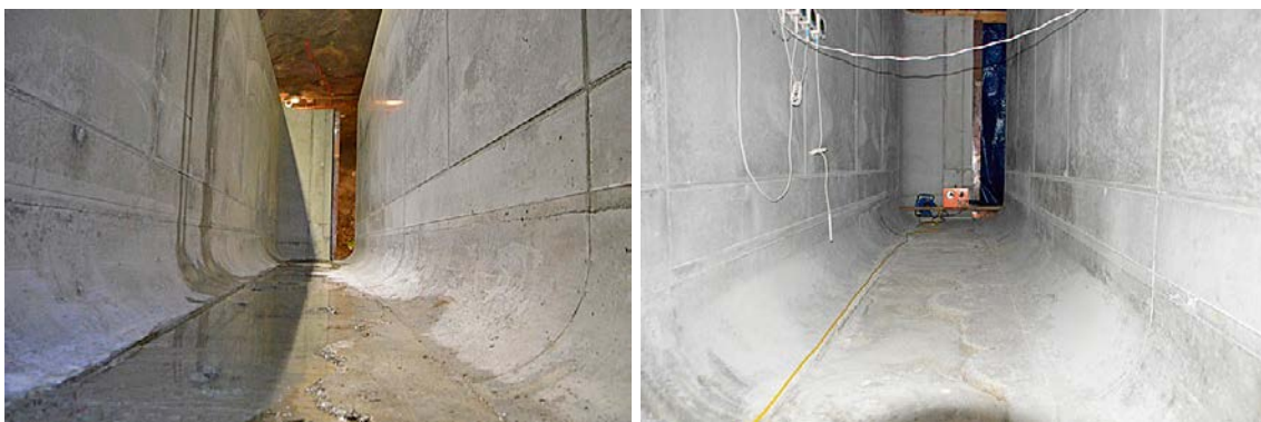
Figure 10-2. The space between section 1 and section 2 prior to start of stress test (Left image) and about 1 month after the start of the stress test (Right image).
