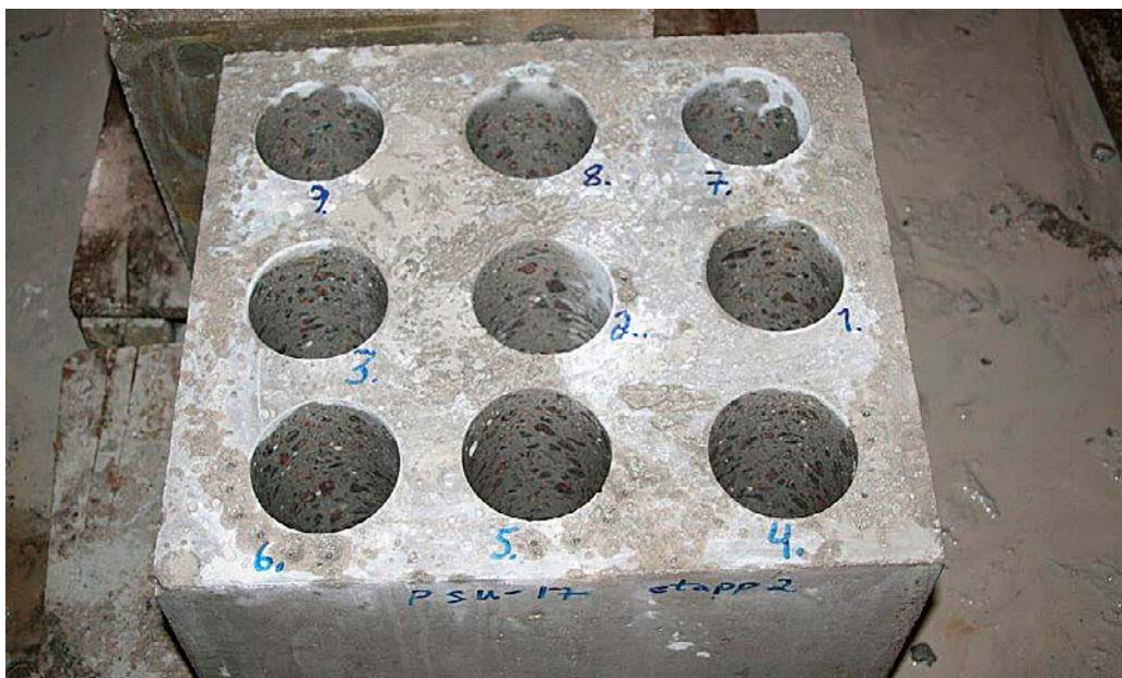
Figure 6-9. The small cube cast from concrete from truck #4 after drilling of cores for testing compressive and tensile strength. Numbers refer to specimens numbers in Table 6-5 and 6-6.
