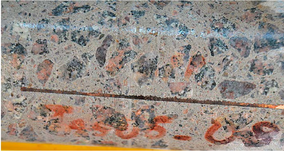
Figure 7-5. Image showing the contact zone between concrete and joint seal from core TAS05_08.
