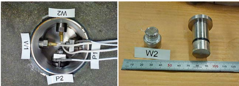
Figure A4-3. Photos of the inner cylinder with attached sensors W1, W2, P1 and P2 (to the left) and of the casing used for the W2-thermocouple psychrometer and one of the pistons used for stress measurement P1 and P2 (to the right).
