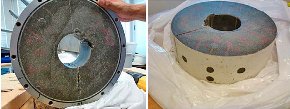
Figure A4-5. Photos of the bentonite ring after dismantling of SH1. The bentonite ring, still inside the steel device but without the inner steel ring, sawn radially and with the sampling marked on the upper surface (to the left) and the dismantled bentonite ring with the filter still left on the outer surface and the sampling marked on the bottom surface (to the right).
