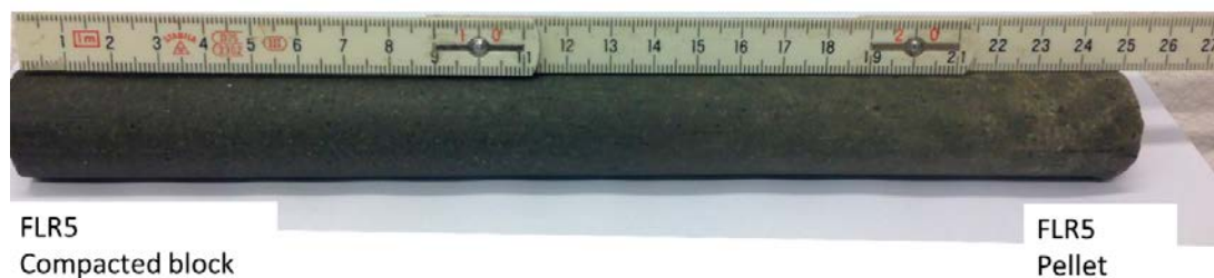
Figure 6-7. The dismantled specimen FLR5.
