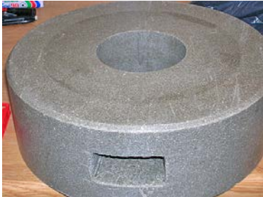
Figure A4-1. Photo of cylinder ring with cavity used for test SH1.
