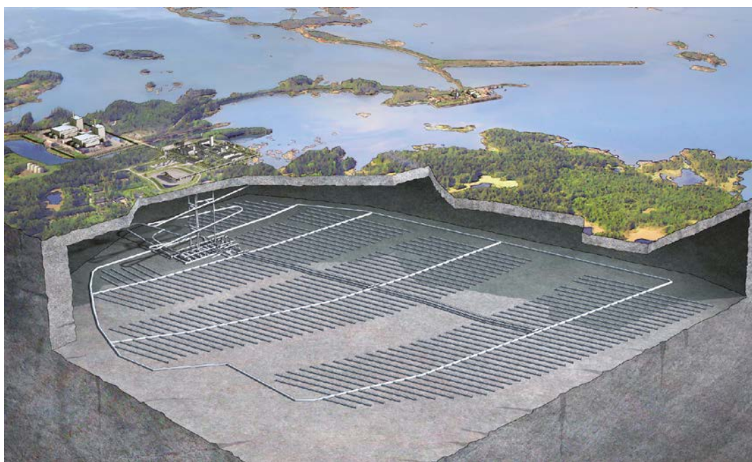
Figure 1-1. Illustration of a possible design of the Spent Fuel Repository at Forsmark.
