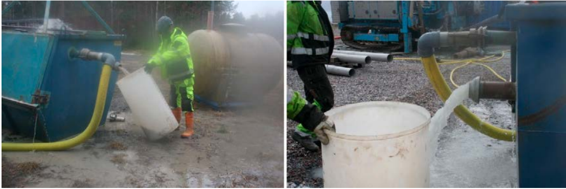
Figure 5-9. Left: In HFM43 the water inflow was measured with a stopwatch and a 200 L measuring vessel. A water inflow of 600 L/min was observed at 114 m drilling length. Right: In HFM44 the accumulated water increased to 500 L/min at 164 m drilling length.
