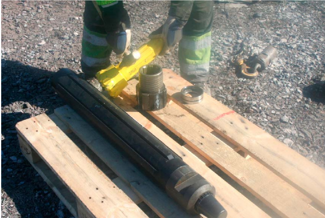
Figure 3-2. The downhole borehole equipment used is aimed for drilling straight boreholes. By using a precision hammer and a centralizer, combined with always starting a new borehole with a new drill bit gives best opportunities to obtain straight boreholes.
