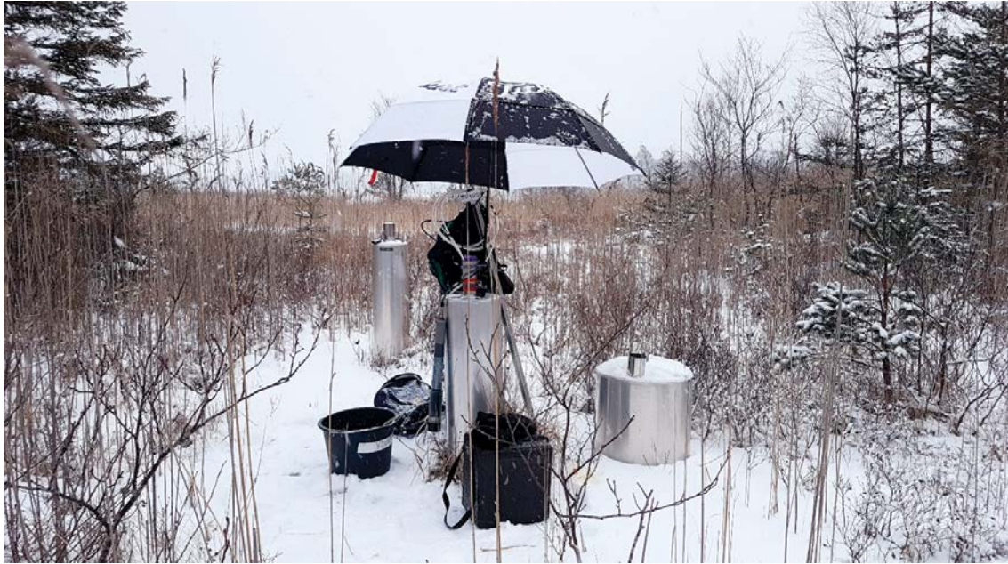
Figure 2-5. Winter sampling of near surface groundwater at the sampling well SFM0032.
